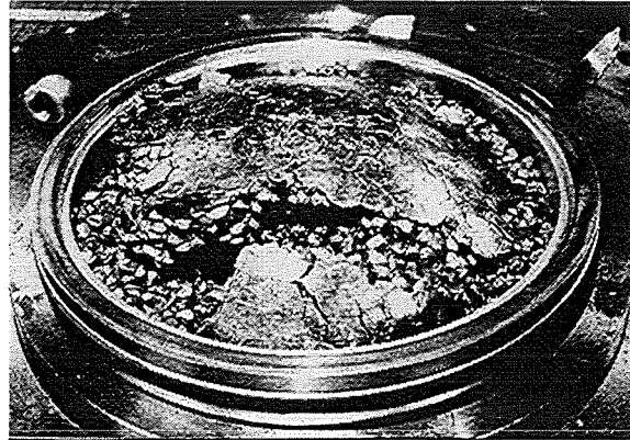
Fig. 4: Test02, plastic deformations of the lead spheres after the impact.
