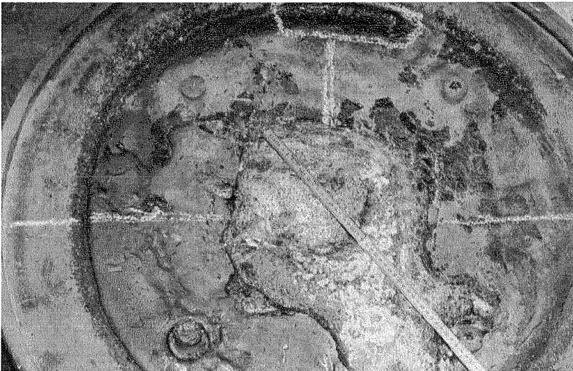
Fig. 2-11b: Test plate upper surface after removal of oxide: penetration remnants and solidified inconel cake (04/1)
