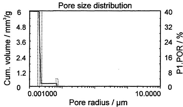
**FIGURE 8: Liquid mercury porosimetry histogram. Pore radius versus cumulative volume for a UO<sub>2</sub> sintered and non-irradiated sample.**
