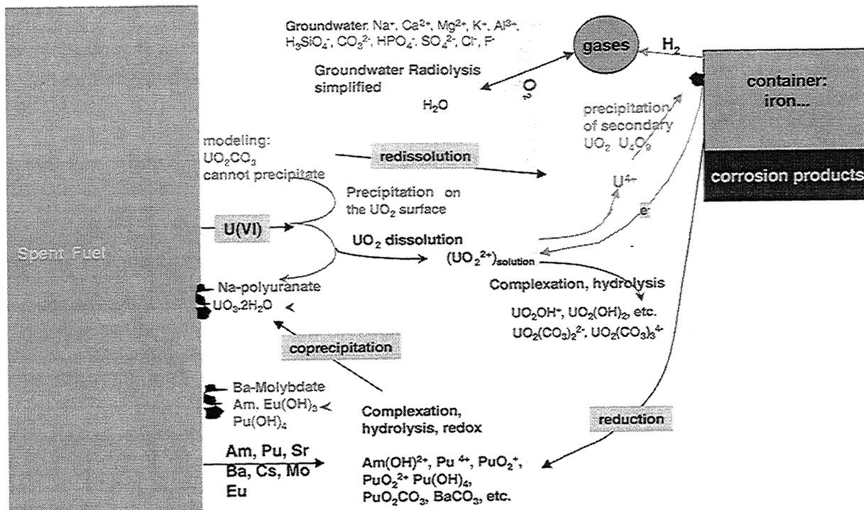
FIGURE IV.4-3. Simplified Spent fuel alteration mechanisms for reaction path modelling
