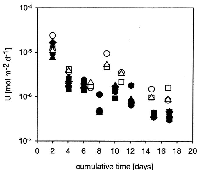
**FIGURE I.4-1. Dissolution rates of uranium from UO<sub>2</sub> pellets during the predissolution period in saline groundwater under anaerobic conditions (N<sub>2</sub>) (filled symbols: S/V= 6.6 m<sup>-1</sup>, open symbols: S/V= 19.8 m<sup>-1</sup>).**
