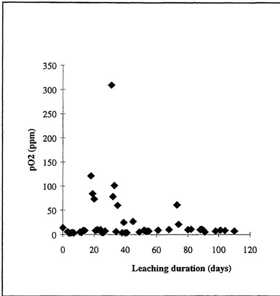
**FIGURE 7 :** Oxygen partial pressure in Ar/CO<sub>2</sub> glove box during dissolution tests.
