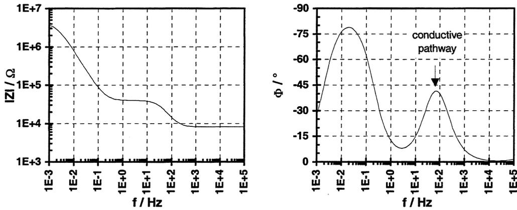
FIGURE. I.6.4: Calculated impedance spectrum of an equivalent circuit of a fuel electrode with conductive pathways ( $R_{\text{bulk}} = 40 \text{ k}\Omega$ ,  $C_{\text{bulk}} = 5 \text{ pF}$ ,  $R_{\text{pol}} = 10 \text{ M}\Omega$ ,  $C_{\text{D}} = 20 \text{ }\mu\text{F}$ ,  $R_{\Omega} = 100 \text{ }\Omega$ ,  $R_{\text{Me,pol}} = 7 \text{ M}\Omega$ ,  $C_{\text{Me,dI}} = 0.1 \text{ }\mu\text{F}$ ,  $R_{\text{por}} = 10 \text{ k}\Omega$ ).
