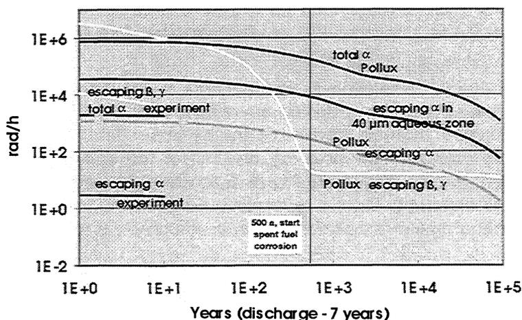
**FIGURE 1: Time dependence of dose rates from spent fuel in experiments (1g in 100 ml soln) and for a water filled Pollux container with 4 tons of fuel. Comparison of dose rates considering the total alpha events with dose rates from alpha events with in an escape depth of 10  $\mu m$  from beneath the fuel surface. Comparison to hypothetical irradiation of total water volume with irradiation of a volume given by the 40  $\mu m$  maximum pathway of alpha particles in water**
