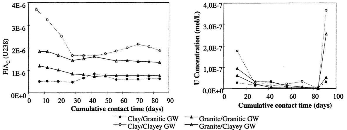
FIGURE III.3.7. Gravelines 3+2 spent fuel-leaching experiment: <sup>238</sup>U FIA<sub>c</sub> and solution concentrations of U versus cumulative leaching time, environmental materials and groundwater composition.
