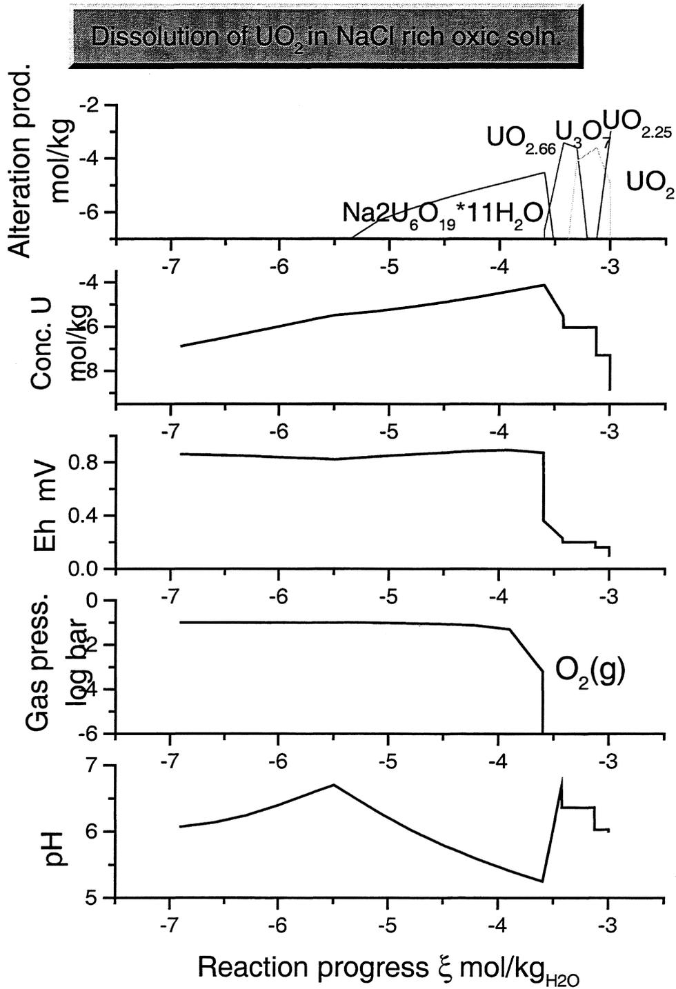
FIGURE IV.1.1: Geochemical simulation (code: EQ3/6) of the reaction path of  $\text{UO}_2$  in 95% saturated NaCl solution in equilibrium with air at 25°C.
