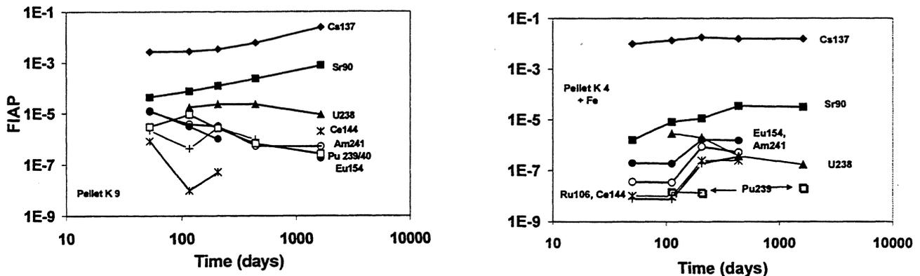
Figure III.1 -1: Effect of iron on the dissolution of spent fuel pellets in 5m NaCl-solution under anaerobic conditions: Sample K9, 1623 days (left), K4, 1619 days in the presence of 8,5 g Fe powder (right).
