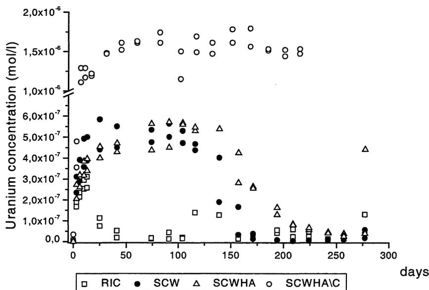
**FIGURE I.4-15: Uranium concentrations in the carbonate rich media and in the medium with low carbonate content as a function of time for the second test series**
