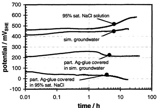
Fig. 15: Open circuit potentials of gold coated brass (MS58) in chloride containing media
