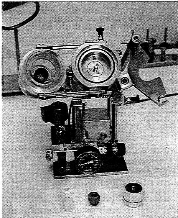
PE-bottle with special lid      electrode head      electrode head support
