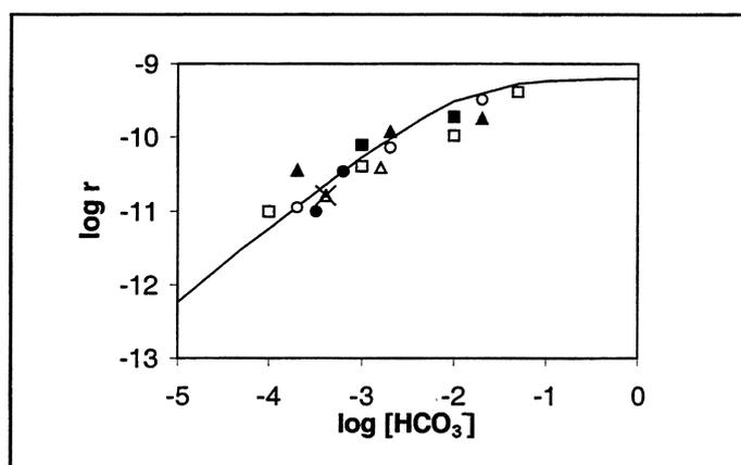
**FIGURE IV.1-7 Comparison between the results obtained by different authors using both spent fuel and unirradiated  $\text{UO}_2$  and the trend predicted by equation IV.1-7, represented by the solid line (■□ [97PAB/CAS], ○, ▲ [95GRA/WIL], ●, △ [89GRA], X this work: experiment UODGW25)**
