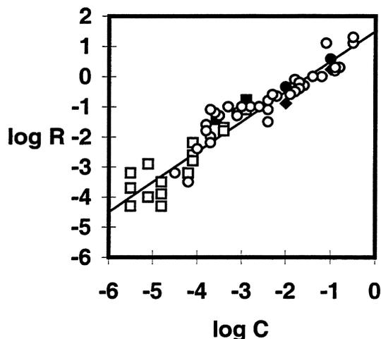
FIGURE 3 : Dissolution rates [mg/m<sup>2</sup>d] vs. Oxidant concentration [mol/l]. ■ O<sub>2</sub> ; □ O<sub>2</sub> and ○ H<sub>2</sub>O<sub>2</sub> ◆ H<sub>2</sub>O<sub>2</sub> and ● ClO<sup>-</sup>
