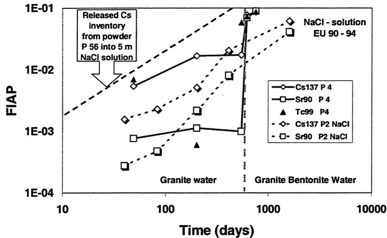
FIGURE I.1 - 10: Comparison of spent fuel powder corrosion data in salt and two granite media. Diagonal for NaCl-media (this project) indicates test P56 with probably oxidised powder
