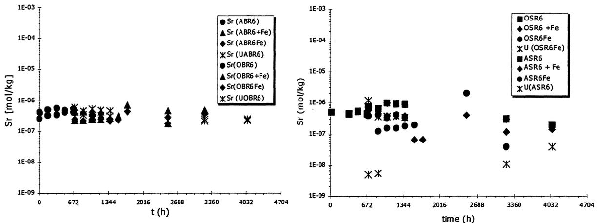
**FIGURE III.1-19 [Sr] vs. time in GBW and in 5 m NaCl for both oxidising and reducing low carbonate conditions. Fe is present in the system after 720 h leaching time**
