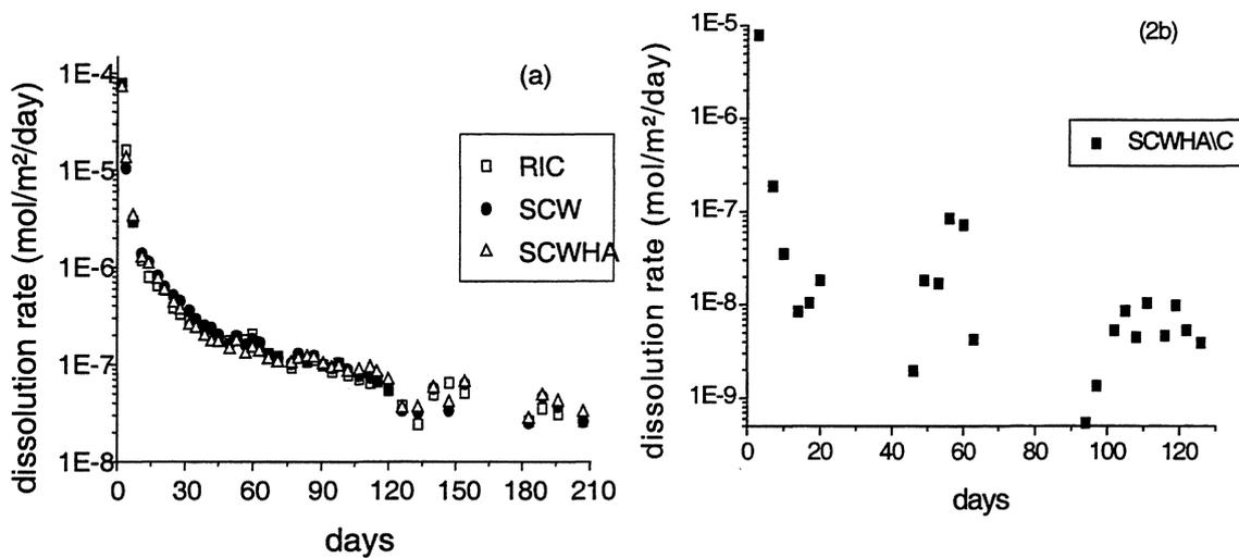
FIGURE I.4-14: UO<sub>2</sub> dissolution rate during the predissolution of the second test series in the carbonate rich media (a) and in the low carbonate medium (b).
