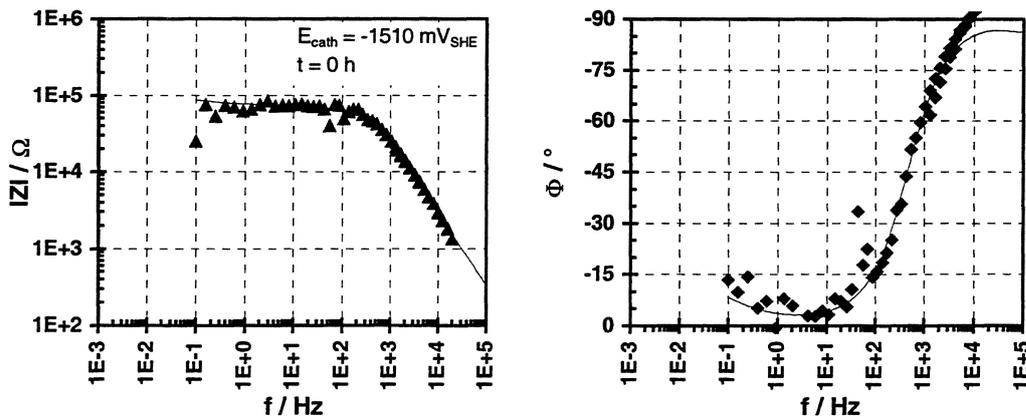
FIGURE I.6.25: EIS spectrum measured during pre-cathodisation of fuel B2 in 95% sat. NaCl solution.
