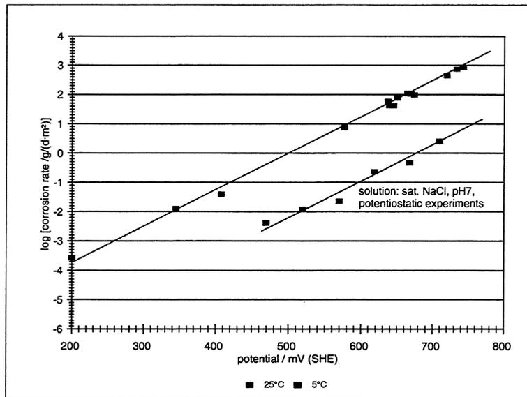
FIGURE I.6-37: Calibration curves for corrosion on  $\text{UO}_2$  in sat. NaCl solution at 25 and 90°C
