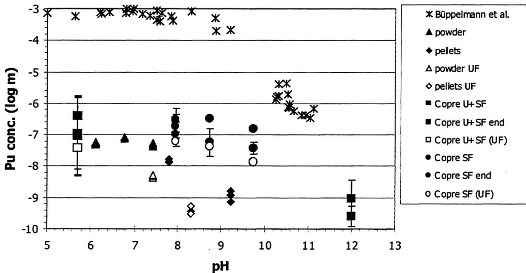
FIGURE II.1.3 Pu conc. from SF, SIMFUEL experiments in saline solutions
