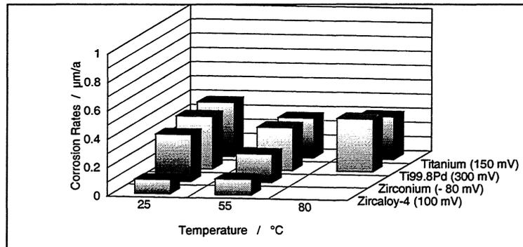
FIGURE I.8-2: Corrosion rates of Zirconium and Titanium at corrosion potential
