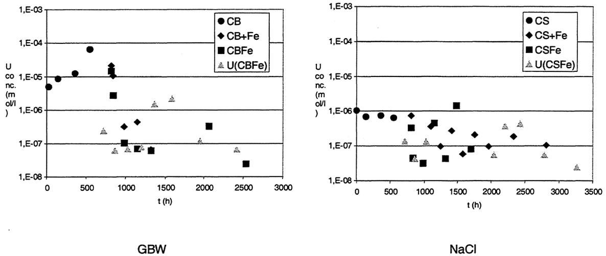
FIGURE III.1-17 [U] against time under  $N_2/CO_2$  ( $p_{f_{CO_2}}=2$ ) atmosphere for both, GBW and NaCl leachants. Fe is present in the system after 720 h leaching time.
