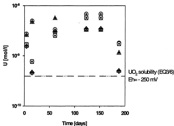
FIGURE III.1-11 Measured uranium concentration (Non-filtered) in anaerobic Allard groundwater ( $\text{N}_2$ ) in the presence of metallic Fe. Solution concentrations in  $0.45\ \mu\text{m}$  filtrates were below the detection limit
