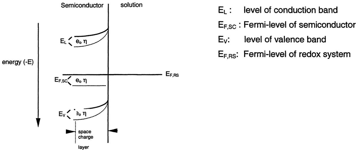
**FIGURE I.6-29: Shift of Fermi-level  $E_{F,SC}$  and conductivity and valence bands in contact with an electrolytic system in absence (solid lines) and presence of applied anodic overvoltage (dashed line)**
