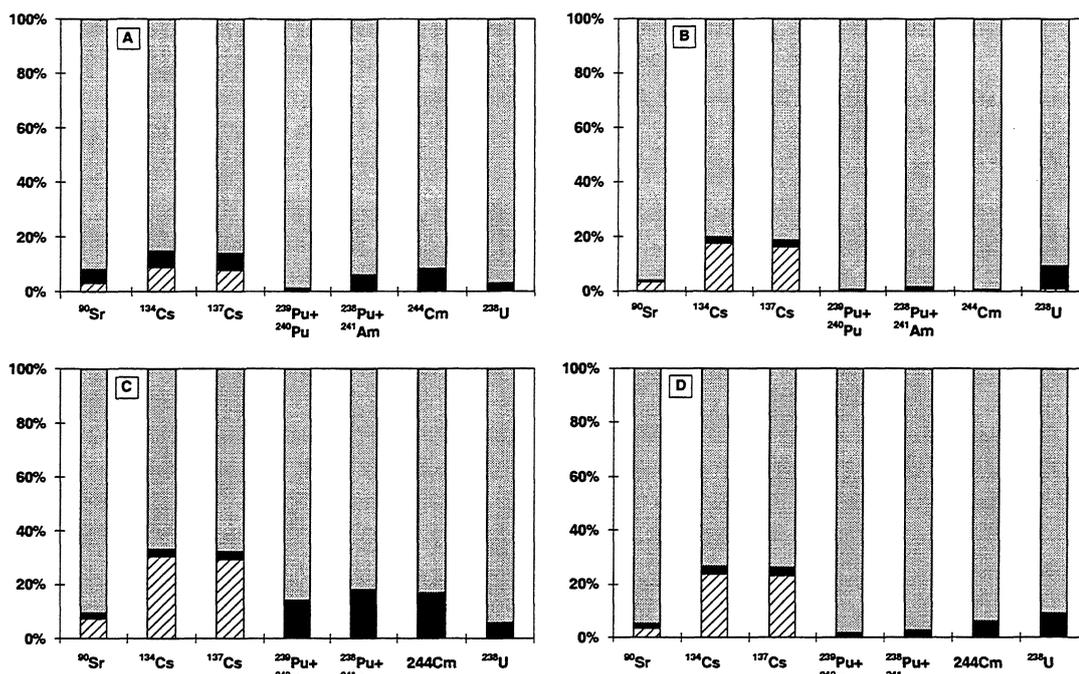
FIGURE III.3.10. Interaction between spent fuel and environmental materials. A: C/GW medium. B: C/CW medium. C: G/GW medium. D: G/CW medium. Key: *Hatched bars*: Aqueous phase inventory fraction; *Dark bars*: Sorbed inventory fraction; *Light bars*: Inventory fraction fixed on environmental materials
