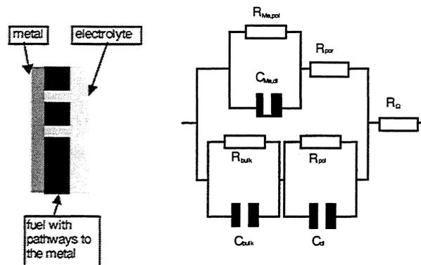
FIGURE. I.6.2: Equivalent circuit of a fuel electrode with conductive pathways like unsealed cracks and/or pores between metal support and electrolyte solution. At the metal/electrolyte interface at the bottom of the pathway an additional polarization resistance  $R_{\text{Me, pol}}$  and a double layer capacitance  $C_{\text{Me, dl}}$  correlated with metal corrosion is expected.  $R_{\text{por}}$  represents resistance of the pathway.
