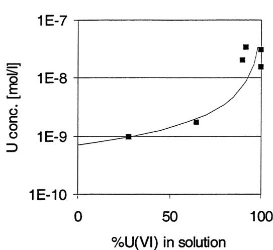
FIGURE I.4-16, dependency of UO<sub>2</sub> solubility under reducing conditions on the experimentally measured U(VI) content in solution.
