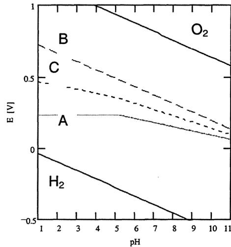
**FIGURE IV.1-4:  $\text{UO}_2$  dissolution,  $\log p\text{O}_2=-29$ ,  $\text{HCO}_3=0$ , pH dependency of (A) equilibrium ref. potential of anodic and (B) cathodic half reaction ( $=E_h$ ) (C) corrosion potential**
