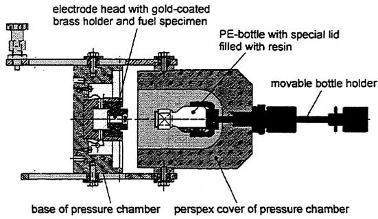
**Fig.I.6.17: Schematic diagram of the impregnation chamber.**
