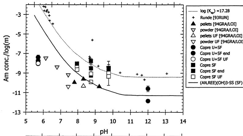
FIGURE IV.2-1 Solubility of Am in case of ideal solid solution formation  $(\text{AN,REE})(\text{OH})_3(\text{s})$ .
