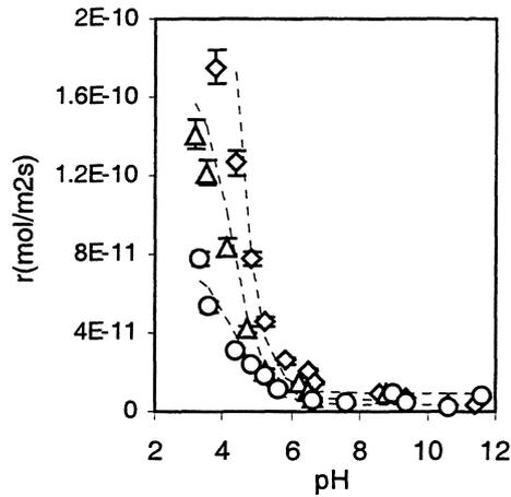
FIGURE 4: Dissolution rates vs. pH. O<sub>2</sub> pressure: ○ 5%; △ 21%; ◇ 100%
