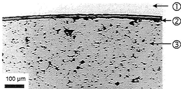
FIGURE. I.6.12: Micrograph of  $\text{UO}_2$  fuel with a burn-up of 53 GWd/t (1: cladding, 2: gap, 3: fuel)
