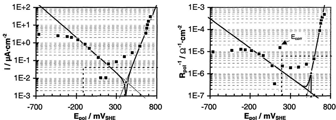
Fig. 1: Potentiostatic polarisation curves obtained from unirradiated  $UO_2$  in air saturated 95% saturated NaCl solution ( $T = 22^\circ C$ ,  $C(O_2) = 7.4$  ppm, initial pH 7.1,  $t_{pol} = 10$  min,  $A_{el} = 0.478$  cm<sup>2</sup>,  $d_{el} = 1.5$  mm).
