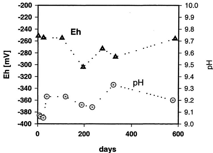
**FIGURE 1.** The measured Eh and pH values in a parallel sample of saline groundwater with 3 ppm S(-II) during a follow-up period of 600 days under anaerobic conditions.
