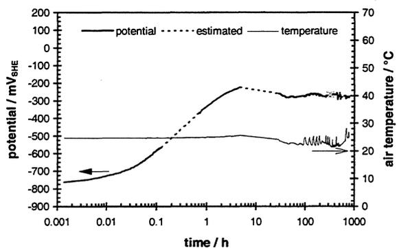
Fig. 14: Open circuit potential of used MOX fuel (burn-up: 21.1 GWd/t) and related temperature, in 95% saturated NaCl solution ( $E_{corr}^{max} = -256 \text{ mV}_{SHE}$ ,  $T: 22 - 28^\circ\text{C}$ ,  $C(\text{O}_2) < 2 \text{ ppm}$ , initial pH 7.2)
