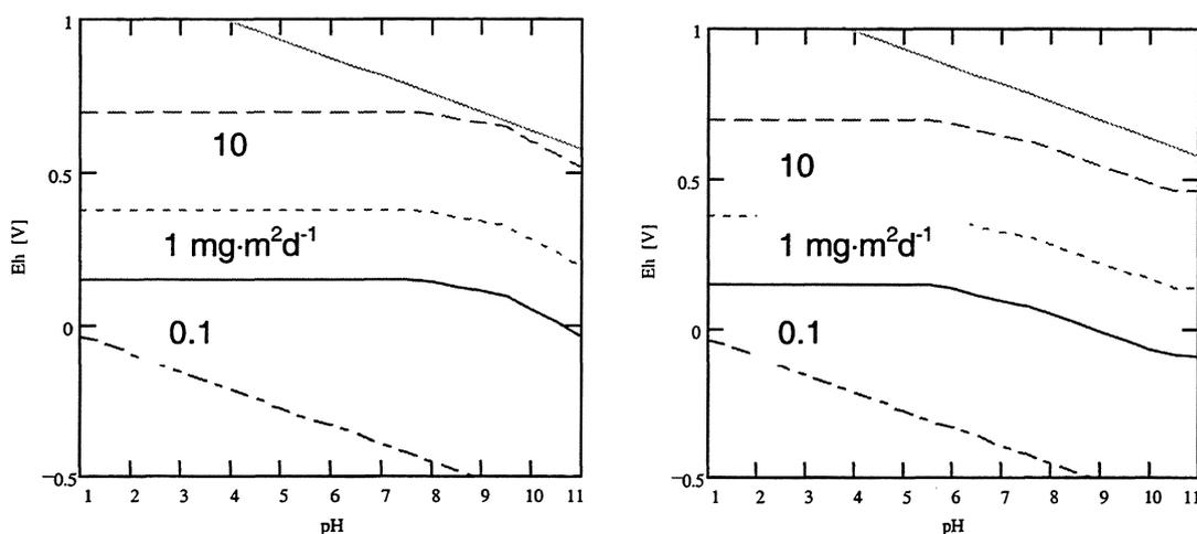
FIGURE IV.4-6: Isolines for equal corrosion rates of UO<sub>2</sub> in Eh-pH-space, (a) in the absence and (b) presence of 0.01 m carbonate
