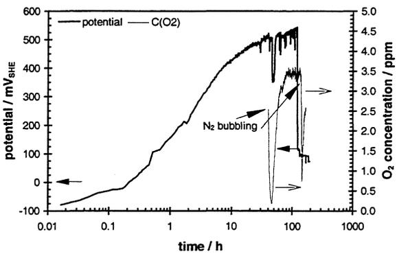
Fig. 8: Open circuit potential of unirradiated UO<sub>2</sub>, related temperature, pH, Eh and oxygen concentration data in 95% saturated NaCl solution ( $^{max}E_{corr} = 543 \text{ mV}_{SHE}$ )
