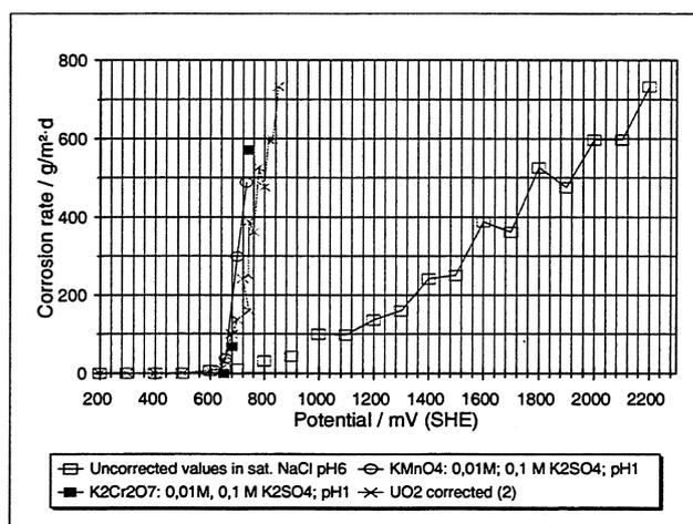
**FIGURE I.6-31: Comparison between corrosion rates depending on potentials, obtained from adding a redox system and also from potentiostatic polarization**
