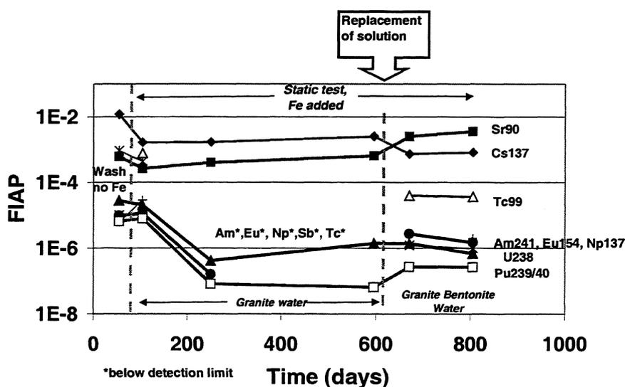
Fig. III.1-3: Corrosion of spent fuel powder in synthetic granite water and granite (bentonite) water in the presence of Fe: Released fractions (non-cumulative) of radioelements as a function of corrosion time (FZK)
