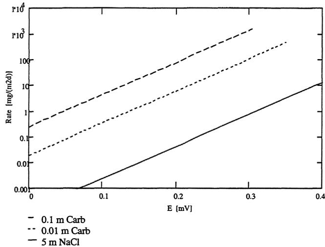
FIGURE IV.1-6: Predicted calibration curves in carbonate containing and carbonate free media
