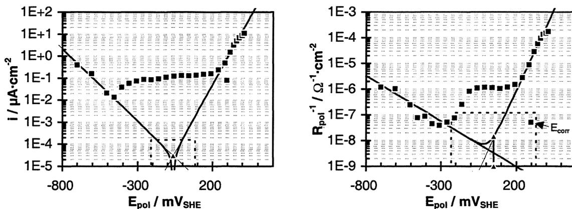
Fig. 2: Potentiostatic polarisation curves obtained from unirradiated  $UO_2$  in  $N_2$ -purged synthetic groundwater ( $T = 23^\circ C$ ,  $p(O_2) < 1$  mbar, initial pH 8.4,  $t_{pol} = 10$  min,  $A_{el} = 0.478$  cm<sup>2</sup>,  $d_{el} = 1$  mm).
