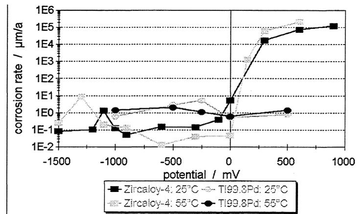
FIGURE I.8-3: Corrosion on Ti99.8Pd and Zircaloy-4
