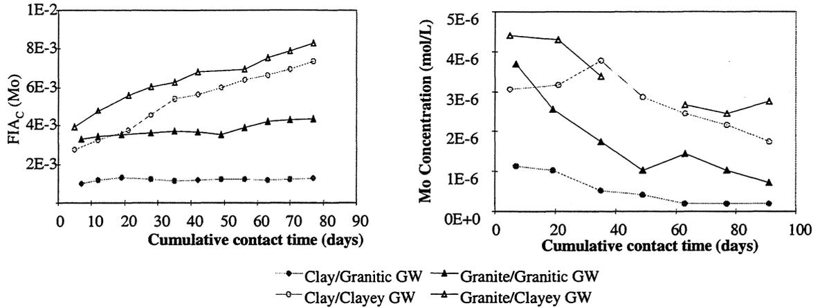
FIGURE III.3.6. Gravelines 3+2 spent fuel-leaching experiment: Mo FIA<sub>c</sub> and solution conc. of Mo versus cumulative leaching time, environmental materials and groundwater composition
