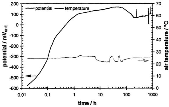
Fig. 9: Open circuit potential of used  $\text{UO}_2$  fuel B2 (burn-up: 31.5 GWd/t) and related temperature, in synthetic ( ${}^{\text{max}}E_{\text{corr}} = 168 \text{ mV}_{\text{SHE}}$ ,  $T: 22 - 28^\circ\text{C}$ ,  $C(\text{O}_2) < 2 \text{ ppm}$ , initial pH 8)
