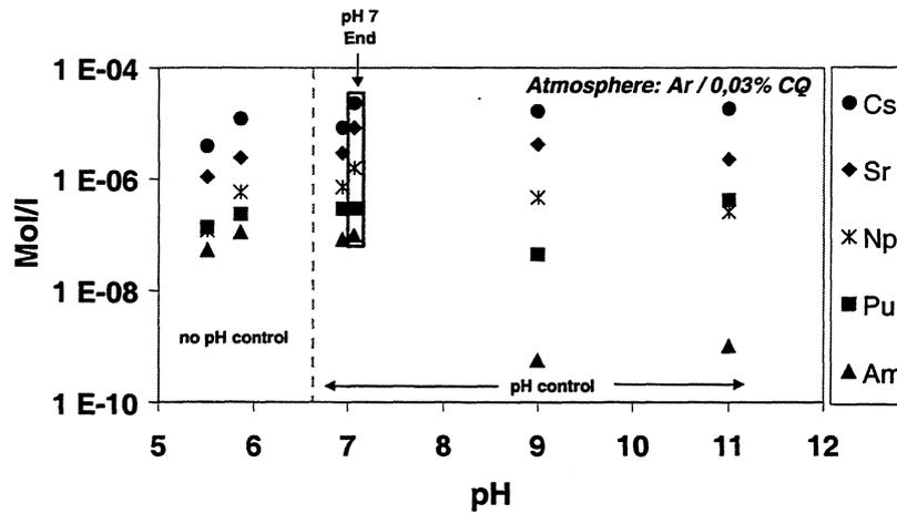
FIGURE I.1-6: Concentrations of radioelements as a function of pH during dissolution of spent fuel powder P56(II) in 5m NaCl solution under Ar / 0,03% CO<sub>2</sub> -Atmosphere
