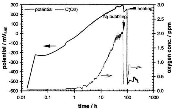
Fig. 7: Open circuit potential of unirradiated UO<sub>2</sub>, related temperature, pH, Eh and oxygen concentration data in 95% saturated NaCl solution ( $^{max}E_{corr} = 299 \text{ mV}_{SHE}$ )
