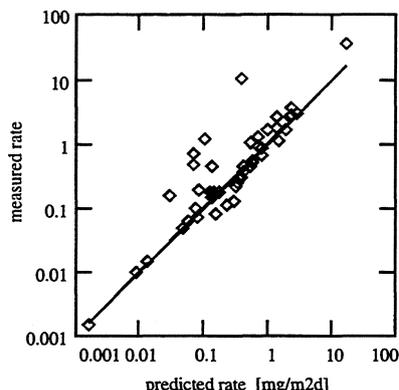
**FIGURE IV.1-5: Comparison of predicted and measured corrosion rates of UO<sub>2</sub> in various groundwaters (pH 1-10, HCO<sub>3</sub> 0-0.1 m, oxic and anoxic)**
