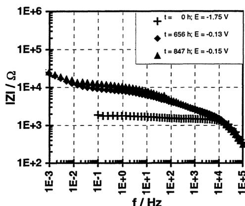
FIGURE I.6.27: EIS spectra measured during an open circuit potential experiment performed on fuel B4 in 95% sat. NaCl solution
