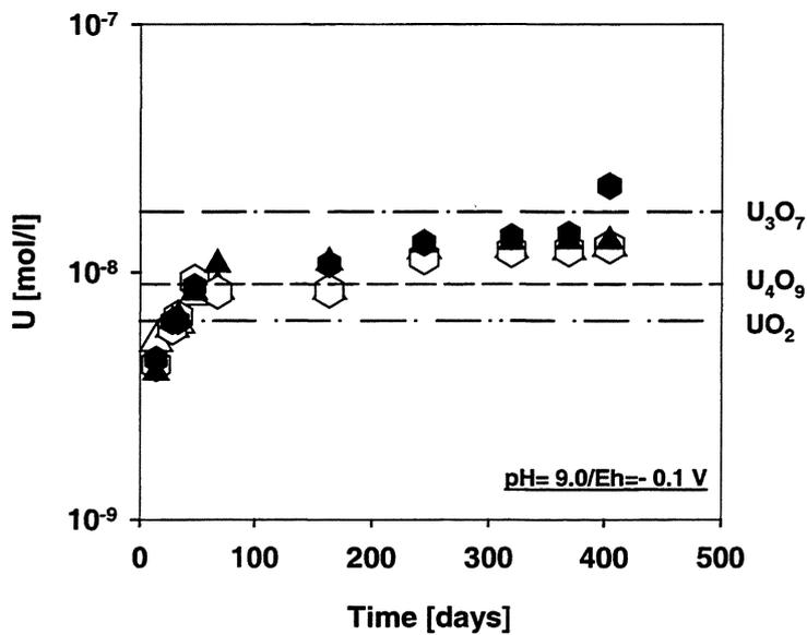
**FIGURE I.4-6. Uranium concentration vs. contact time in anaerobic ( $N_2$ ) saline (upper figure) and modified Allard (lower figure) groundwaters during dissolution of  $UO_2$  pellets,  $S/V=0.66 m^{-1}$ . The measured data are for two parallel experiments in each of the figures. The dashed lines show the theoretical solubilities of uranium oxides in equilibrium (EQ3/6, composite database) at measured pH and Eh values.**
