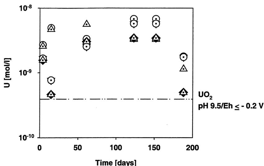
**FIGURE I.4-10. Uranium concentration vs. contact time in modified Allard groundwater during dissolution of  $\text{UO}_2$  pellets ( $S/V = 19.8 \text{ m}^{-1}$ ) in the presence of metallic Fe. The measured data (unfiltered samples) is for two parallel experiments (I: black symbols, II: open symbols). The dashed line shows the theoretical solubility of  $\text{UO}_2$  at measured pH in reducing conditions (EQ3/6, composite database).**
