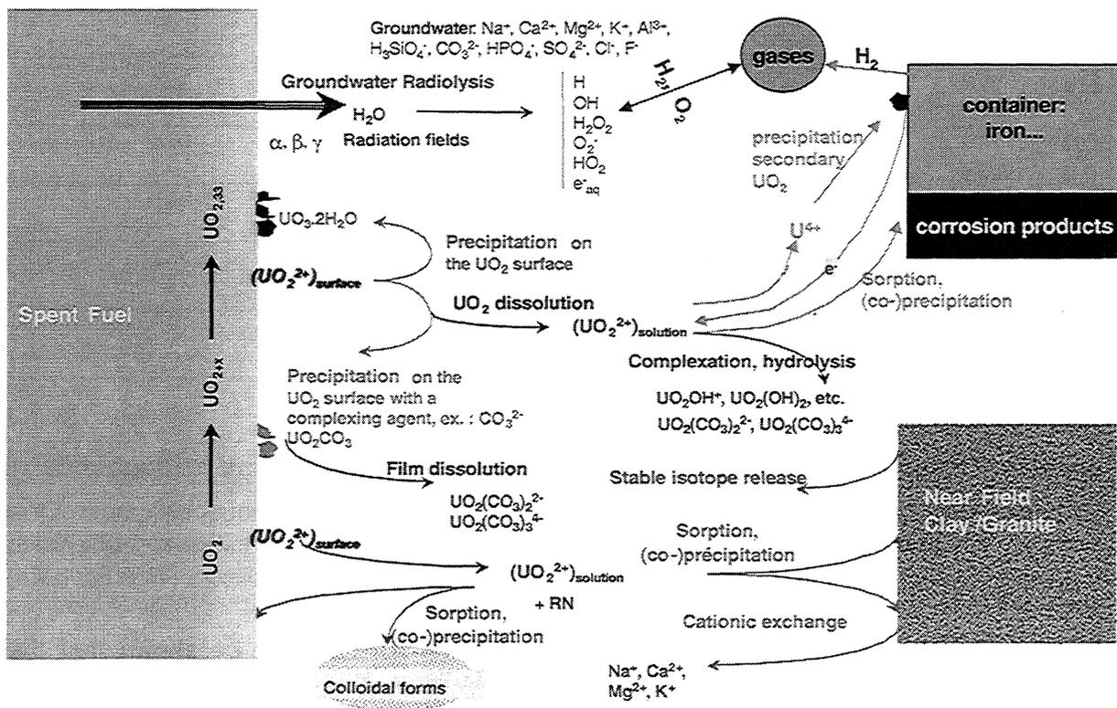
FIGURE IV.4-2. Spent fuel alteration mechanisms and mechanisms controlling radionuclide concentration in solution in presence of environmental materials
