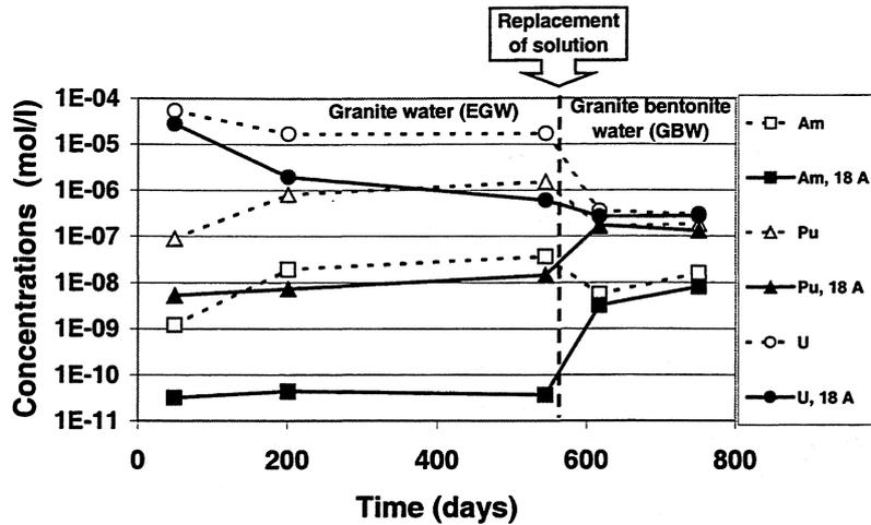
FIGURE I.1 – 11: Concentrations of Am, Pu and U in 0,45 µm and 18 A filtered aliquots during static spent fuel powder corrosion in granite and granite bentonite ground water.
