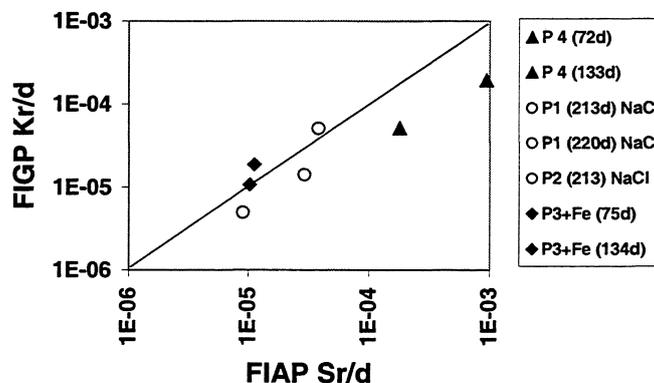
Figure III.1-5: Comparison of Kr-release rates vs. Sr release rates during corrosion of spent fuel powders in GBW (P3,P4) and P1,P2 (NaCl)
