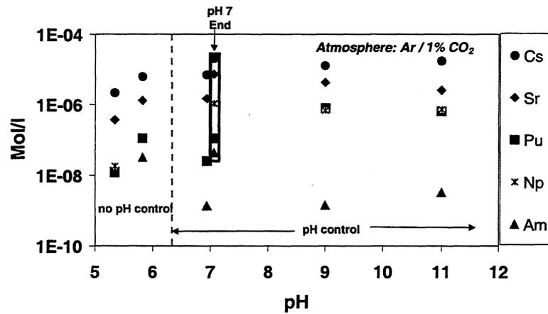
FIGURE I.1-7: Concentrations of radioelements as a function of pH during dissolution of spent fuel powder P56(III) in 5m NaCl solution under Ar / 1 % CO<sub>2</sub> -Atmosphere
