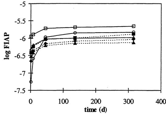
FIGURE I.3.7: FIAP values for uranium. ◆ MOX fuel (12 GWd/tU), ■ MOX fuel (20 GWd/tU), ▲ MOX fuel (25 GWd/tU), △ UO<sub>2</sub> fuel (30 GWd/tU), □ UO<sub>2</sub> fuel (50 GWd/tU) and ○ UO<sub>2</sub> fuel (50 GWd/tU with two series of defects)
