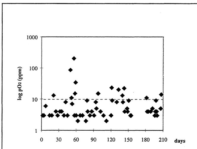
**FIGURE 4 :** Oxygen partial pressure in Ar/CO<sub>2</sub> glove box during predissolution stage
