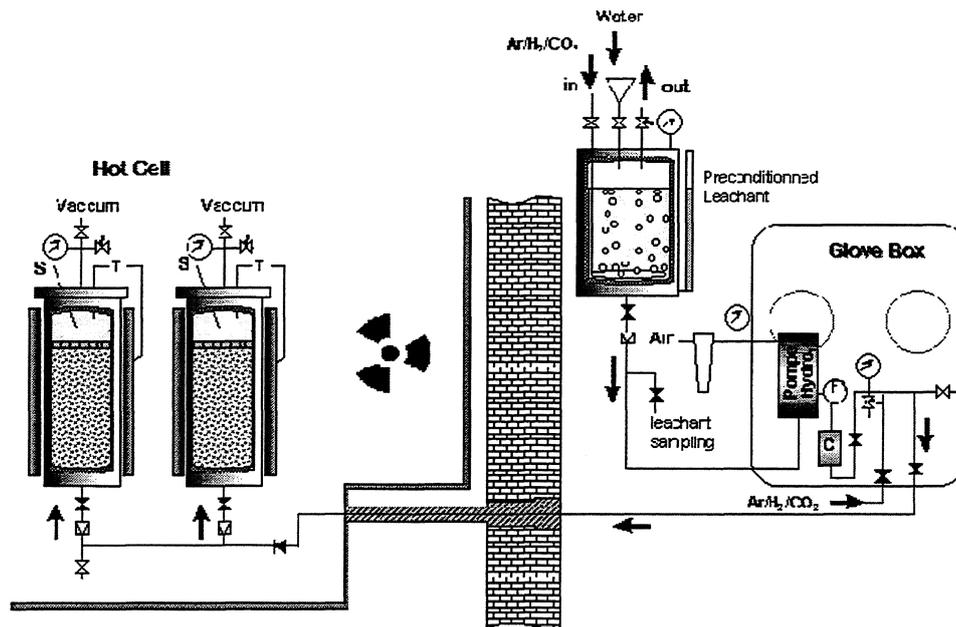
**FIGURE II.3.1 : Schematic representation of integral leach tests, including preconditioning devices and redox control for groundwater outside and leaching apparatus inside the hot-cells.**
