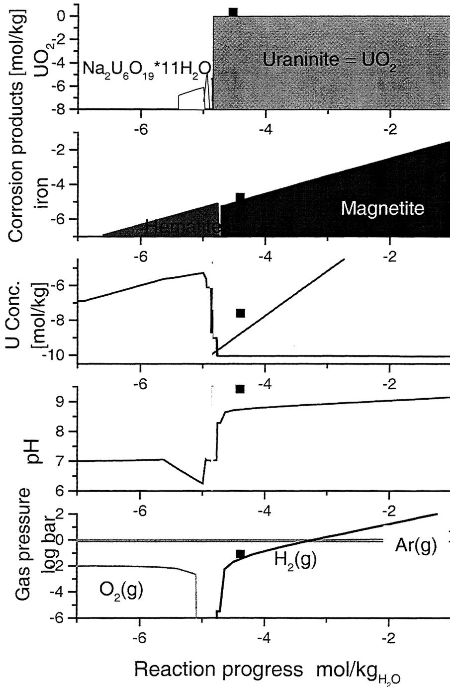
FIGURE IV.1.-2: Geochemical simulation of the reaction path of  $\text{UO}_2$  in 95% saturated NaCl solution under anoxic closed system conditions (absence of radiolysis). Black dots: Experimental data, Appendix 2, TABLE 19)
