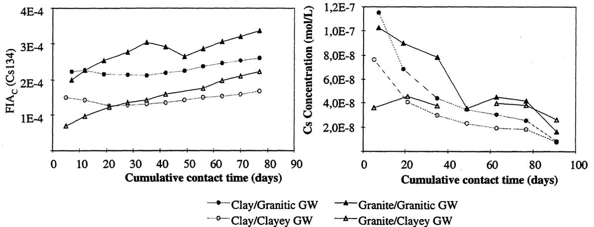
FIGURE III.3.5. Gravelines 3+2 spent fuel-leaching experiment: <sup>134</sup>Cs FIA<sub>C</sub> and solution concentrations of Cs versus cumulative leaching time, environmental materials and groundwater composition
