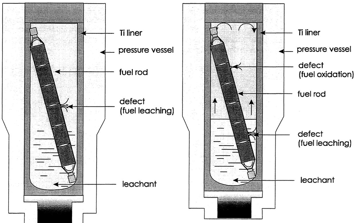
FIGURE I.3.1: Schematic representation of the experimental set-up (leaching of fuel rod, 1 defect immersed).
