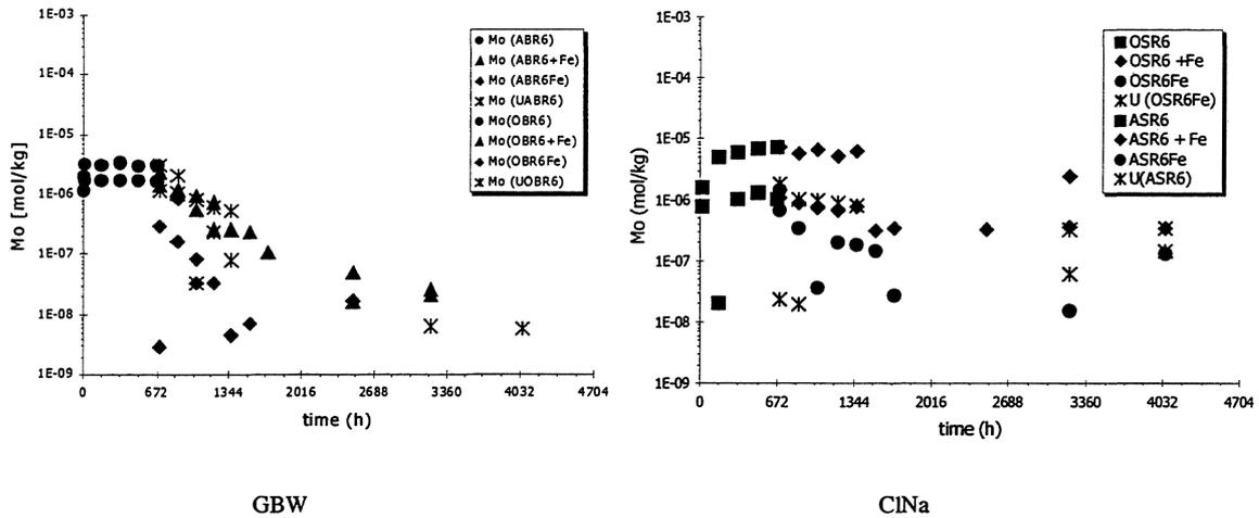
FIGURE III.1-20 [Mo] against time in GBW and in 5 m NaCl for both oxidising and reducing low carbonate conditions. Fe is present in the system after 720 h leaching time.
