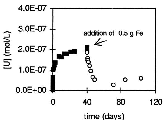
FIGURE III.1-12 Uranium concentration vs. time in the UOFGW experiment
