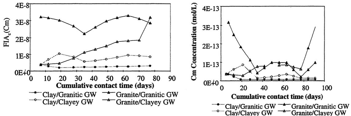
Figure III.3.9. Gravelines 3+2 spent fuel leaching experiment:  $^{244}\text{Cm}$   $\text{FIA}_c$  and solution concentrations of Cm versus cumulative leaching time, environmental materials and groundwater composition
