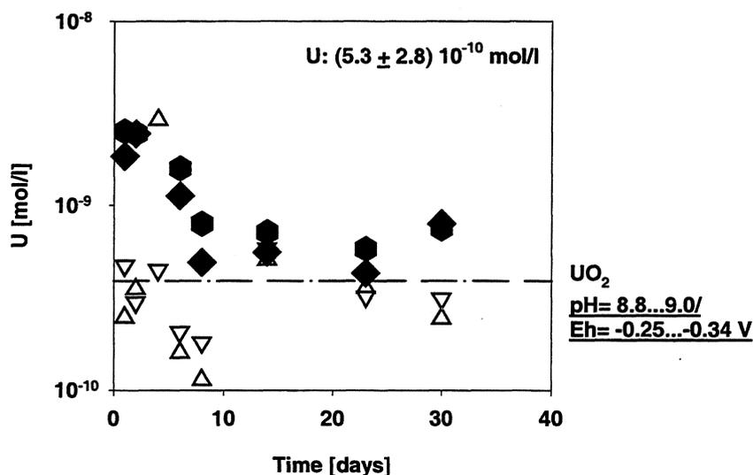
FIGURE I.4-11. U-Concentrations in the oversaturation experiments in modified Allard groundwater under anoxic conditions (open symbols: without S(-II) addition, filled symbols: with 3 ppm S(-II)). The dashed line shows the theoretical solubility of  $\text{UO}_2$  (EQ3, composite database) at measured Eh values.
