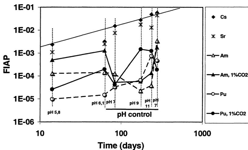
**FIGURE I.1-4: Effect of CO<sub>2</sub> on the release of Pu, Am, as a function of time during dissolution of spent fuel powder in 5m NaCl solution**
