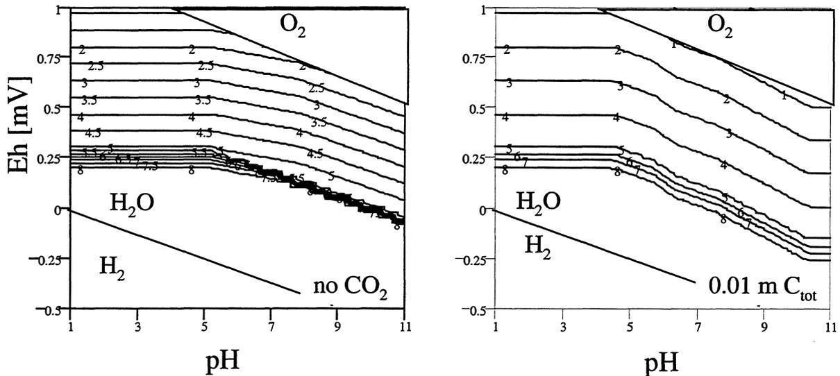
**FIGURE IV.4-7: Estimated times (log yr.) necessary for the complete dissolution of a container with 5 tons of spent fuel in groundwater flowing with a hypothetical rate of  $1 \text{ m}^3/\text{yr}/\text{canister}$ . Transition from electrochemical (oxic) rate control to solubility control under reducing conditions. Comparison of results with and without carbonate**
