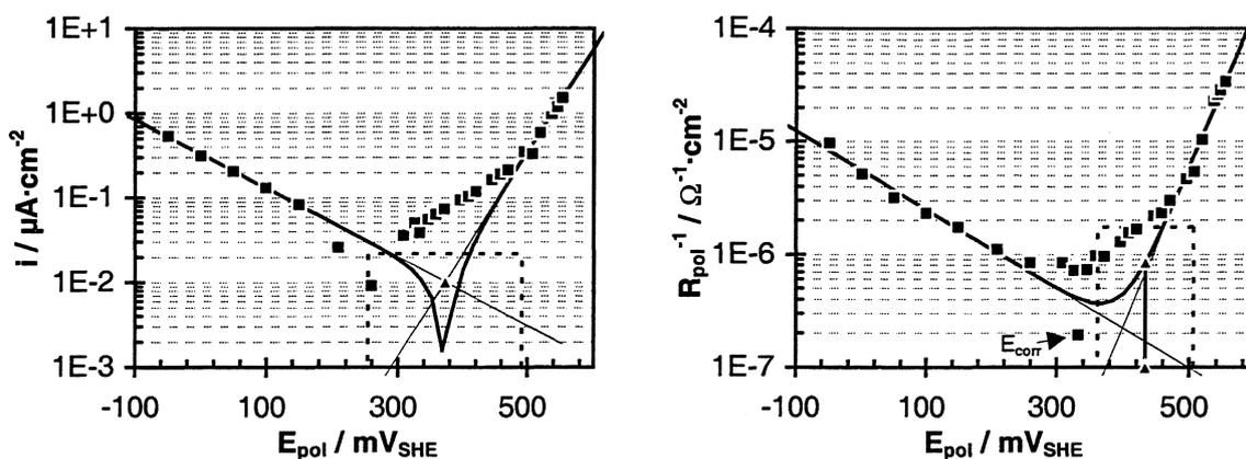
FIGURE. I.6.22: Potentiostatic polarization curves obtained from unirradiated  $\text{UO}_2$  in simulated groundwater ( $T = 60^\circ\text{C}$ ,  $p(\text{O}_2) < 1 \text{ mbar}$ , initial pH 7.7).
