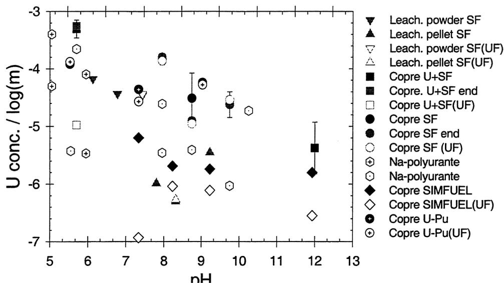
FIGURE II.1.4 U concentration from SF, SIMFUEL, UO<sub>2</sub>, U-Pu experiments in saline solutions.
