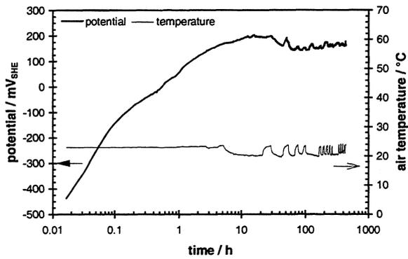
Fig. 10: Open circuit potential of used  $\text{UO}_2$  fuel B2 (burn-up: 31.5 GWd/t) and related temperature, in synthetic groundwater ( ${}^{\text{max}}E_{\text{corr}} = 204 \text{ mV}_{\text{SHE}}$ ,  $T: 20 - 25^\circ\text{C}$ ,  $C(\text{O}_2) < 2 \text{ ppm}$ , initial pH 7.6)
