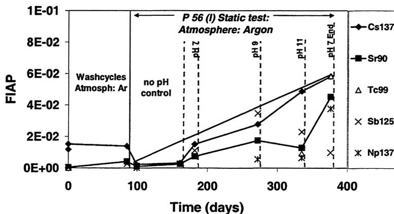
FIGURE I.1-2: Released fractions of matrix bound radionuclides Cs137, Sr90, Np137, Tc99 as a function of time during dissolution of spent fuel powder P56(I) in 5m NaCl solution under Ar-Atmosphere
