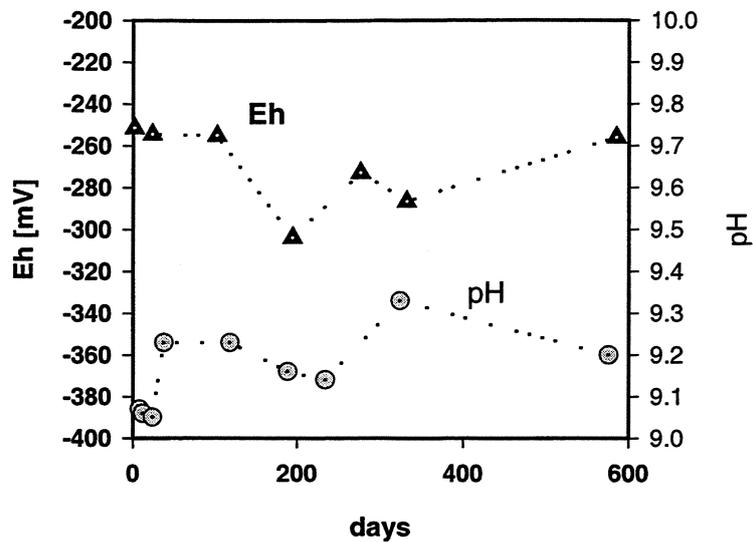
**FIGURE 6:** The measured Eh and pH values in a parallel sample of saline groundwater with 3 ppm S(-II) during a follow-up period of 600 days under anaerobic conditions.
