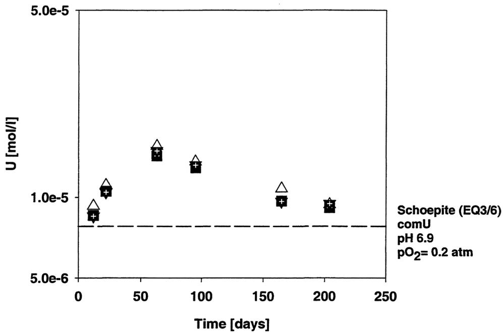
FIGURE I.4-4. Uranium concentration vs. contact time in air-saturated near-field groundwater during dissolution of  $\text{UO}_2$  powder,  $S/V = 1000 \text{ m}^{-1}$  (filled symbols: unfiltered samples, open symbols: filtered samples, 12 000 M). The dashed line shows the theoretical solubility of schoepite (comU= Data0.com.R2 [92WOL]).
