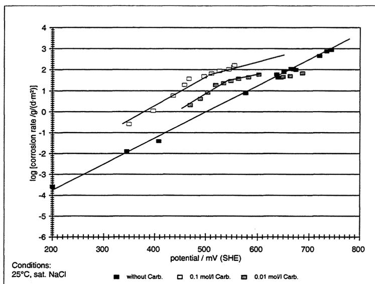
**FIGURE I.6-36: Comparison of calibration curves for  $\text{UO}_2$  corrosion rates vs. potential in presence and absence of carbonate**
