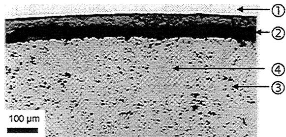
FIGURE. I.6.13: Micrograph of MOX fuel with a burn-up of 24 GWd/t (1: cladding, 2: gap, 3:  $\text{UO}_2$  matrix of fuel, 4: Pu-rich agglomerates)
