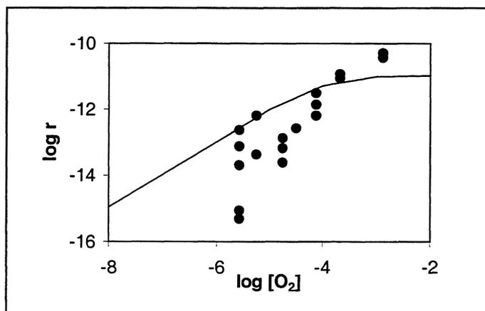
**FIGURE IV.1-8 Comparison with the experimental data obtained by [92SHO/SUN] using UO<sub>2</sub> and electrochemical experiments, and the trend predicted by equation IV.1-8, represented by the solid line.**
