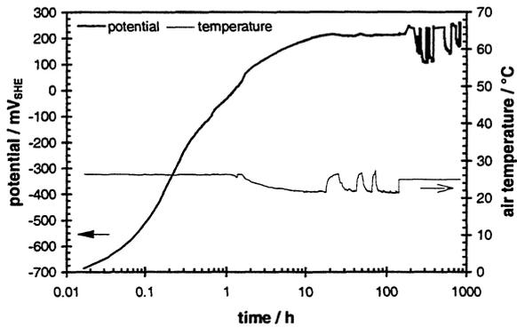
Fig. 11: Open circuit potential of used  $\text{UO}_2$  fuel B3 (burn-up: 45.2 GWd/t) and related temperature, in synthetic groundwater ( ${}^{\text{max}}E_{\text{corr}} = 260 \text{ mV}_{\text{SHE}}$ ,  $T: 22 - 28^\circ\text{C}$ ,  $C(\text{O}_2) < 2 \text{ ppm}$ , initial pH 8)
