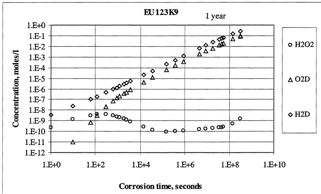
FIGURE 2 Radiolysis in phase 3 (surface layer with  $\beta, \gamma$  radiation). 5 m NaCl solution.
