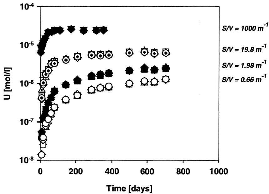
FIGURE I.4-5. Uranium concentration vs. contact time in air-saturated saline groundwater in the experiments with different  $S/V$ . The measured data at each  $S/V$  is for two parallel experiments.
