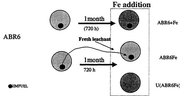
**FIGURE III.1-14 Example for test procedure (Anoxic conditions and GBW (ABR6))**
