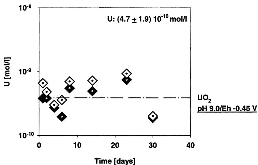
FIGURE I.4-12. Concentrations of uranium vs. time in the oversaturation experiments in modified Allard groundwater under anoxic conditions in the presence of metallic Fe. The dashed line shows the theoretical solubility of  $\text{UO}_2$  (EQ3, composite database) at measured Eh value.
