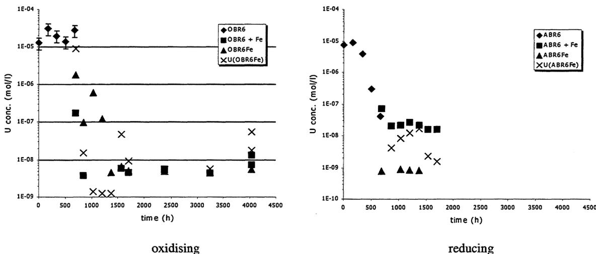
FIGURE III.1-15 [U] evolution under oxidising and reducing conditions respectively in GBW ( $\log f_{\text{CO}_2}=-3.5$ ). Fe is present in the system after 720 h leaching time.
