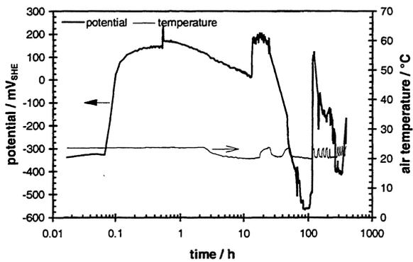
Fig. 12: Open circuit potential of used  $\text{UO}_2$  fuel B4 (burn-up: 53.1 GWd/t) and related temperature, in synthetic groundwater ( ${}^{\text{max}}E_{\text{corr}} = 239 \text{ mV}_{\text{SHE}}$ ,  $T: 22 - 25^\circ\text{C}$ ,  $C(\text{O}_2) < 2 \text{ ppm}$ , initial pH 7.6)
