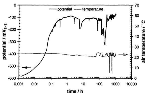
FIGURE. I.6.24: Open circuit potentials of  $\text{UO}_2$  fuel B2 in 95% sat. NaCl solution (initial pH = 7.3,  $\text{C}(\text{O}_2) < 2 \text{ ppm}$ ).
