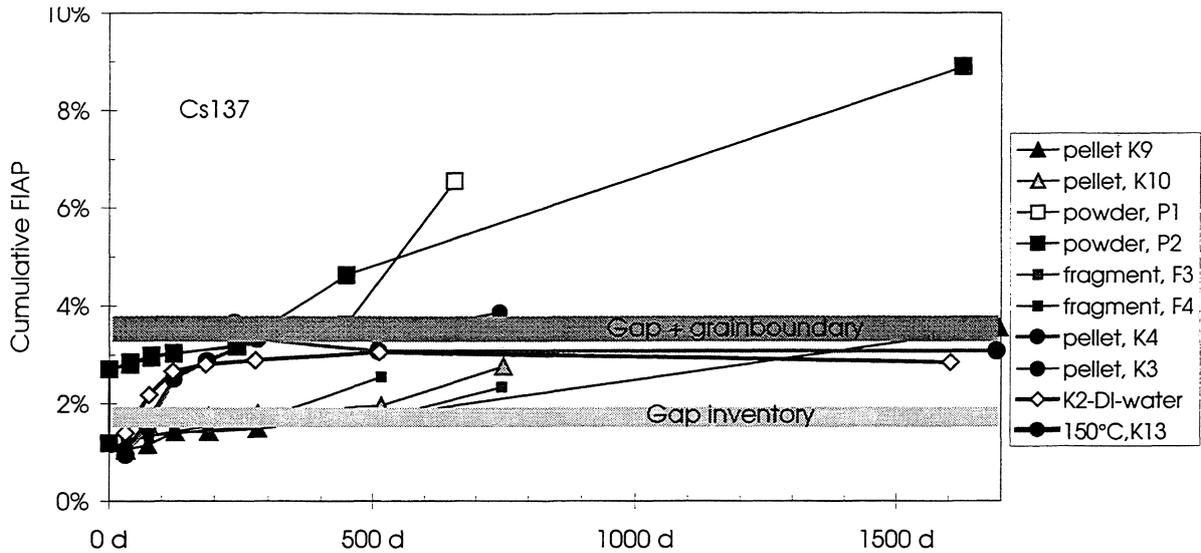
**FIGURE IV.4-1: Cs release data from high burnup fuel powders and pellets to determine gap and grain boundary inventories**
