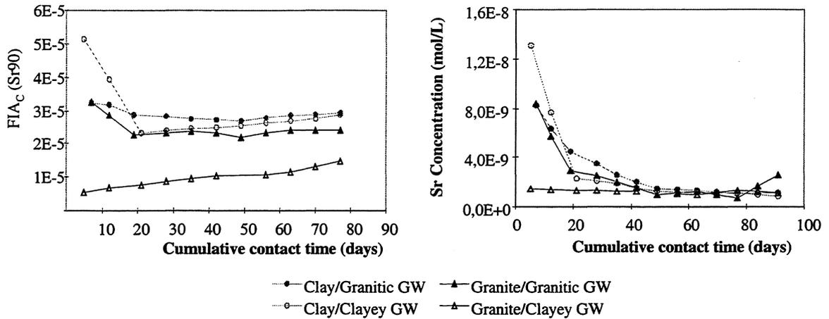
FIGURE III.3.4. Gravelines 3+2 spent fuel leaching experiment: <sup>90</sup>Sr FIA<sub>c</sub> versus cumulative leaching time, environmental materials and groundwater composition
