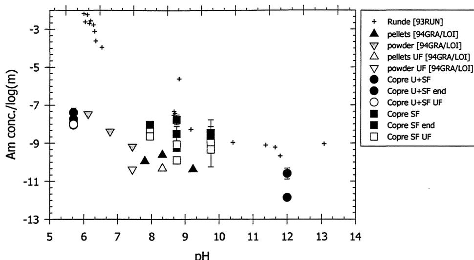
FIGURE II.1.1 Am conc. from leaching and coprecipitation SF test in saline solutions.
