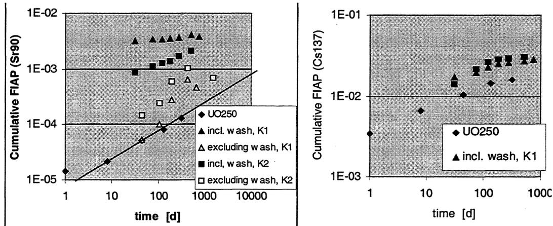
FIGURE 1.3-9. Comparison of cumulative release fractions of Cs137 and Sr90 from decladdled and non-decladdled (preset defects) high burnup spent UOX fuel (ca. 50 MWd/kg<sub>BM</sub>) in deionized water.
