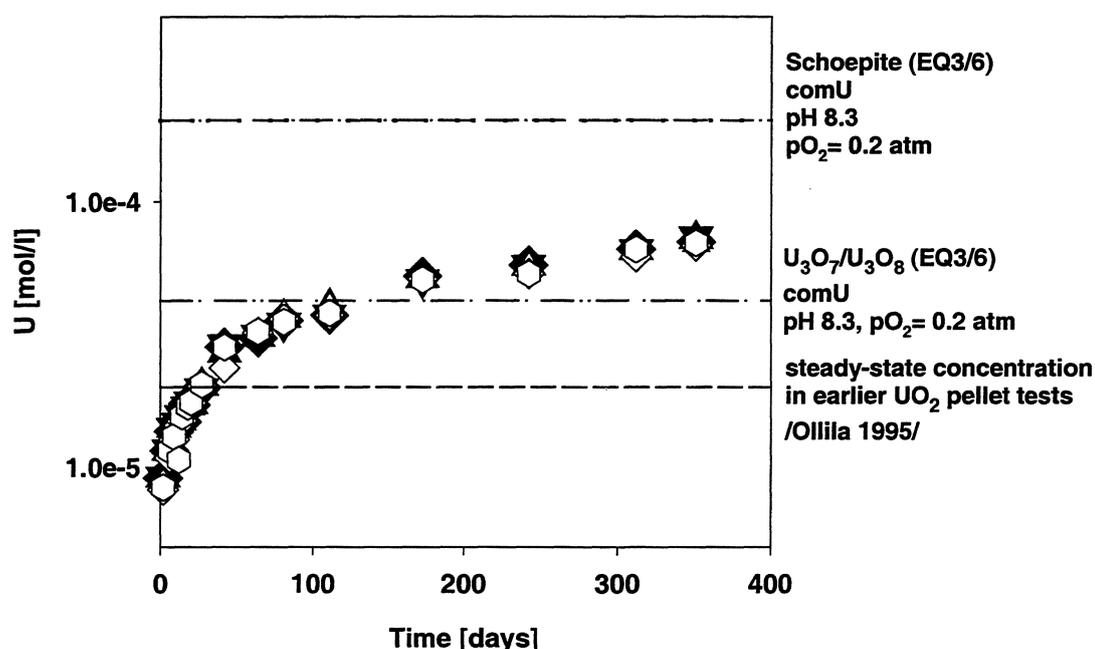
**FIGURE I.4.2.** Uranium concentration vs. contact time in air-saturated Allard groundwaters during dissolution of  $\text{UO}_2$  powder,  $S/V=1000 \text{ m}^{-1}$  (filled symbols: Allard groundwater [81ALL/LAR], open symbols: modified Allard groundwater [98VUO/SNE], see Appendix 4., Table 1). The dashed lines show the theoretical uranium solubilities in equilibrium with the marked phases (comU= Data.0.com.R2 [92WOL]).
