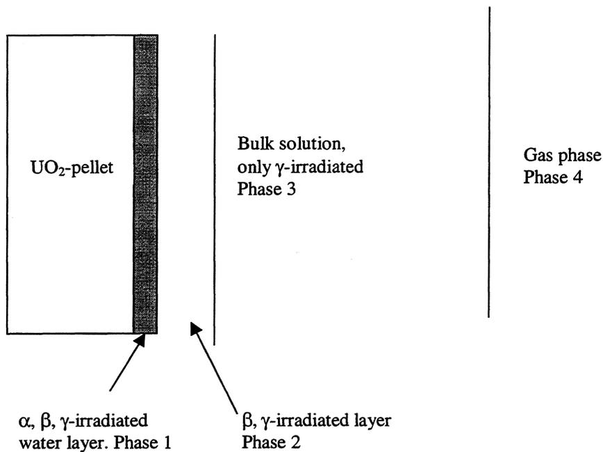
**FIGURE IV.3-1: Phases considered in radiolysis model**
