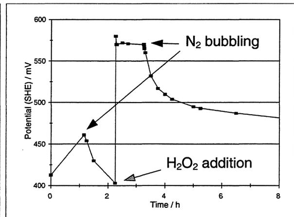
**FIGURE 1.6-35: potential of platinum electrode 0.1M  $\text{H}_2\text{O}_2$  with bubbling of nitrogen**
