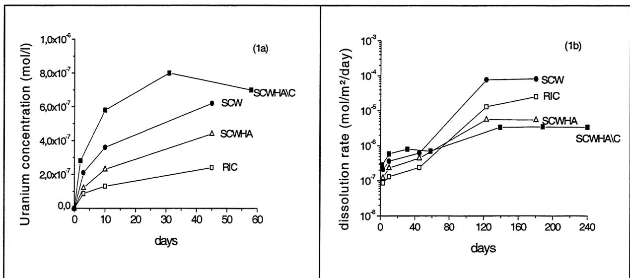
FIGURE I.4-13: Mean uranium concentrations of the first series of solubility tests in the first 58 days (1a) and until 240 days (1b). (RIC = real Boom Clay water; SCW= Synthetic Clay Water; SCWHA= Synthetic Clay Water with humic acids; SCWHA\C = Synthetic Clay Water with humic acids and low carbonate content.
