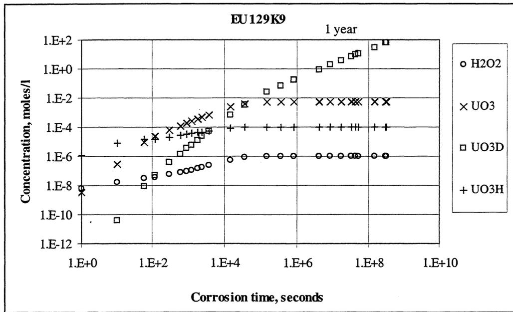
FIGURE 1 Radiolysis in phase 3 (surface layer with  $\beta, \gamma$  radiation). 5 m NaCl solution.
