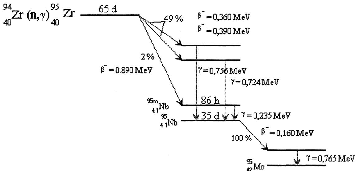
FIGURE I.8-1.: Block diagram of  $^{95}\text{Zr}$  decay
