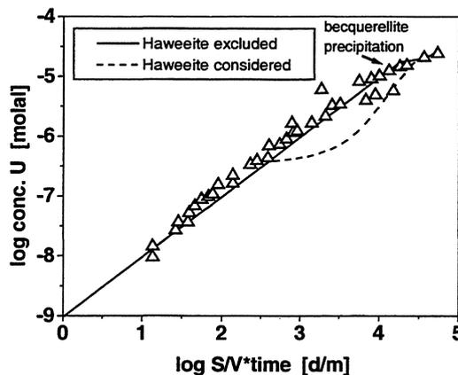
**FIGURE IV.1-3: Time dependent reaction path of UO<sub>2</sub> dissolution in oxic saline granite waters (EQ3/6-calculation by FZK)**
