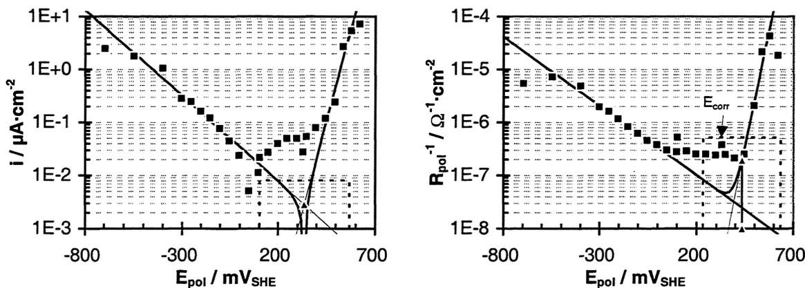
Fig. 3: Potentiostatic polarisation curves obtained from unirradiated  $UO_2$  in  $N_2$ -purged synthetic groundwater ( $T = 60^\circ C$ ,  $p(O_2) < 1$  mbar, initial pH 7.4,  $t_{pol} = 20$  min,  $A_{el} = 0.478$  cm<sup>2</sup>,  $d_{el} = 0.9$  mm).
