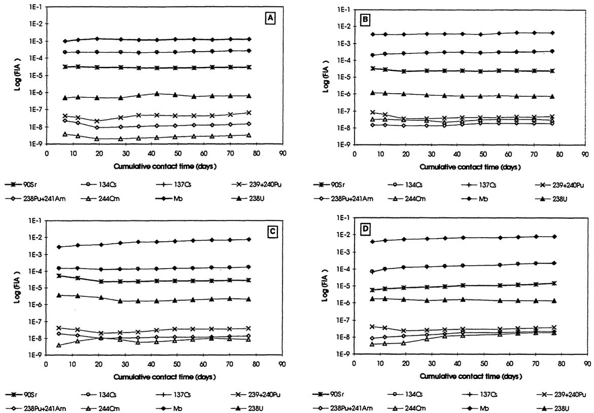
FIGURE III.3.3. Gravelines 3+2 spent fuel leaching experiment: FIA<sub>C</sub> of radionuclides and elements Clay/Granite water medium ; (B) Granite/ Granite water medium. (C) Clay/Clayey water medium; (D) Granite/Clayey water medium.
