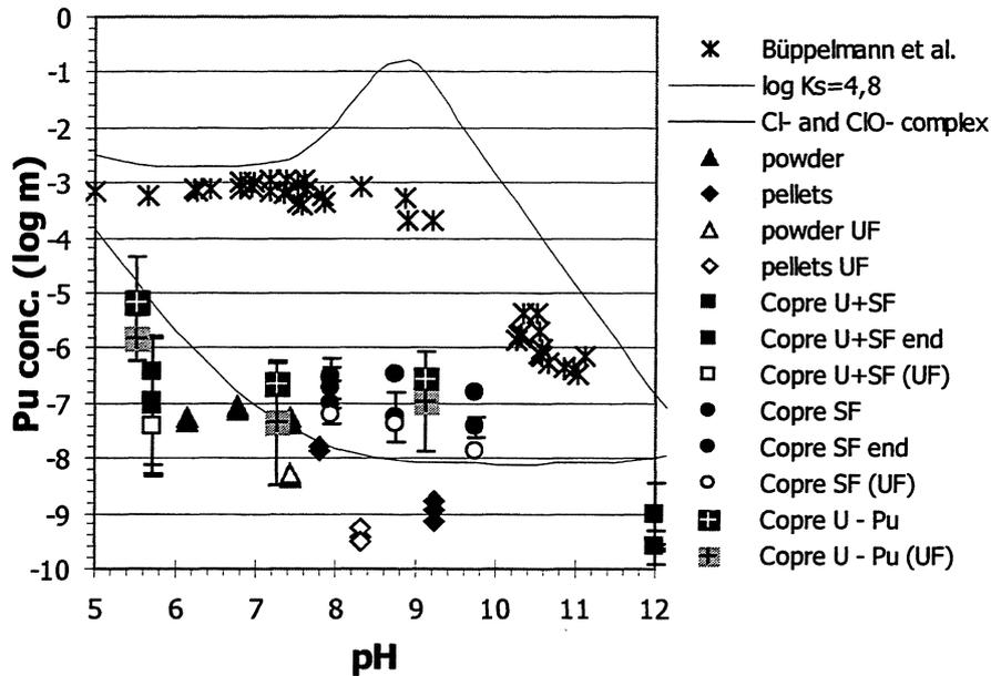
FIGURE II.2.1 Pu concentration from leaching and coprecipitation of SF and U/Pu tests in saline solutions.
