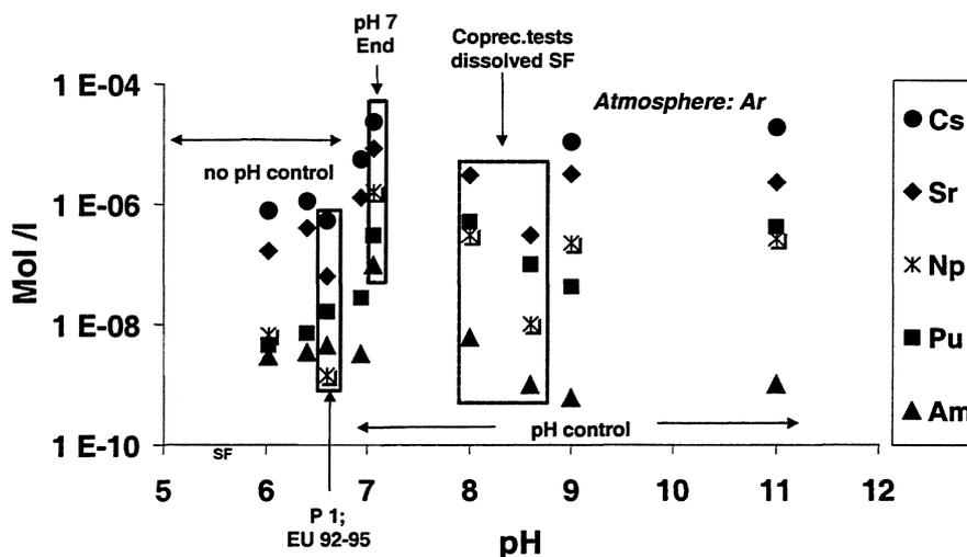
**FIGURE I.1-5: Concentrations of radioelements as a function of pH during dissolution of spent fuel powder P56(I) in 5m NaCl solution under Ar-Atmosphere**
