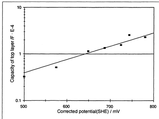
**FIGURE I.6-33 : Capacity vs. corrected potential in sat. NaCl solution at  $25^\circ C$**
