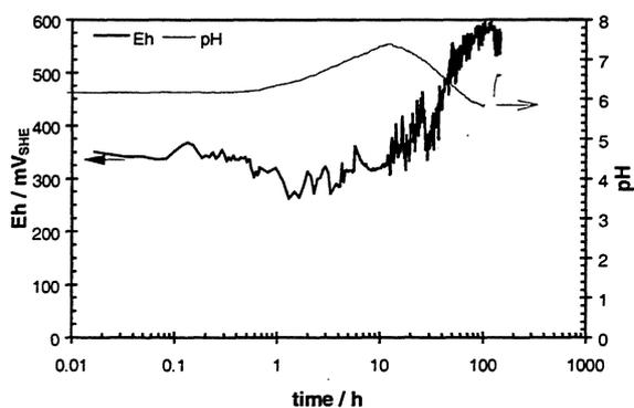
Fig. 6: Open circuit potential of unirradiated  $UO_2$  and related temperature, pH and Eh data at  $22^\circ C$  in 95% saturated NaCl solution ( $E_{corr}^{max} = 226$   $mV_{SHE}$ )
