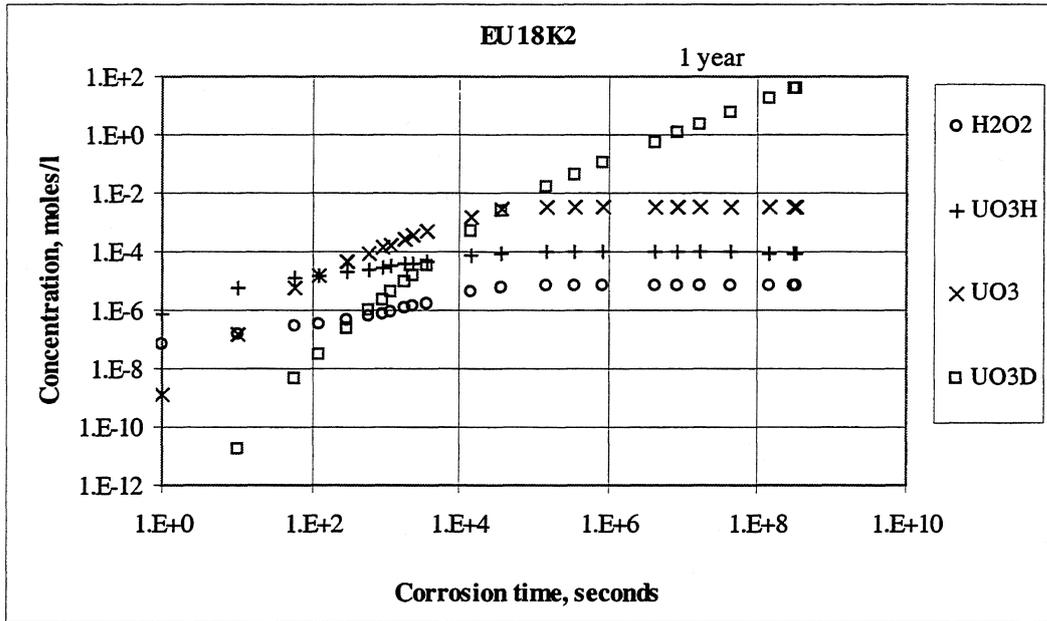
**FIGURE IV.3-2 Radiolysis in phase 1 (surface layer with  $\alpha,\beta,\gamma$  radiation). Deionized water. (Calculation EU18, Table 7, Appendix 9)**
