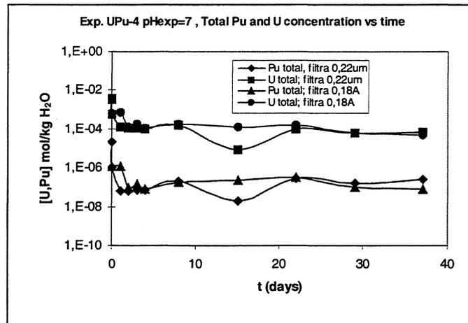
FIGURE II.2.2 Evolution of U and Pu conc. in 5 m NaCl.
