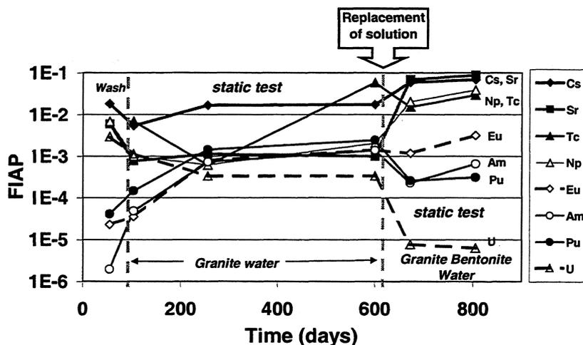
**FIGURE I.1 – 8: Fractions of the inventory of radioelements in solution during corrosion of spent fuel powder in granite and granite bentonite water.**
