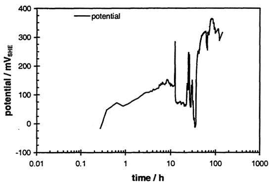
Fig. 5: Open circuit potential of unirradiated  $UO_2$  at  $60^\circ C$  in  $N_2$ -purged synthetic groundwater ( $E_{corr}^{max} = 364$   $mV_{SHE}$ ,  $C(O_2) = 0.05$  ppm, initial pH 7.7)
