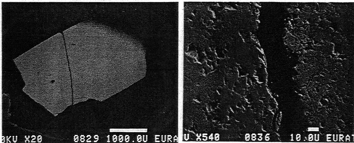
**Fig. I.6.16:** SEM micrographs of a spent fuel sample divided into two separate parts by a crack. Left side remains as polished and right side shows grain boundary attack.
