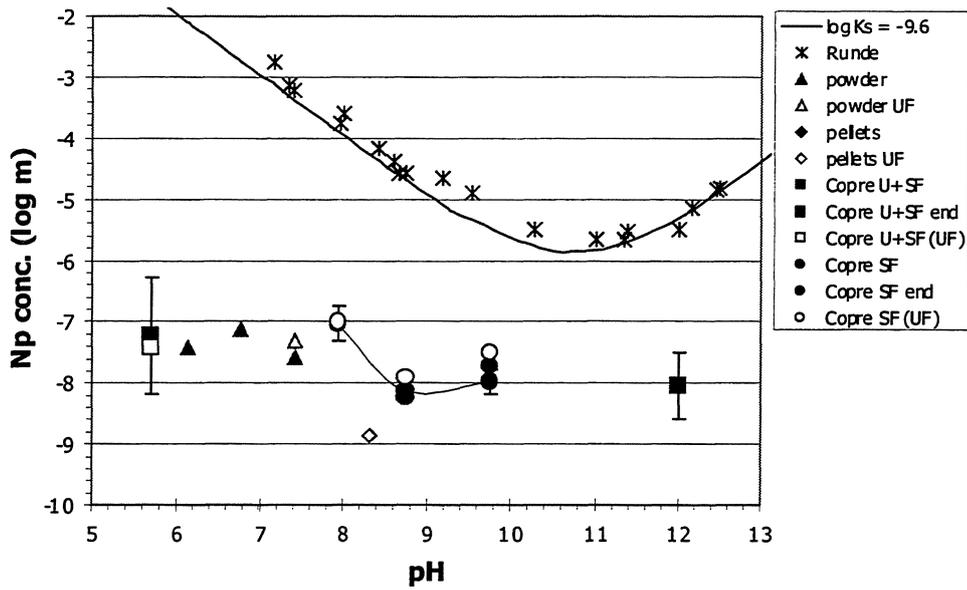
FIGURE II.1.2 Np conc. from leaching and coprecipitation tests in saline solution
