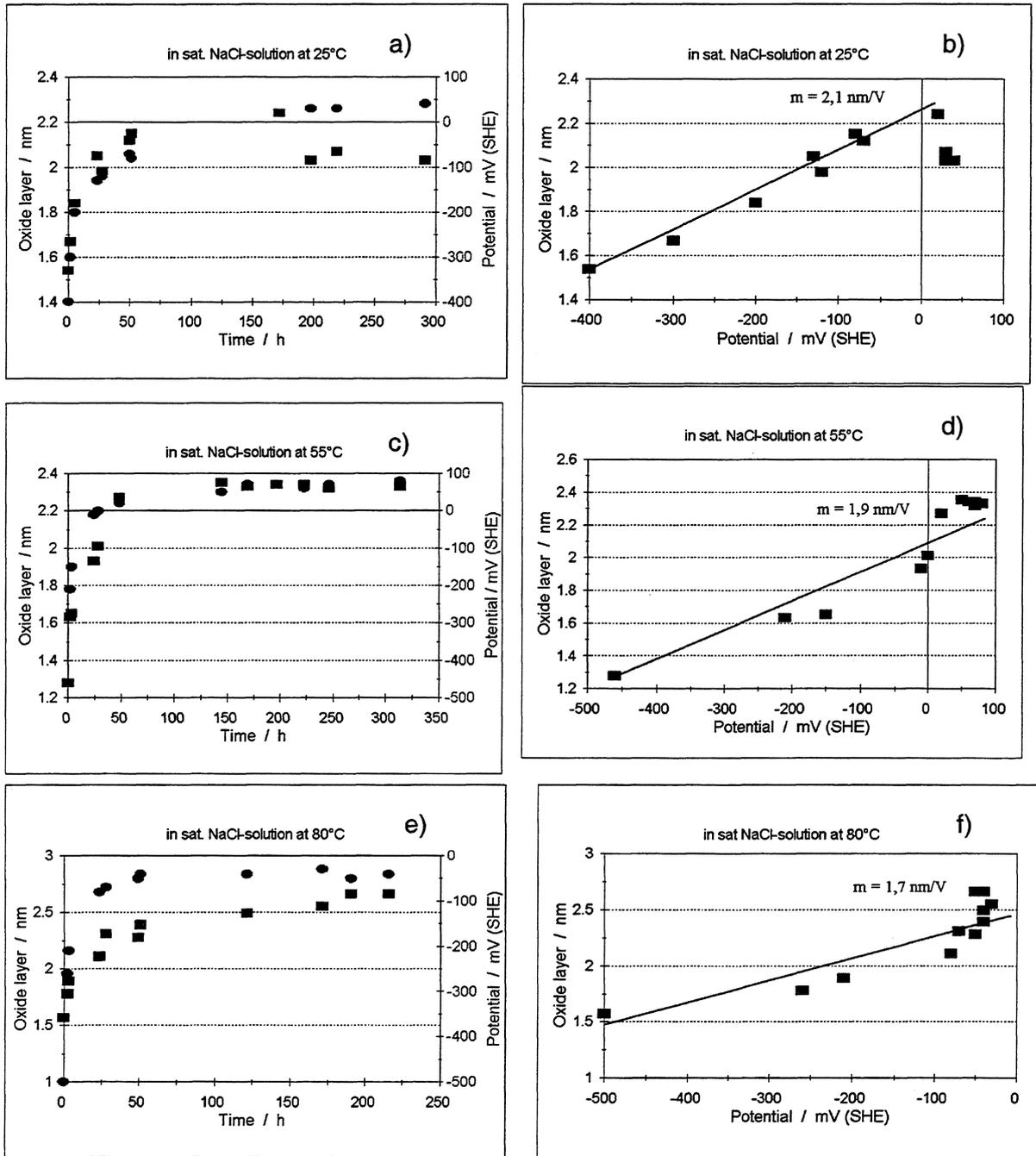
**FIGURE I.8-4 a-f: Formation of oxide layer and its thickness on zircaloy-4 electrode in saturated NaCl solution**
