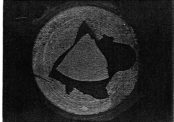
**FIGURE. I.6.15:** Piece of spent fuel (B4) mounted on brass stub of electrode head (diameter of brass stub: 10 mm) and embedded and polished.
