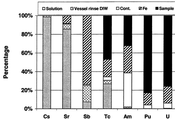
Figure III.1 -2: Dissolution of pellet K 4 for 1619 days in 5 m NaCl-solution under anaerobic conditions in the presence of 8,5 g Fe powder
