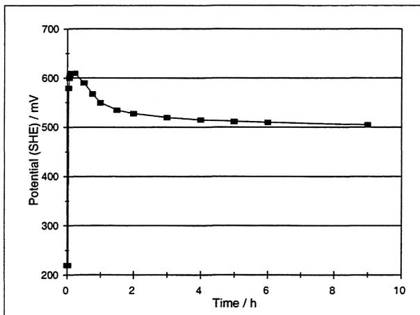
**FIGURE 1.6-34: Corrosion potential of  $\text{UO}_2$  0.1M  $\text{H}_2\text{O}_2$  95% sat. NaCl solution**
