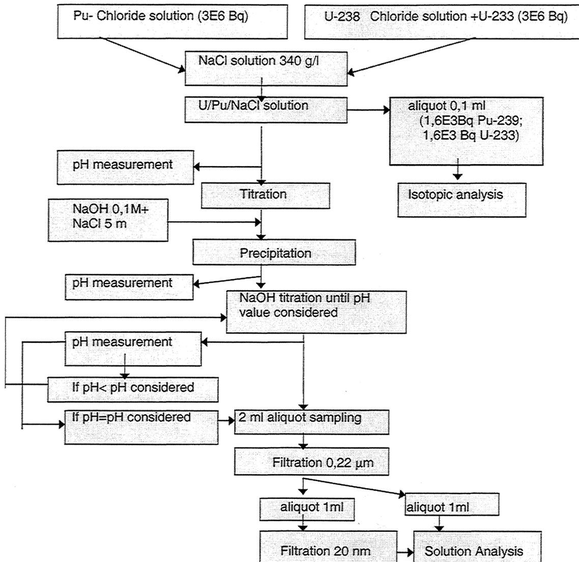
**FIGURE 1 Coprecipitation: Experimental Procedure**
