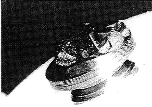
**FIGURE. I.6.14:** Piece of spent fuel (B4) mounted on brass stub of electrode head (diameter of brass stub: 10 mm).
