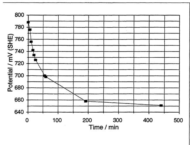
**FIGURE I.6-30: Effect of the decrease in concentration of oxidizing species on corrosion potentials in closed system: left: Schematic view: Partial current densities in presence of MnO<sub>4</sub><sup>-</sup>.  $U_1$  and  $U_2$  are the corrosion potentials at  $t_1$  and  $t_2$  respectively. right: Experimental data: Change of corrosion potential of a UO<sub>2</sub>-electrode after addition of 0.01 M KMnO<sub>4</sub> at 25°C, pH = 1, with time**
