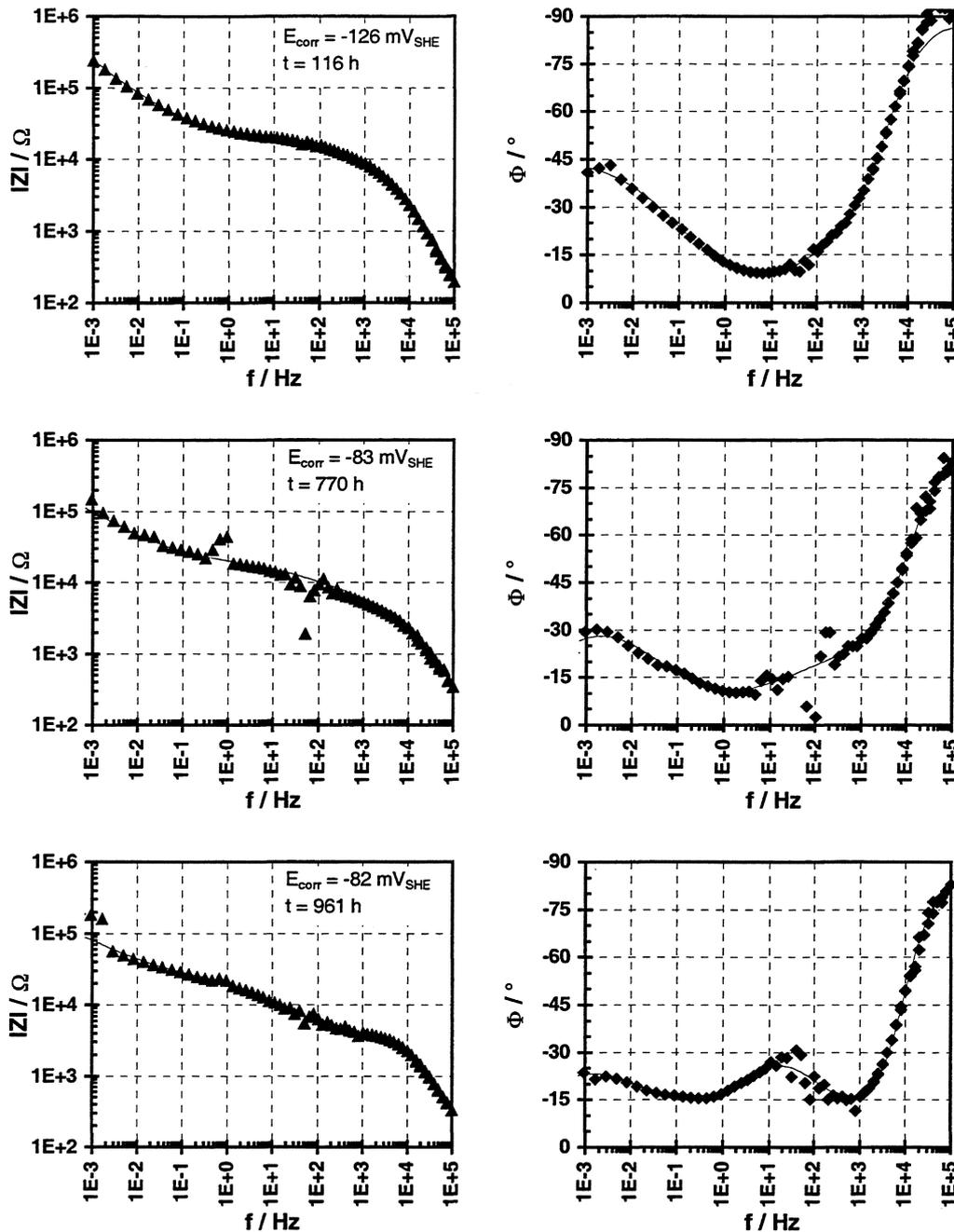
FIGURE I.6.26: EIS spectra series (part I) showing the evolution of conductive pathways measured during an open circuit potential experiment performed on fuel B2 in 95% sat. NaCl solution (continuous line: fitted data using equivalent circuit shown in FIGURE I.6.2).
