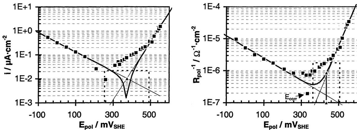
Fig. 4: Potentiostatic polarisation curves obtained from unirradiated  $UO_2$  in  $N_2$ -purged synthetic groundwater ( $T = 60^\circ C$ ,  $p(O_2) < 1$  mbar, initial pH 7.7,  $t_{pol} = 60$  min,  $A_{el} = 0.478$   $cm^2$ ,  $d_{el} = 1$  mm).
