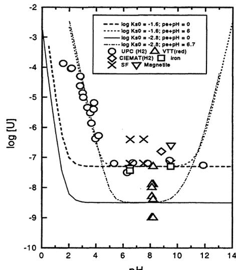
FIGURE 2 : Uranium concentration vs. pH under reducing conditions.
