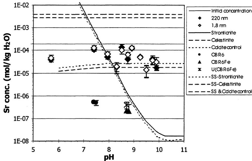
FIGURE IV.2-2 Sr concentration from experimental and calculated data.
