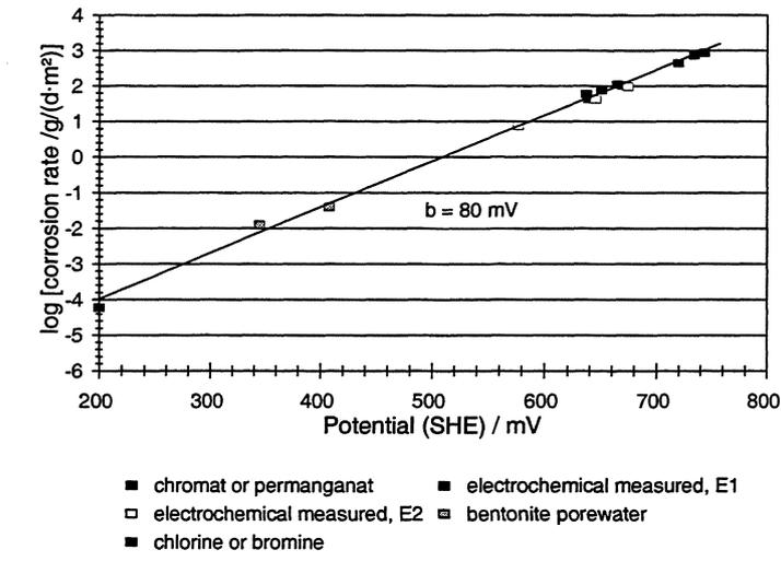
**FIGURE I.6-32: calibration curve for determining the corrosion rates from potentials at  $UO_2$  at  $25^\circ C$ . The specific systems used:  $0.01M K_2Cr_2O_7$ , pH1 in sat. NaCl,  $0.01M KMnO_4$ , pH1 in sat. NaCl, sat. bromine in sat. NaCl, 1 atm chlorine in sat. NaCl. The electrochemical measurements (E1 and E2, two different electrodes), carried out in sat. NaCl**
