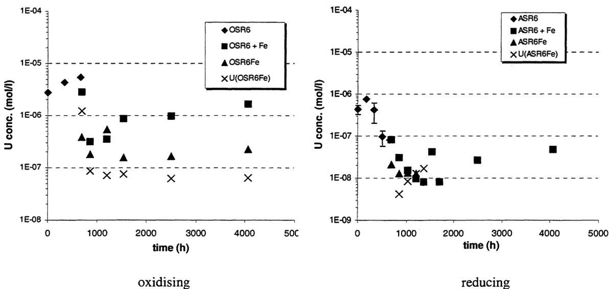
FIGURE III.1-16 Uranium concentration against time under oxidising and reducing conditions respectively in 5m NaCl. Fe is present in the system after 720h leaching time
