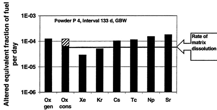
FIGURE I.1 - 9: Comparison of fractional release rates of radionuclides, fission gases and oxygen in granite water and granite bentonite water.
