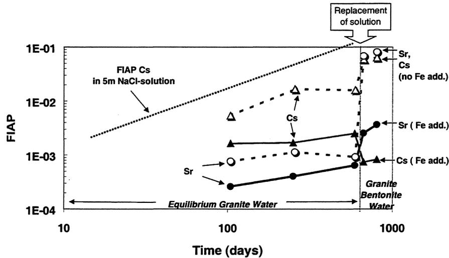
Fig. III.1-4 : Comparison of cumulative Sr and Cs release data from tests with (sample P3) and without iron (P4) present (compare Fig. I.1-8 with Fig. III.1-3)
