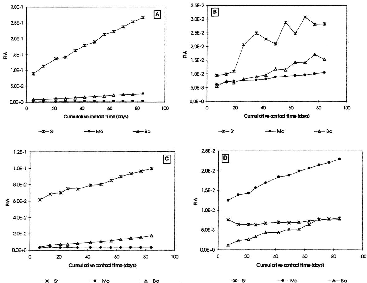
FIGURE III.3.13. Simfuel leaching experiments: FIAc of elements (A) Clay/Granite water medium ; (B) Granite/ Granite water medium. (C) Clay/Clayey water medium; (D) Granite/Clayey water medium.
