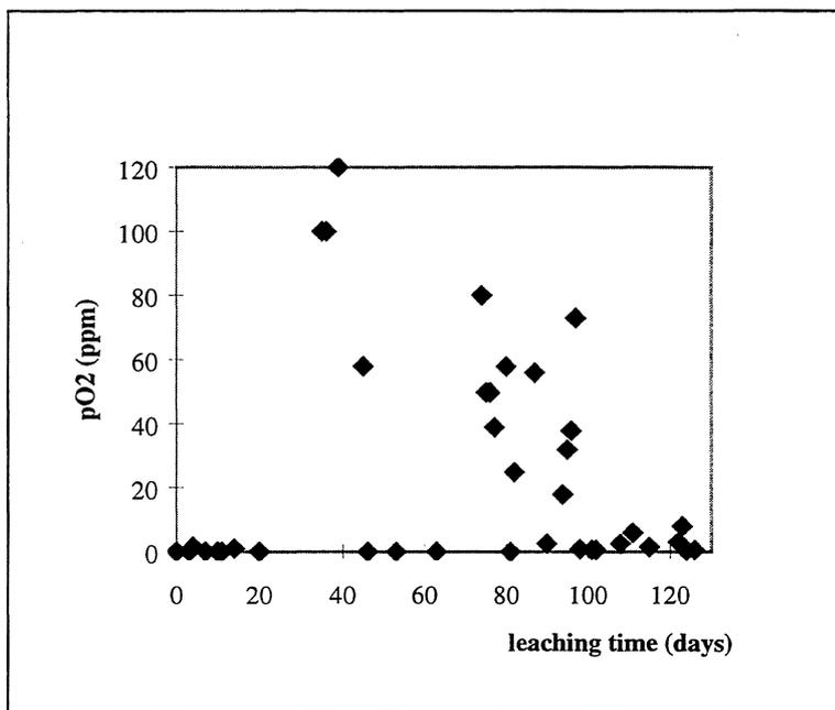
**FIGURE 6 :** *Oxygen partial pressure in Ar glove box during predissolution stage*
