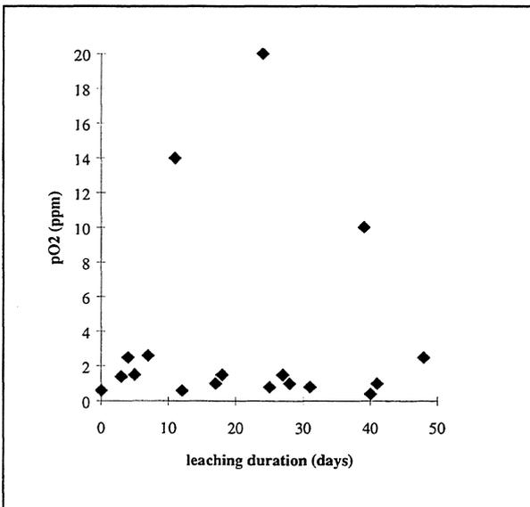
**FIGURE 8 :** Oxygen partial pressure in Ar glove box during dissolution tests.
