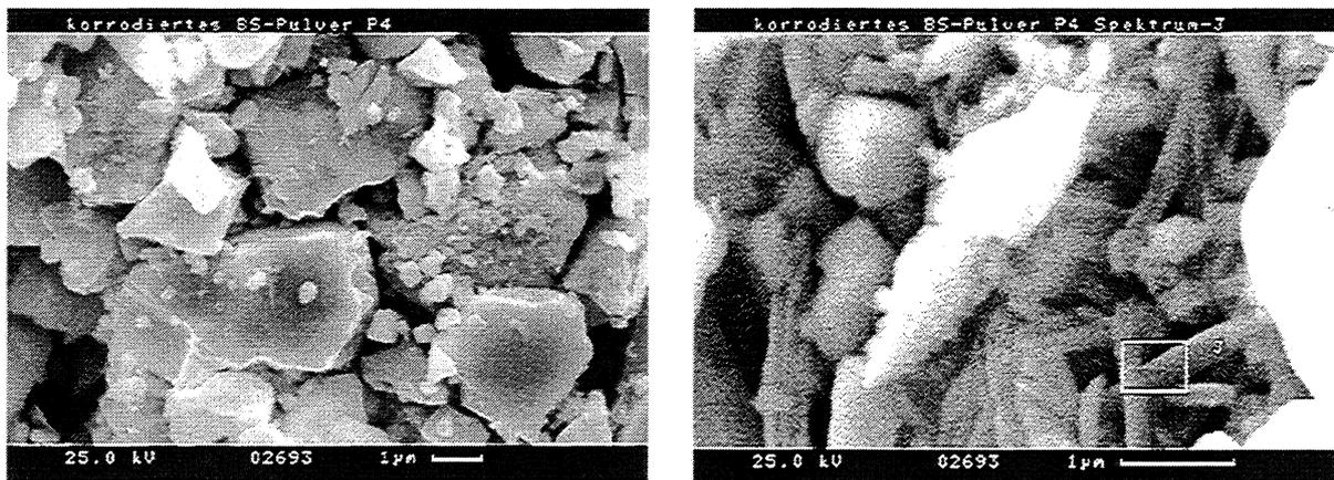
FIGURE I.1 – 12: Spent fuel particles from powder P4 after corrosion over 805 days first in EGW granite water and then in GBW granite bentonite water under Ar / 0,03 %CO<sub>2</sub> atmosphere at 25°C. At position "J" U, Si and O were found by EDX analyses.
