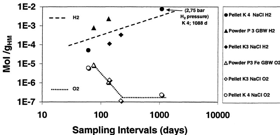
Figure III.1-6: Amounts of hydrogen and oxygen occurring during corrosion of spent fuel in the presence of Fe.
