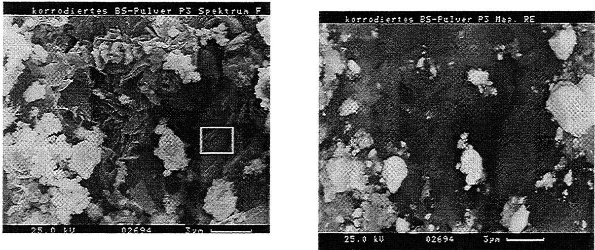
**Figure III.1-9: Newly formed Mg-Fe-O-Phase (dark crystals, white rectangle point of EDX analyses), spent fuel particles, corrosion products. Secondary electron image on the left; back scattered electron image on the right (bright particles: heavy elements [spent fuel particles], grey or dark particles [Fe, Mg,... containing phases]**
