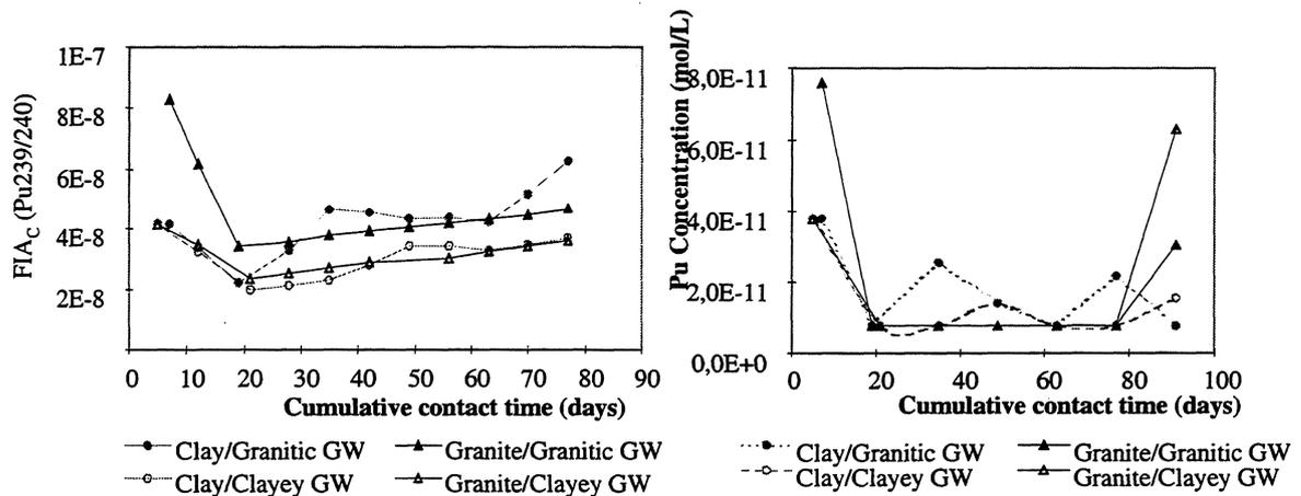
FIGURE III.3.8. Gravelines 3+2 spent fuel experiment:  $^{239+240}\text{Pu}$  FIA<sub>c</sub> and solution concentrations of Pu versus cumulative leaching time, environmental materials and groundwater composition
