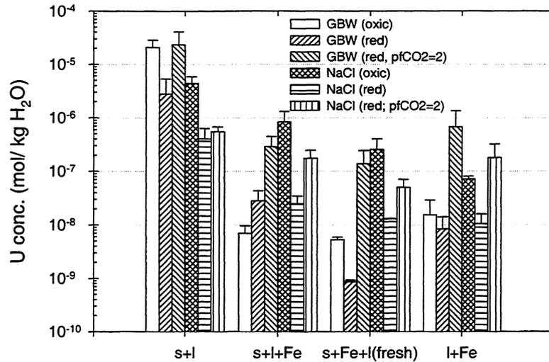
**FIGURE III.1-18: Comparison of U concentrations in solution of various tests with and without iron being present**
