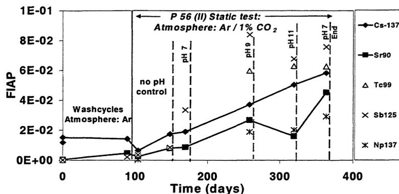
**FIGURE I.1-3: Released fractions of matrix bound radionuclides Cs137, Sr90, Np137, Tc99 as a function of time during dissolution of spent fuel powder P56(II) in 5m NaCl solution under Ar/ 1% CO<sub>2</sub>-Atmosphere**
