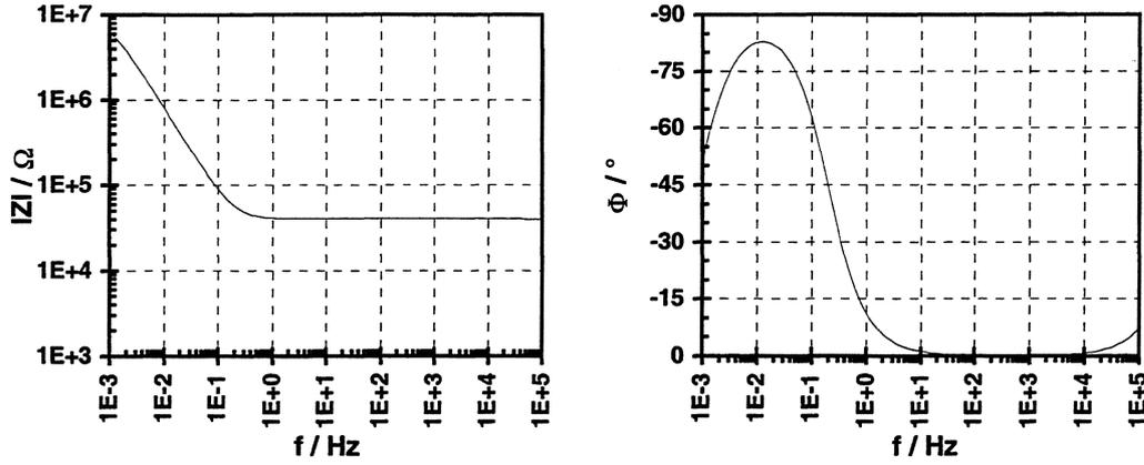
FIGURE. I.6.3: Calculated impedance spectrum for an equivalent circuit of a fuel electrode without any conductive pathways ( $R_{\text{bulk}} = 40 \text{ k}\Omega$ ,  $C_{\text{bulk}} = 5 \text{ pF}$ ,  $R_{\text{pol}} = 10 \text{ M}\Omega$ ,  $C_{\text{D}} = 20 \text{ }\mu\text{F}$ ,  $R_{\Omega} = 100 \text{ }\Omega$ ).
