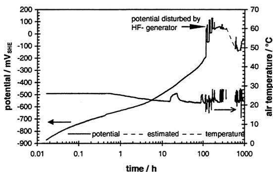
FIGURE. I.6.23: Open circuit potentials of  $\text{UO}_2$  fuel B4 in 95% sat. NaCl solution (initial pH = 7.3,  $\text{C}(\text{O}_2) < 2 \text{ ppm}$ ).
