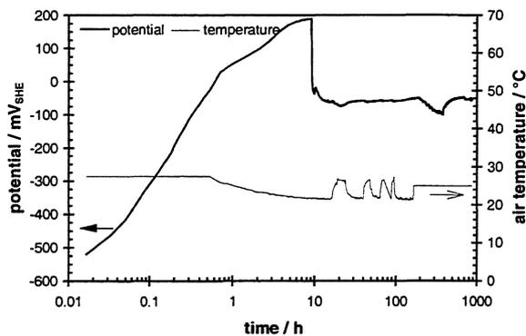
Fig. 13: Open circuit potential of used UO<sub>2</sub> fuel B4 (burn-up: 53.1 GWd/t) and related temperature, in 95% saturated NaCl solution ( $E_{corr}^{max} = 190 \text{ mV}_{SHE}$ ,  $T: 22 - 28^\circ\text{C}$ ,  $C(\text{O}_2) < 2 \text{ ppm}$ , initial pH 7.2)
