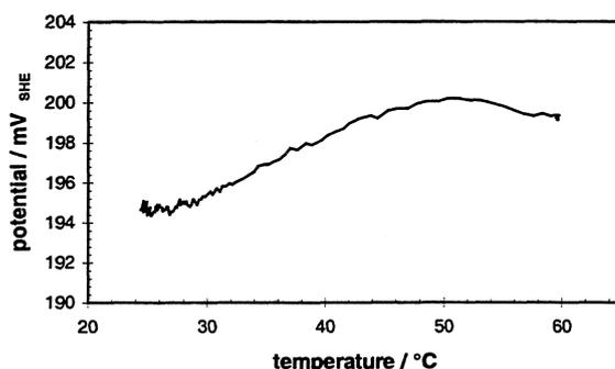
**FIGURE I.6.21: Temperature stability of a double junction Ag/AgCl gel electrode measured in simulated ground water vs. a saturated calomel electrode at 22°C.**
