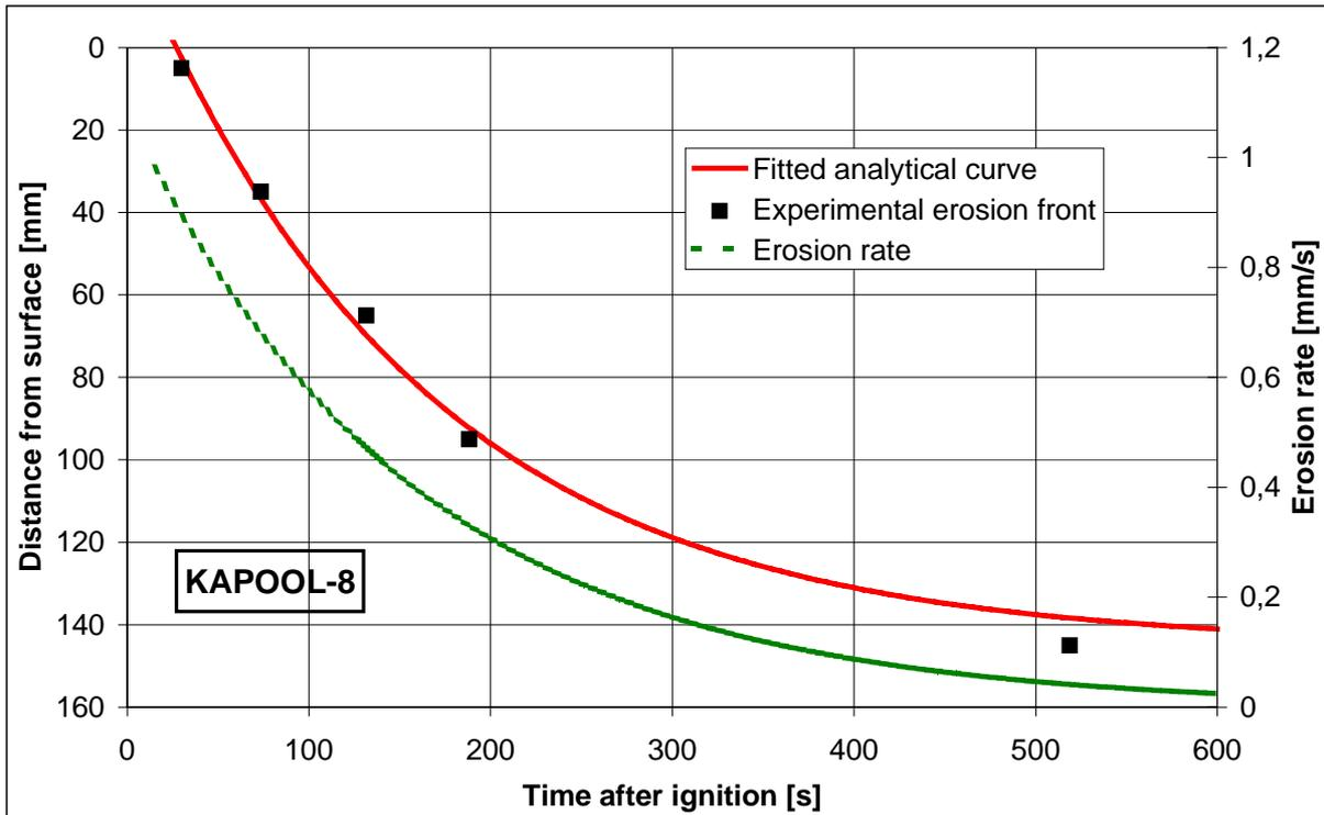
**Figure 18:** Erosion front with fitted analytical curve and erosion rate
