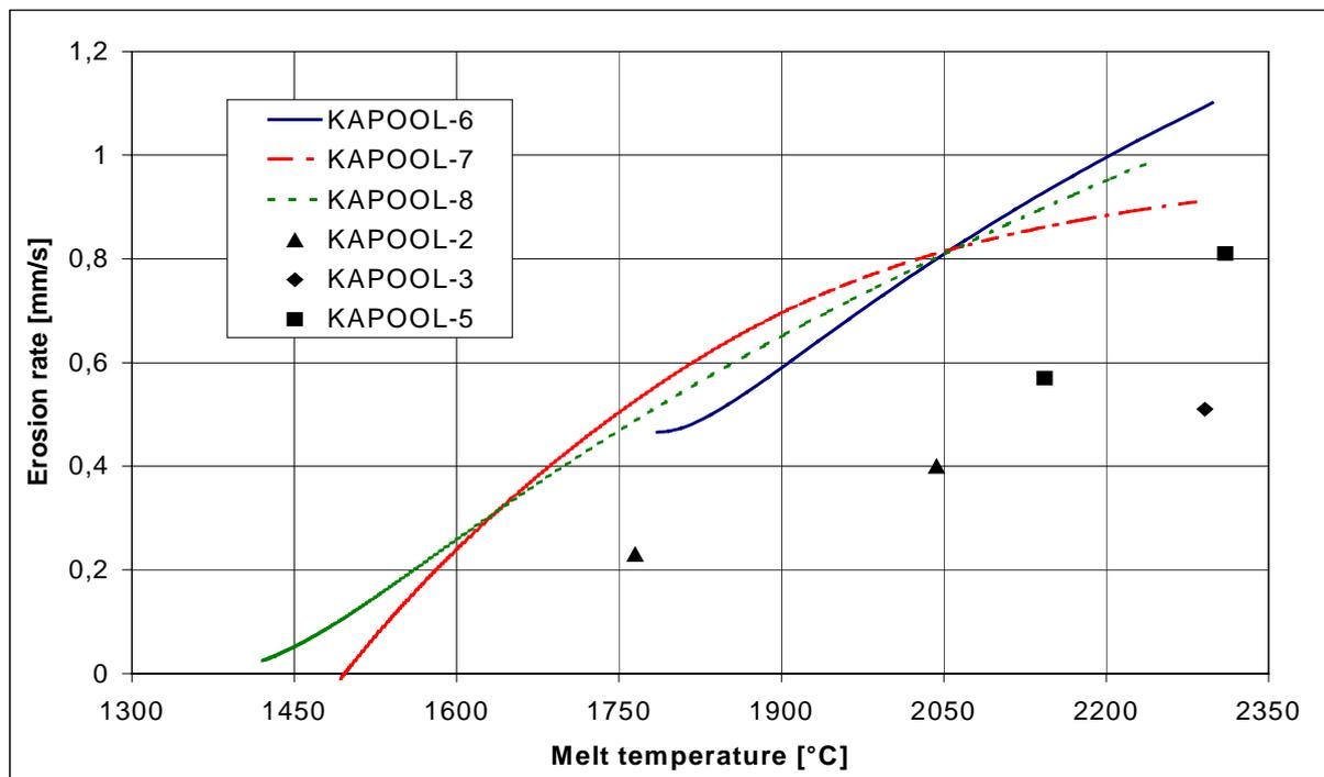
**Figure 19:** Erosion rates for the glass-concrete (KAPOOL 2/3/5) and the sacrificial concrete VM281Q (KAPOOL 6/7/8) as a function of the iron melt temperature
