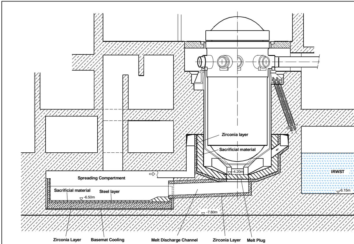
**Figure 1:** Concept of the EPR core catcher
