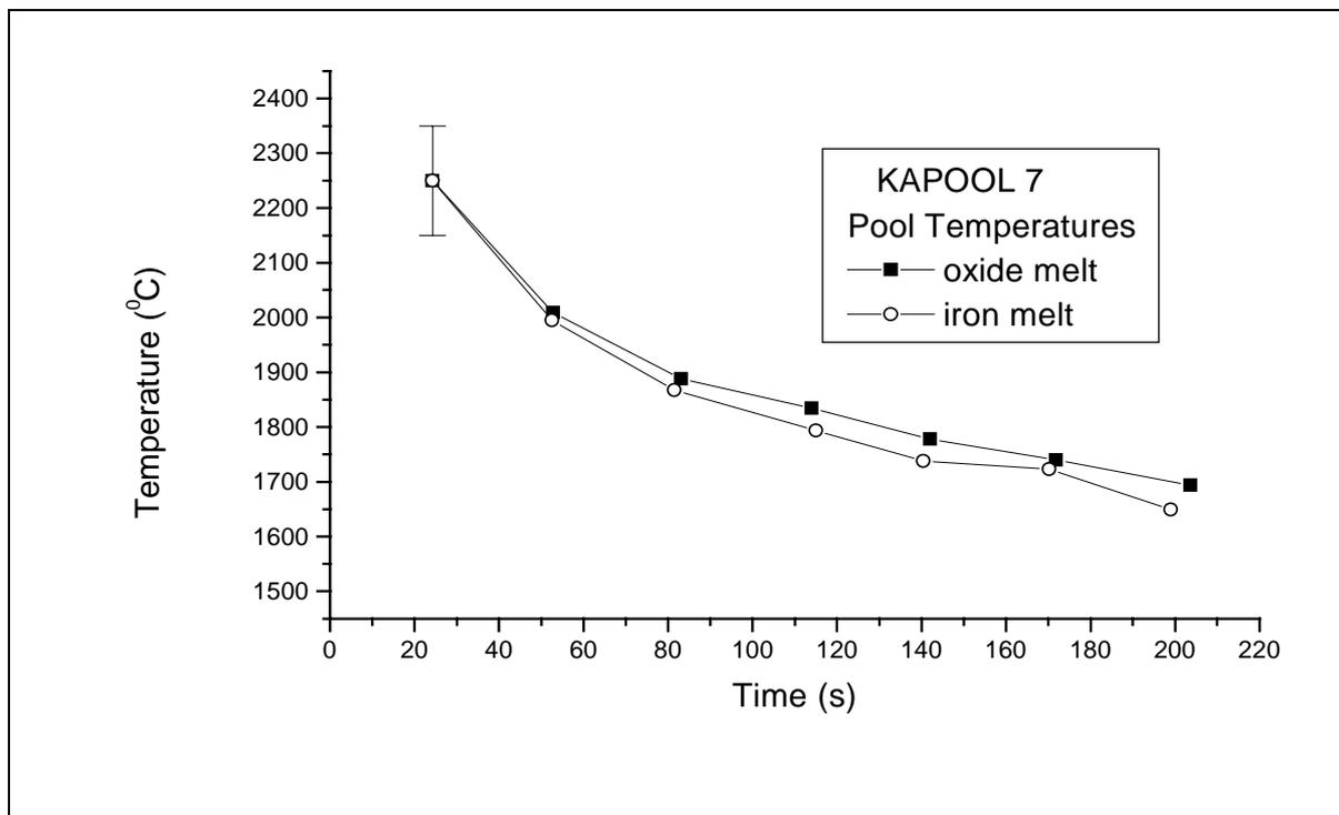
**Figure 8:** Transient melt temperatures in the iron- and oxide pools of KAPOOL 7
