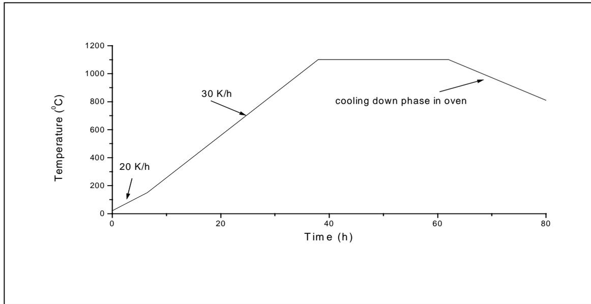
**Figure 2:** Required temperature treatment of insulating ceramics
