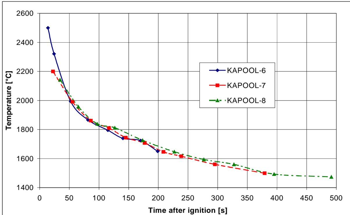
**Figure 12:** Comparison of the iron pool temperatures in all three KAPOOL tests
