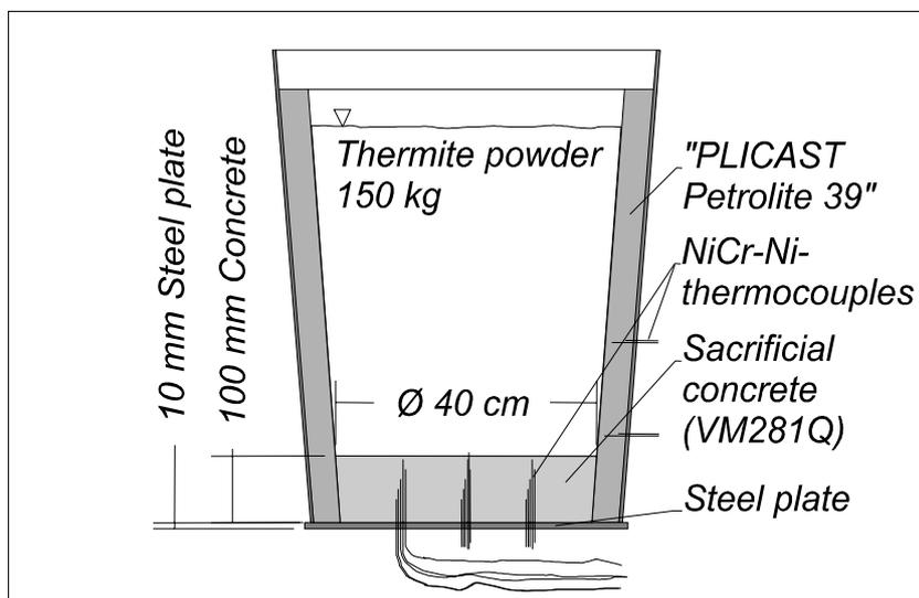
**Figure 3:** Setup of the KAPOOL 6 container
