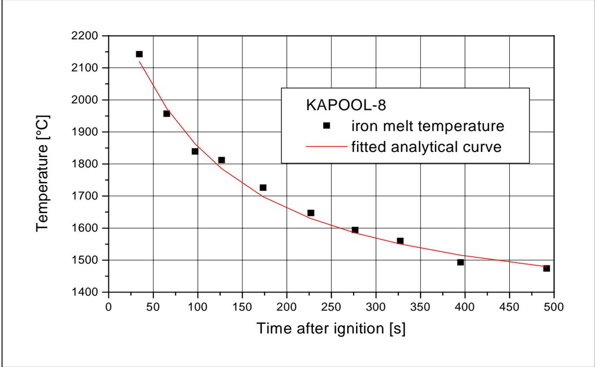
**Figure 15:** Transient iron melt temperature, included is the fitted analytical curve
