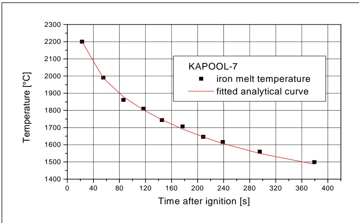
**Figure 14:** Transient iron melt temperature, included is the fitted analytical curve
