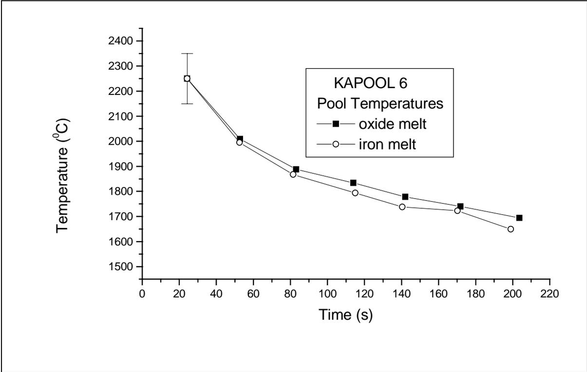
**Figure 4:** Transient iron- and oxide melt temperatures in KAPOOL 6
