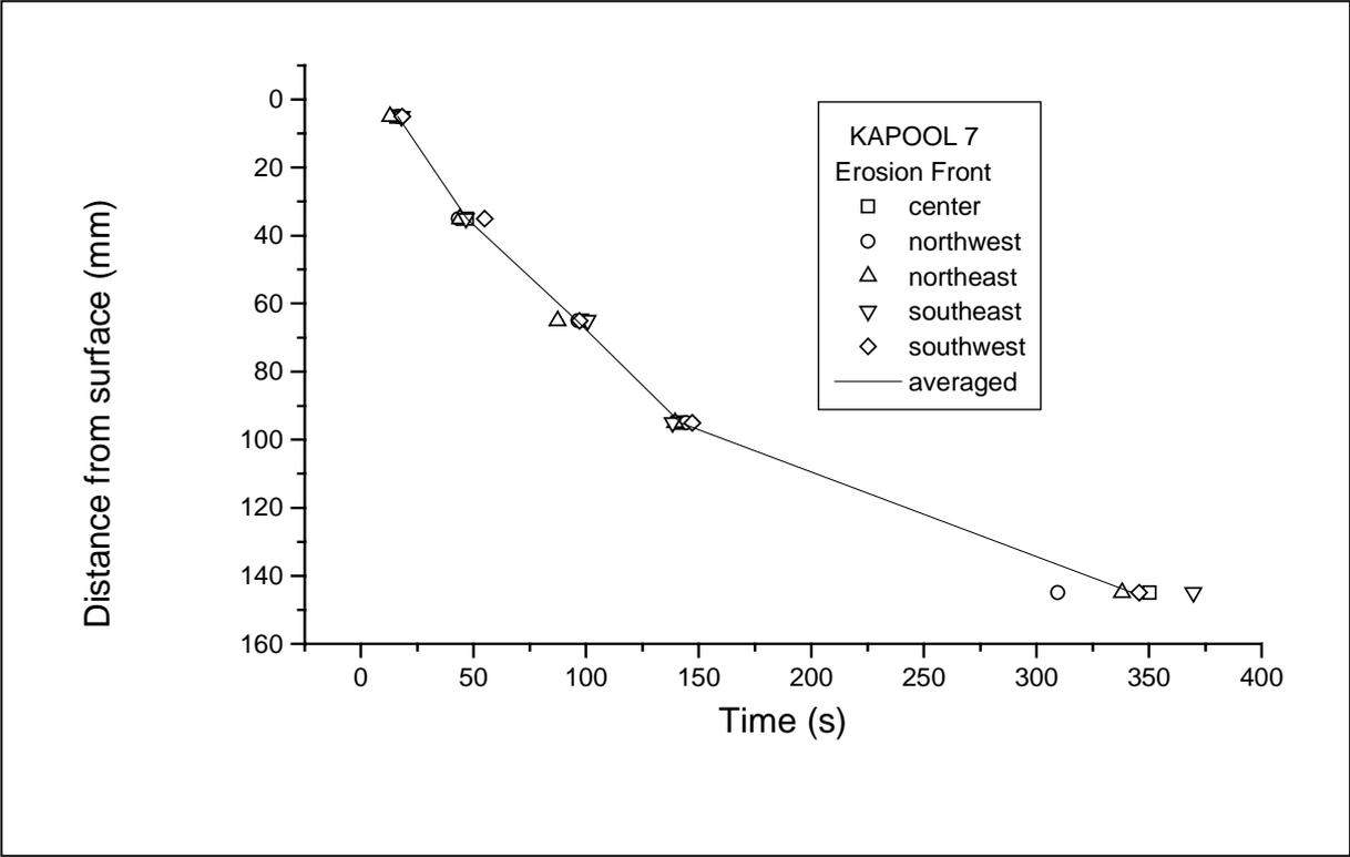
**Figure 7:** Erosion front in the sacrificial concrete of KAPOOL 7
