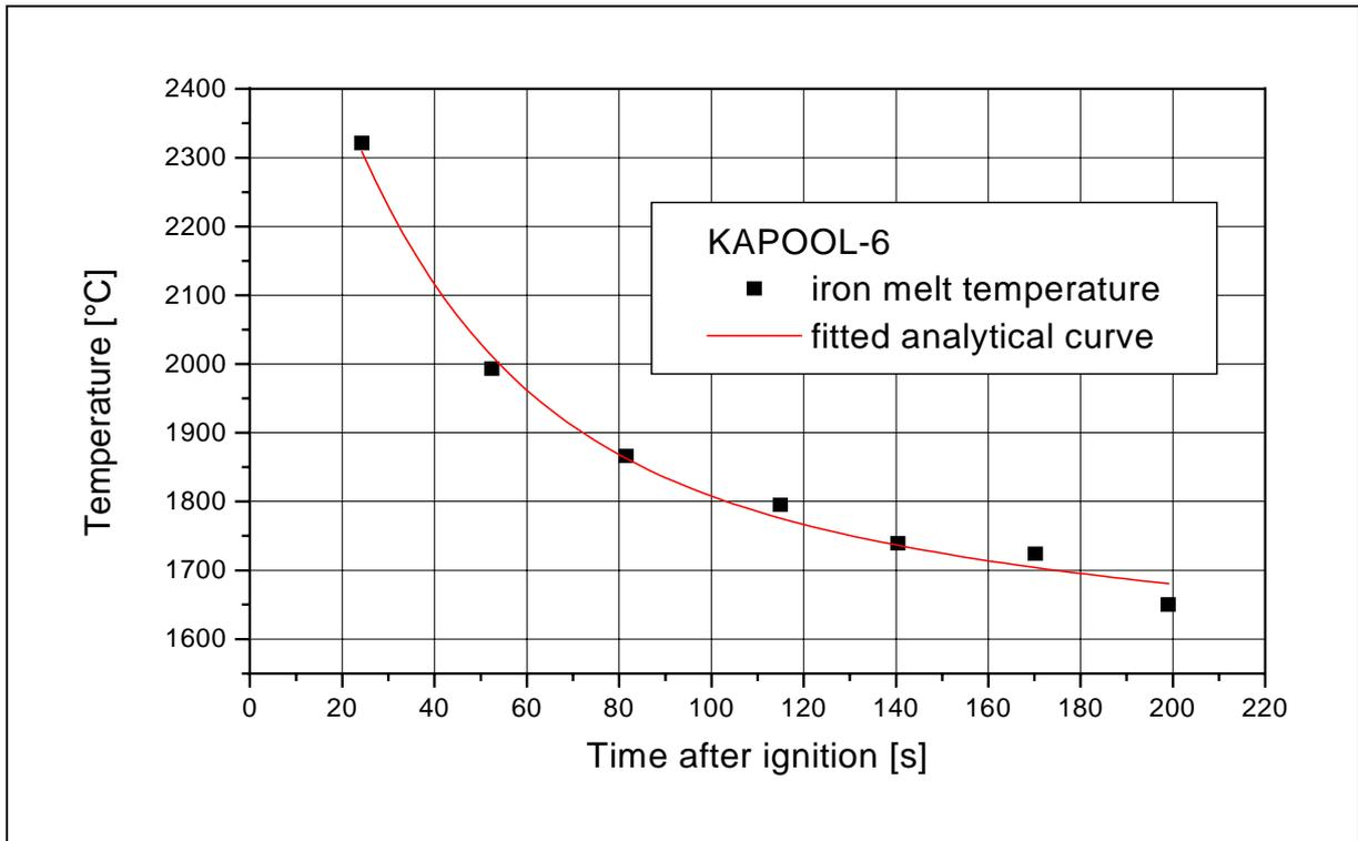
**Figure 13:** Transient iron melt temperature, included is the fitted analytical curve
