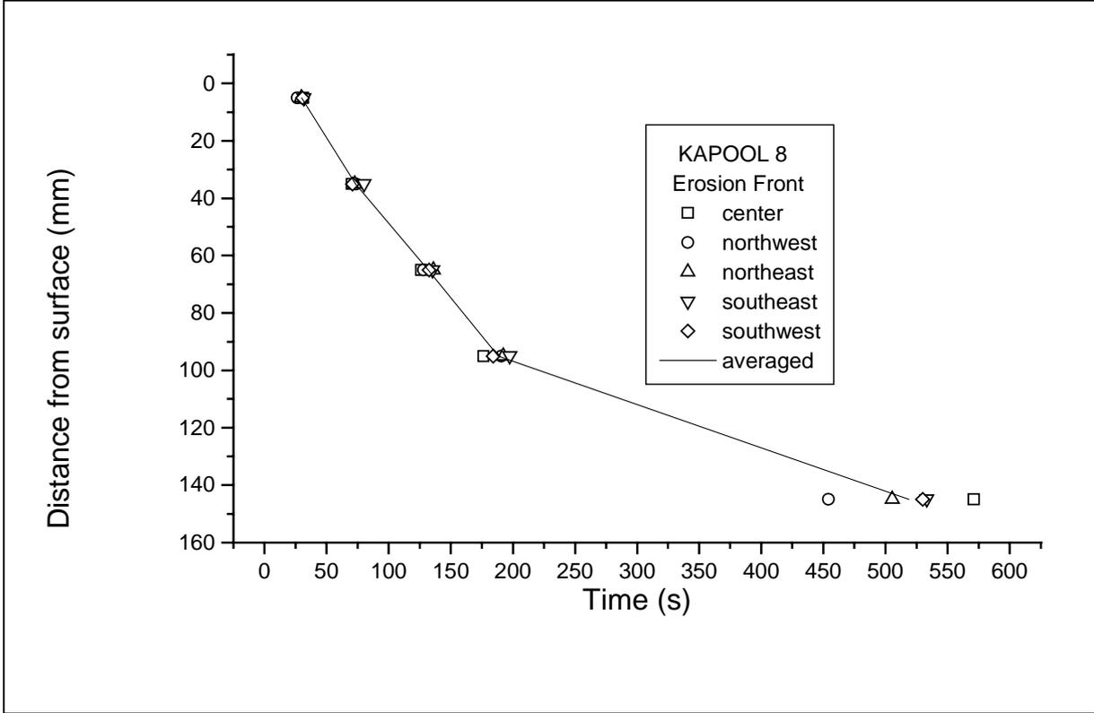
**Figure 10:** Erosion front in the sacrificial concrete of KAPOOL 8
