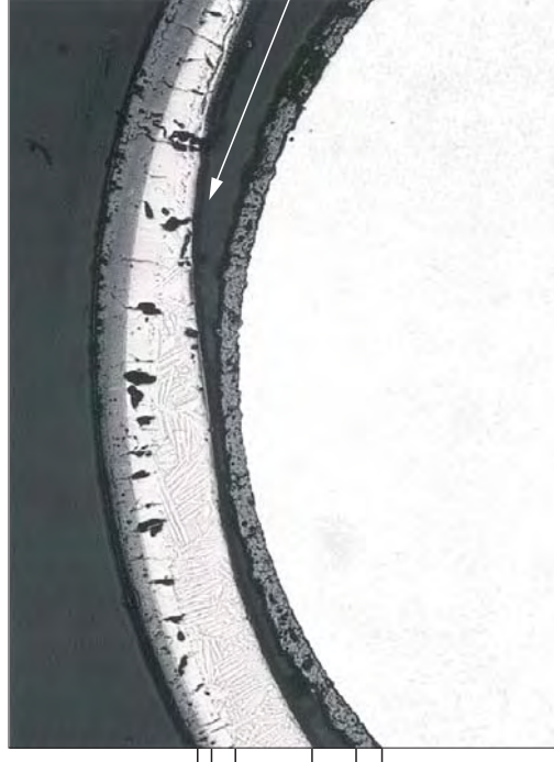
Melting and relocation of Zry-4 cladding
