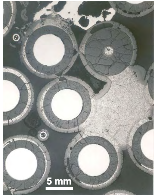
Interaction of relocated melt with ZrO 2 shells
