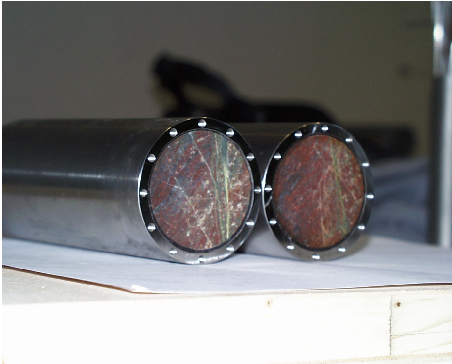
Fig. 13 ASPÖ core sample embedded in a stainless steel sleeve; top and bottom ends.
