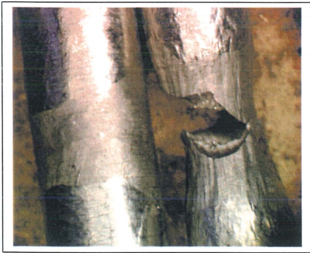
Figure 45. Cast material with the laser beam weld zone of the left hand specimen show marginal necking inside the weld metal and a fracture occurrence outside the weld metal (inside the base metal of the cast steel). The right hand specimen consisting of forged material and the laser beam weld zone shows the fracture event inside the weld metal. The weld metal's yield strength is inferior to the base metal.
