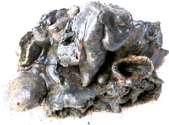
Fig. 30: Particle collected after the test showing broken edges and a shrinking crack.
