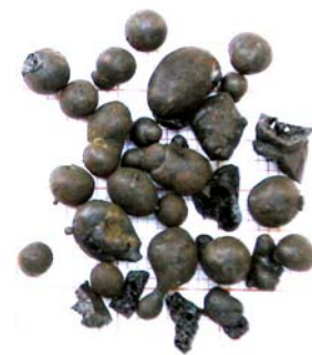
Fig. 38: Particles sampled at the fragment catcher, sieve fraction 5 – 10 mm.
