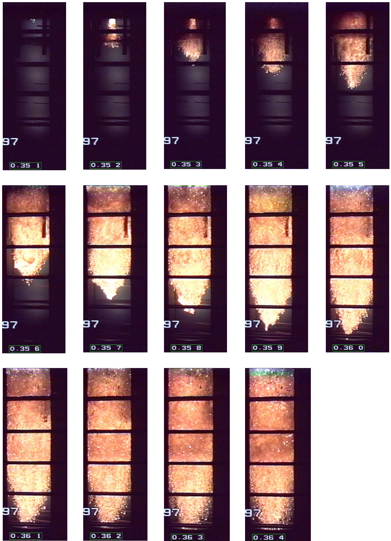
Fig. 2: Selected frames of the video film taken during test PM13. The time difference between two frames is 0.100 s, where the second frame corresponds to time about zero.
