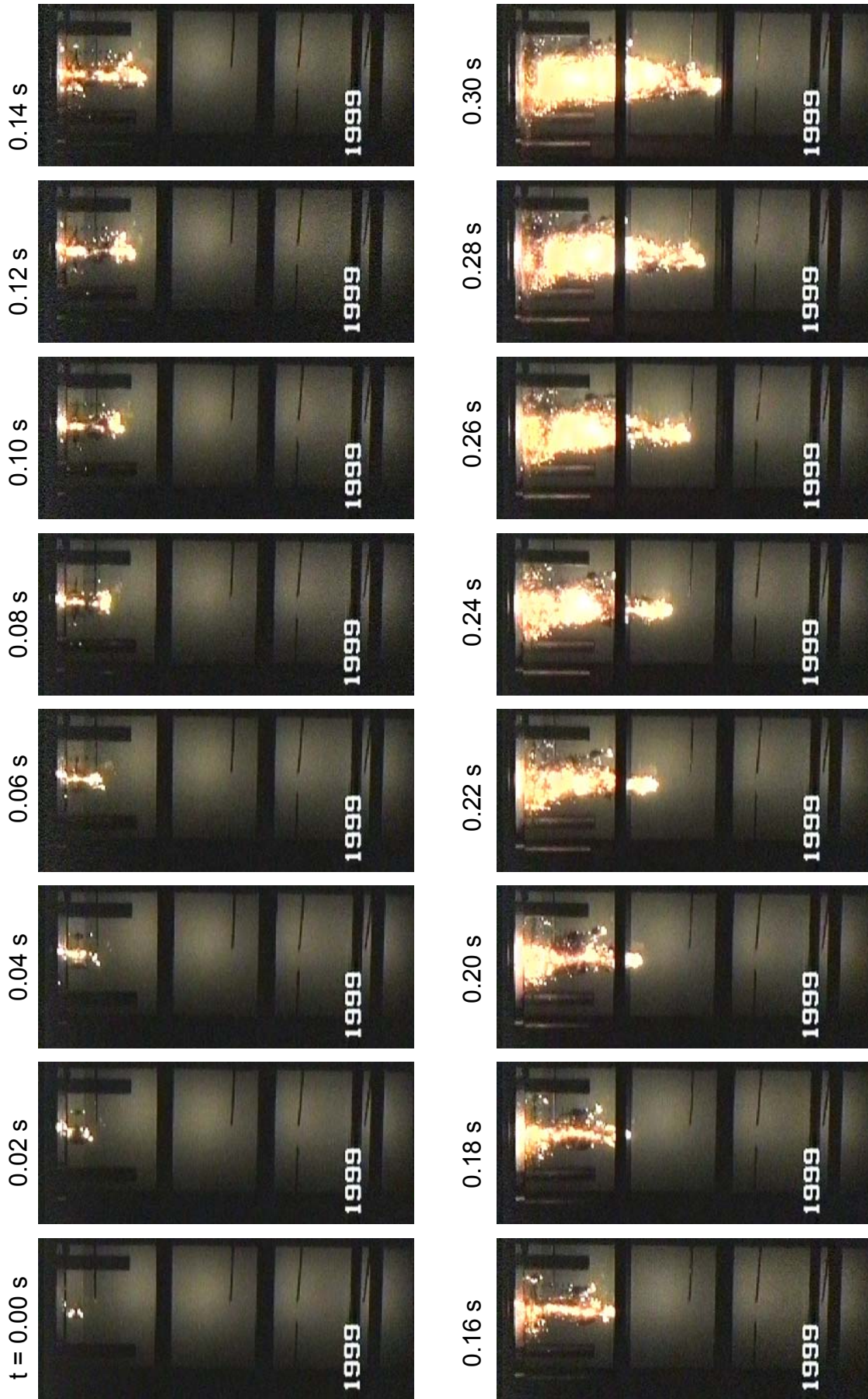
Fig. D1: PM18. Progression of the interaction zone under the condition of moderate initial water subcooling (26 K). Part 1: smaller time steps.
