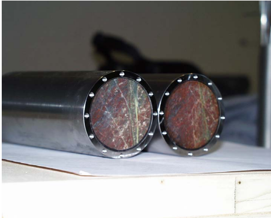
Fig. 1 Äspö core samples embedded in a stainless steel sleeve; top and bottom ends.
