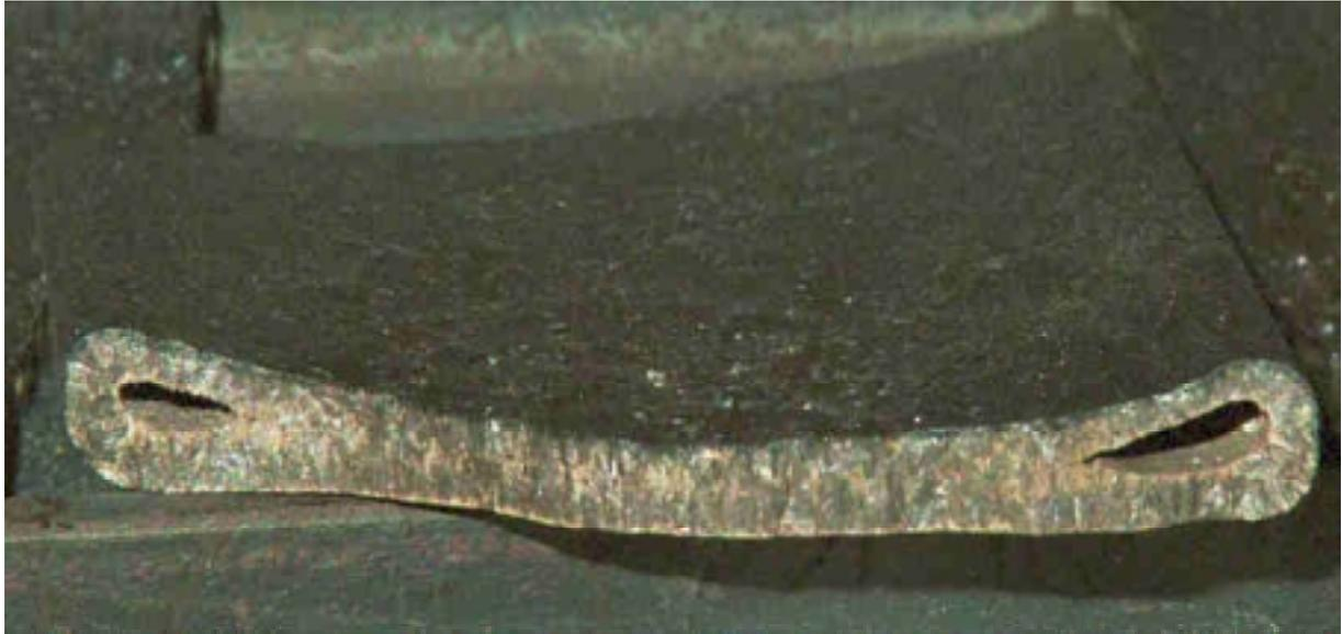
Figure 9: Cross-section of the solidified melt after the test
