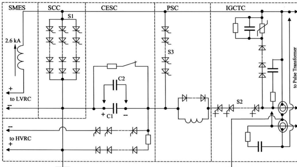
Fig. 2-3: Diagram of cabinets SSC, CESC, PSC, IGCTC and the SMES
