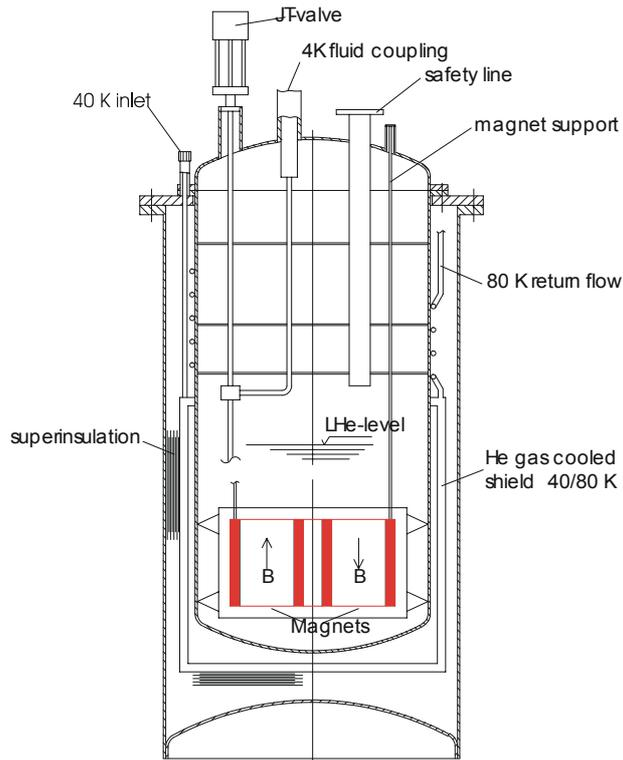
Fig. 3 SMES magnet system; 2 solenoids with antiparallel field in their cryostat (Ø 1.25 m).
