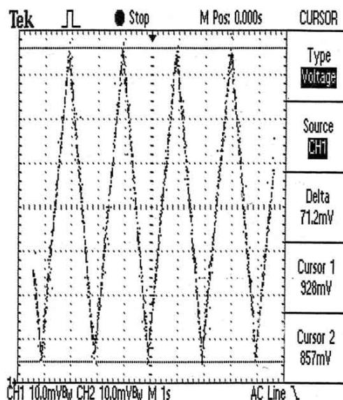
Fig. 8 Current in the load (46 mH).  $I_{max} = 650$  A,  $I = 50$  A,  $T = 1$  s
