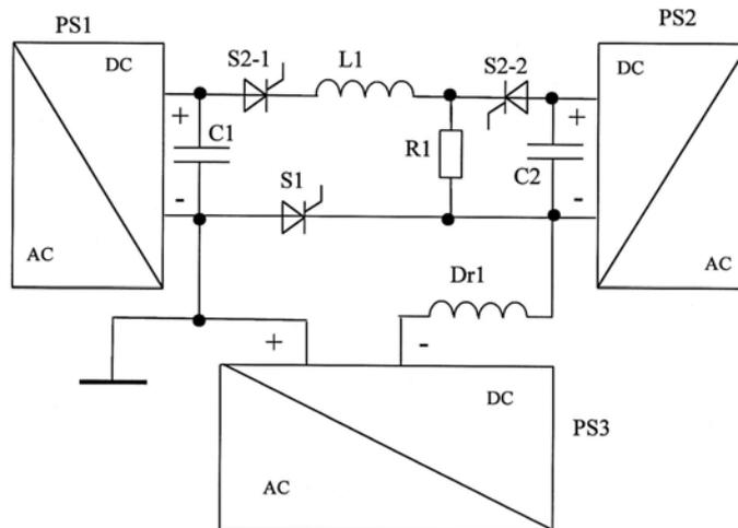
Fig. 10 Simplified circuit diagram for the 1 MW modulator test arrangement (PS1 is the modulator high-voltage power supply, PS3 is the modulator low-voltage power supply, PS2 is an extra power supply made available by ESTEL, Dr1 is a normal conducting inductance simulating the SMES, L1 replaces the leakage inductance of the pulse transformer, S1 is the SMES thyristor switch, S2-1 and S2-2 together simulate the operation of the IGCT switch)
