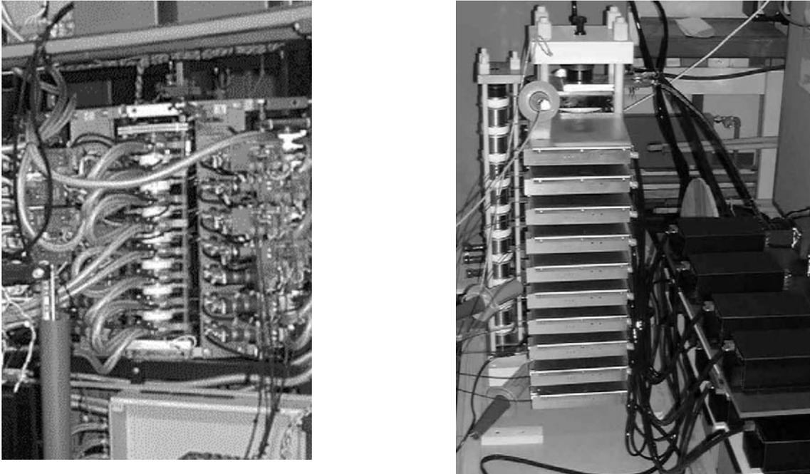
Fig. 5 Thyristor switch S1 (left) and IGCT switch S2 (right) during pre-testing on the manufacturer's site.
