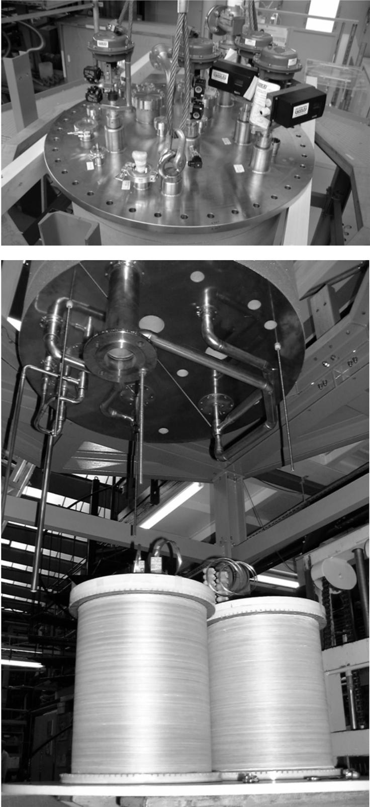
Fig. 7: SMES Magnets (bottom) and Cryostat Top Flange (top)
