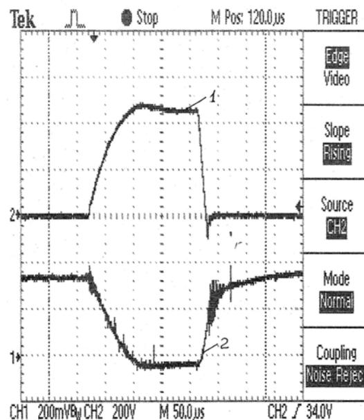
Fig. 11: Currents in the thyristor switches S2-1 (trace1) and S1 (trace 2) of the 1 MW MTA (bigger time unit 50  $\mu$ s, bigger current unit 100 A)
