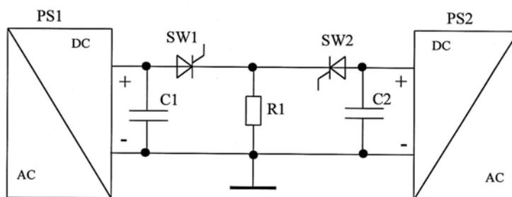
Fig. 9 Simplified circuit diagram for the dynamic test of the High-Voltage Power Supply
