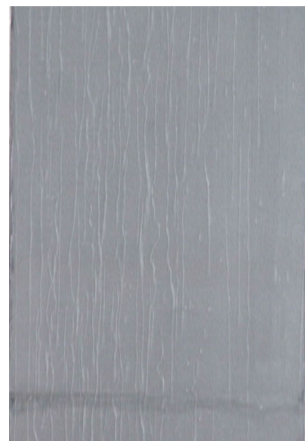
Figure 3.37: Water film on the heated wall with EISENGLIMMER
