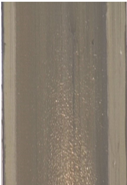
Figure 3.36: Water film on the heated wall with Carbo Zinc®
