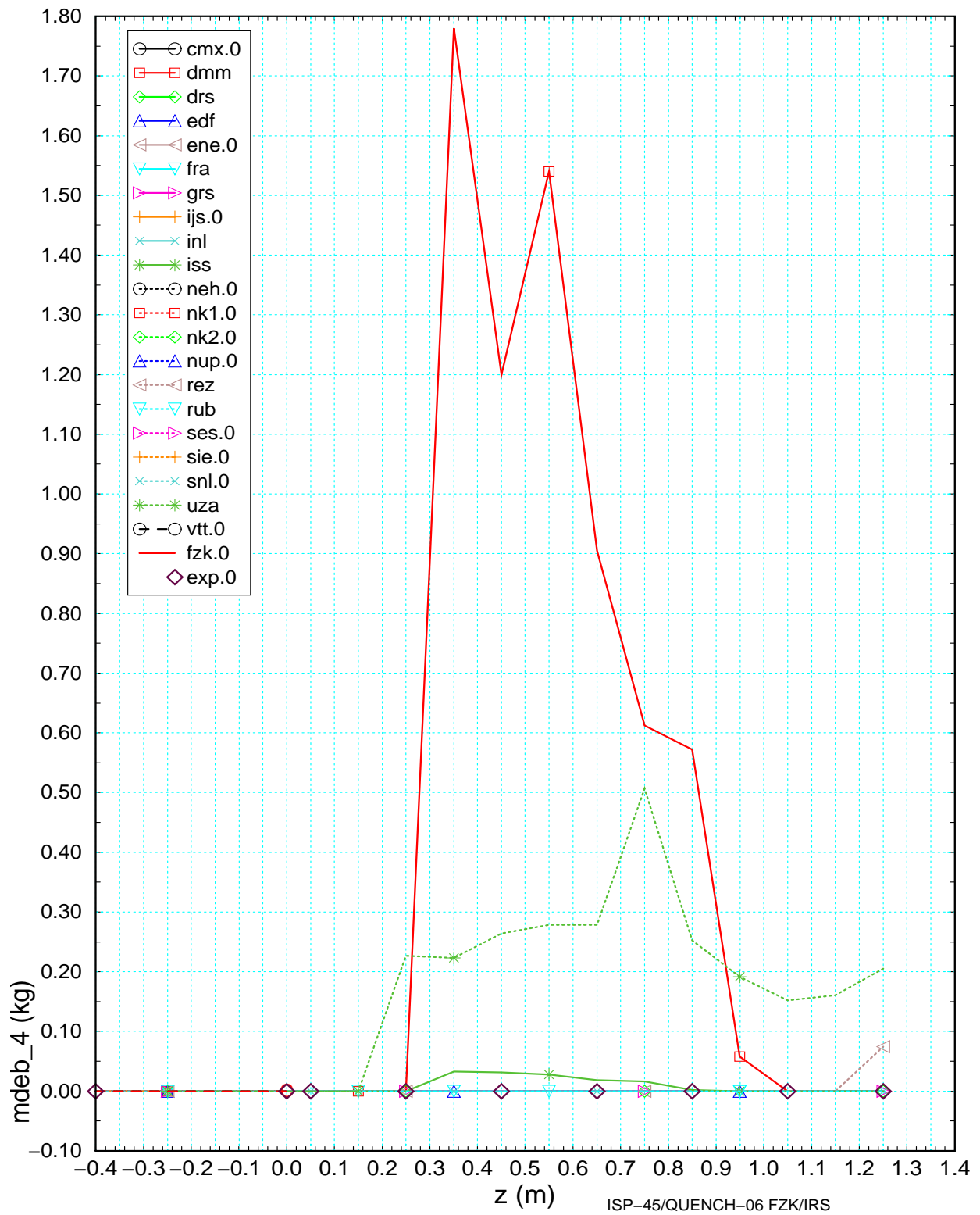
Figure 4.43 Axial profile of accumulated debris calculated by the participants for t=8000 s compared to experimental results.
