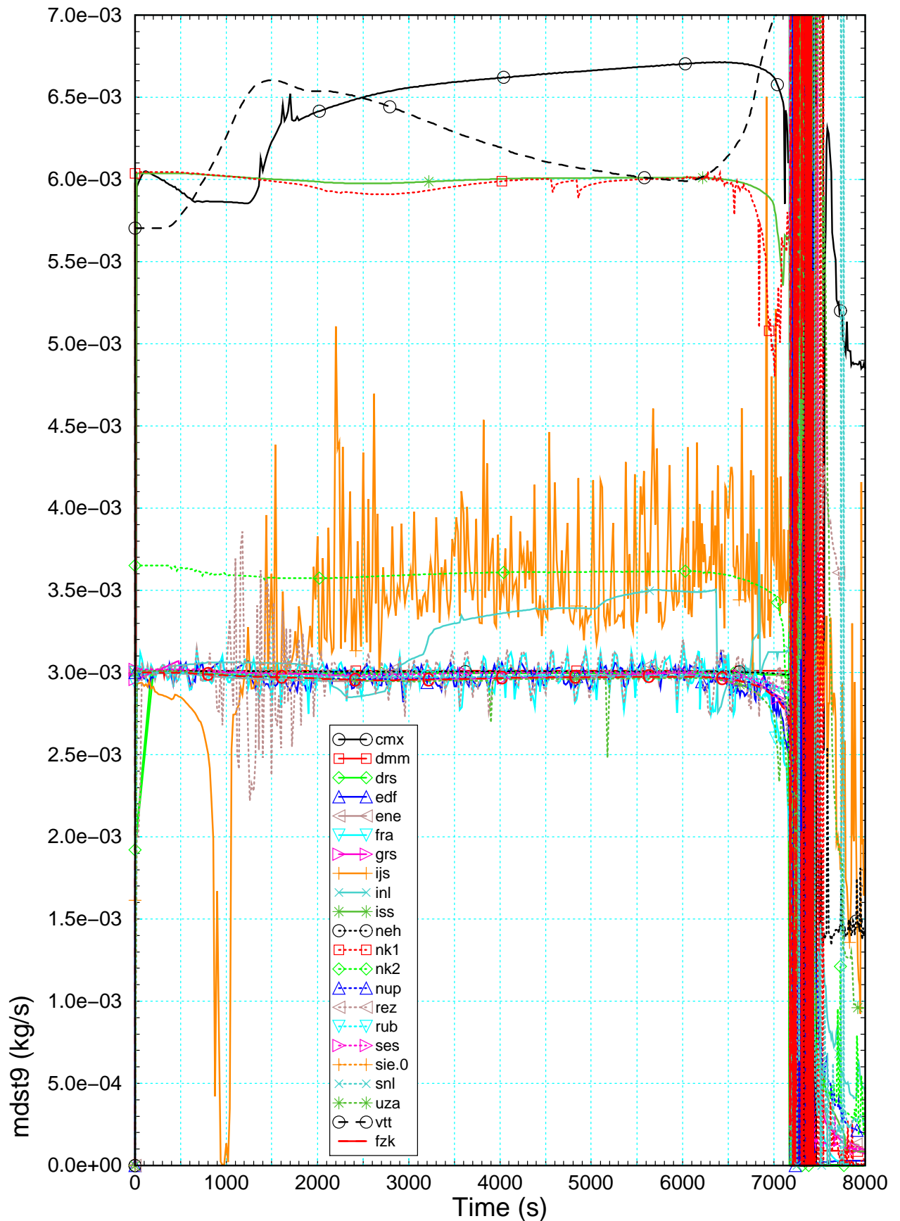
Figure 4.7 Steam mass flow rate (mdst9) at the bundle outlet calculated by participants and by FZK post-test analyses (-C-).
