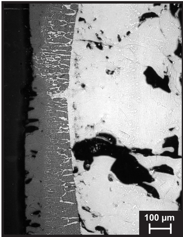
Cladding near TC position
