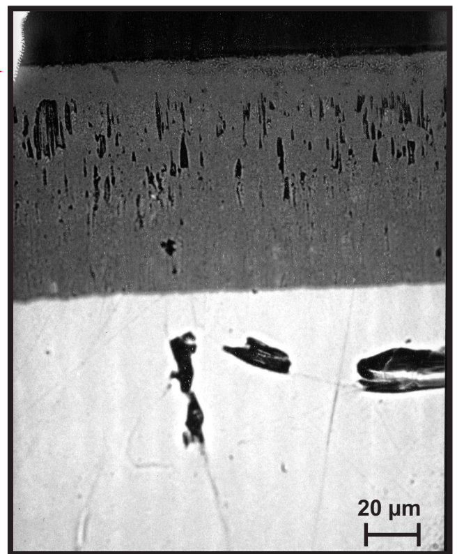
Rod No. 2 (inner row) , peak temperature below 1800 K.
