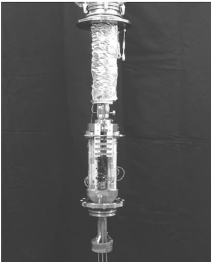
Fig. 1: 10 kA HTS current lead consisting of two conduction-cooled Bi-2212 tubes and a gas-cooled copper wire bundle heat exchanger
