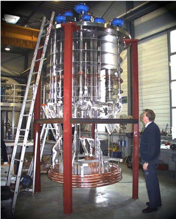
Fig. 2: Internal structures of 3000 l control cryostat
