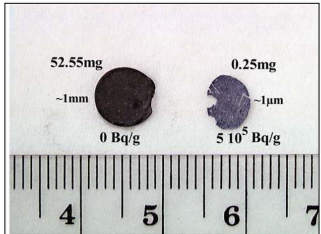
Fig. 2: Thick and thin disc after the RF heating under moist argon
