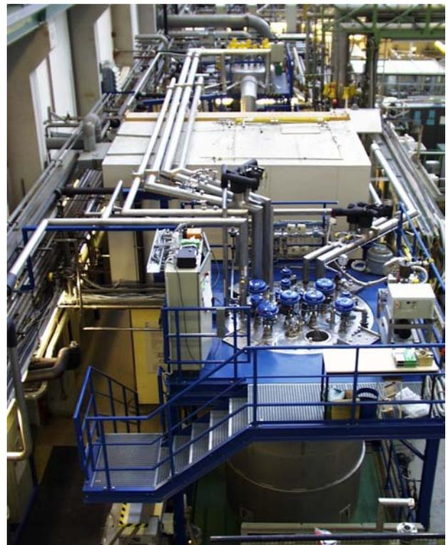
Fig. 3: TIMO facility showing new 3000 l control cryostat and cryotransfer line to cold valves box
