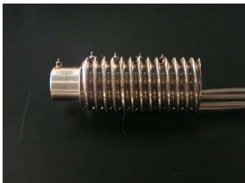
Fig. 6: Five pole electric potential probe for installation in the test sections (b) and (c)
