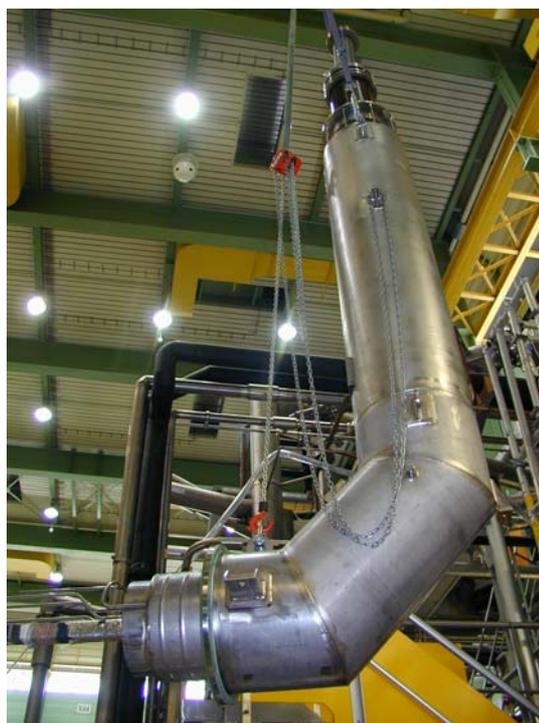
Fig. 1: One of the assembled power feedthroughs ready for installation at the flange of the TOSKA vacuum vessel
