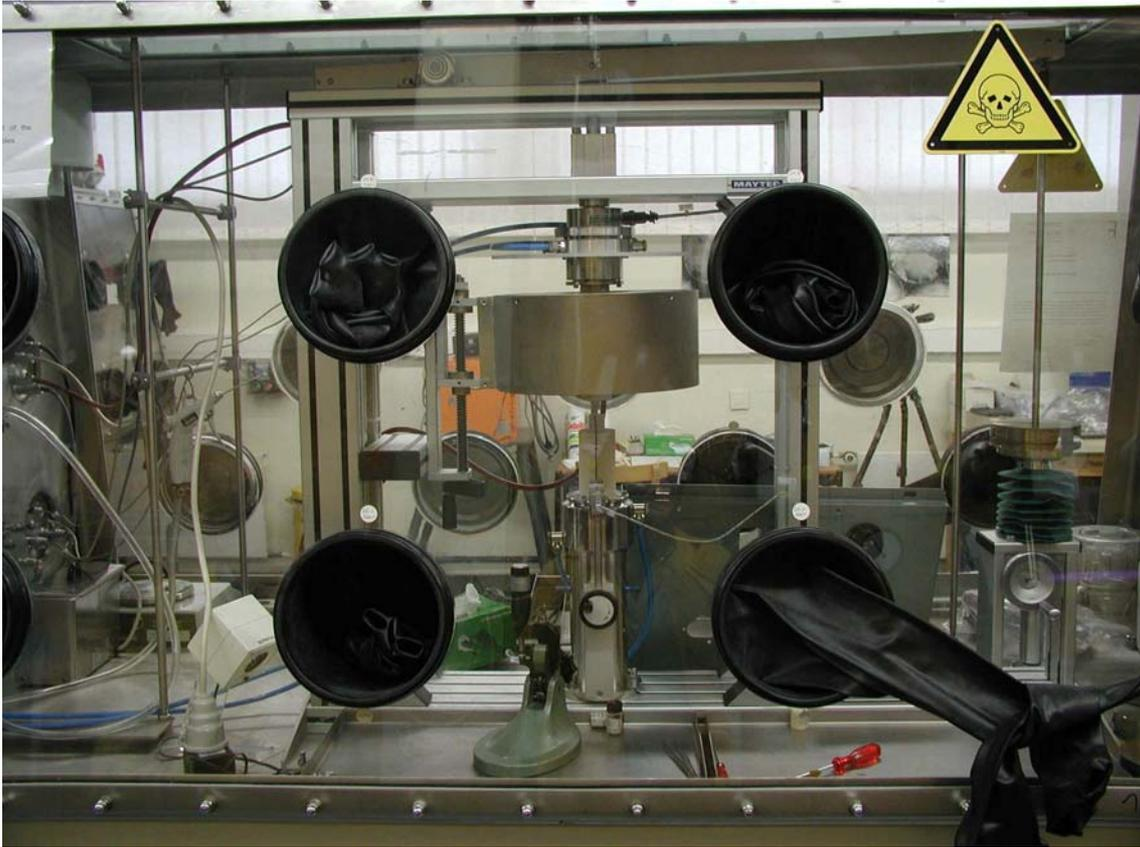
Fig. 2: High Temperature Creep Measurement on Be-Pebbles
