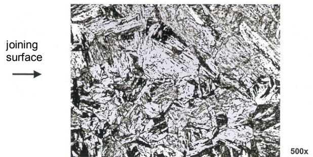
FW specimen with dry-milled joining surface
