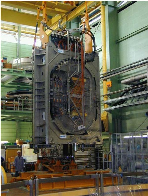
Fig. 2: The ITER TFMC configuration in the TOSKA assembling area
