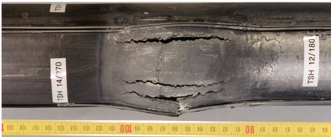
Fig. 37: QUENCH-05; Posttest appearance of the shroud at different orientations
