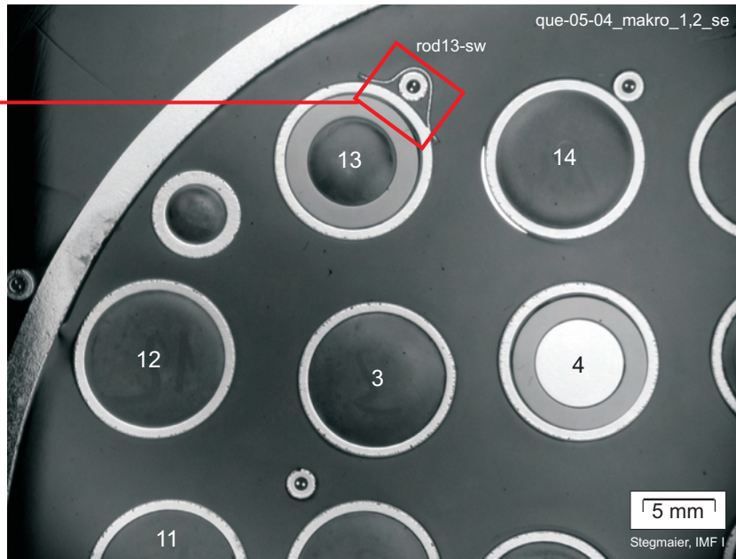
TC attachment clamp at welding position; crack surfaces oxidized.
