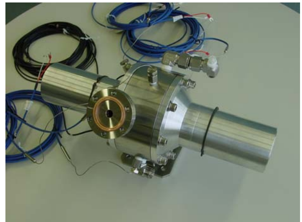
Fig. 6: Complete view of the diamond window housing.
