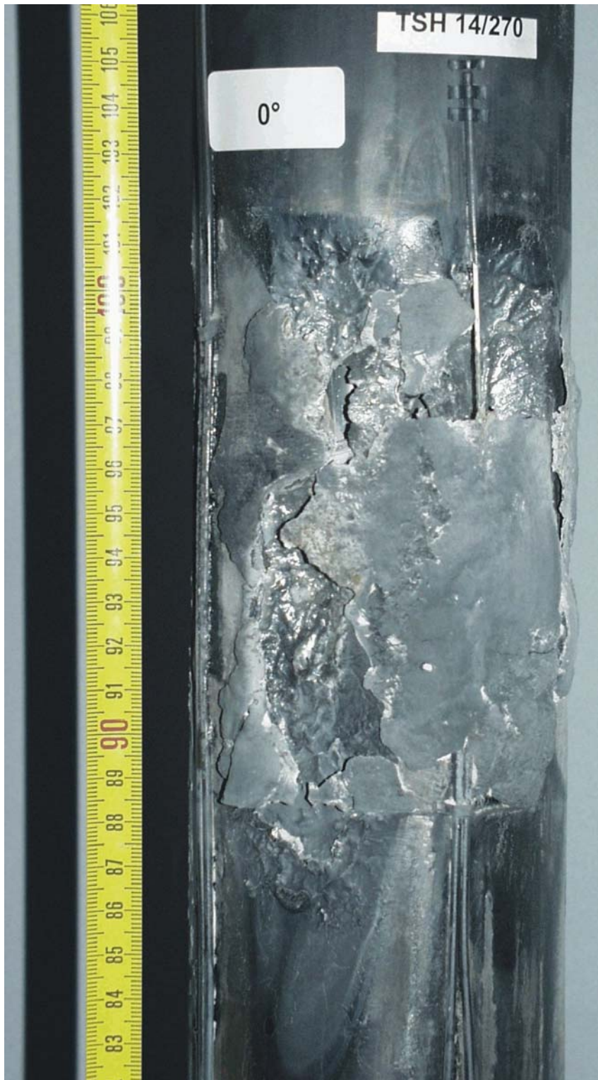
Figure 3.4 Shroud failure location above 0.85 m.
