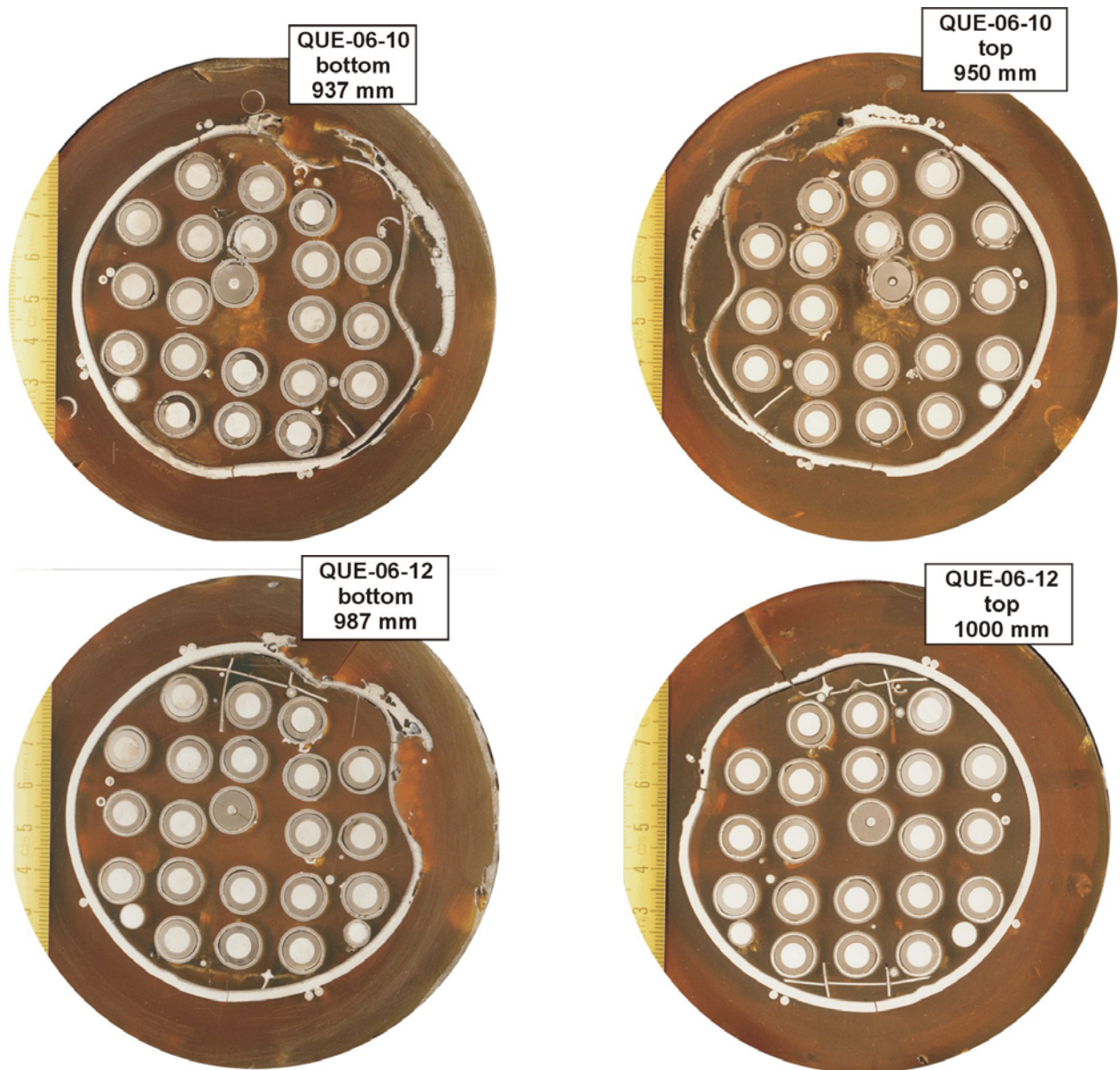
Figure 3.6 Bundle cross sections: top: at 0.937 m and 0.95 m, and bottom 0.987 m and 1.0 m.
