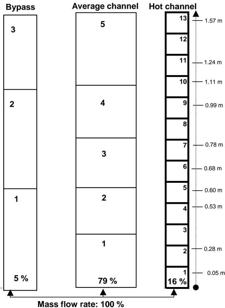
Figure 3-2 Core mass flow rate redistribution among the hot, average and bypass channels
