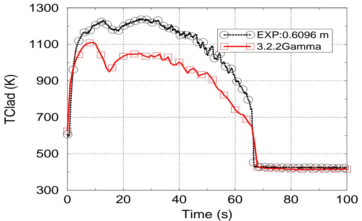
Figure 4-12 Predicted and measured cladding temperature at 0.53 and 0.6 m (hot channel)
