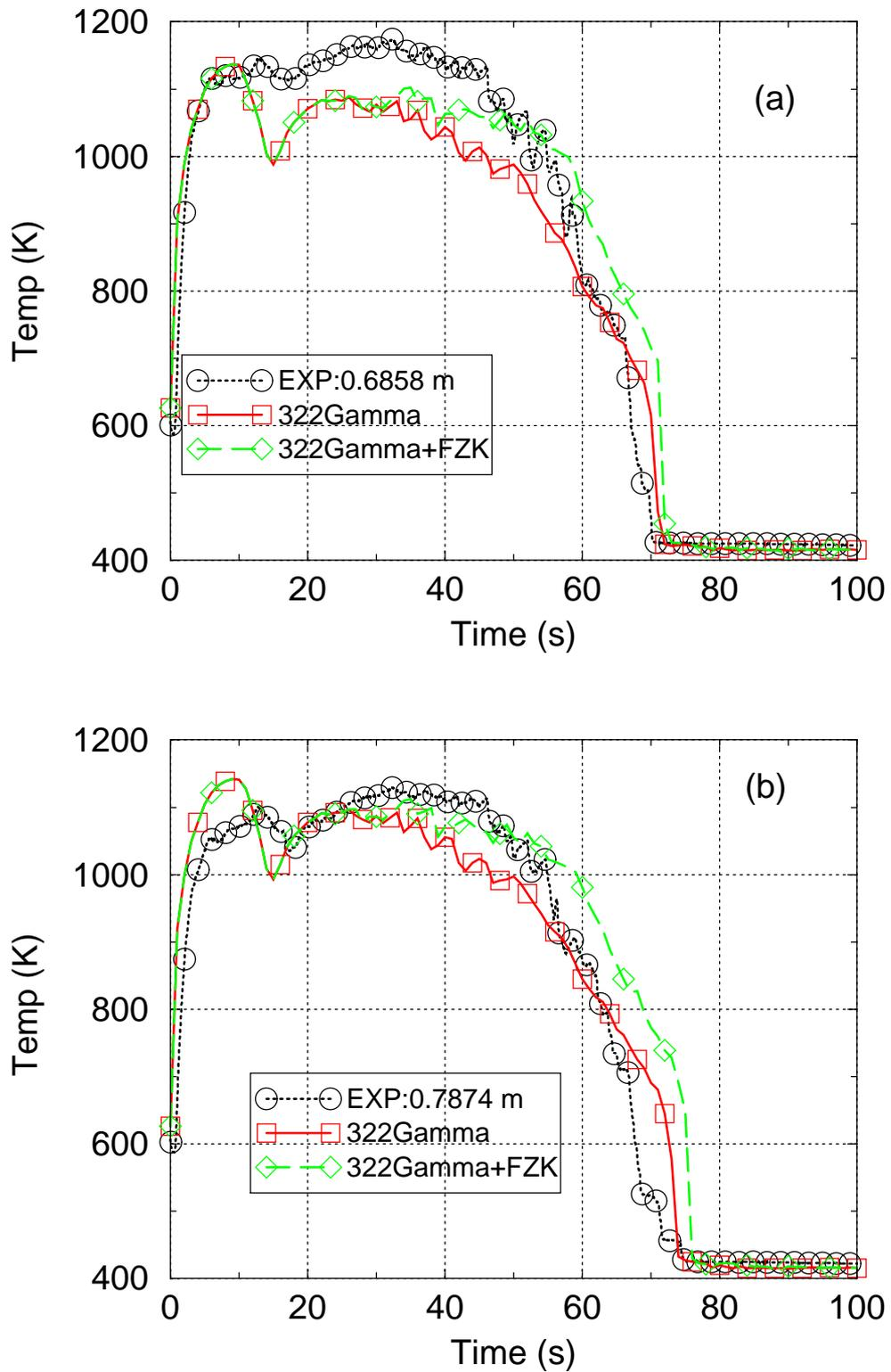
Figure 4-21 Comparison of data with predictions of cladding temperature
