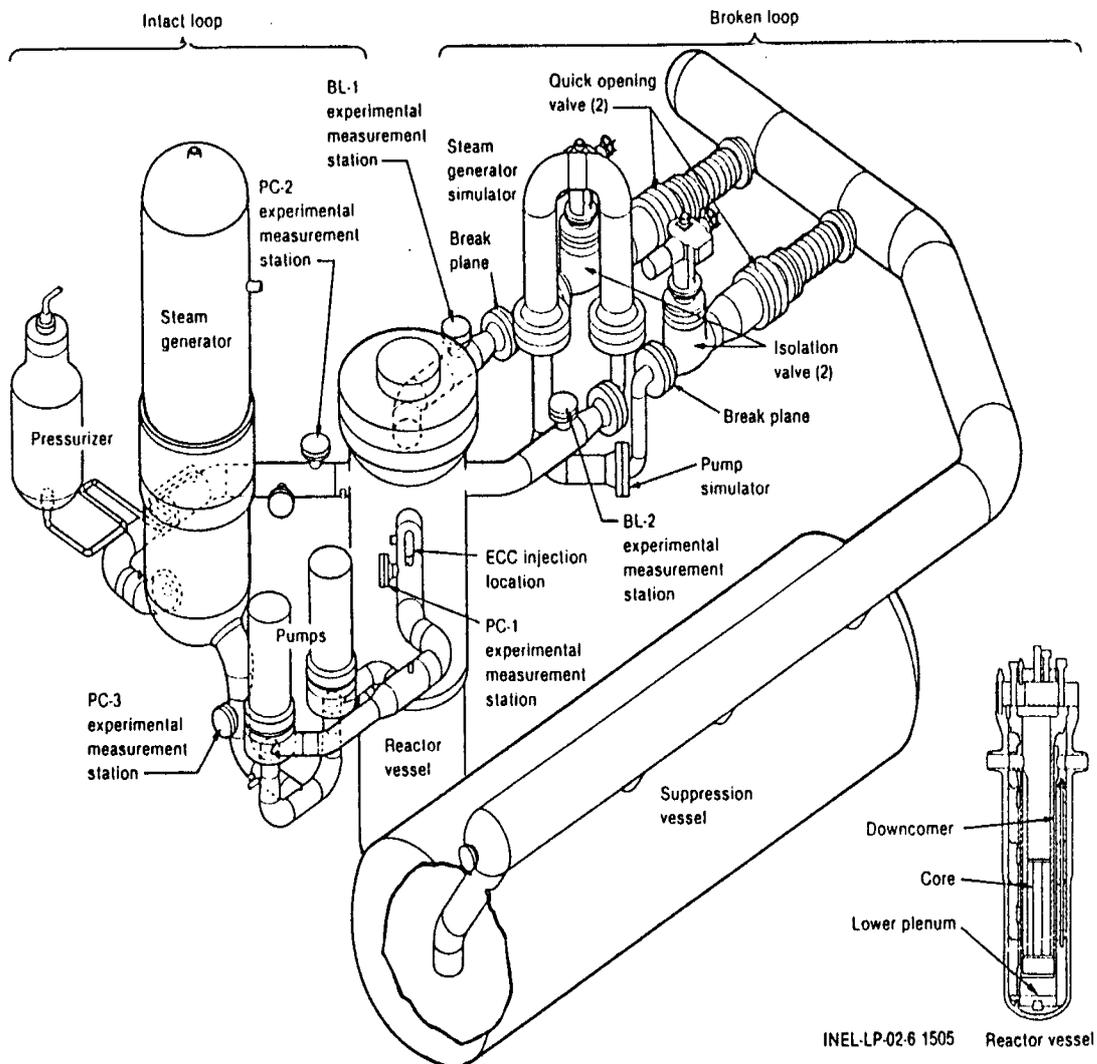
Figure 2-1 The LOFT test facility with major components
