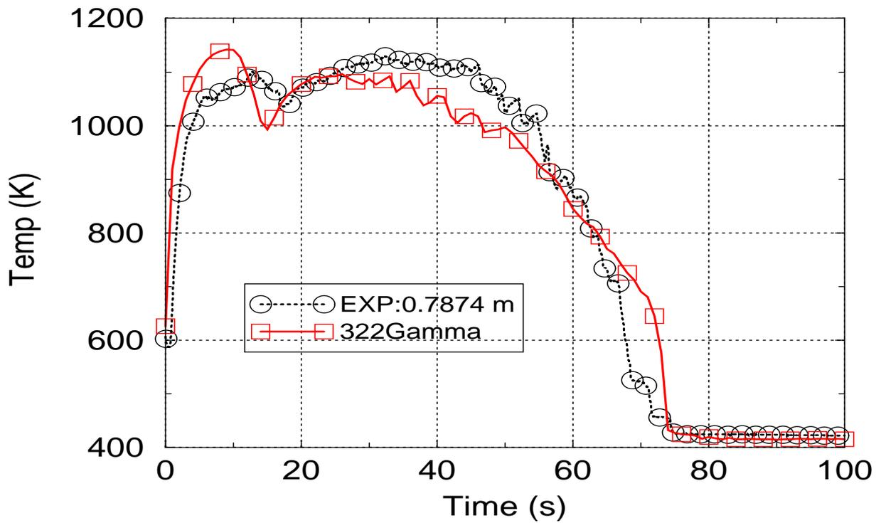
Figure 4-13 Predicted and measured cladding temperature at 0.68 and 0.78 m (hot channel)
