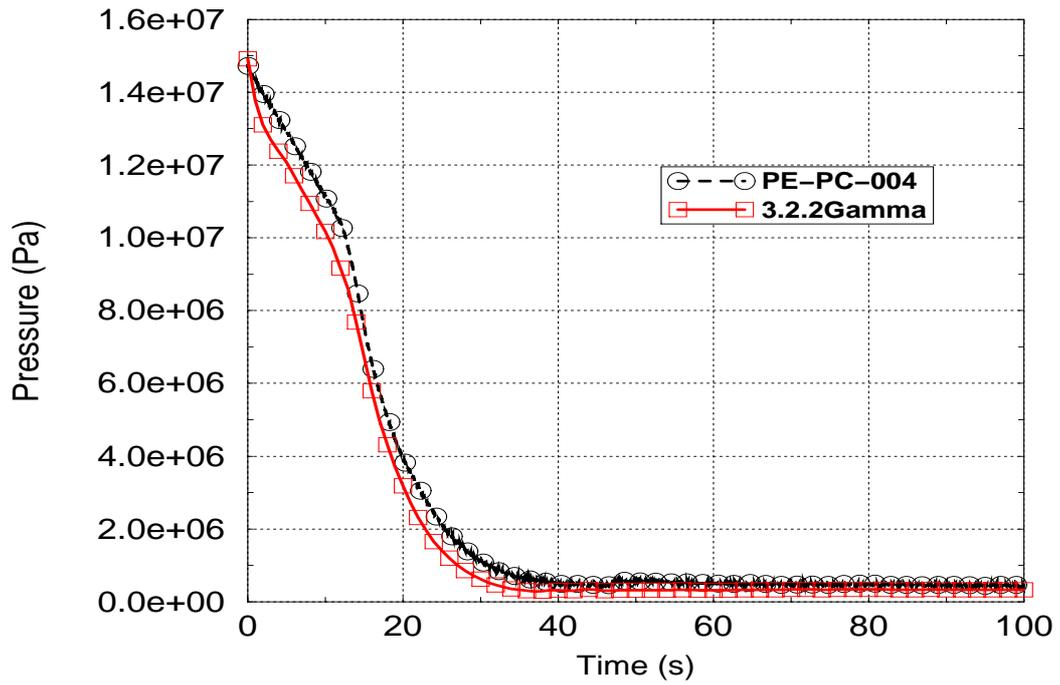
Figure 4-1 Calculated and measured pressurizer pressure
