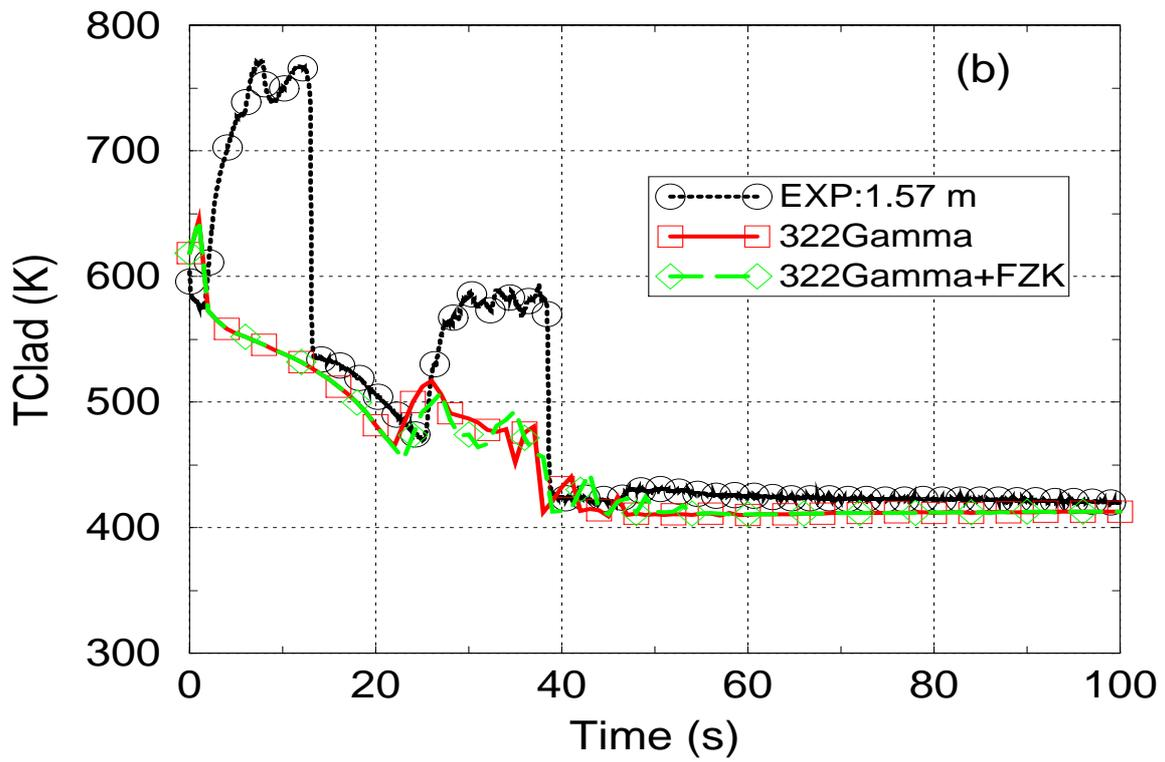
Figure 4-23 Comparison of data with predictions of cladding temperature
