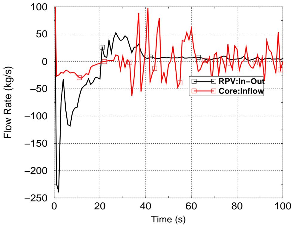
Figure 4-6 Calculated net mass flow rate through the core
