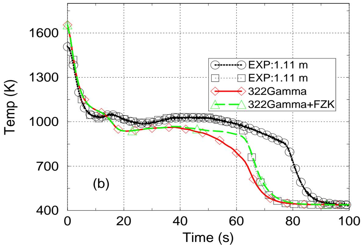
Figure 4-25 Comparison of data with predictions of fuel centre line temperature
