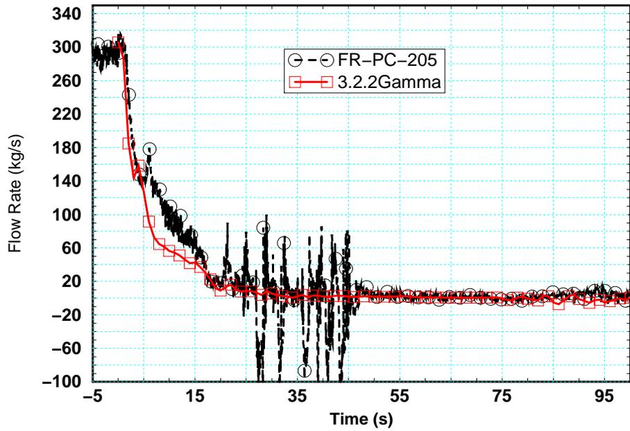
Figure 4-4 Calculated and measured mass flow rate through the intact hot/cold legs
