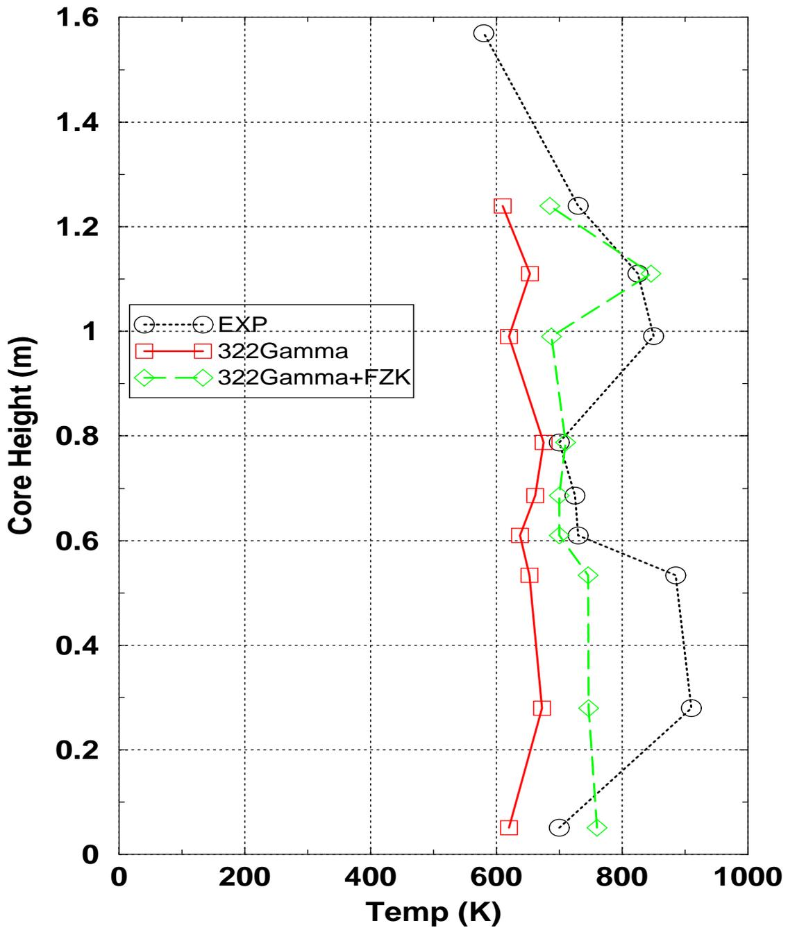
Figure 4-24 Comparison of predicted quench temperature versus data
