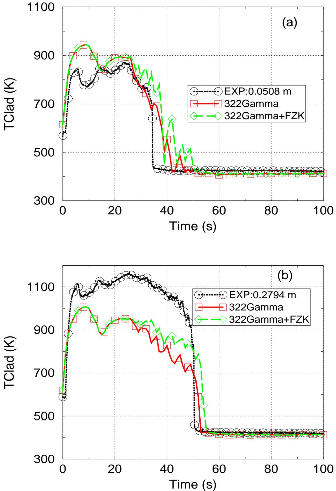
Figure 4-19 Comparison of data with predictions of cladding temperature
