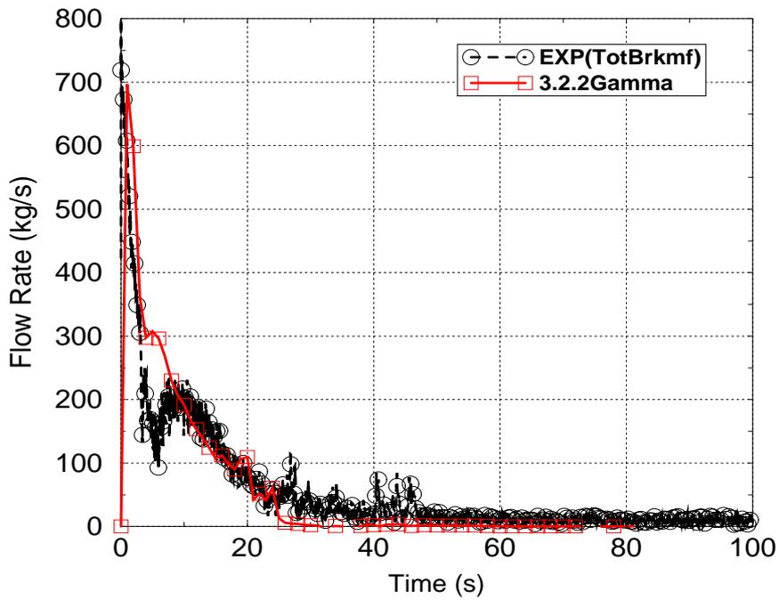
Figure 4-5 Calculated and measured total outflow through both breaks
