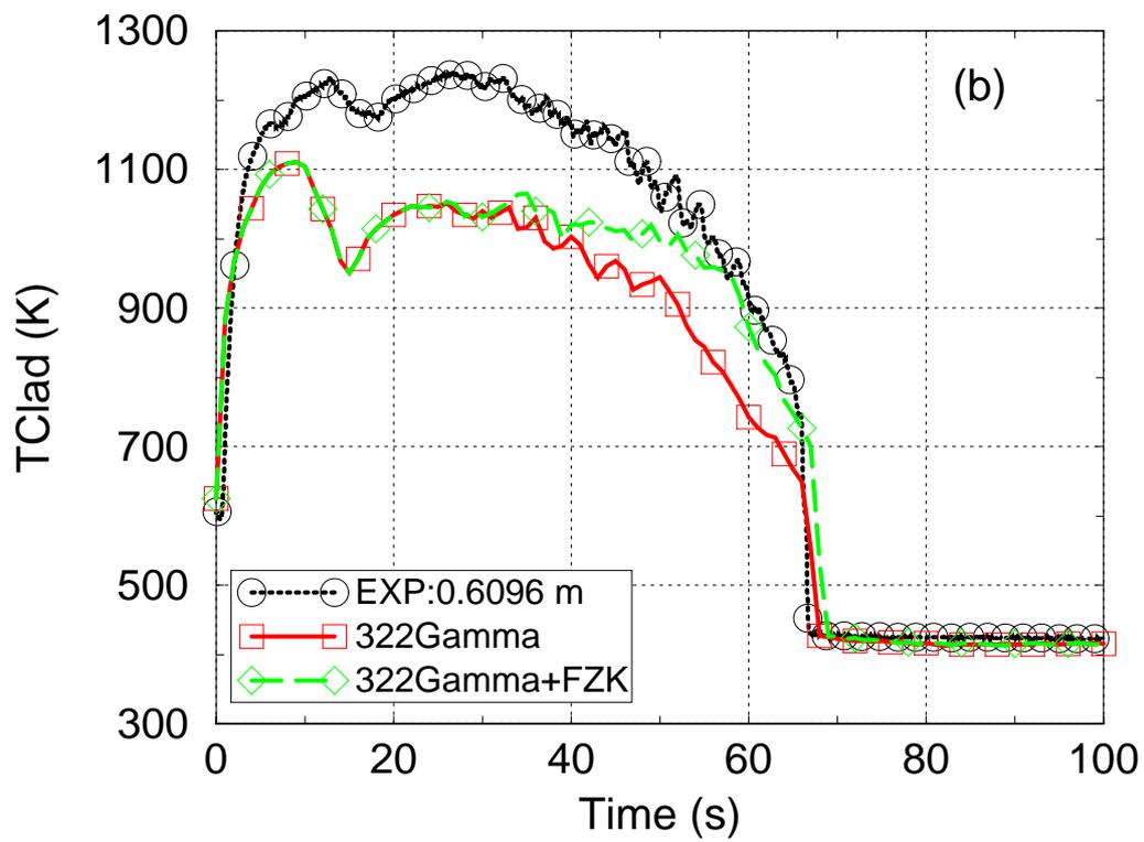
Figure 4-20 Comparison of data with predictions of cladding temperature
