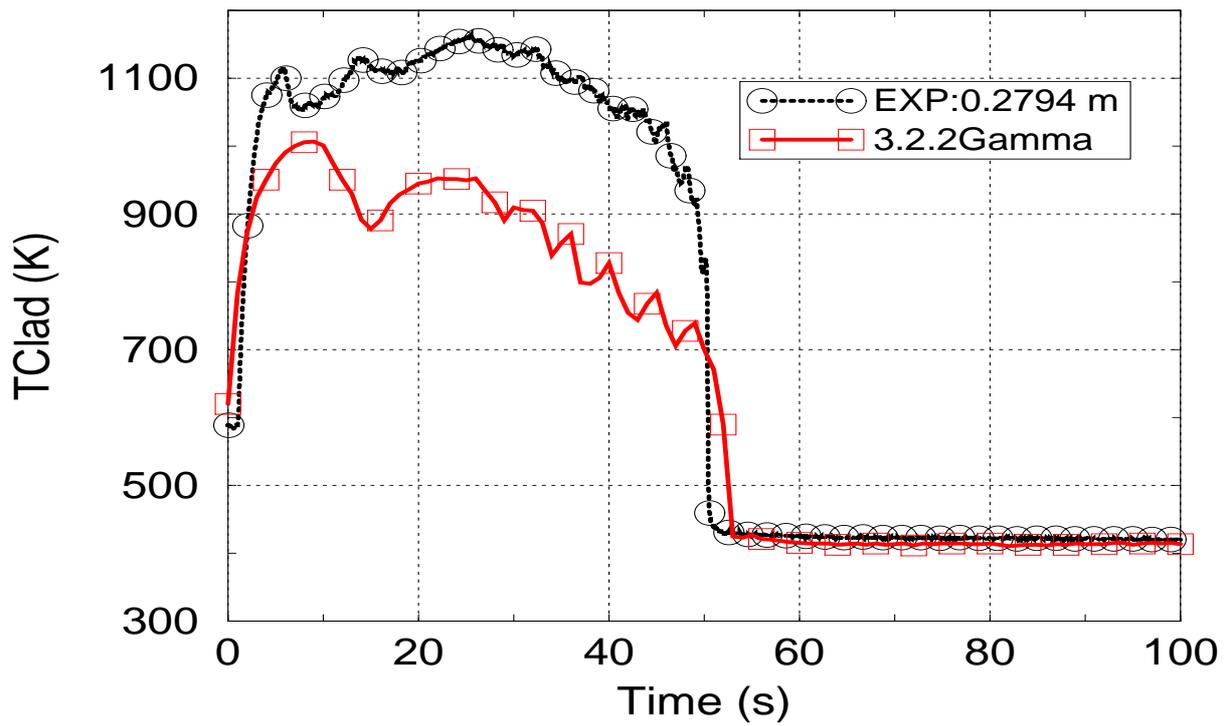
Figure 4-11 Predicted and measured cladding temperature at 0.05 and 0.27 m (hot channel)
