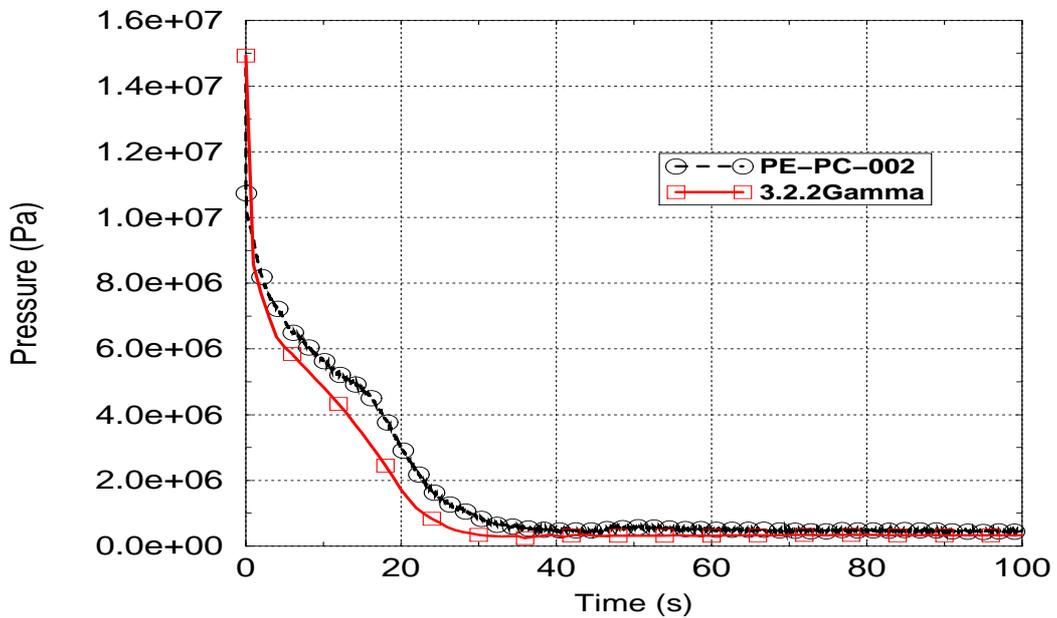
Figure 4-2 Predicted and measured hot leg pressure
