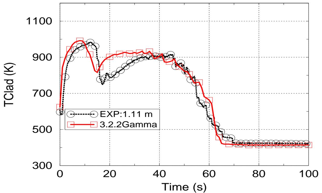
Figure 4-14 Predicted and measured cladding temperature at 0.99 and 1.11 m (hot channel)
