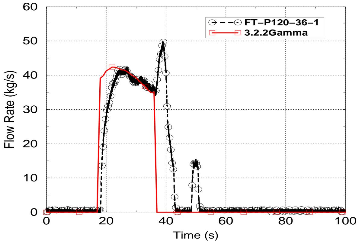
Figure 4-8 Calculated and measured accumulator mass flow rate
