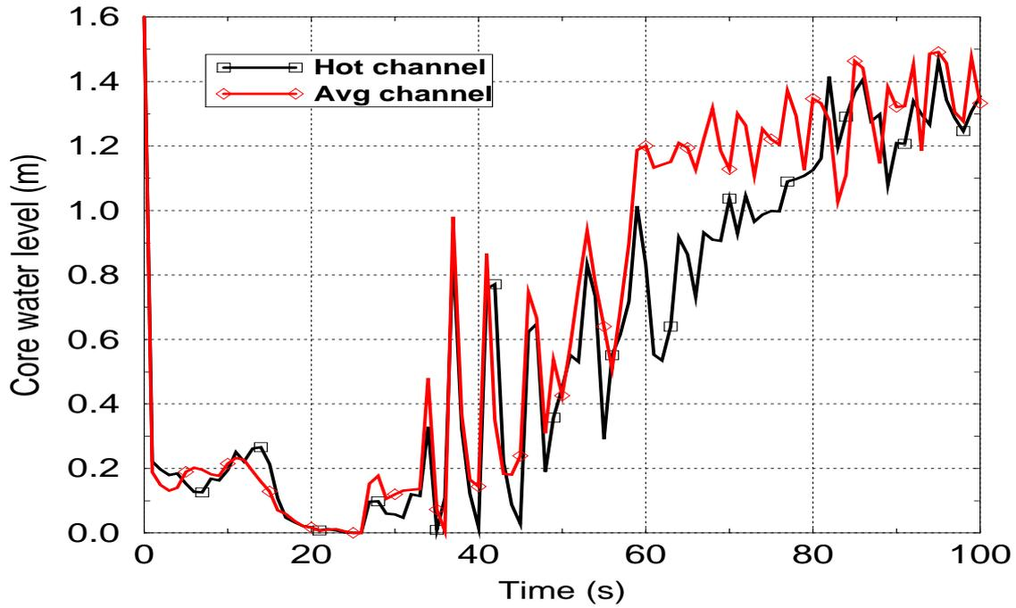
Figure 4-7 Calculated water level in hot and average core channel
