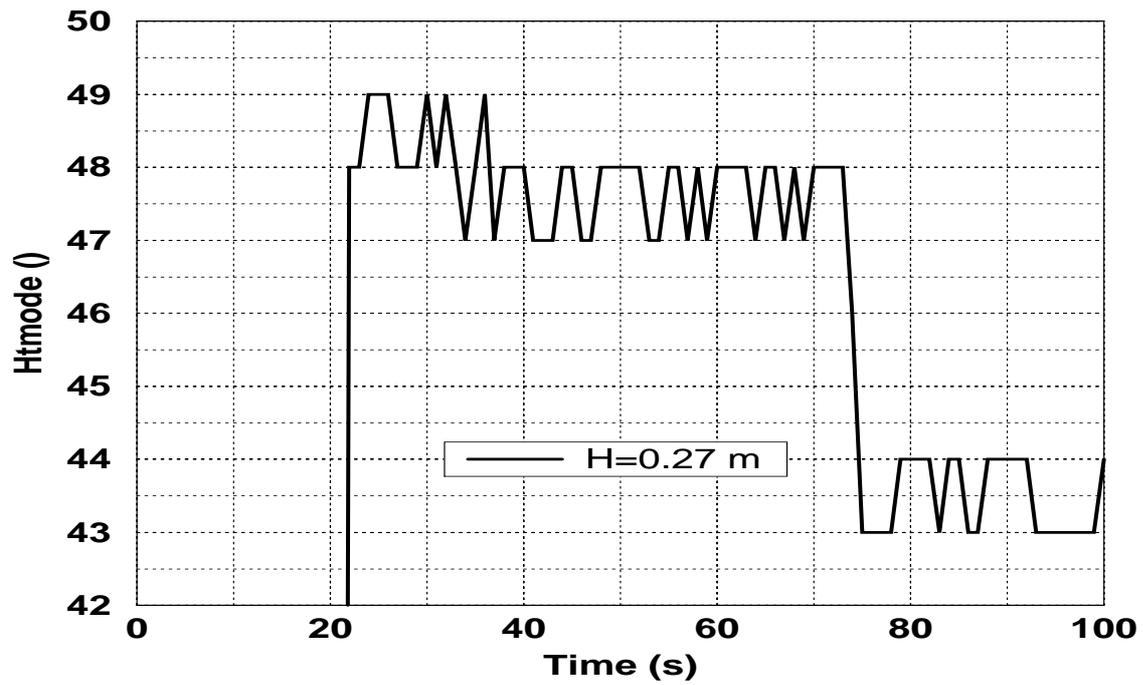
Figure 4-16 Predicted heat transfer modes at 0.27 m elevation
