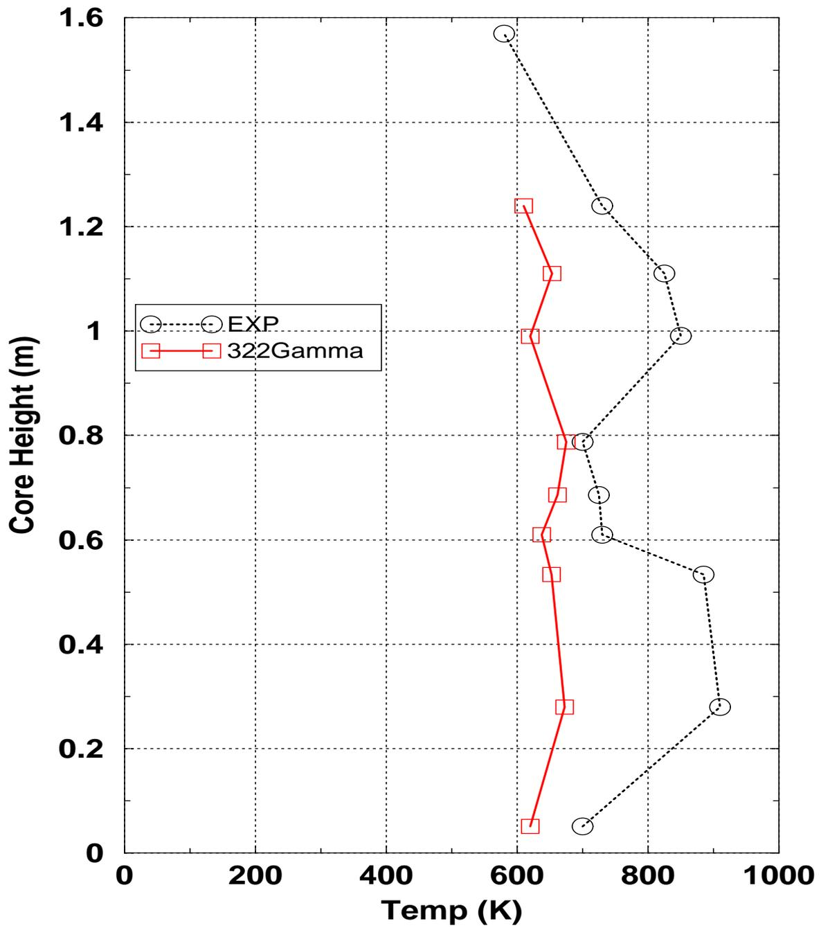
Figure 4-18 Predicted and measured quench temperature along the core height
