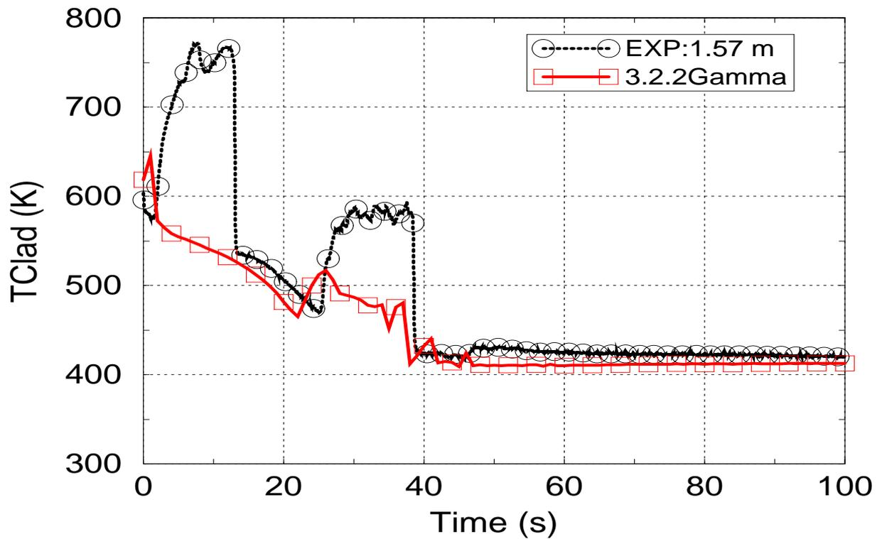
Figure 4-15 Predicted and measured cladding temperature at 1.24 and 1.57 m (hot channel)
