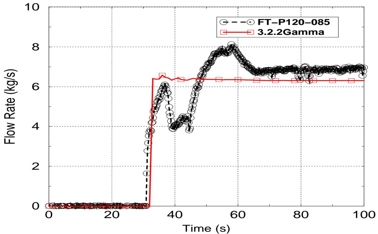
Figure 4-9 Calculated and measured LPIS-mass flow rate
