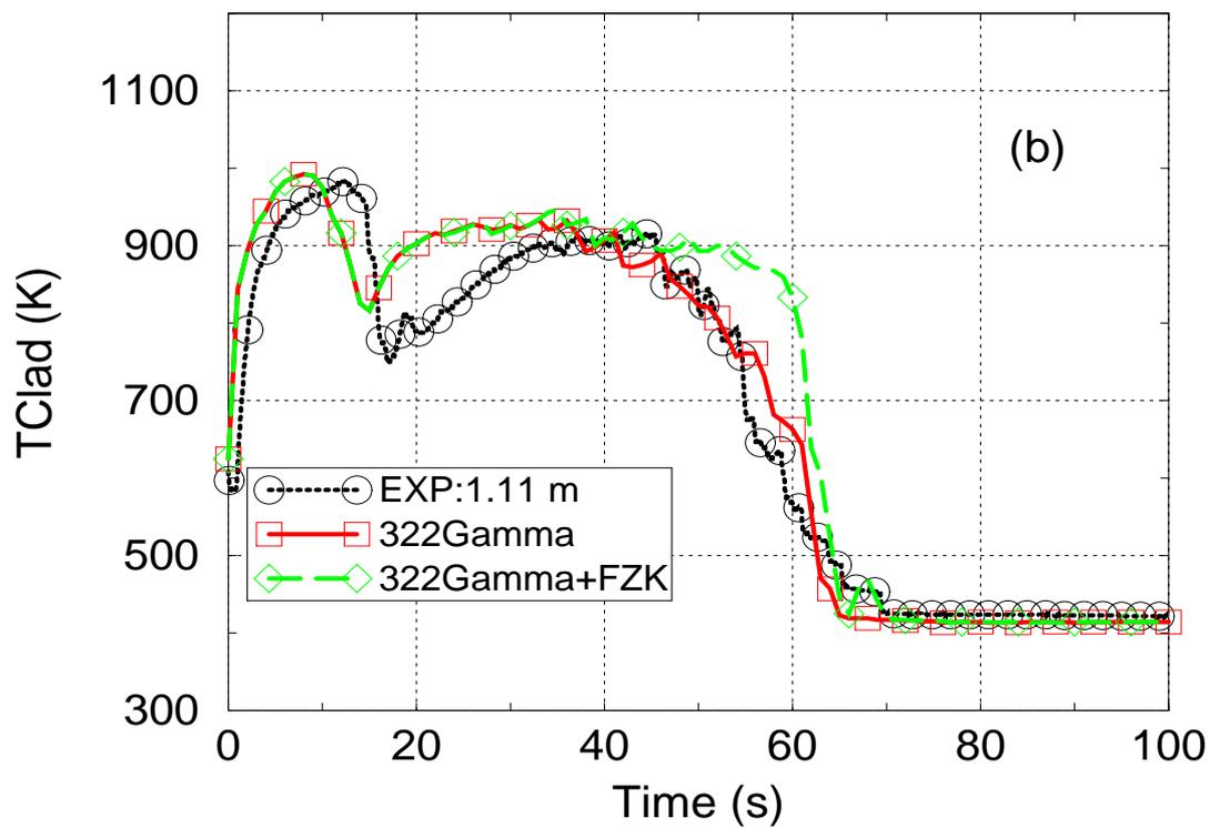
Figure 4-22 Comparison of data with predictions of cladding temperature
