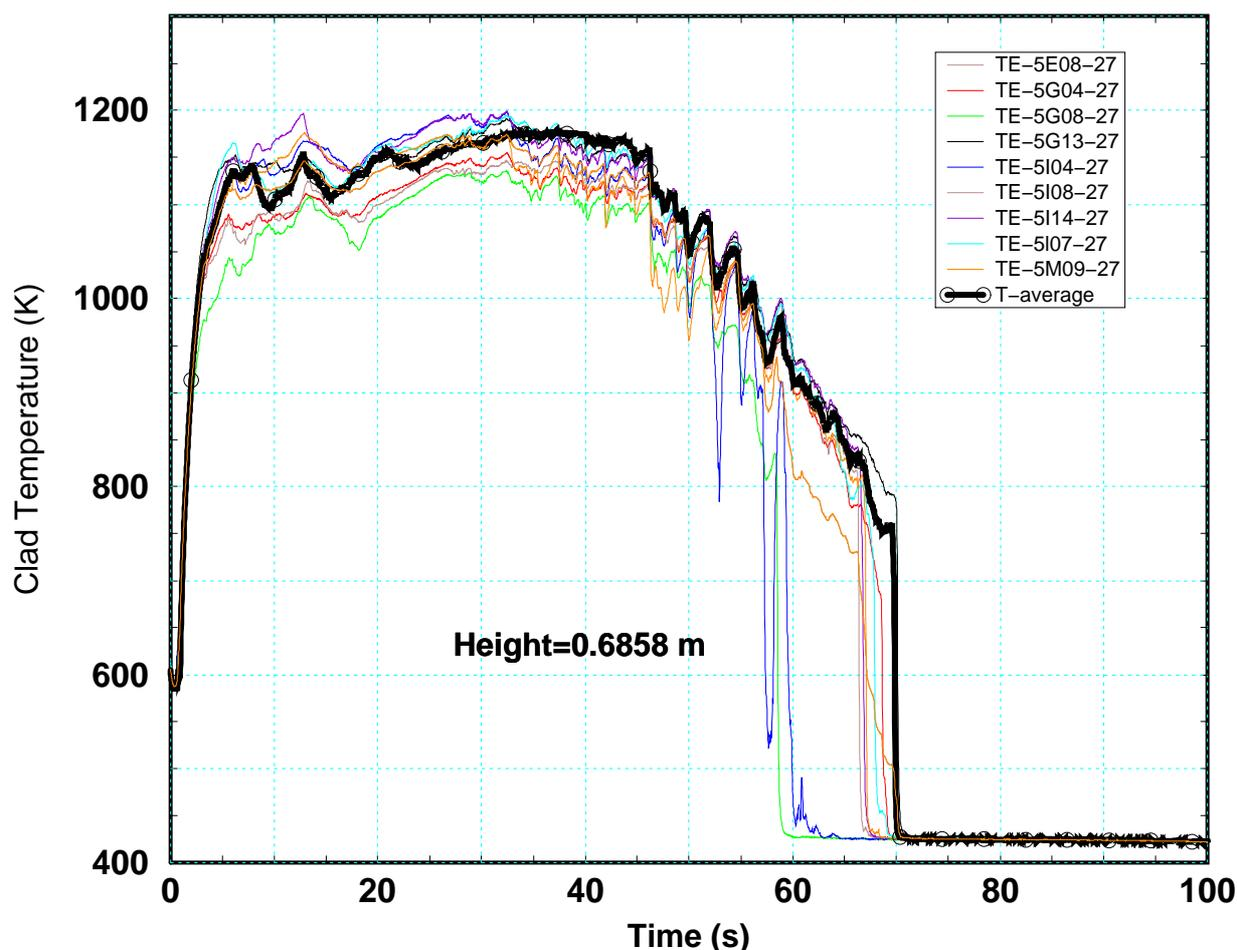
Figure 4-10 Measured cladding temperature at elevation 0.6858 m
