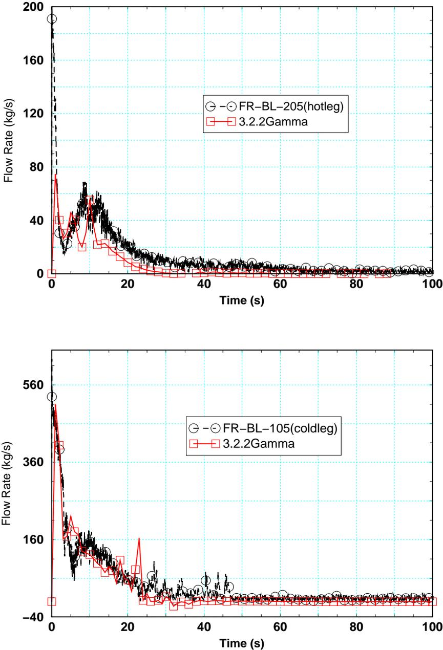
Figure 4-3 Calculated and measured mass flow rate through the broken hot/cold legs
