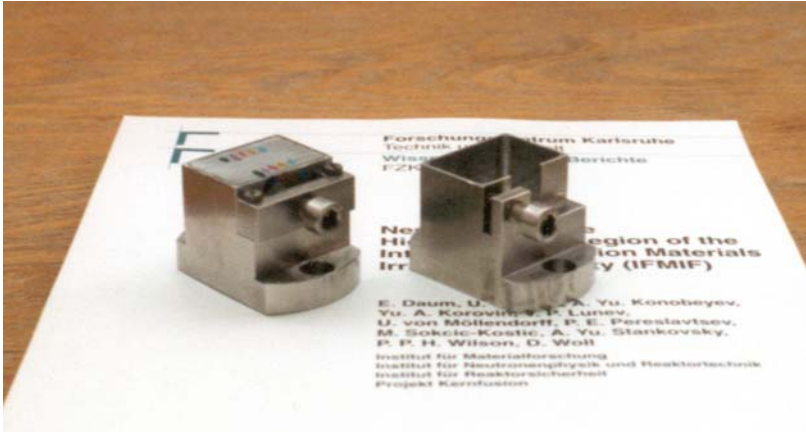
Figure 2-5 Lithium target hood A and empty target hood, seen from downstream side
