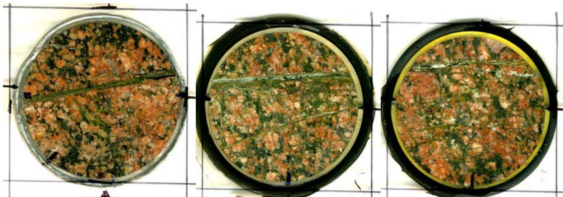
Fig. 4-2 Slice #1, #16 and slice #24 of core #2 (colored resin in the periphery)
