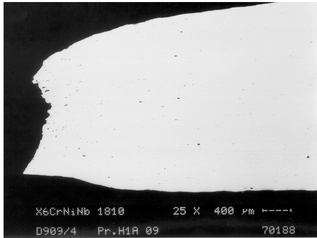
Middle length cut through the fracture (polished, 25x)
