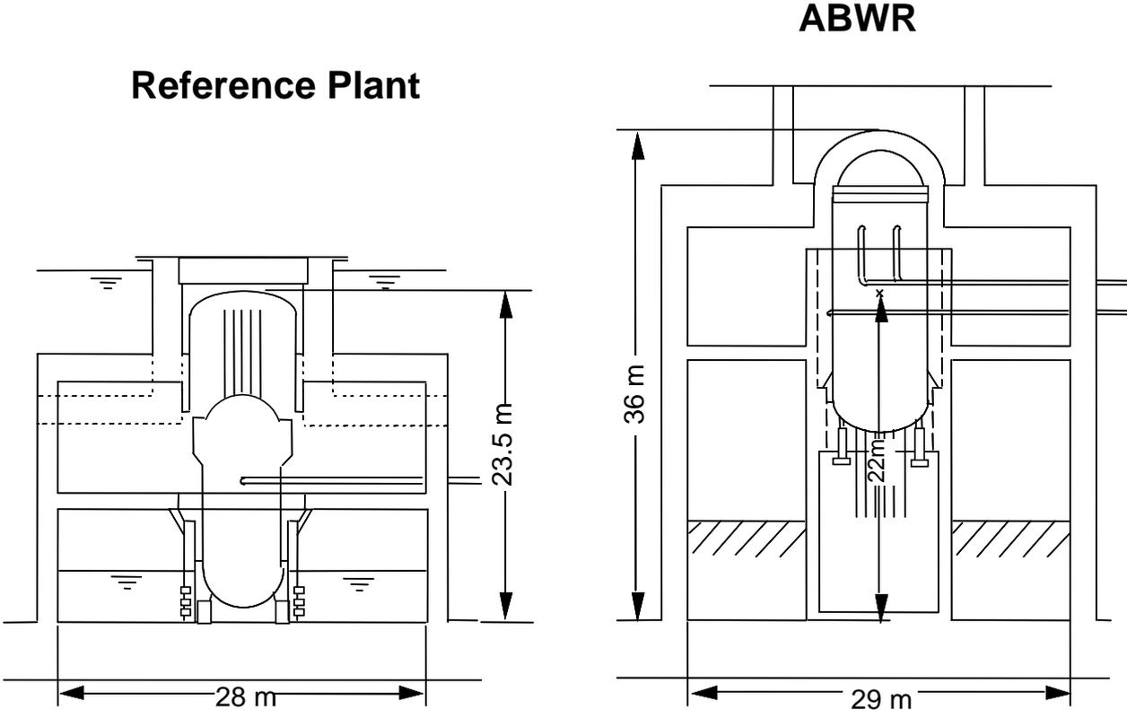
Figure 2-10 Comparison of the containment layout of the reference plant versus ABWR
