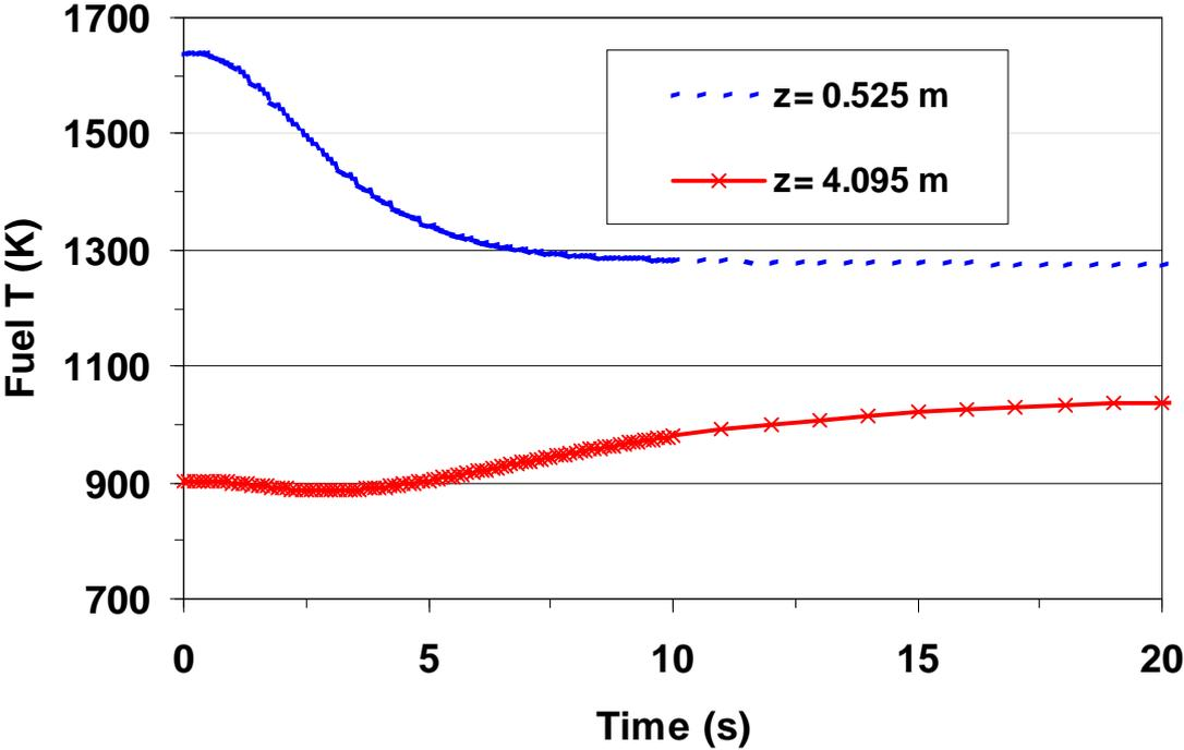
Figure 6-9 Predicted fuel center line temperature at two core elevations
