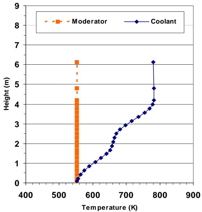
Figure 4-3 Temperature distribution along the core and hotbox
