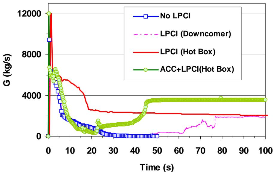
Figure 7-15 Predicted break outflow for different option of LPCI-injection
