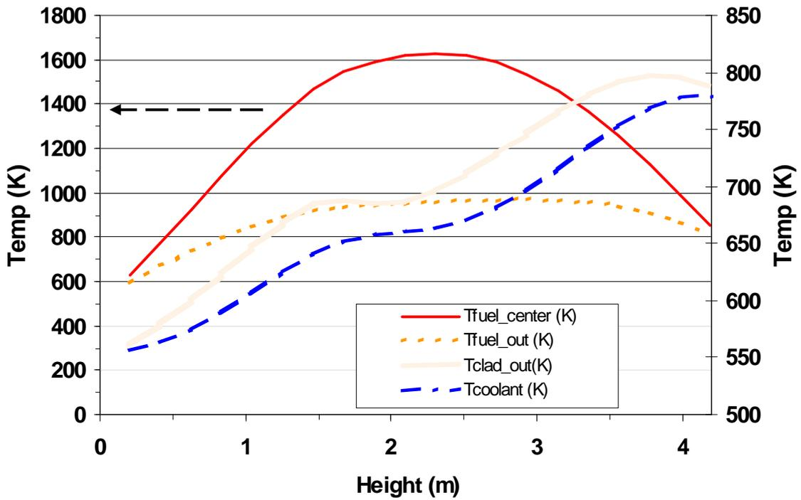
Figure 4-4 Axial distribution of the fuel, cladding and coolant temperature in the core
