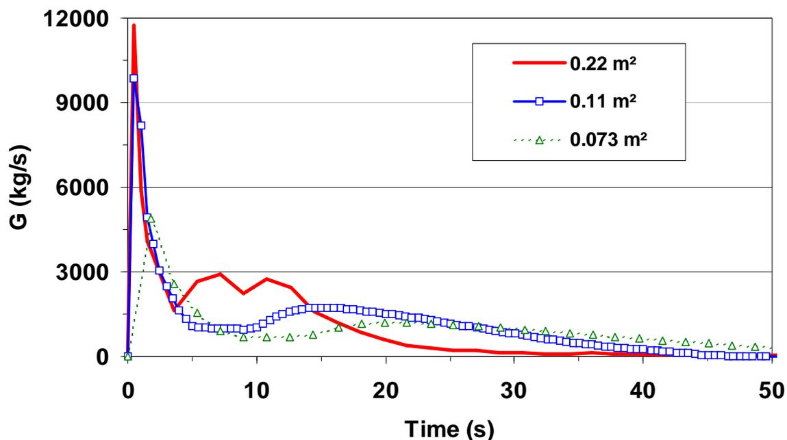
Figure 7-3 Break outflow during the blowdown phase of LB-LOCA
