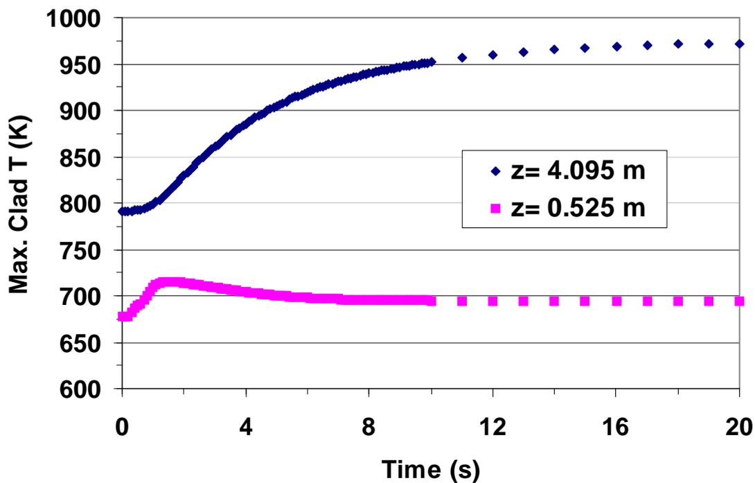
Figure 6-10 Predicted maximal cladding temperature
