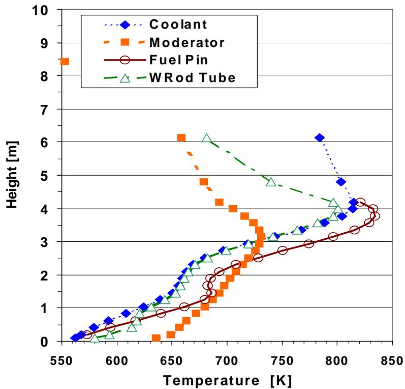
Figure 4-7 Axial temperature of coolant, moderator, fuel pin, and WR-tube (Case 1)
