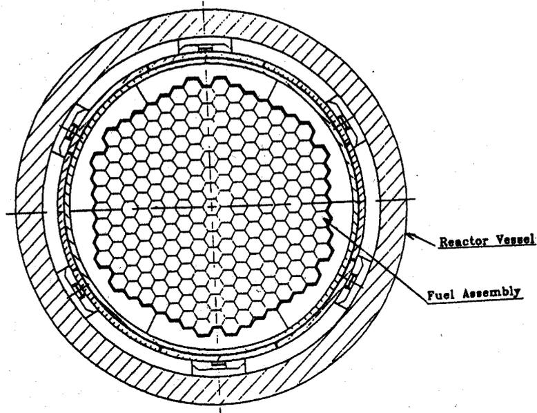
Figure 2-4 Section through the RPV of the reference plant
