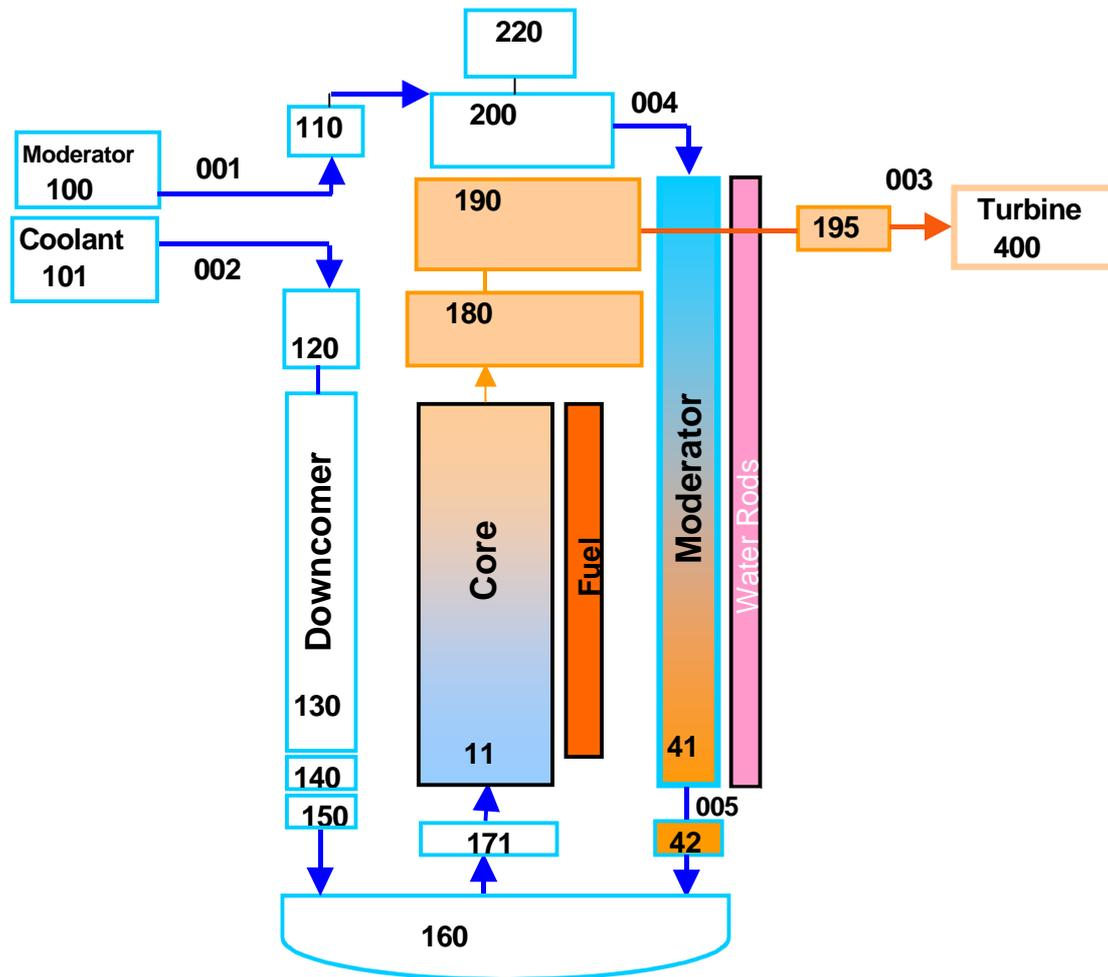
Figure 4-1 Simplified model of the reference plant for the RELAP5-simulation
