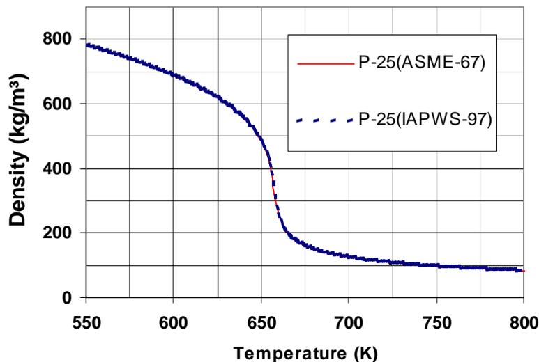
Figure 3-1 Comparison of the density predicted by steam tables ASME-67 and IAPWS-97
