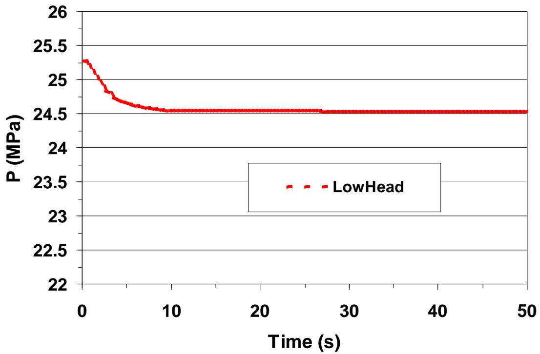
Figure 6-13 Pressure evolution of the RPV predicted by RELAP5
