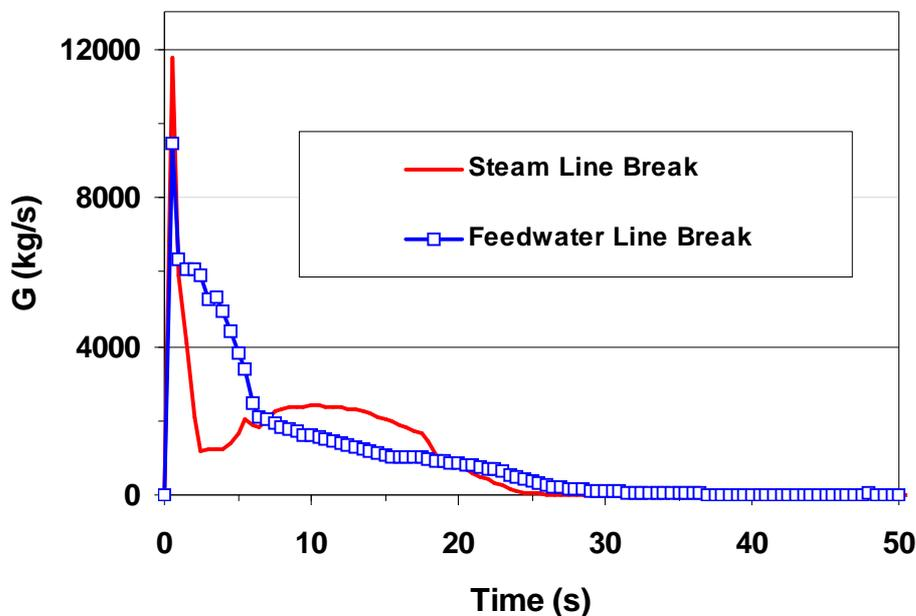
Figure 7-11 Predicted break outflow rate for steam and feedwater line break
