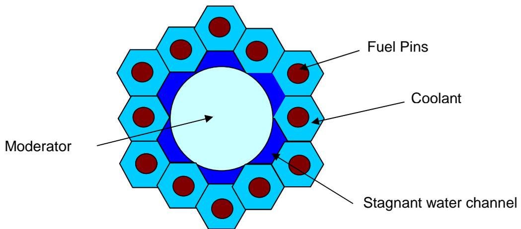
Figure 2-7 Design of a moderator rod with isolation (stagnant water) with surrounding pins.
