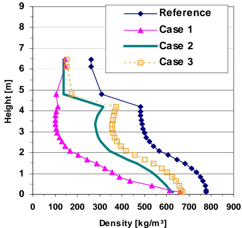
Figure 4-8 Comparison of the averaged core density for cases 1 to 3
