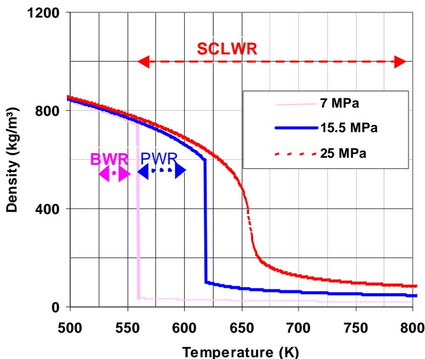
Figure 2-1 Coolant density as function of the coolant temperature
