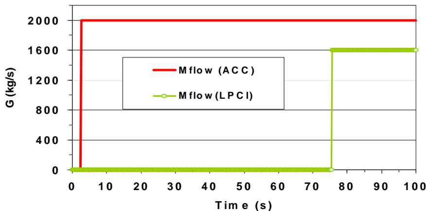
Figure 7-19 Predicted time for injection of ACC and LPCI
