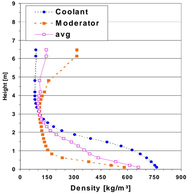
Figure 4-6 Axial distribution of the coolant and moderator density (Case 1)
