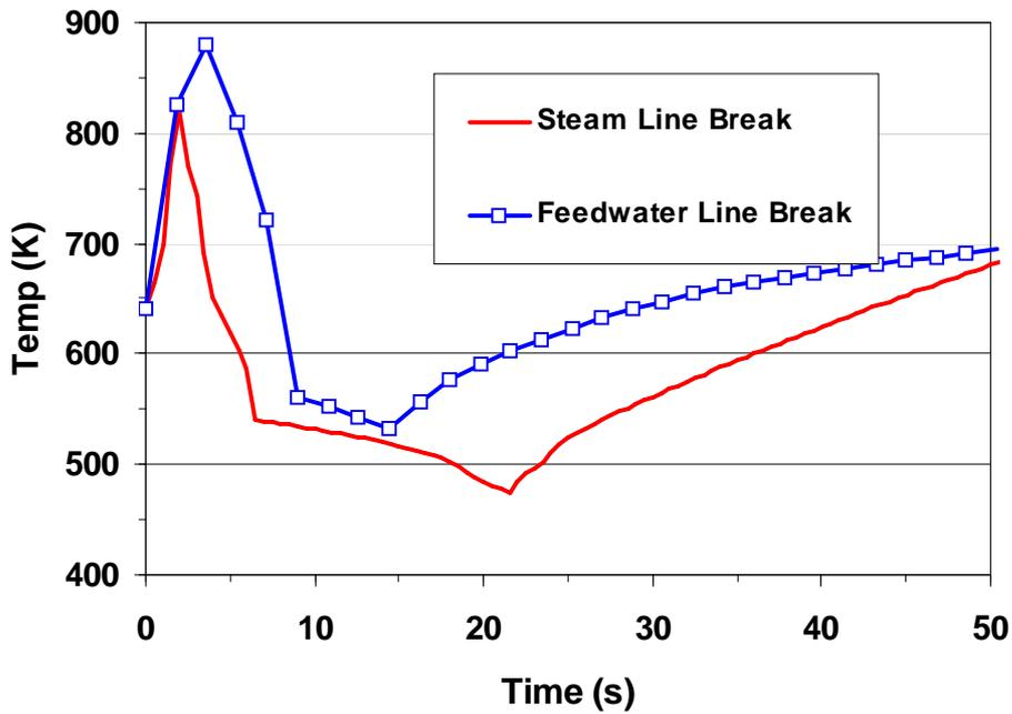
Figure 7-13 Predicted cladding temperature at 3.045 m height for the feedwater and steam line break
