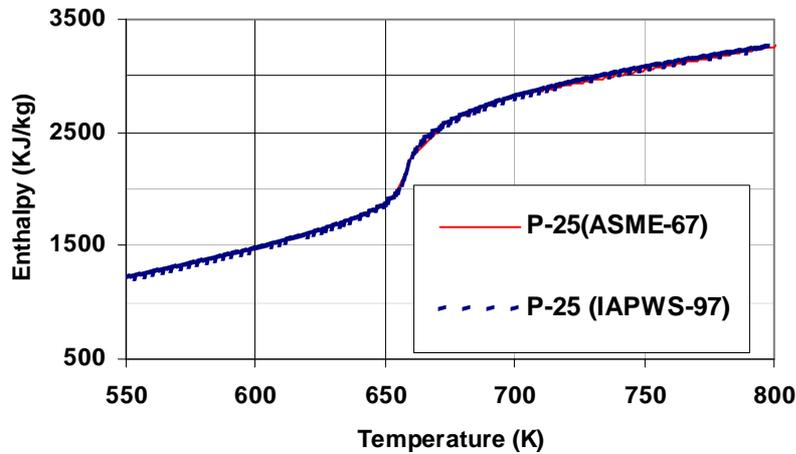
Figure 3-2 Comparison of the enthalpy predicted by steam tables ASME-67 and IAPWS-97
