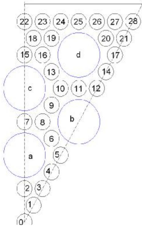
Figure 2-6 One-twelve of a fuel assembly (reference plant)
