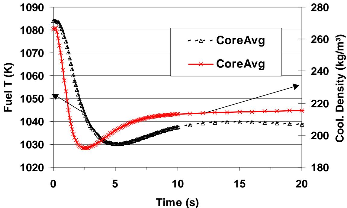
Figure 6-5 Evolution of the core averaged coolant density and fuel rod temperature
