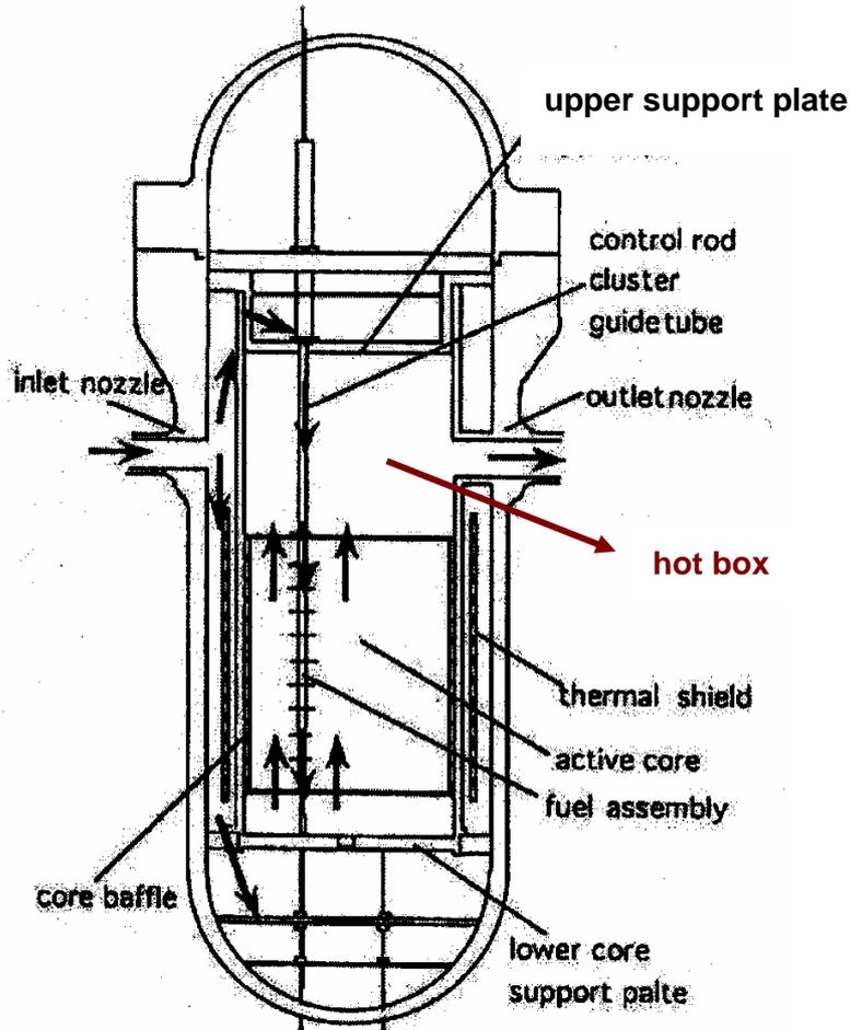
Figure 2-8 Schematic representation of the coolant and moderator flow through the core of the reference plant
