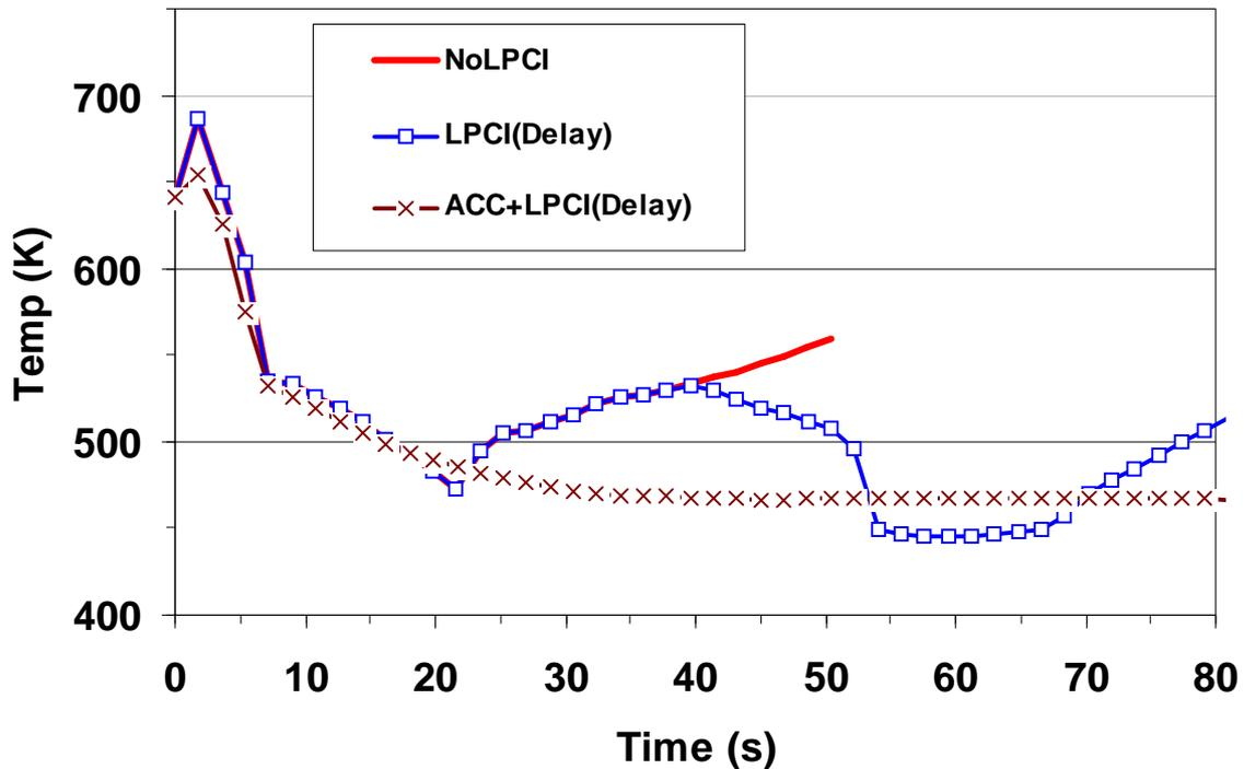
Figure 7-10 Comparison of the predicted maximal cladding temperature at 3.045 m
