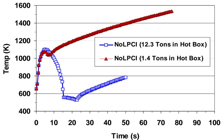
Figure 7-20 Predicted maximal cladding temperature for different fluid inventory in the hot box
