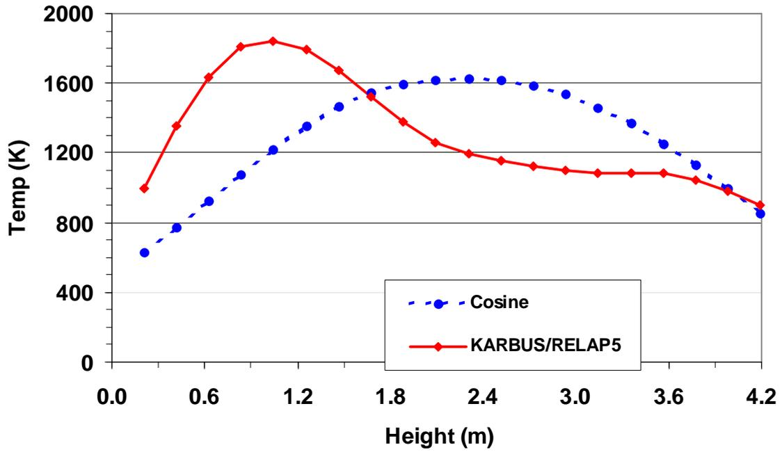
Figure 5-4 Fuel center line temperature distribution along the active core
