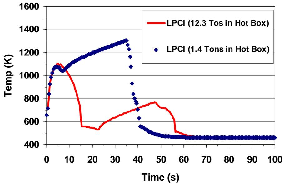
Figure 7-21 Predicted maximal cladding temperature for different fluid inventory in the hot box
