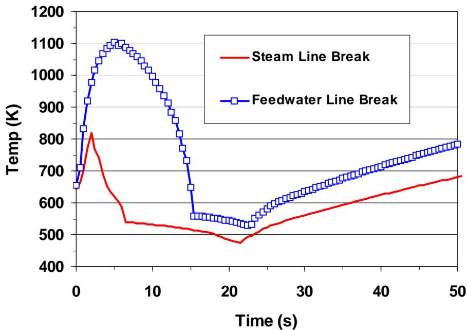
Figure 7-14 Predicted maximal cladding temperature for steam line (3.045 m) and feedwater line (1.995 m)
