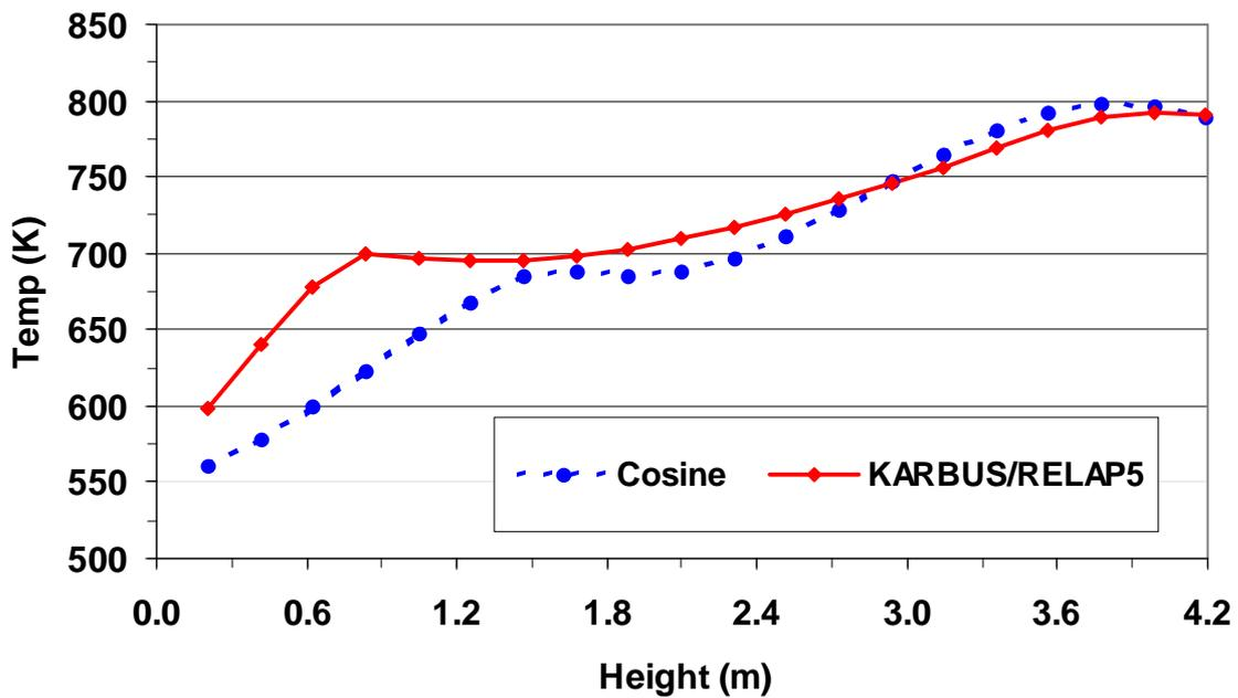
Figure 5-5 Cladding temperature distribution along active core
