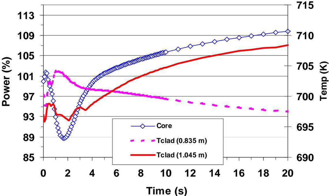
Figure 6-3 Relative thermal power and maximal cladding temperature at 0.835 m height
