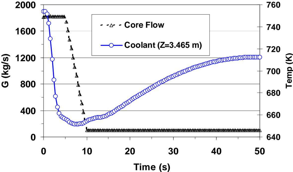
Figure 6-11 Coolant mass flow rate and predicted coolant temperature at height 3.465 m
