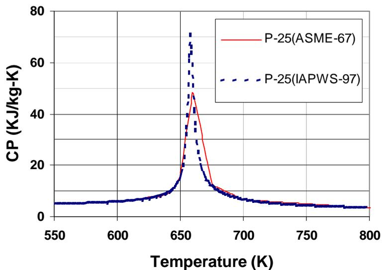
Figure 3-3 Comparison of the heat capacity as predicted by two different steam tables
