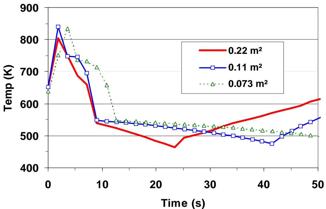
Figure 7-5 Cladding temperature evolution during the blowdown phase of LB-LOCA
