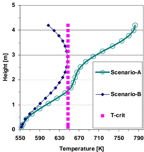
Figure 7-1 Axial coolant temperature distribution at steady state for scenario A and B
