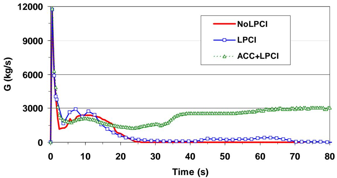
Figure 7-8 Predicted break outflow for three different scenarios
