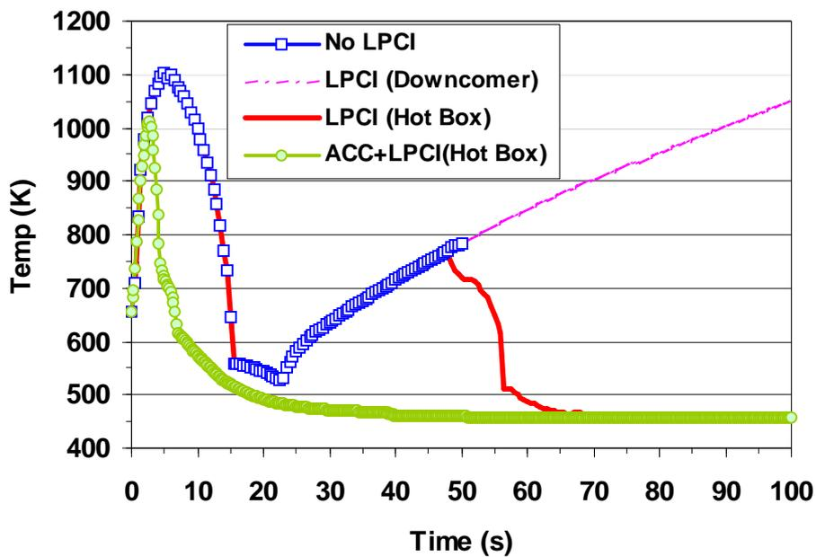
Figure 7-17 Predicted maximal cladding temperature for the studied cases
