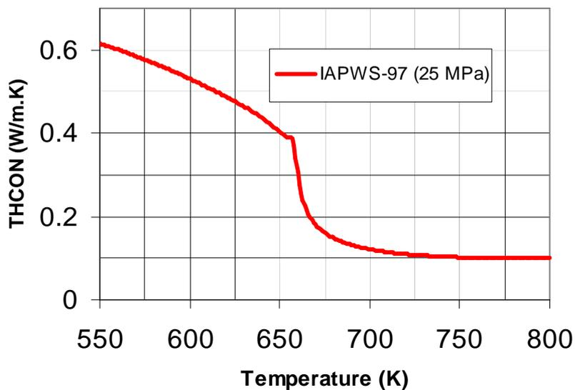
Figure 2-3 Thermal conductivity as function of the coolant temperature for 25 MPa [Wagn97]
