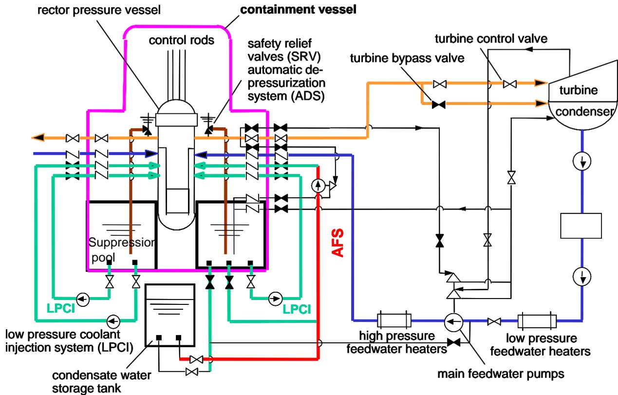
Figure 2-9 Schematic representation of the safety features of the reference plant
