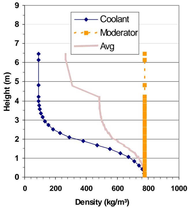
Figure 4-2 Density distribution along the core and hot box
