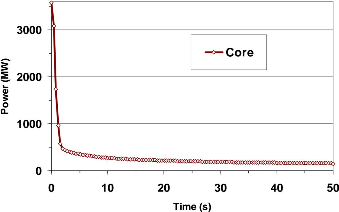
Figure 6-12 Thermal power reduction after scram
