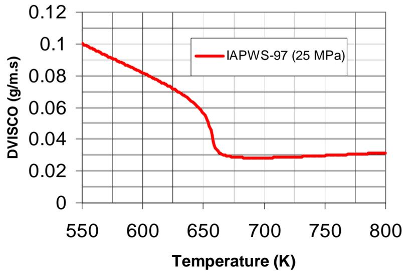
Figure 2-2 Dynamic viscosity as function of the coolant temperature for 25 MPa [Wagn97]
