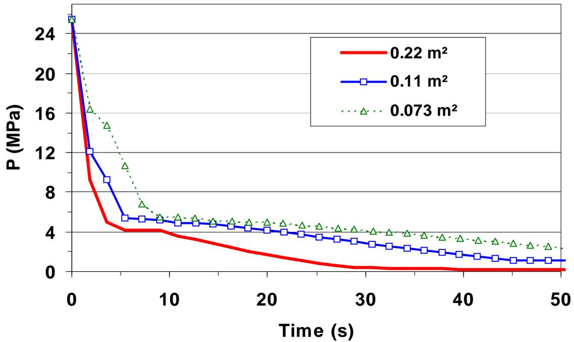
Figure 7-4 RCS-Pressure evolution during the Blowdown phase of LB-LOCA
