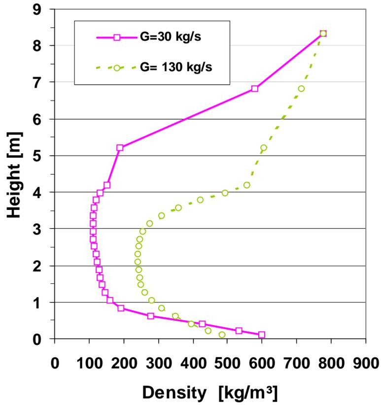
Figure 4-9 Comparison of the moderator density in water rod for different flow rates
