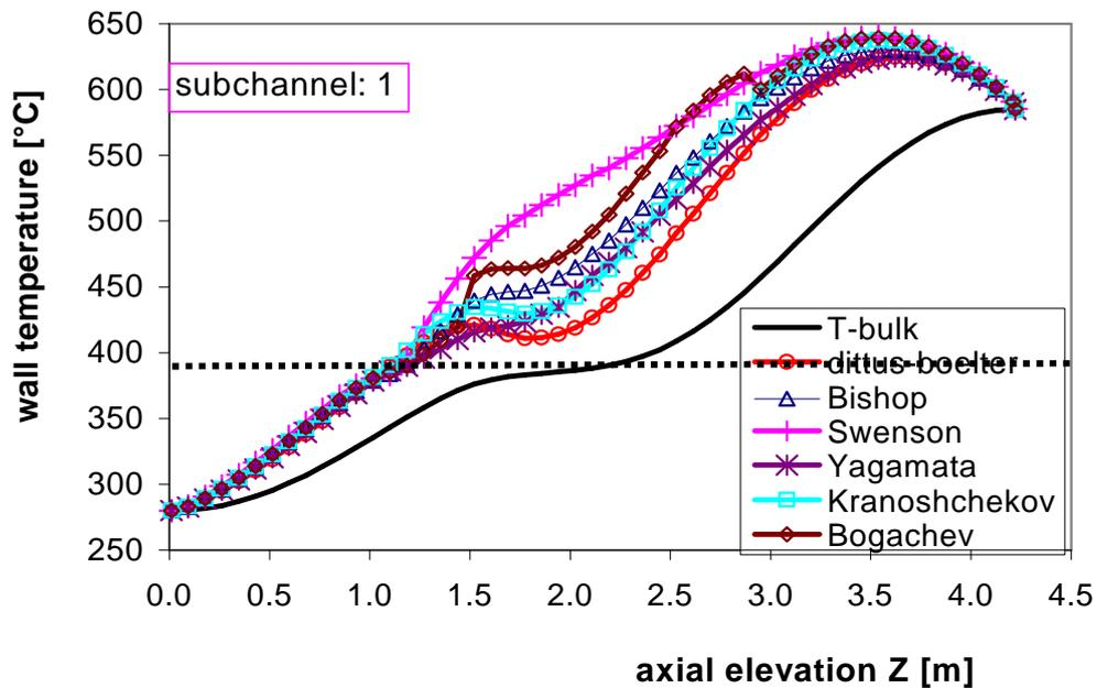
Figure 3-4 Comparison of the wall temperature versus the core height predicted by different correlations
