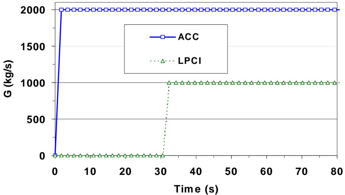
Figure 7-9 Injection rate of the accumulators and of the LPCI
