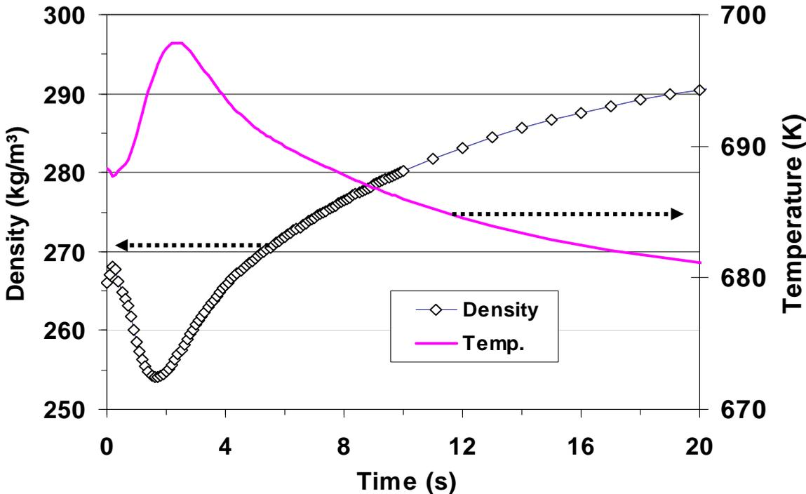
Figure 6-2 Core average coolant density and coolant temperature evolution
