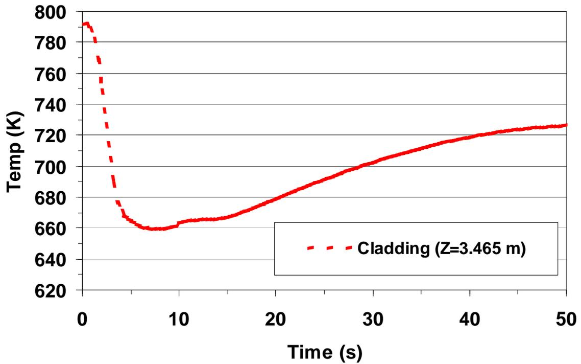
Figure 6-14 Maximal cladding temperature during the transient
