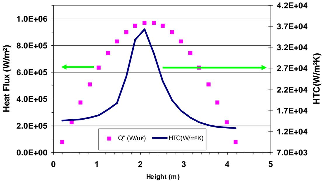
Figure 4-5 Axial heat flux and heat transfer coefficient distribution in the core
