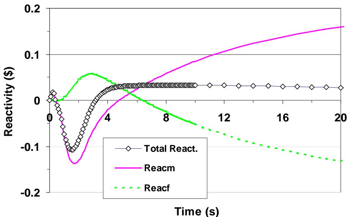
Figure 6-4 Evolution of the total reactivity compared to the contributions due to moderator (reacm) and fuel temperature (reactf)
