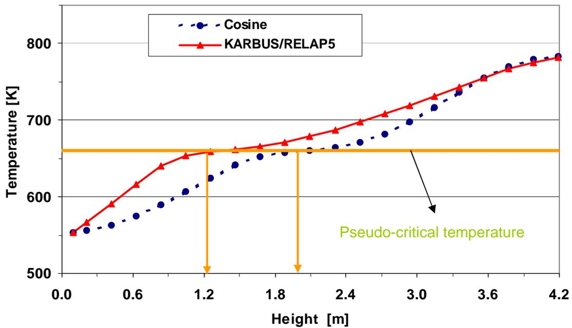
Figure 5-3 Predicted coolant temperature distribution for the reference case
