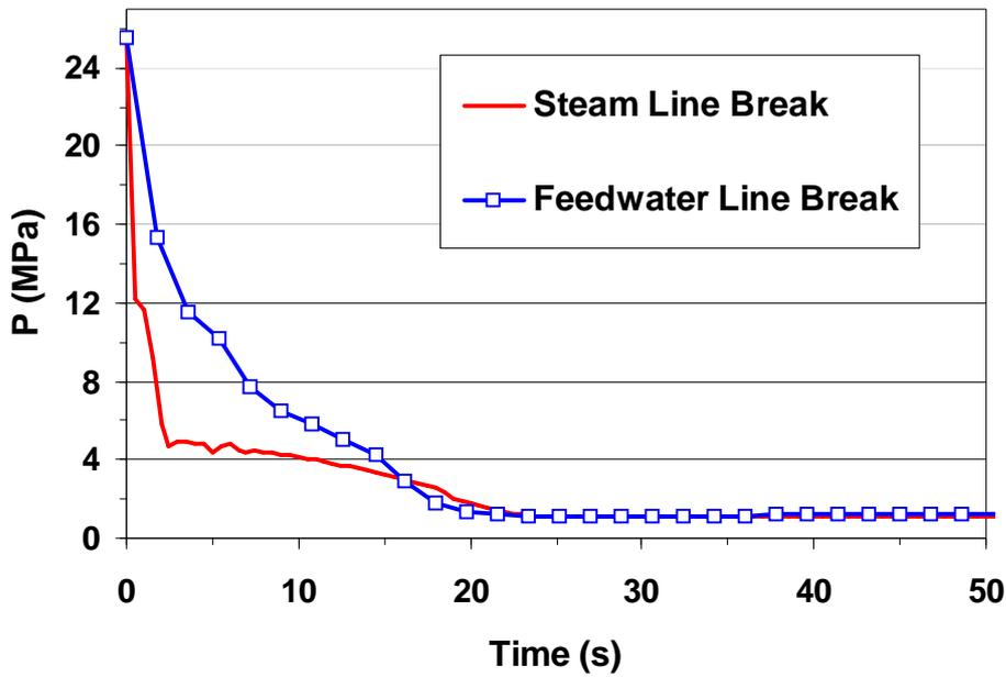
Figure 7-12 Predicted system pressure for steam line and feedwater line break
