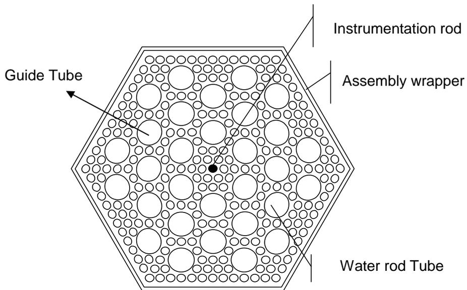
Figure 2-5 Section through the fuel assembly of the reference plant
