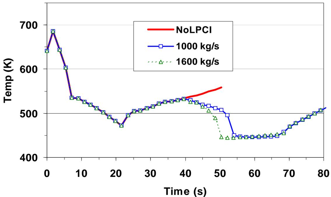
Figure 7-7 Comparison of predicted cladding temperature for the LB-LOCA
