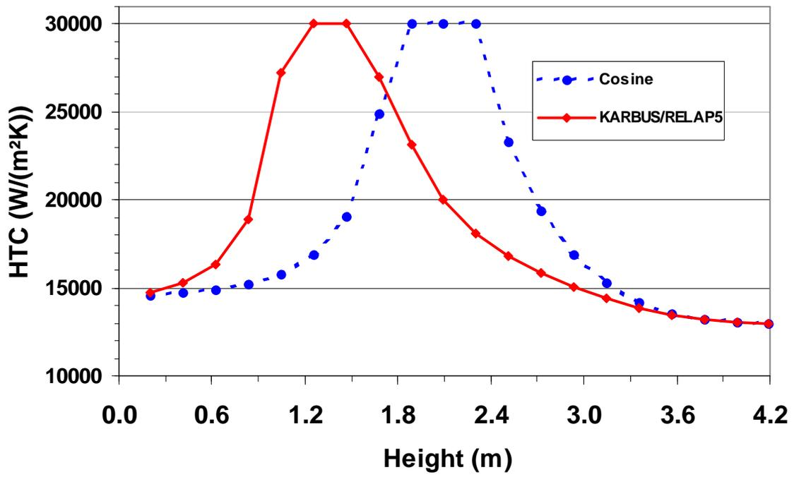
Figure 5-6 Comparison of the heat transfer coefficient for two axial power profiles
