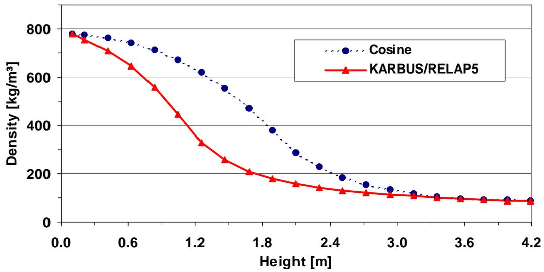
Figure 5-2 Predicted coolant density distribution for the reference case
