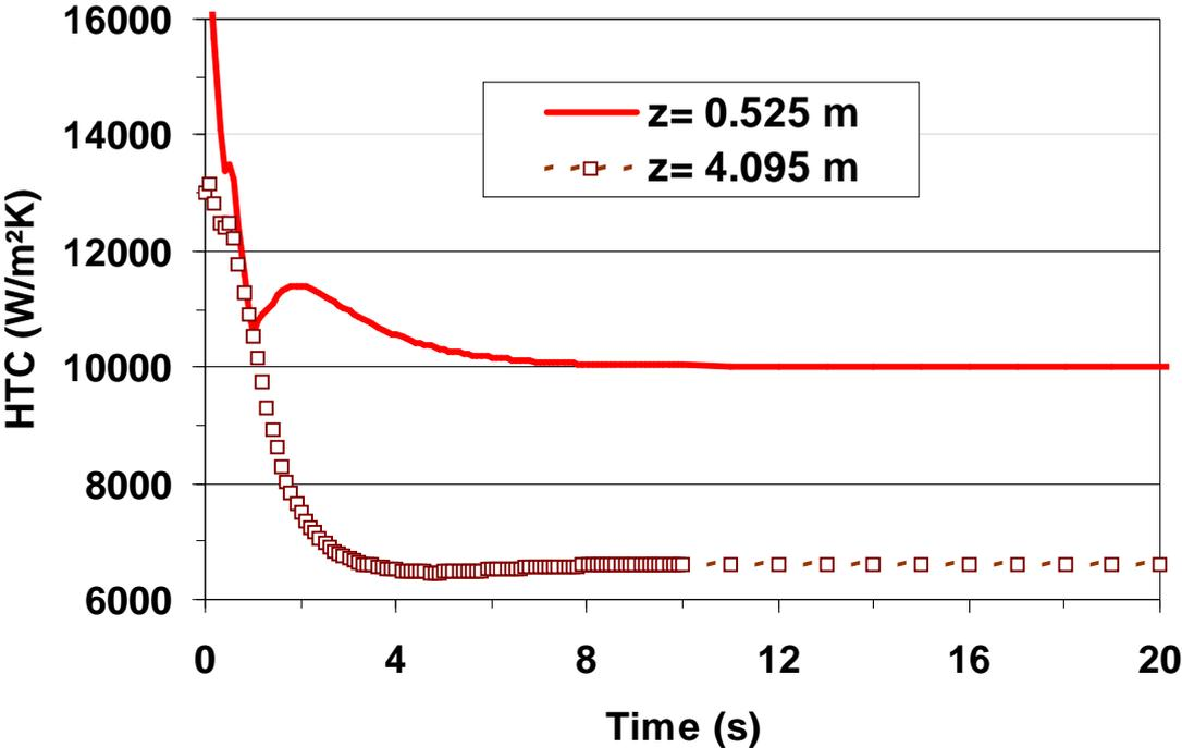
Figure 6-8 Predicted heat transfer coefficient for two core elevations
