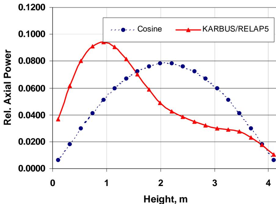
Figure 5-1 Comparison of assumed cosine-shaped and predicted power profile
