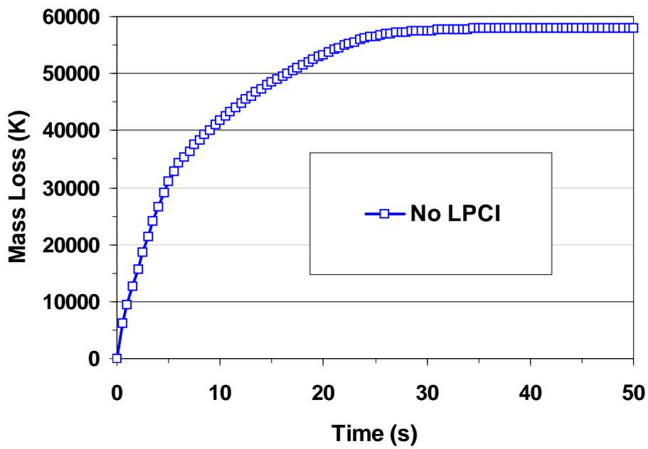
Figure 7-16 Predicted integrated fluid inventory that leaves the reactor pressure vessel
