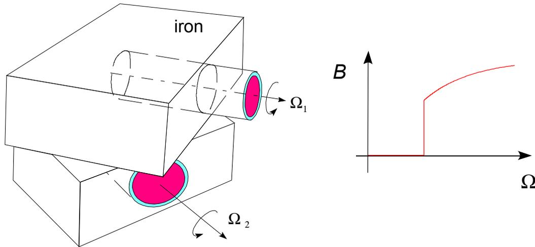
Figure 3.2. a) Principle sketch of the Lowes & Wilkinson (1968) laboratory model of the Geomagnetic Dynamo, b) saturation of magnetic induction as a function of the angular velocity  $\Omega$ .
