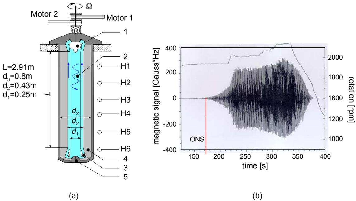
Figure 3.3. a) The Riga test section, test fluid sodium: 1 Impeller, 2 helical flow region, 3 vortex free return flow channel, 4 stagnant sodium, 5 stainless steel container,  $H_1 \rightarrow H_6$  Hall probe sensor positions. b) Measured time signal of radial component of the self-excited magnetic field; (—) recorded rotation rate of pump impeller; (.....) and (ONS) onset of self-excitation (Gailitis et al. (2001)).
