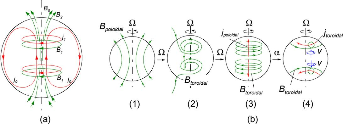
Figure 2.3. Self-excitation of seed magnetic fields by a)  $\alpha^2$ -dynamo, b)  $\alpha$ - $\Omega$ -dynamo.
