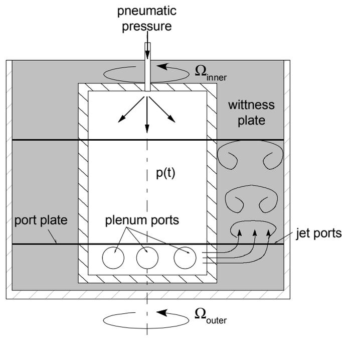
Figure 3.7. Principle sketch of the New Mexico  $\alpha$ - $\Omega$ -dynamo experiment after Colgate et al. (2001).
