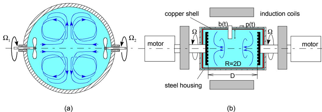
*Figure 3.6.* Principle sketch of the driving mechanism for the flow in spheres and cylinders to establish the Dudley & James (1989) flow topology. a) Forest et al. (2000) and Lathrop et al. (2000), b) Pinton et al. (2000).
