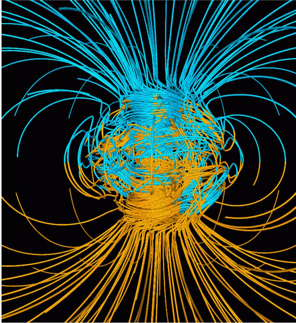
*Figure 2.6.* A three-dimensional magnetic field structure simulated by the Glatzmaier-Roberts geodynamo model. The field lines are drawn out to two Earth's radii. The magnetic field is wrapped around the "tangent cylinder" to the solid core due to the shear of the zonal fluid flow (after Glatzmaier & Roberts (1995)).
