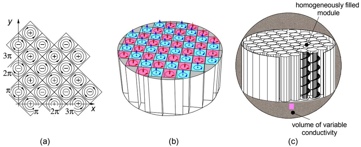
Figure 2.5. Unconfined and confined periodic vortex fields as a basis for dynamo action. a) Roberts' periodic vortex field, b) Busse's vortex arrangement in a cylindrical domain, c) Tilgner's (1997) and Rädler's (1998) spherical containment.
