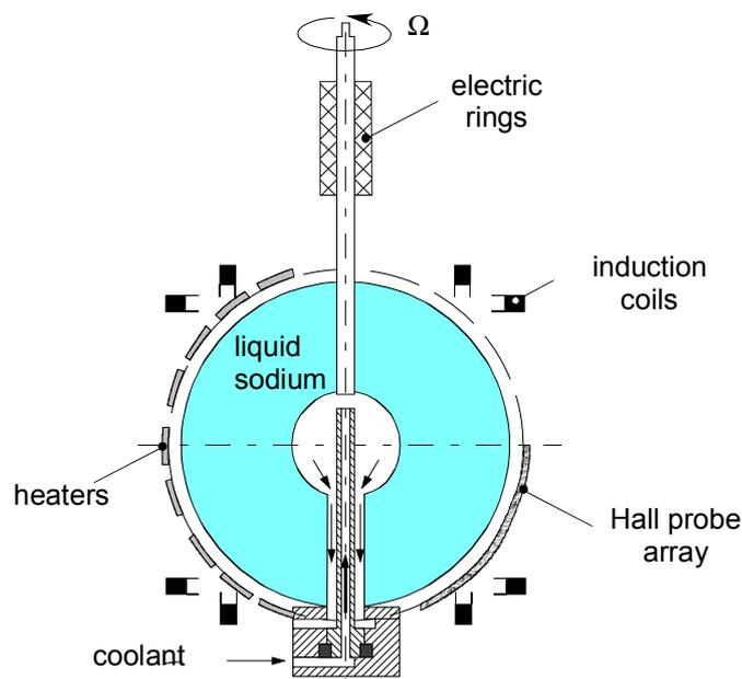
Figure 3.9. Experimental setup for a convection-driven dynamo experiment after Lathrop (2000).
