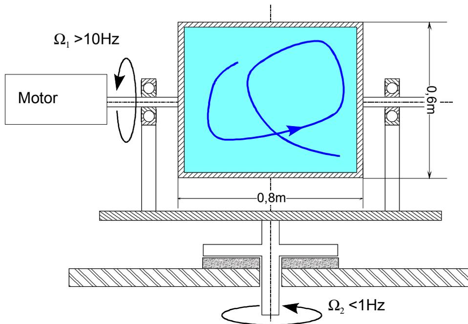
Figure 3.8. Sketch of the French precession flow driven dynamo experiment after J. Alemany et al. (2000); proposed design data: cylinder diameter: 0.6 m, height: 0.8 m, rotation rates:  $\Omega_1 < 10$  Hz,  $\Omega_2 < 1$  Hz, achievable magnetic Reynolds numbers  $R \leq 150$ .
