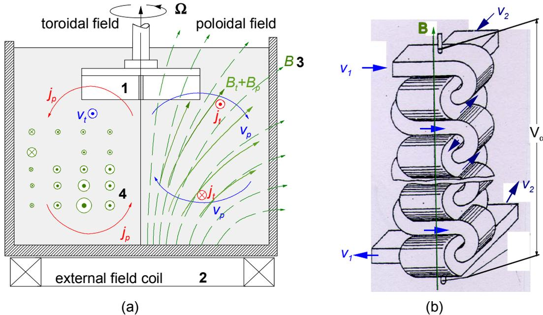
Figure 3.1. a) Lehnert's (1957) experiment of stirred sodium in a cylindrical container penetrated by an external magnetic field: 1 stirring propeller, 2 coil for external field generation, 3 initial poloidal magnetic field, 4 induced toroidal magnetic field components. b) Principle sketch of the Riga  $\alpha$ -Effect experiment by Steenbeck et al. (1967).
