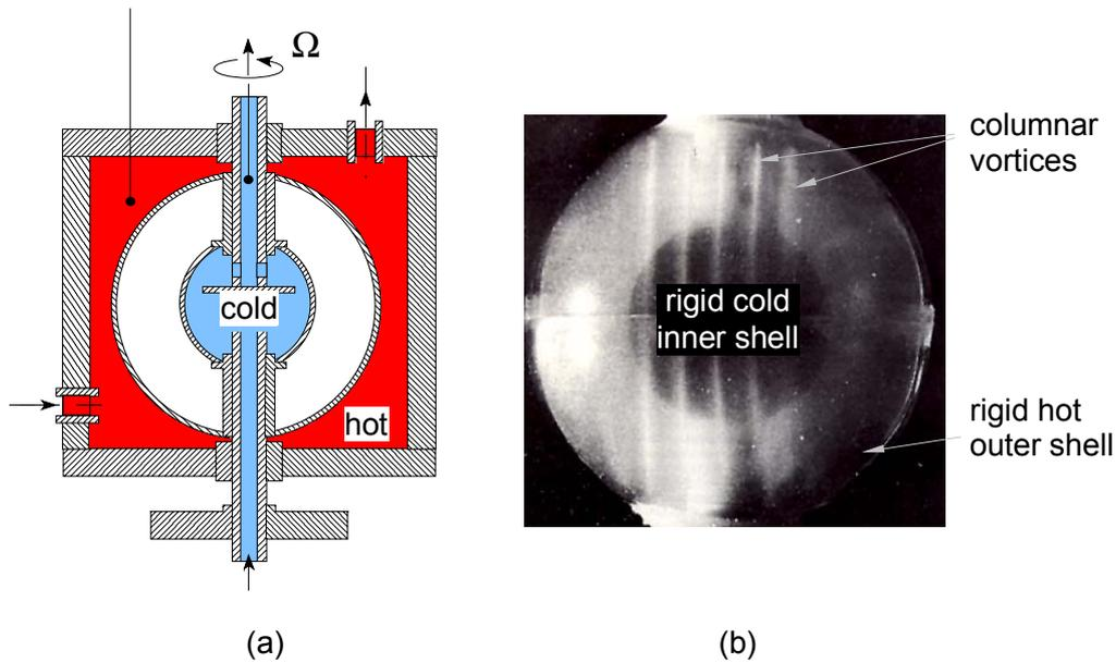
Figure 1.4: Test apparatus of Carrigan & Busse (1983), a) design of the test section, b) visualisation of Taylor-Proudman columns by light reflecting flow tracers mixed into the test fluid.
