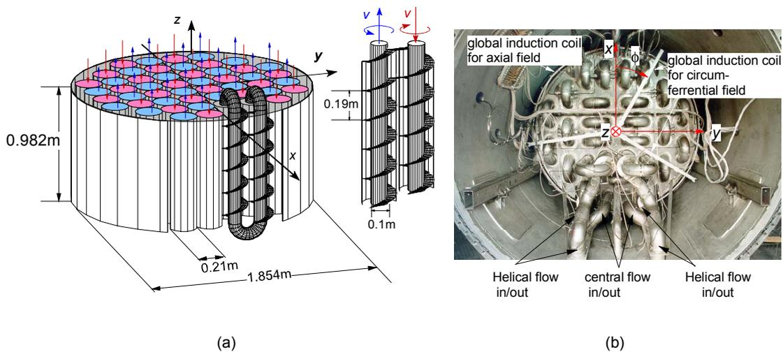
Figure 3.4. a) Principle sketch of the Karlsruhe dynamo module. b) Photo of the technical performance of the module.
