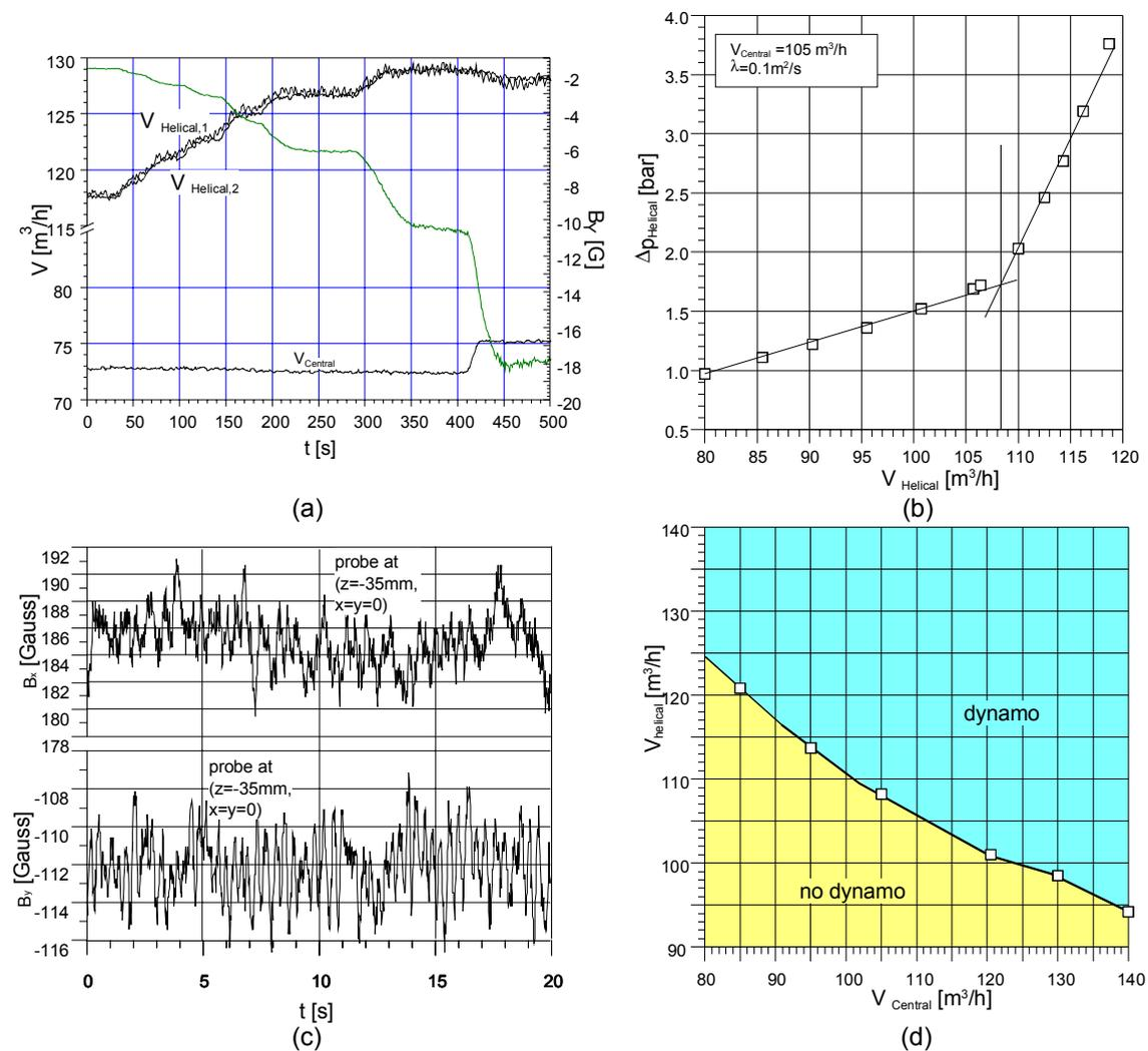
Figure 3.5. Experimental results of the Karlsruhe dynamo experiment: a) self-excitation of the magnetic induction demonstrated by the y-component  $B_y$  and transitions to saturation after each increase of the volumetric flow rate, b) pressure loss increase after self-excitation, c) time fluctuations of the saturated magnetic field, d) phase diagram for dynamo action.
