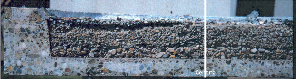
Figure 23: Porous concrete layer after test, sectioned in direction NE to SW
