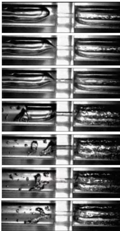
Figure 11: Bubble behavior at orifice (msec)
