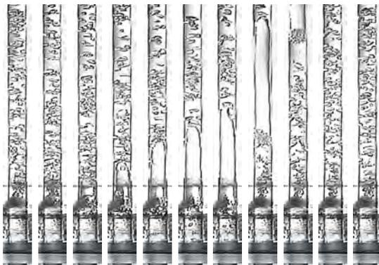
Figure 3: Flow pattern transition in upward flow ( $j_L = 0.1$  m/s,  $j_G = 0.03$  m/s,  $\tau = 2$  s,  $\Delta j_L = 0.327$  m/s, vertical upward flow, successive photo period 0.2s).
