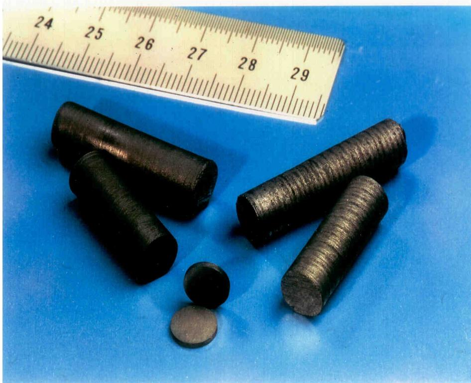
Fig.1. Cylindrical specimens and disks from graphite (left, darker) and CFC (right, striated metallic appearance) obtained by coring virgin JET tiles.
