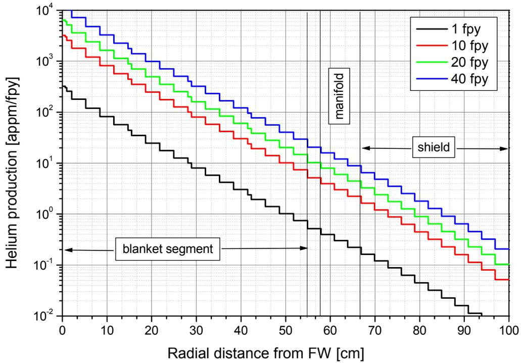
Fig.. 5-9: PPCS model A: Radial profiles of the Helium produced in the Eurofer structure of the inboard WCLL blanket segment at torus mid-plane.
