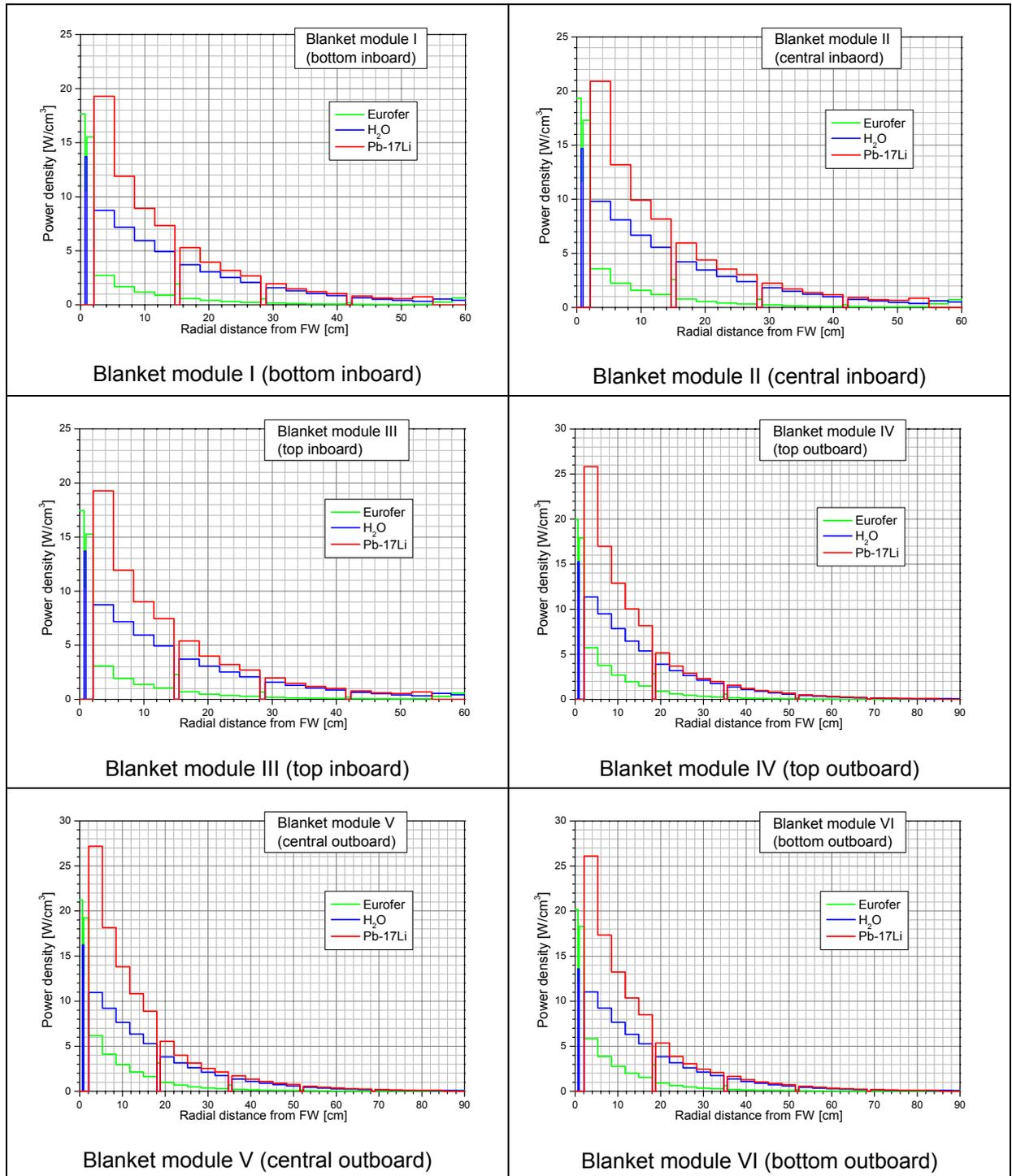
Fig. 5-5: PPCS model A: Radial power density profiles for the different materials in the WCLL blanket modules I-VI
