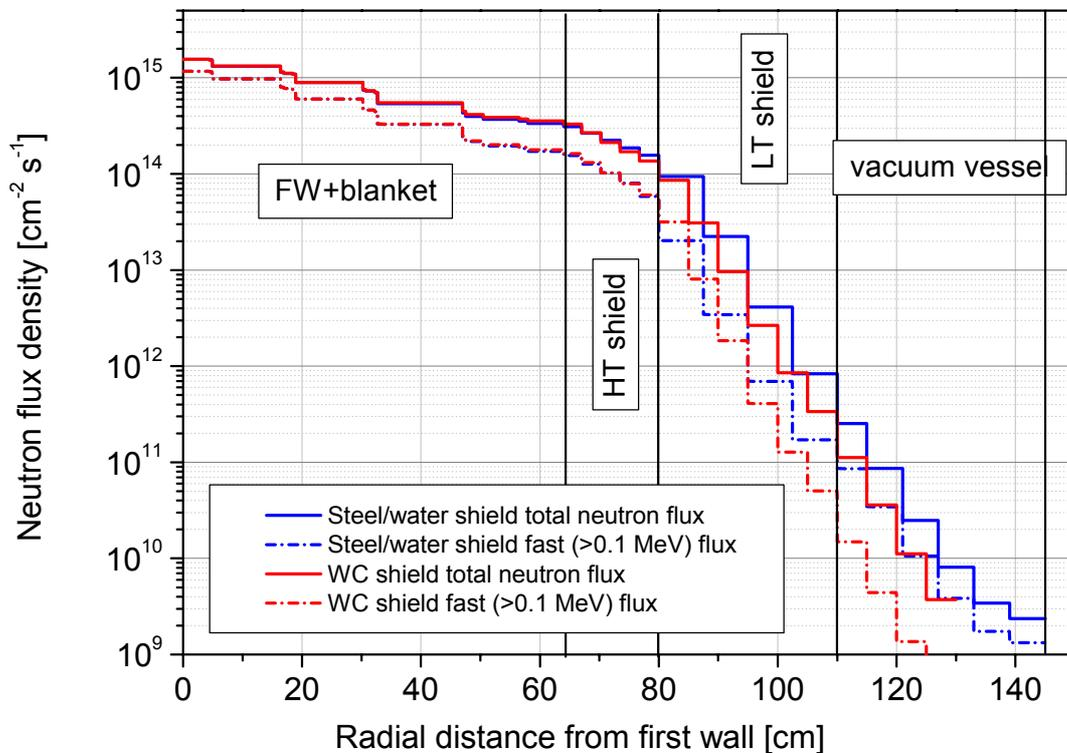
Fig. 5-16: PPCS model C: Radial neutron flux profiles at the inboard mid-plane for different shield variants of the DCLL blanket
