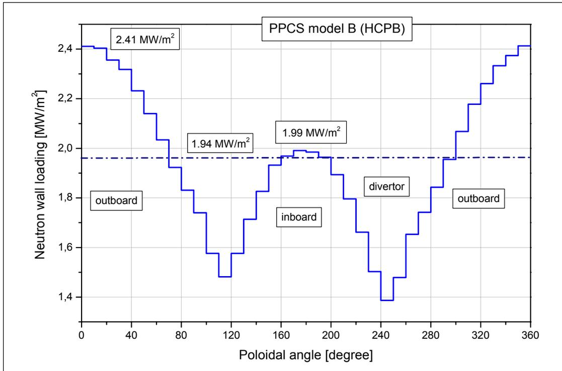
Fig. 5-2: PPCS model B (HCPB): Poloidal neutron wall loading distribution.
