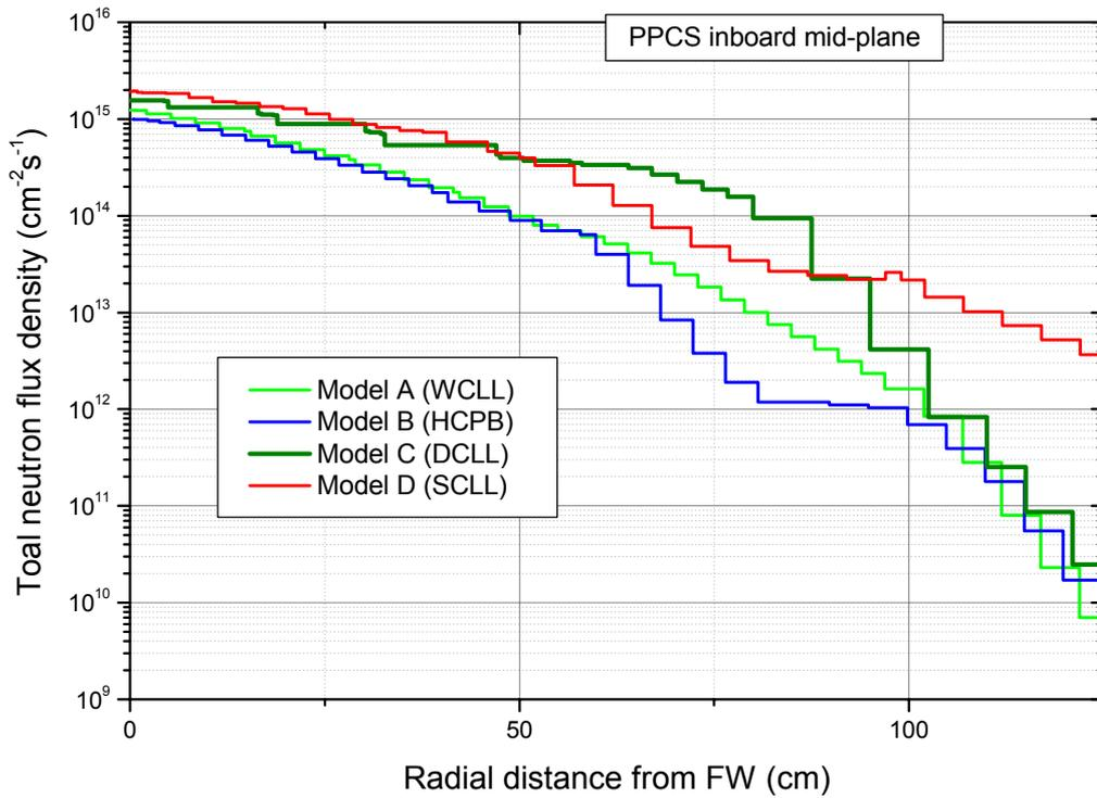
Fig. 5-13: Total neutron flux densities: Radial profiles at the inboard mid-plane of the four PPCS power plants
