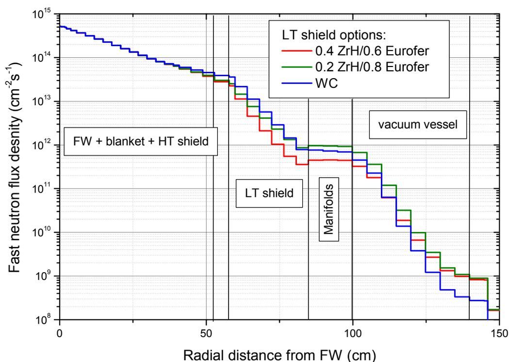
Fig. 5-15: PPCS model B: Fast ( $E > 0.1$  MeV) neutron flux profiles at the inboard mid-plane for different shield variants of the HCPB blanket.
