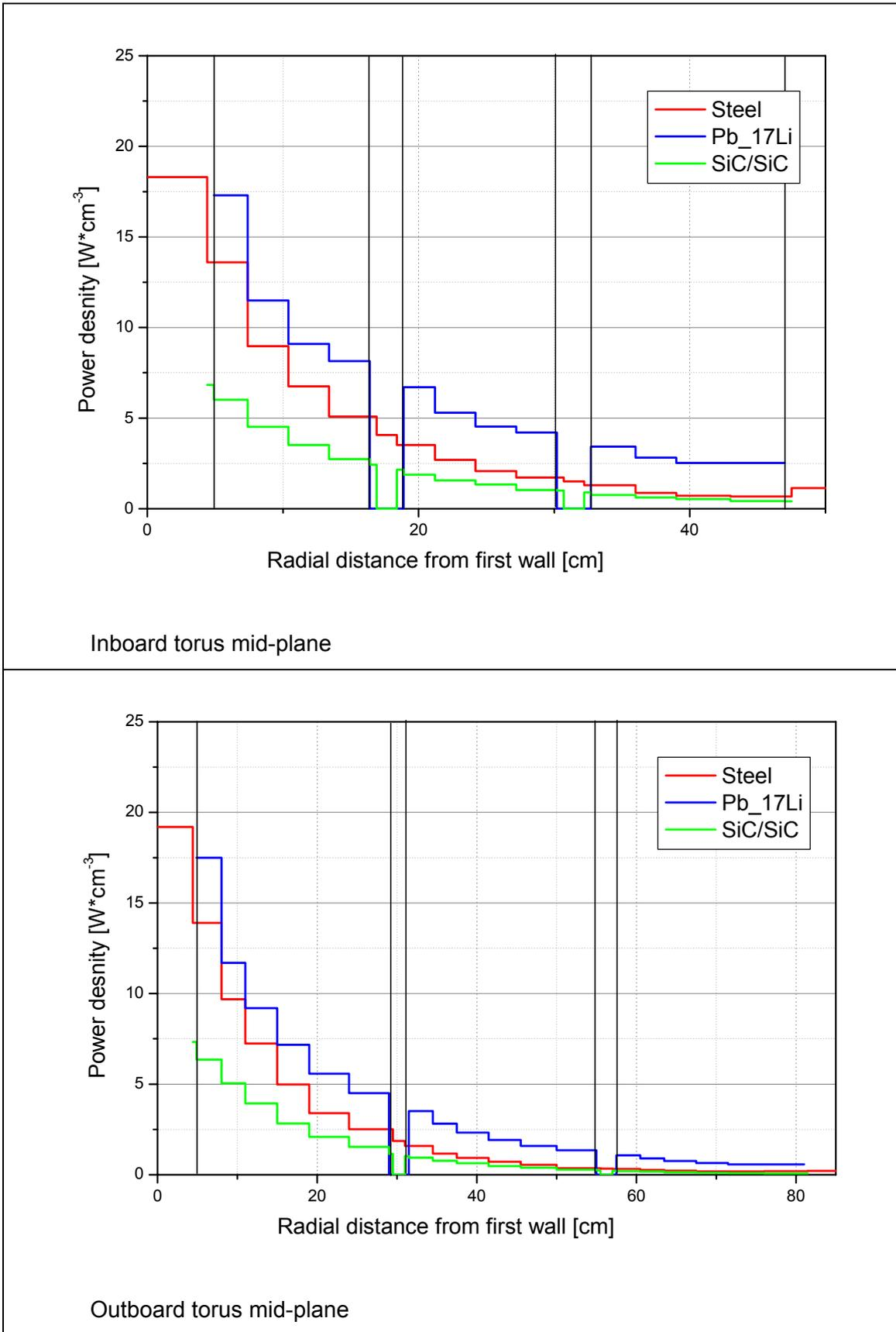
Fig. 5-7: PPCS model C: Radial power density profiles of the materials in the inboard and outboard DCLL blanket segments at torus mid-pane
