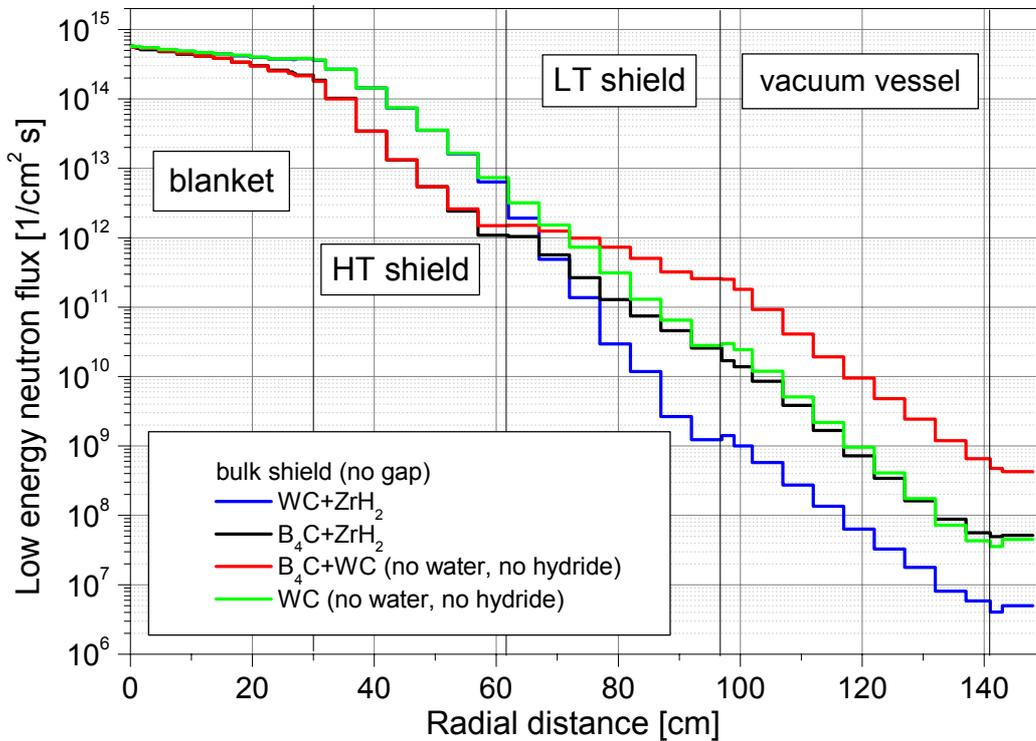
Fig. 5-19: PPCS model D (SCLL): Low energy ( $E < 0.1$  MeV) neutron flux profiles at the inboard mid-plane for WC and B<sub>4</sub>C shield variants without segment gap.
