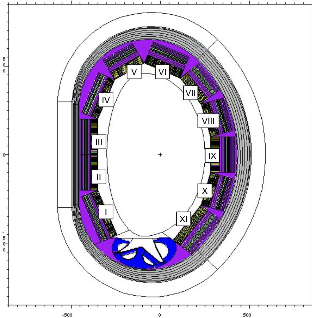
Fig. 3-3 PPCS model B (HCPB): vertical cut through MCNP torus sector model
