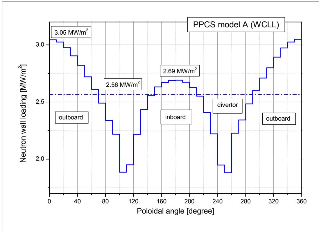
Fig. 5-1: PPCS model A (WCLL): Poloidal neutron wall loading distribution
