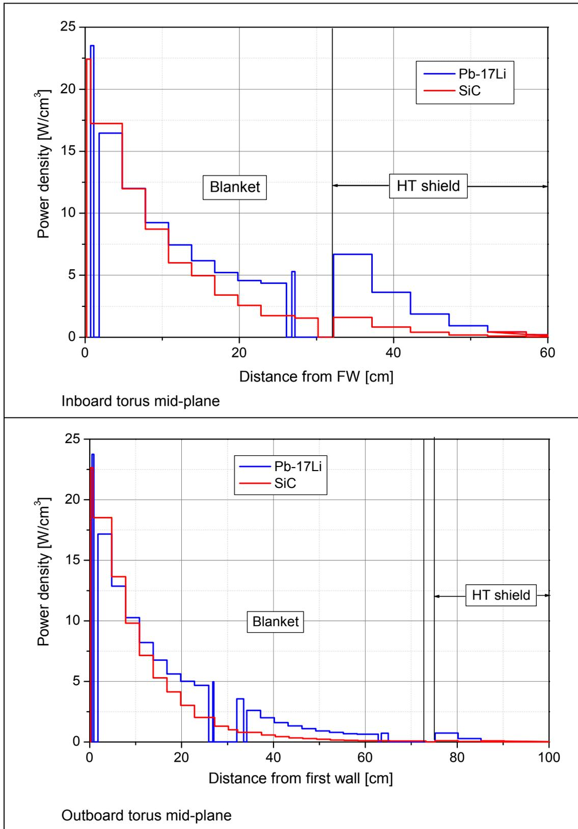
Fig. 5-8: PPCS model D: Radial power density profiles of the materials in the inboard and outboard SCLL blanket segments at torus mid-plane
