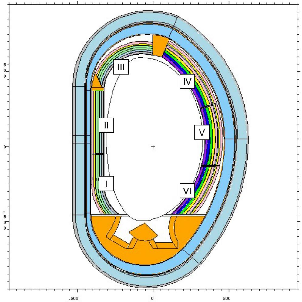
Fig. 3-1 PPCS model A (WCLL): vertical cut through MCNP torus sector model.
