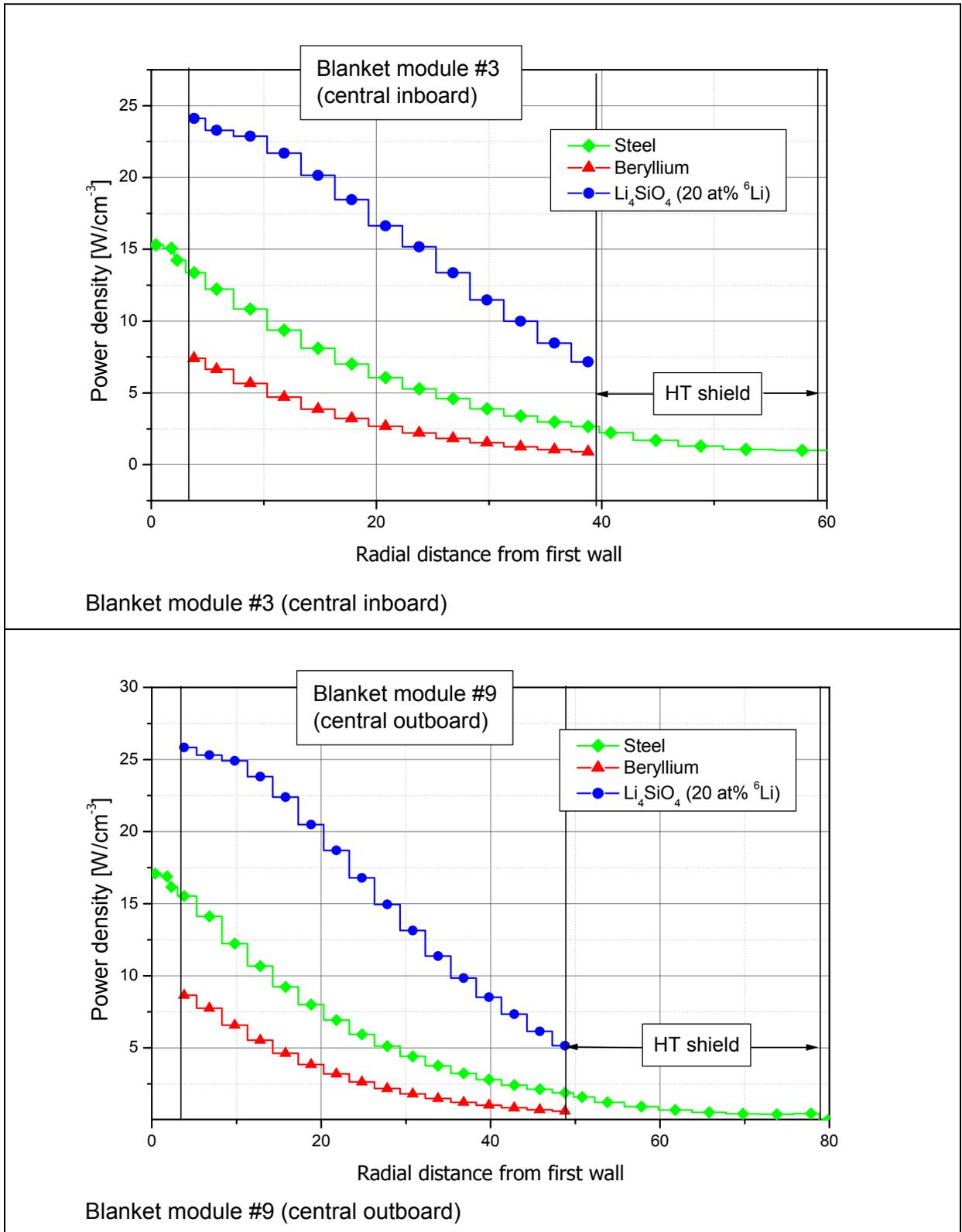
Fig. 5-6: PCS model B: Radial power density profiles of the materials in the central in-board and outboard HCPB blanket modules
