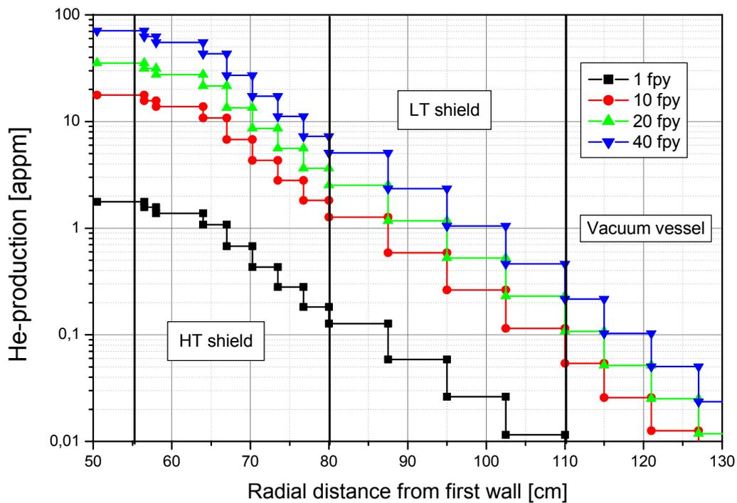
Fig. 5-11: PPCS model D: Radial profiles of the Helium produced in the Eurofer structure of the HT and LT shields of the inboard DCLL blanket segment at torus mid-plane.
