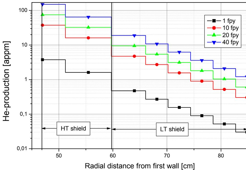
Fig. 5-10: PPCS model B: Radial profiles of the Helium produced in the Eurofer structure of the HT and LT shields of the central inboard HCPB blanket module.
