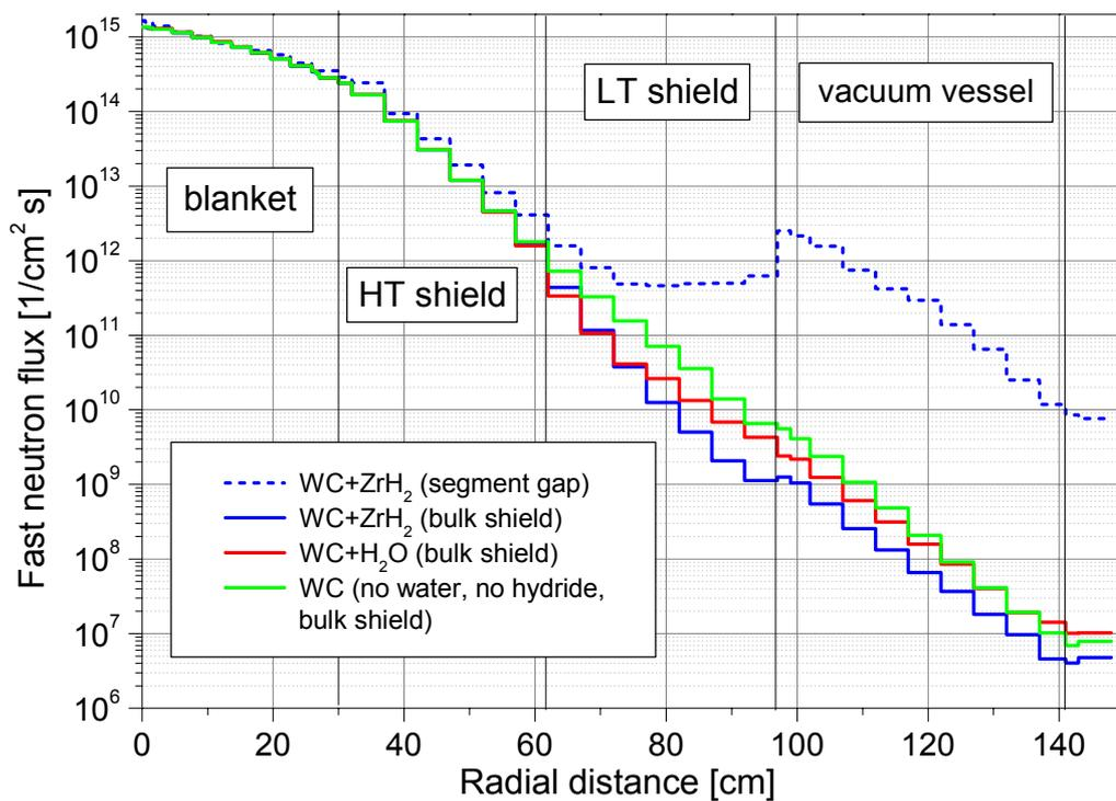
Fig. 5-17: PPCS model D (SCLL): Fast ( $E > 0.1$  MeV) neutron flux profiles at the inboard mid-plane for different WC shield variants with and without segment gap.
