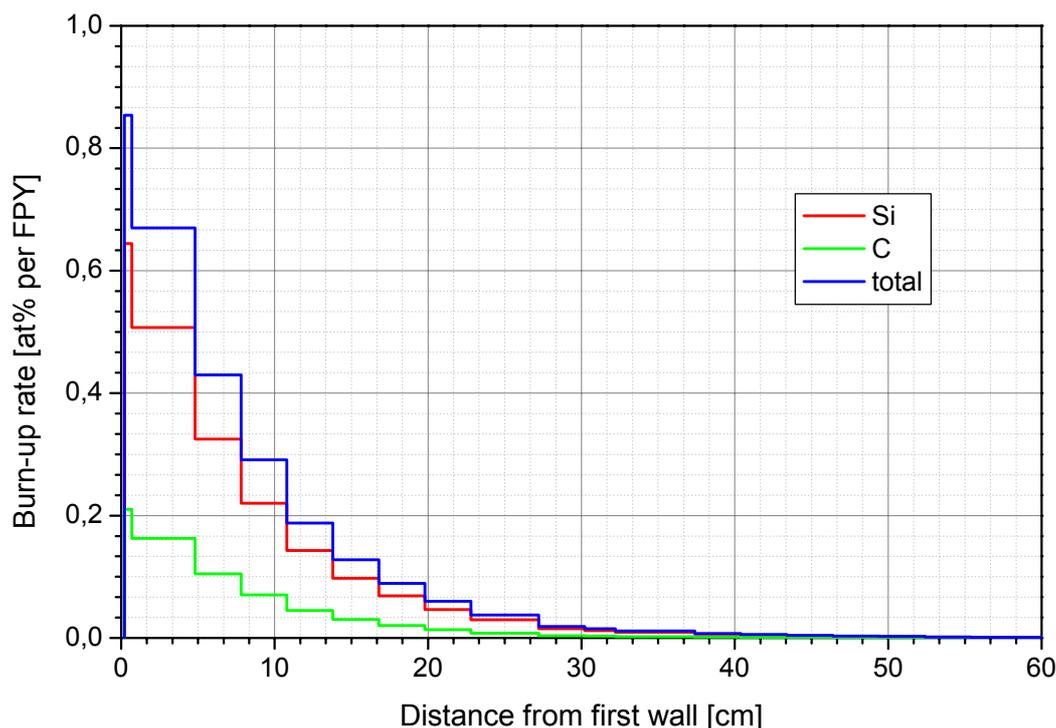
Fig. 5-12: PPCS model D: Radial profile of SiC burn-up in SCLL outboard blanket segment at torus mid-plane.
