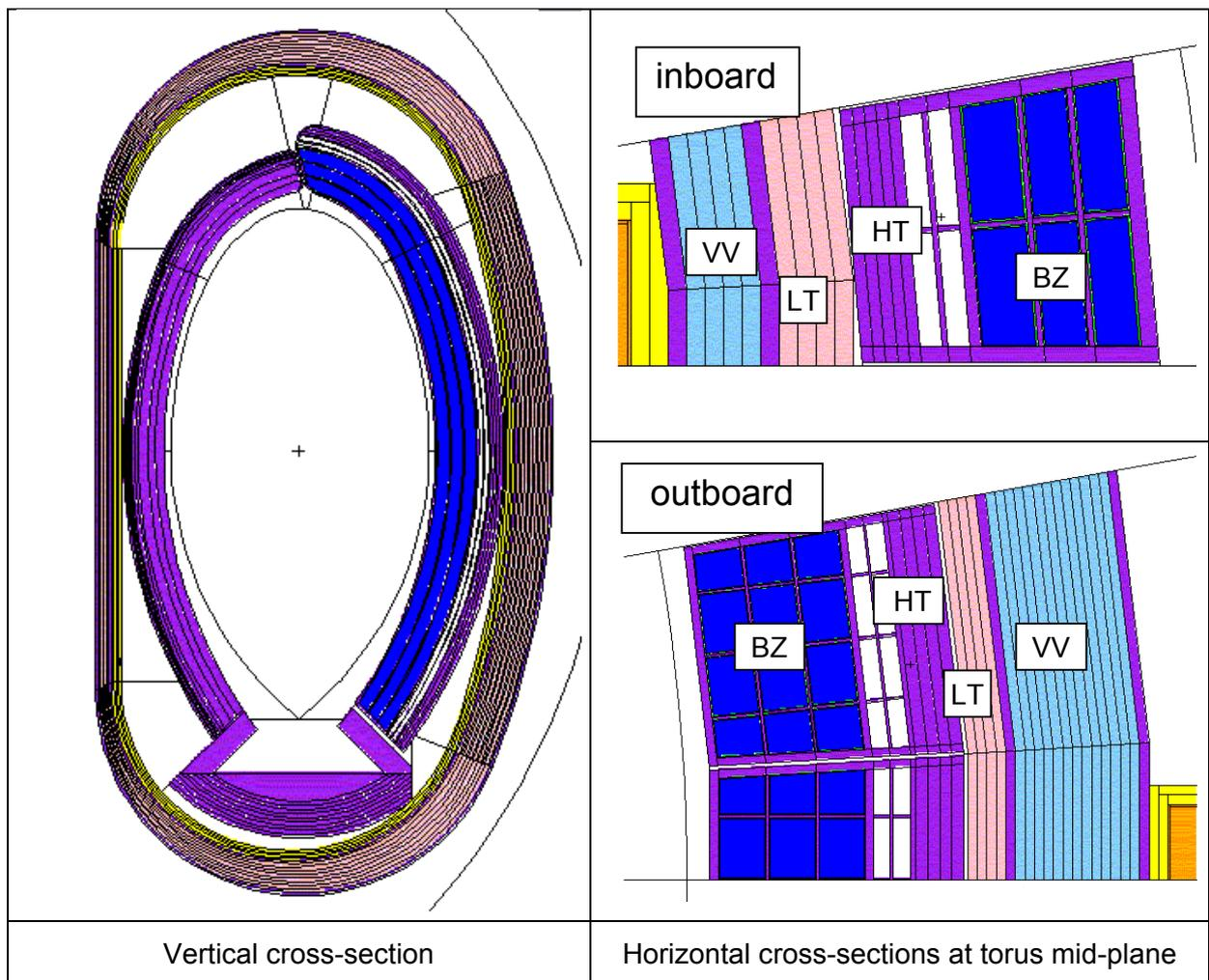
Fig. 3-6: PPCS model C (DCLL): MCNP torus sector model (10°)
