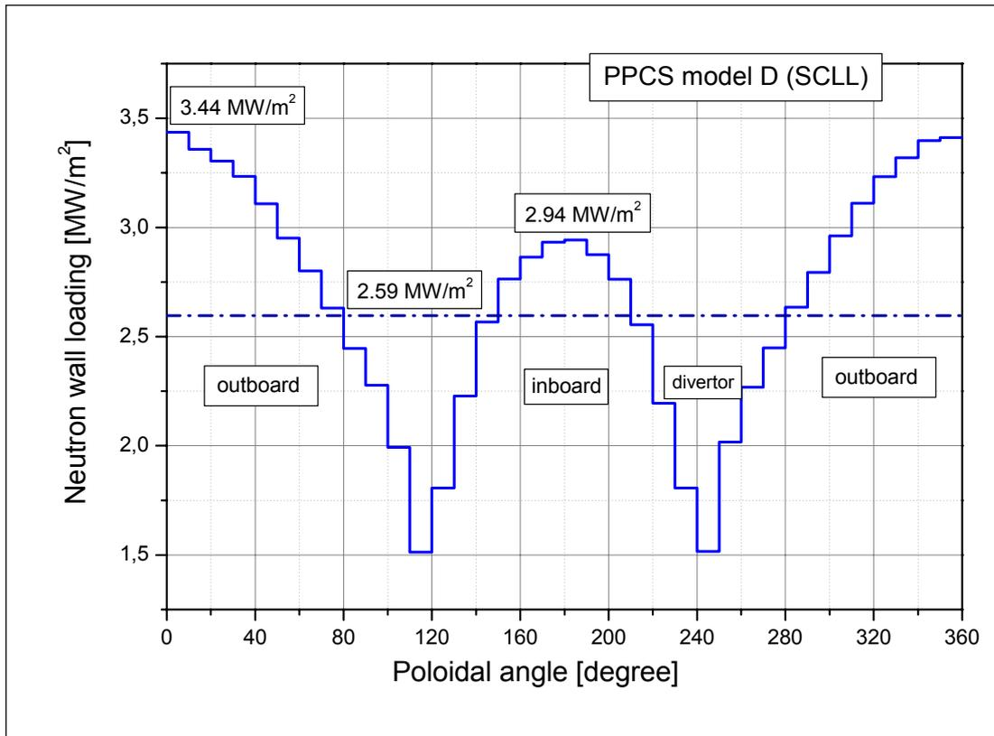
Fig. 5-4: PPCS model D (SCLL): Poloidal neutron wall loading distribution
