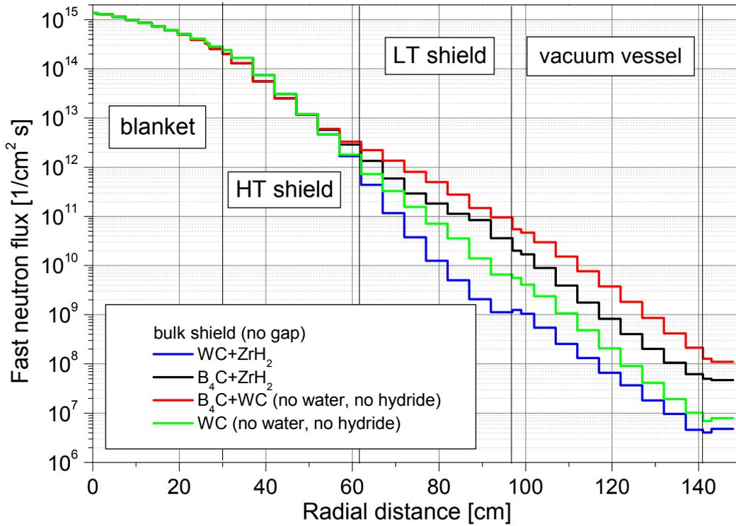
Fig. 5-18: PPCS model D (SCLL): Fast ( $E > 0.1$  MeV) neutron flux profiles at the inboard mid-plane for WC and B<sub>4</sub>C shield variants without segment gap.
