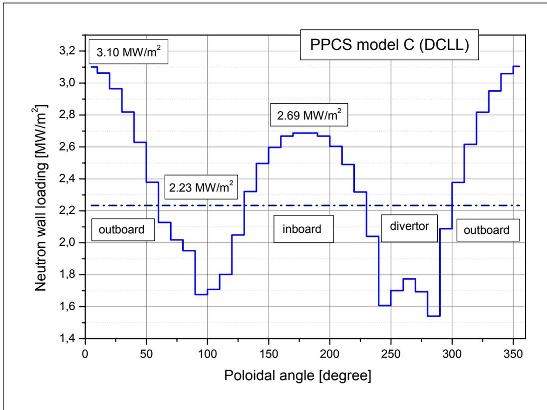
Fig. 5-3: PPCS model C (DCLL): Poloidal neutron wall loading distribution.
