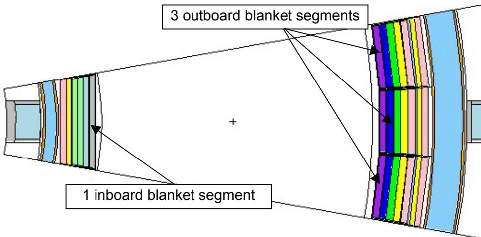
Fig. 3-2 PPCS model A (WCLL): horizontal cut through MCNP torus sector model (20°)
