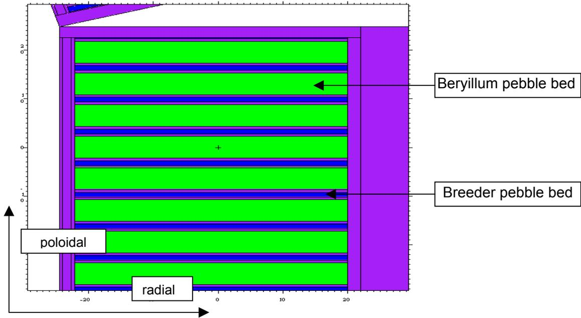
Fig. 3-5 PPCS model B (HCPB): Poloidal-radial arrangement of pebble beds (central outboard HCPB blanket module, cut through MCNP model)
