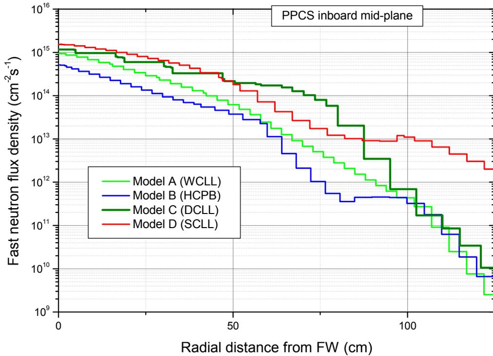
Fig. 5-14: Fast ( $E > 0.1$  MeV) neutron flux densities: Radial profiles at the inboard mid-plane of the four PPCS power plants
