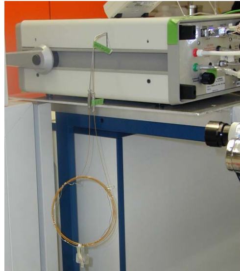
Fig. 1: The micro gas chromatograph used for hydrogen isotope analysis with the external analytical column.
