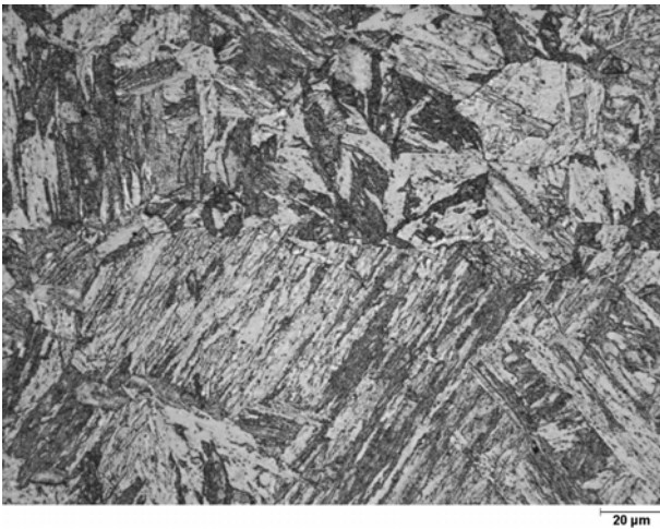
Fig. 1: Micrograph of the EB seal welded FW specimen with dry-milled surface after the 2nd HIP step.
