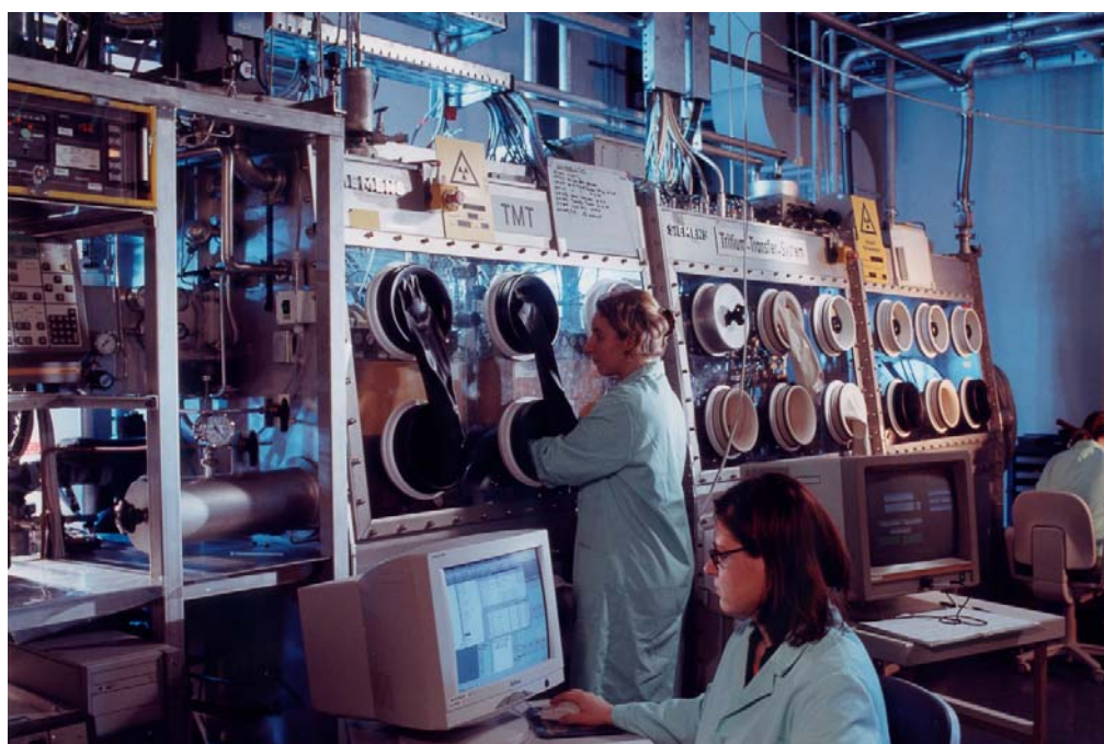
The Tritium Transfer System and Tritium Measurements at TLK
