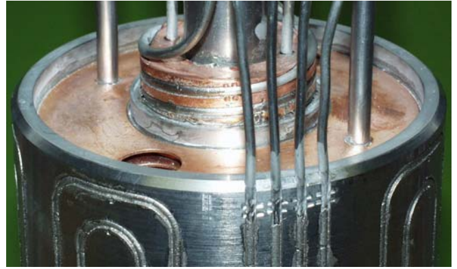
Fig. 3: Upper most fins and thermocoax heaters after the brazing process.
