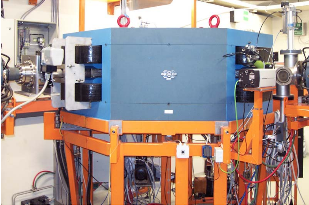
Fig. 2: Magnet of the Karlsruhe compact cyclotron with two induction coils.
