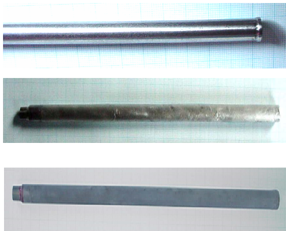
Fig. 1: Steel tubes for HD processing (from top to bottom). Tube as delivered after surface conditioning. Tube after aluminization by HD. Tube after heat treatment.
