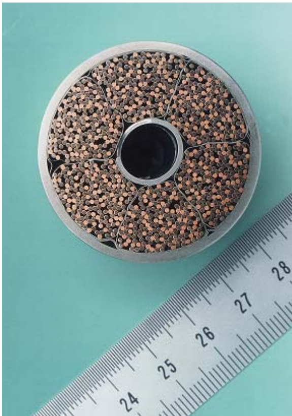
Fig. 5: The conductor cross section of the TFMC with the central hole and the bundle region (light strands: Cu; dark strands: Nb 3 Sn)
