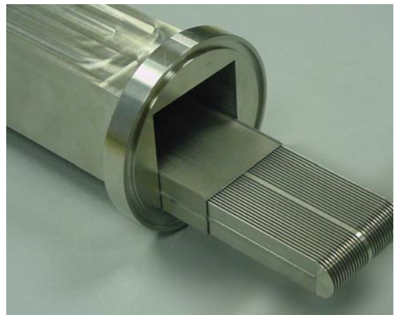
Fig. 6: Manufacturing test of capsule, rig and container; the outer surfaces and the grooves on the capsule surface (design variant with heaters wound vertically) are milled; all hollow spaces are spark eroded; the container has a flange on both sides; the wall thickness is 1mm; the components are made from solids which were annealed before milling and spark erosion.
