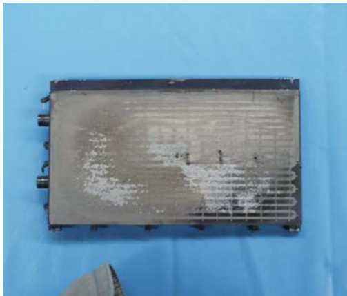
Fig. 3: Locally baked ceramic pebbles at the heating plate.
