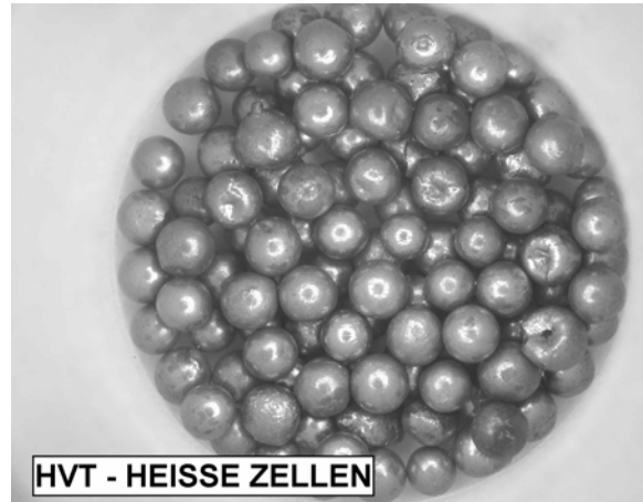
Fig. 1: 1 mm NGK beryllium pebbles (FZK Hot cells: optical microscopy).
