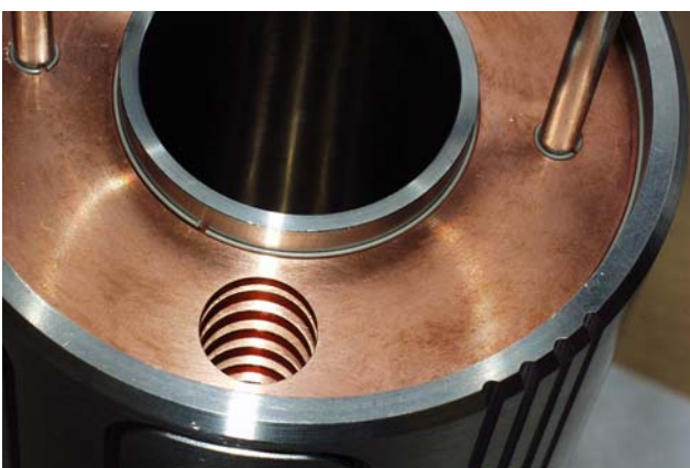
Fig. 2: Upper most Cu fins between internal and external walls with brazing rings.
