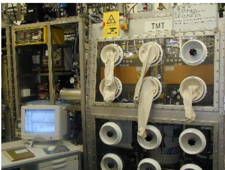
Fig. 3.2.3: View on a large section of the TMT glove box: On the left side the main electronic equipment is visible, whereas GC1 and GC2 are seen on the left and right side behind the upper window of the TMT glove box.
