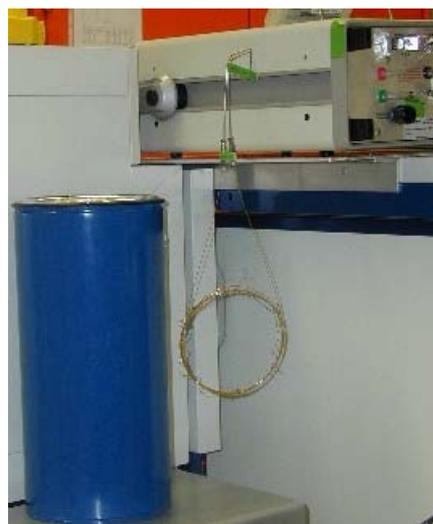
Fig. 3.5.4: Agilent  $\mu$ GC1 with external analytical column placed in liquid nitrogen and freely hanging. The oven for regeneration of the column is visible behind the dewar in the photo on the right side.
