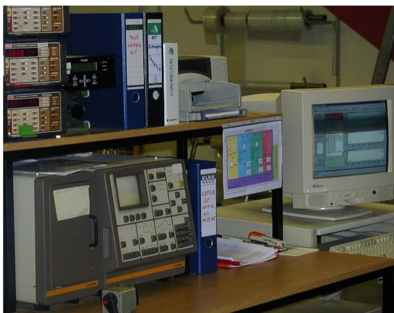
Fig. 3.3.5: Part of the electronic units to control the gas chromatograph GC3.
