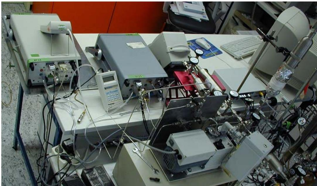
Fig. 3.5.3: Bird view on the experimental set-up of the micro gas chromatographs  $\mu$ GC1 and  $\mu$ GC2 and on the pipe work used for preparation and injection of samples.
