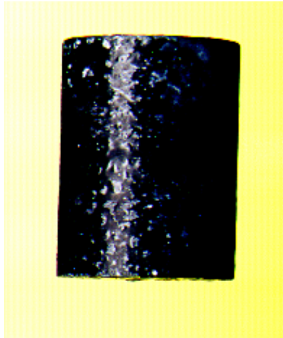
Fig.17: Dense B 4 C pellet after exposure to Ar-steam at 1000 °C
