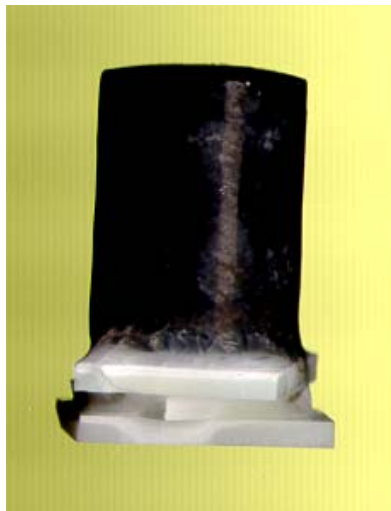
Fig. 14: Flow down of oxide scale. The sample support is covered by a glassy B_2O_3 skin
