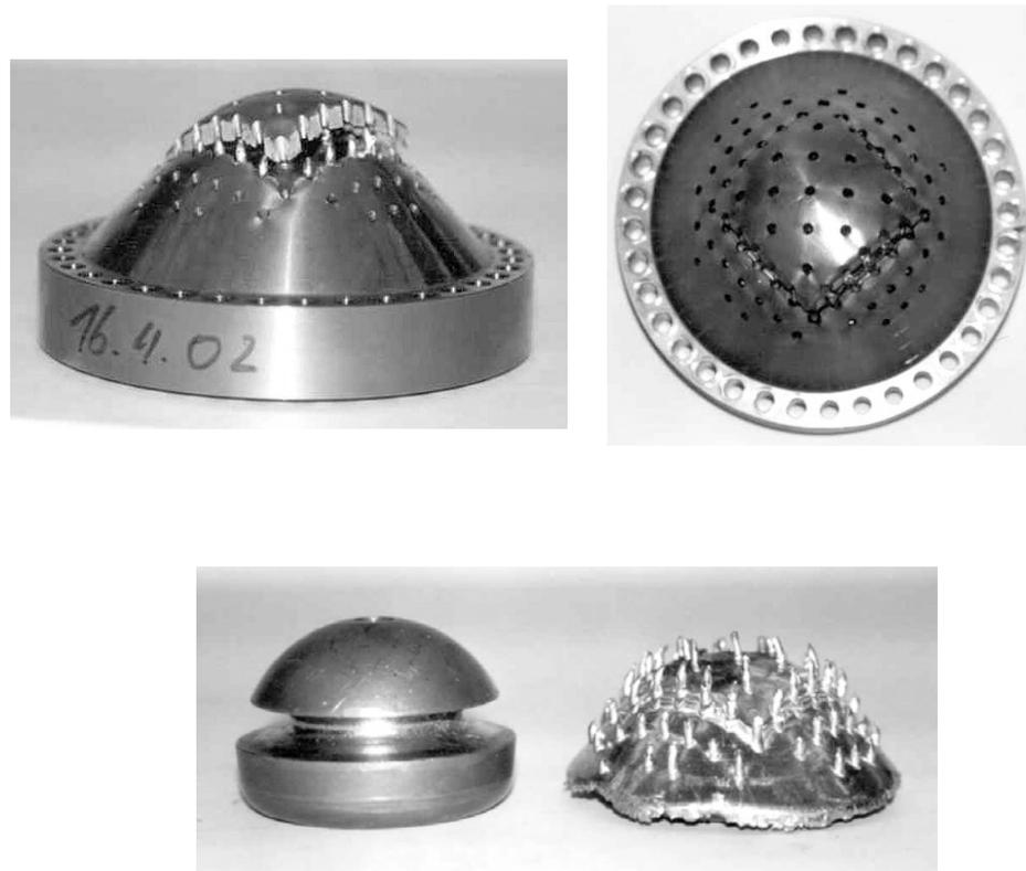
**Fig. 12:** Failure of a small specimen with holes and lead mass with the large specimens
