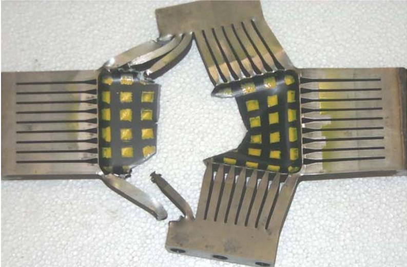
**Fig. 14:** Specimen EO with hole before and after the test
