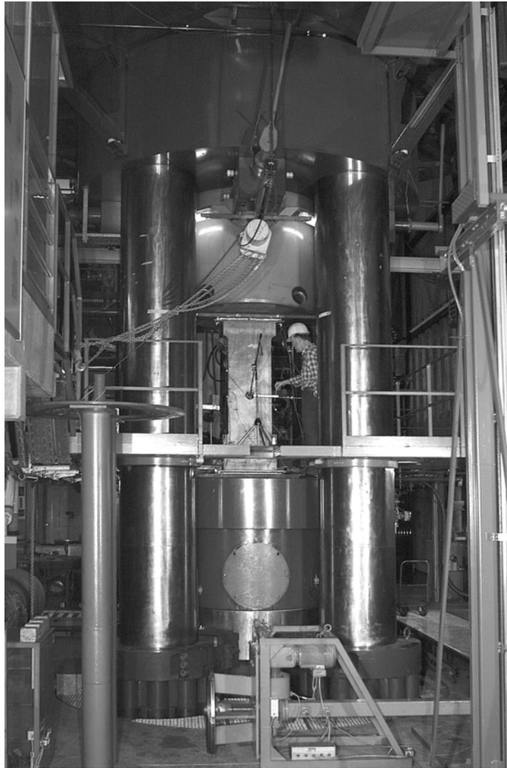
**Fig. 3:** Tensile testing machine of 100 MN (MPA) used for the flat specimen of 200 mm wall thickness
