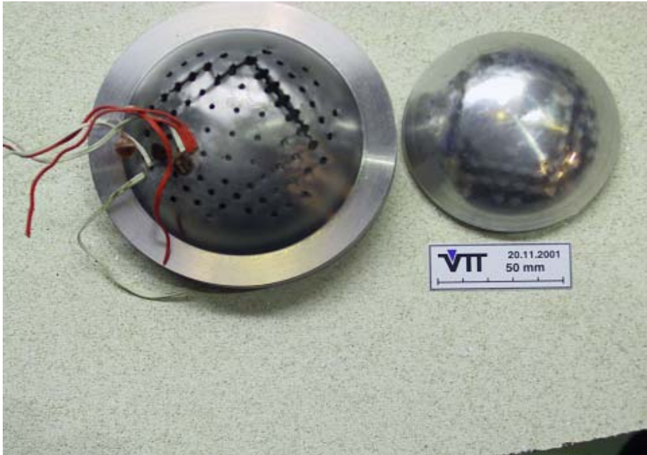
Fig. 3.1.3-7: Failure of the small specimen EZ1 and deformation of the liner
