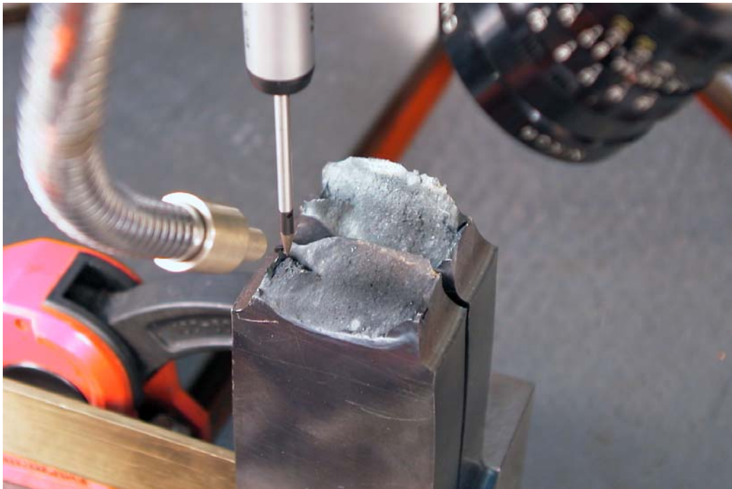
Fig. 3.1.4-2: Fracture surfaces of the broken parts of a specimen to be scanned by the mechanical probe of a three dimensional measuring machine.
