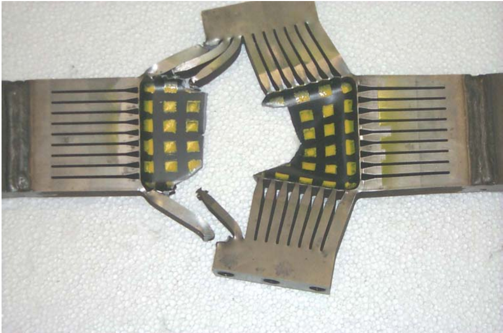
Fig. 3.1.3-16: Specimen EO with hole before and after the test
