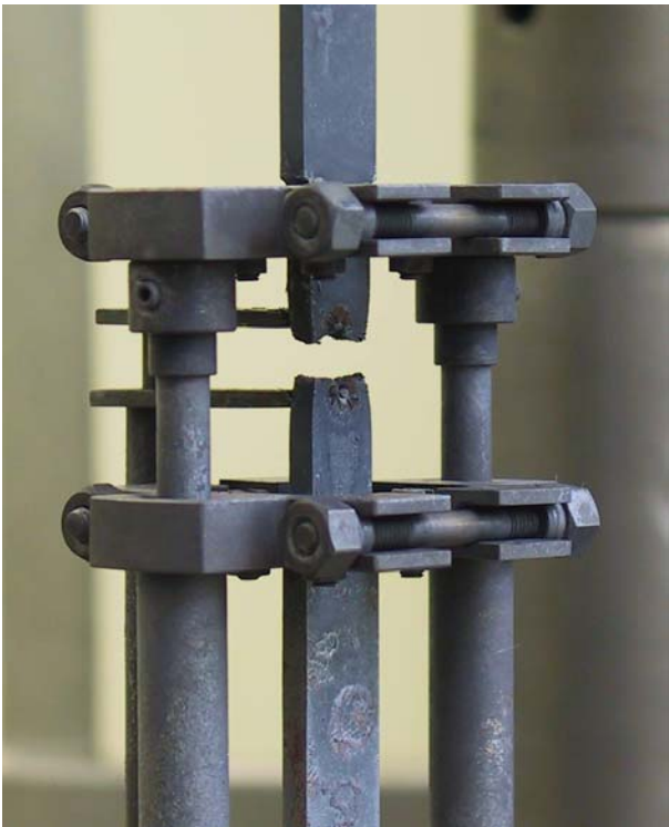
Heating facility and measurement on flat specimens of 4 mm wall thickness at 850 °C
