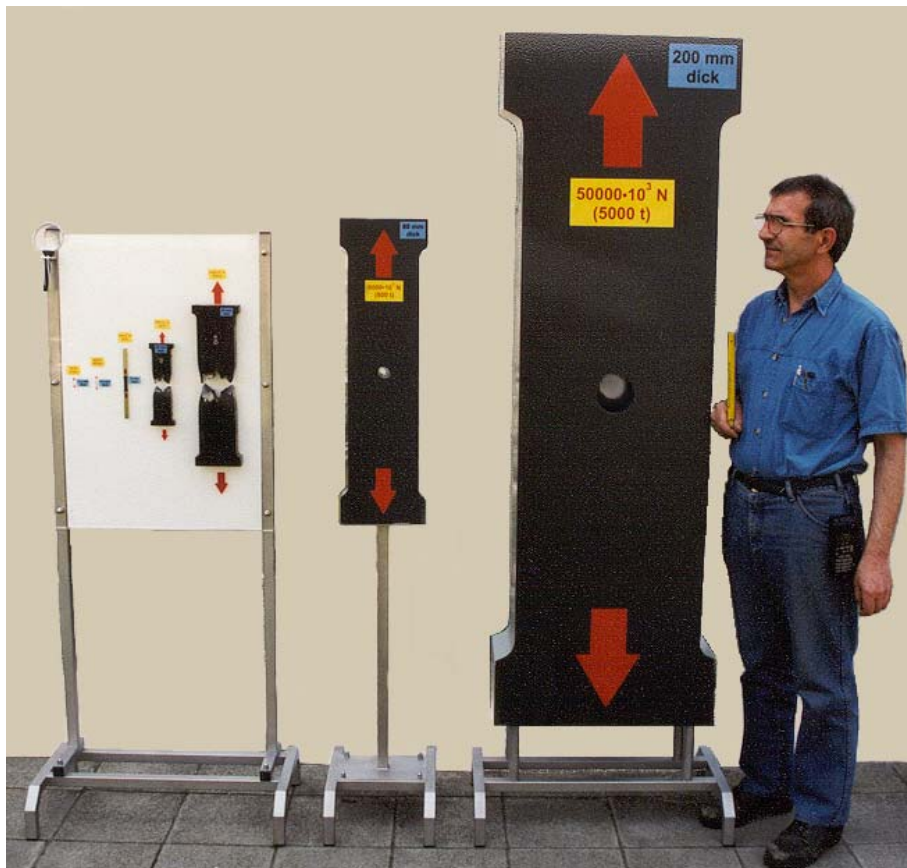
Fig. 2.1.1-3: Flat specimens with a hole. The smallest specimen has a thickness of 4 mm, the largest a thickness of 200 mm
