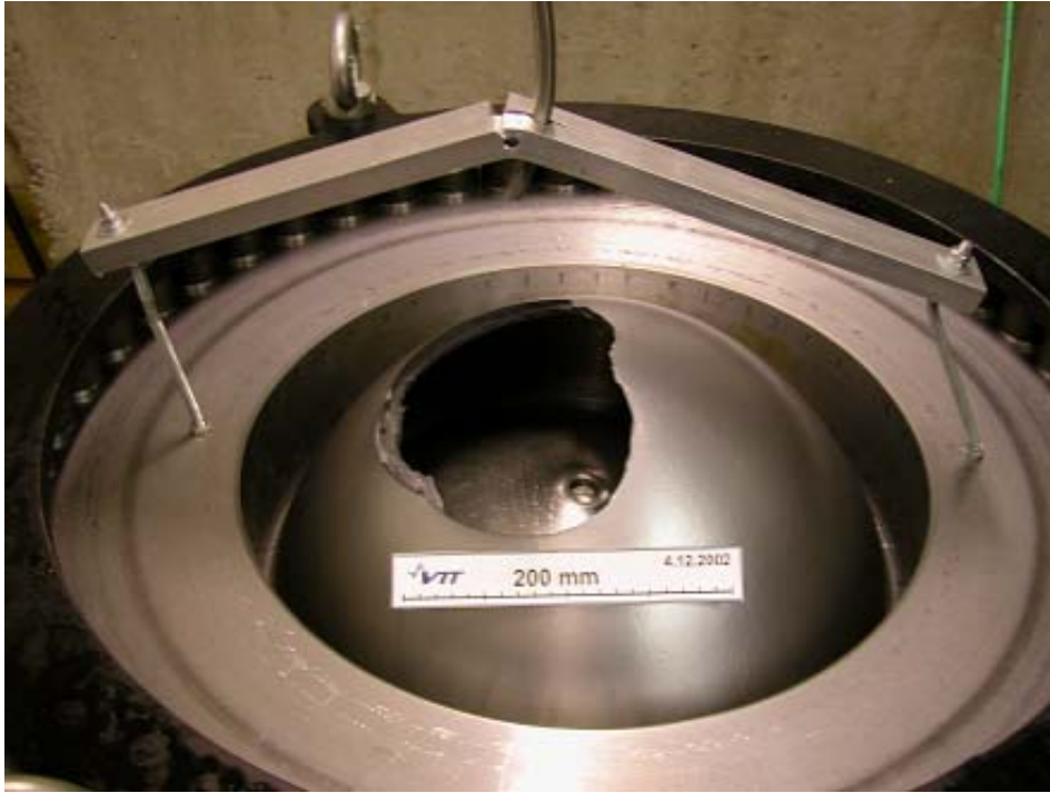
Fig. 3.1.3-6: Failure of the large specimen EW. A large part of the specimen was completely torned off.
