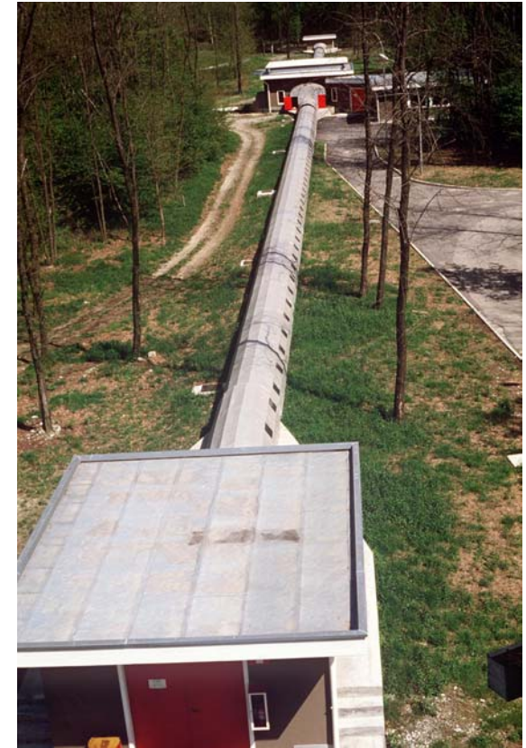
Fig. 3.1.2-24: (a) Principle of functioning and dimensions of the large Hopkinson bar at the Large Dynamic Test Facility (LDTF) of the JRC-Ispra. (b) External view of the LDTF.
