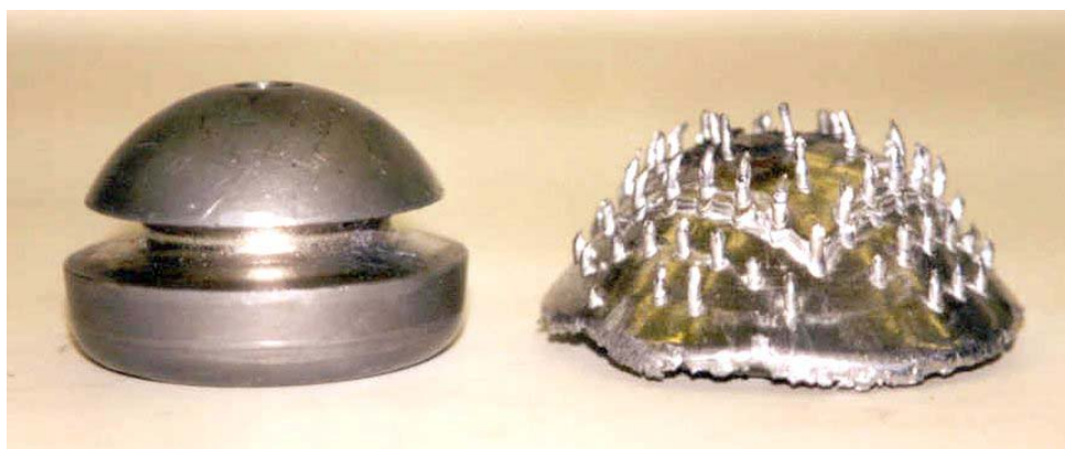
Fig. 3.1.3-12: Failure of the small specimen FO1 and lead mass before and after the impact
