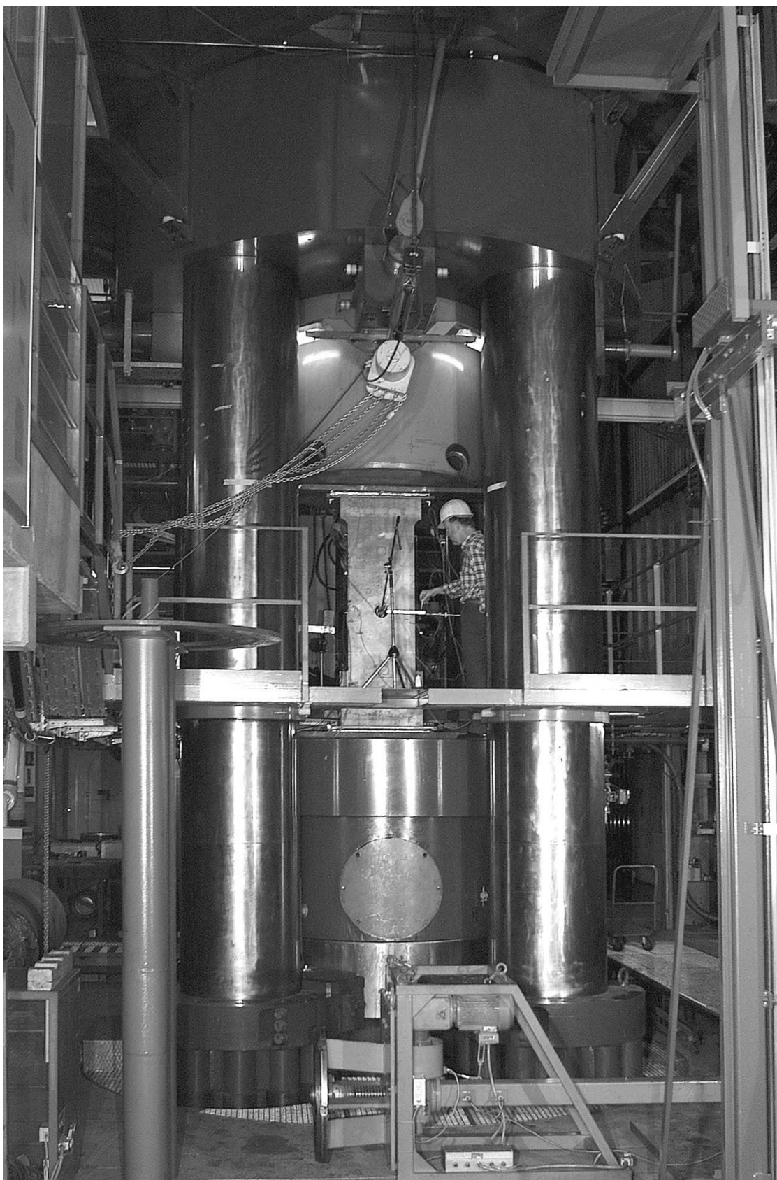
Fig. 3.1.2-1: Tensile testing machine of 100 MN (MPa) used for the flat specimen of 200 mm wall thickness
