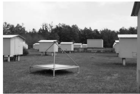
Fig. 2. Antennas for the measurement of radio emission in air showers are set-up at the KASCADE experiment.
