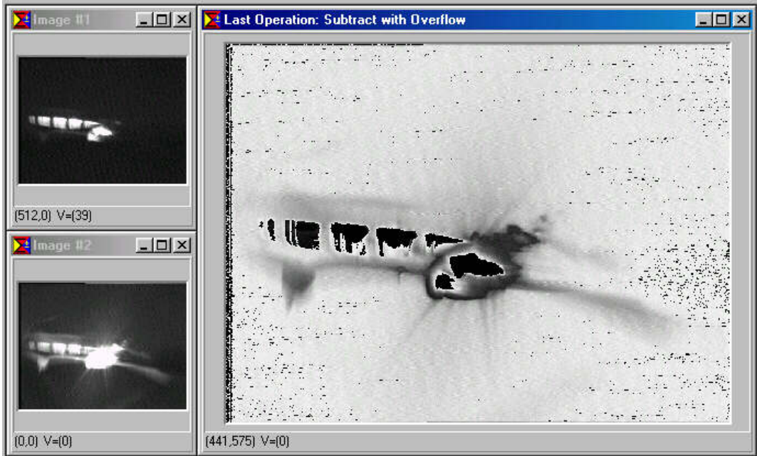
Figure 20: “Subtraction with overflow” of image 1 (“Tv52”) @ 1200 °C / 1550 °C and image 2 (“Tv53”) @ 1250 °C / 2250 °C
