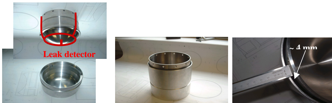
Figure 10: Photos of the dummy parts of the lower target part. (1) target window with the catcher and the schematically leak detector; (2) inner shell of the lower target enclosure; (3) assembling of (1) and (2); (4) zoom on the 4mm wide insulating gap between the T91 liquid metal container and the LTE (to be filled up with the thermal shield).
