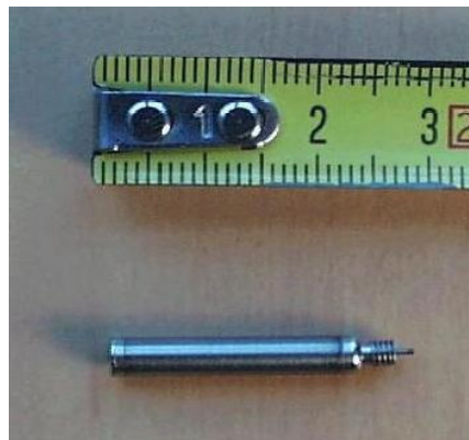
Figure 8: Photography of a fission micro-chamber.
