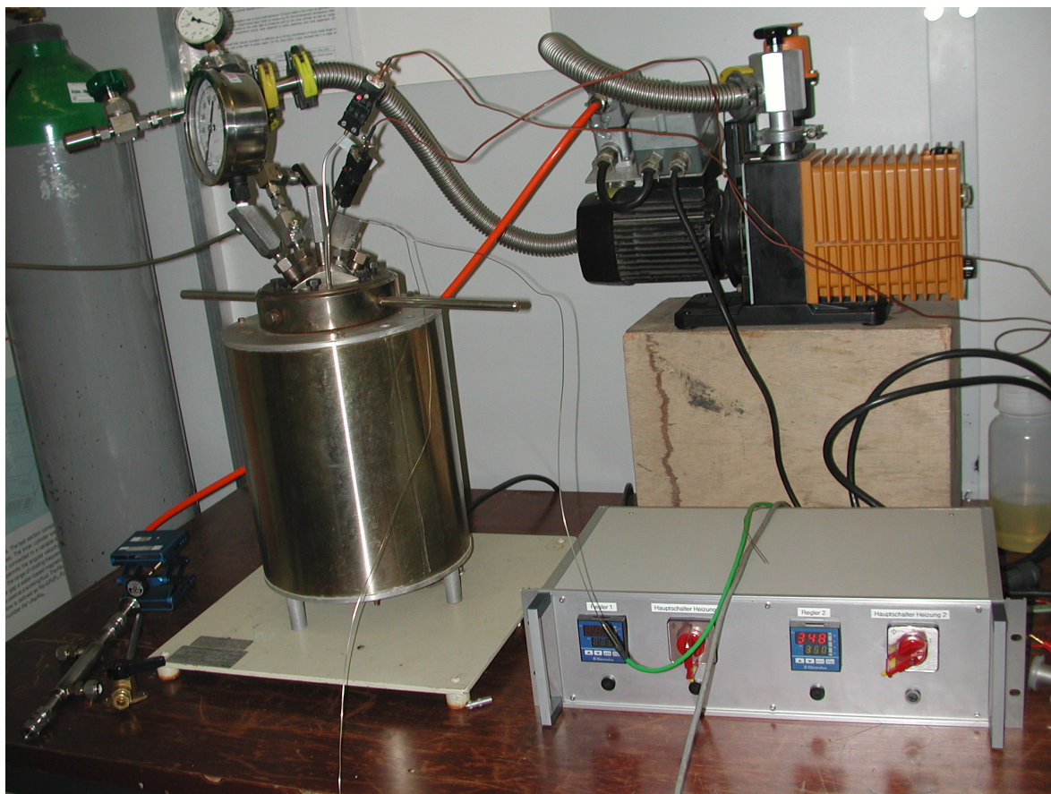
Figure 1. Photo of the DTHT-LBE interaction experimental set-up.
