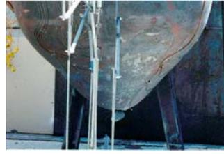
Uniform heating, failure at 1000 K
