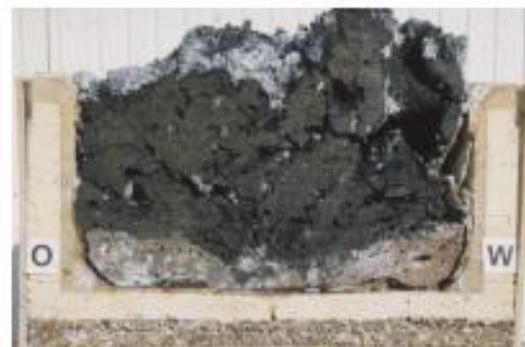
Solidification of the simulated core melt in COMETPC
