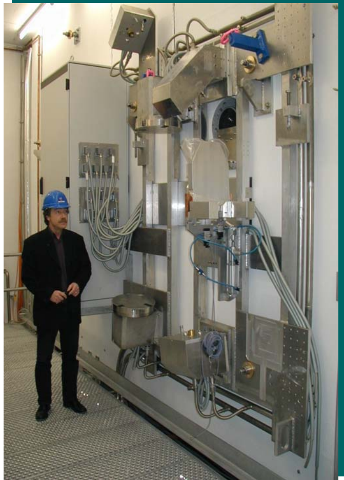
Fig. 3: Matching optics and polarizers for one gyrotron.
