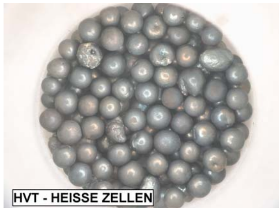
Fig. 1: Be pebbles with 1mm diameter from NKG produced by REP.
