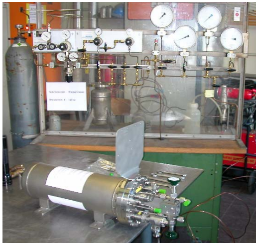
Fig. 2: Equipment used for the pressure tests of the various volumes inside the hydrogen storage bed.
