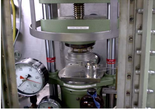
Fig. 2: 20 ton hydraulic press for tablet fabrication in a furnace.
