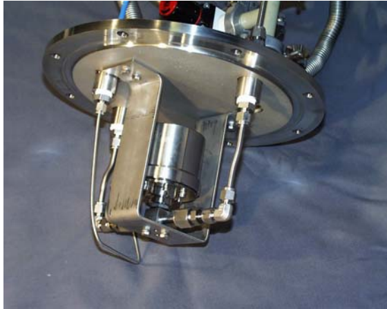
Fig. 4: Calibrated JET-approved (valve+orifice) device for flow control.
