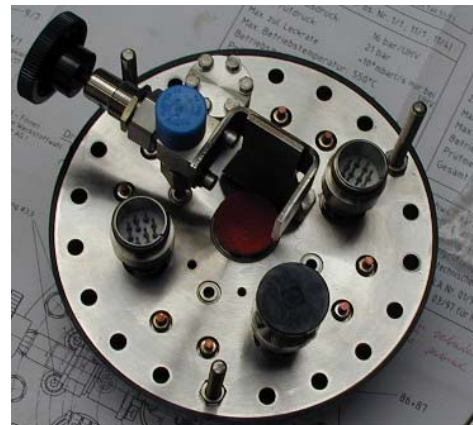
Fig. 1: CF-150 flange and various welded items such as feedthroughs for high electrical currents and for thermocouples.
