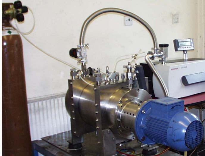
Fig. 2: Pilot pump under leak testing.
