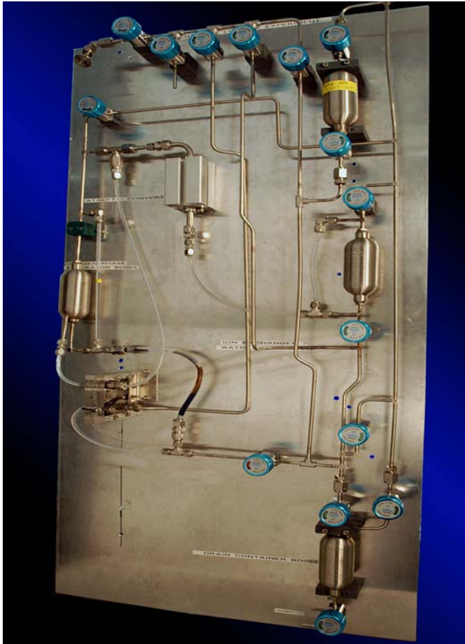
Fig. 1: Experimental rig for endurance testing of a small electrolyser cell.
