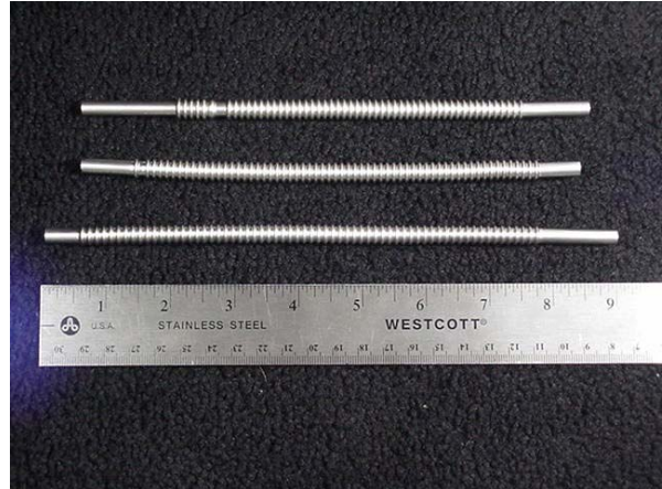
Fig. 3: Palladium /silver tube bellows for the production of advanced PERMCAT's.
