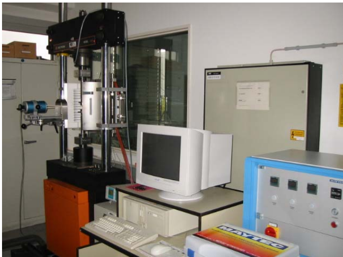
Fig. 1: Modernized LCF-testing facility with furnace, strain measurement system and control devices
