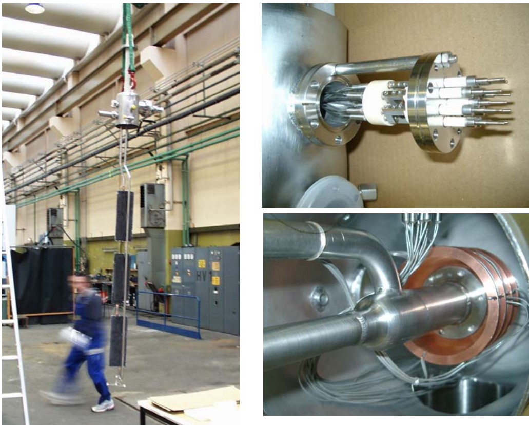
Fig. 2: Complete view and manufacturing details (internal and external feedthroughs for heaters and temperature sensors) of the PCP interior system.
