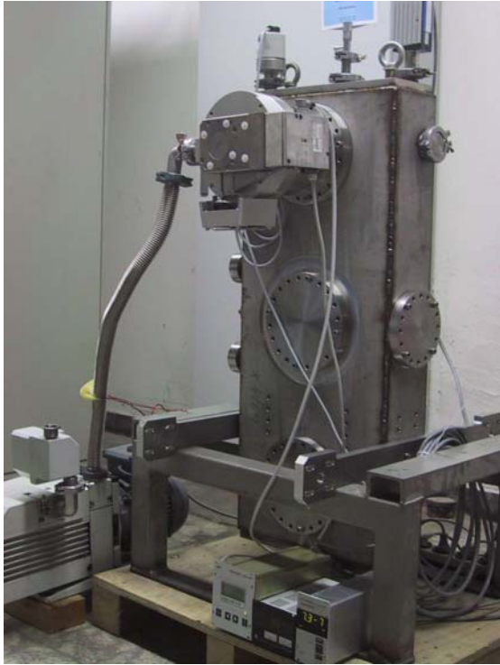
Fig. 5: First diagnostic and pumping chamber for LEBT measurements.
