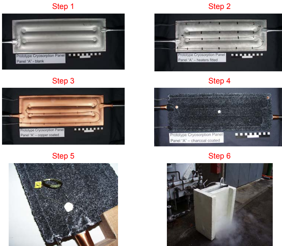
Fig 1: Manufacturing steps for the cryopanel: (1) blank panel, (2) attachment of resistance heaters, (3) copper coating, (4) charcoal bonding, (5) equipment of cryotemperature sensors, (6) thermal cycling in liquid nitrogen for quality control.
