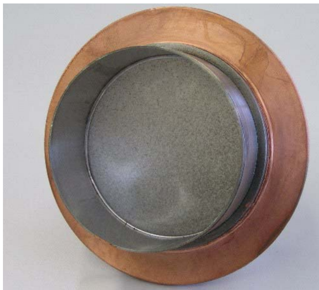
Fig. 1: High power CVD diamond disk for 170 GHz torus window with electroplated Cu on outer section of Al-braze and cooling rim
