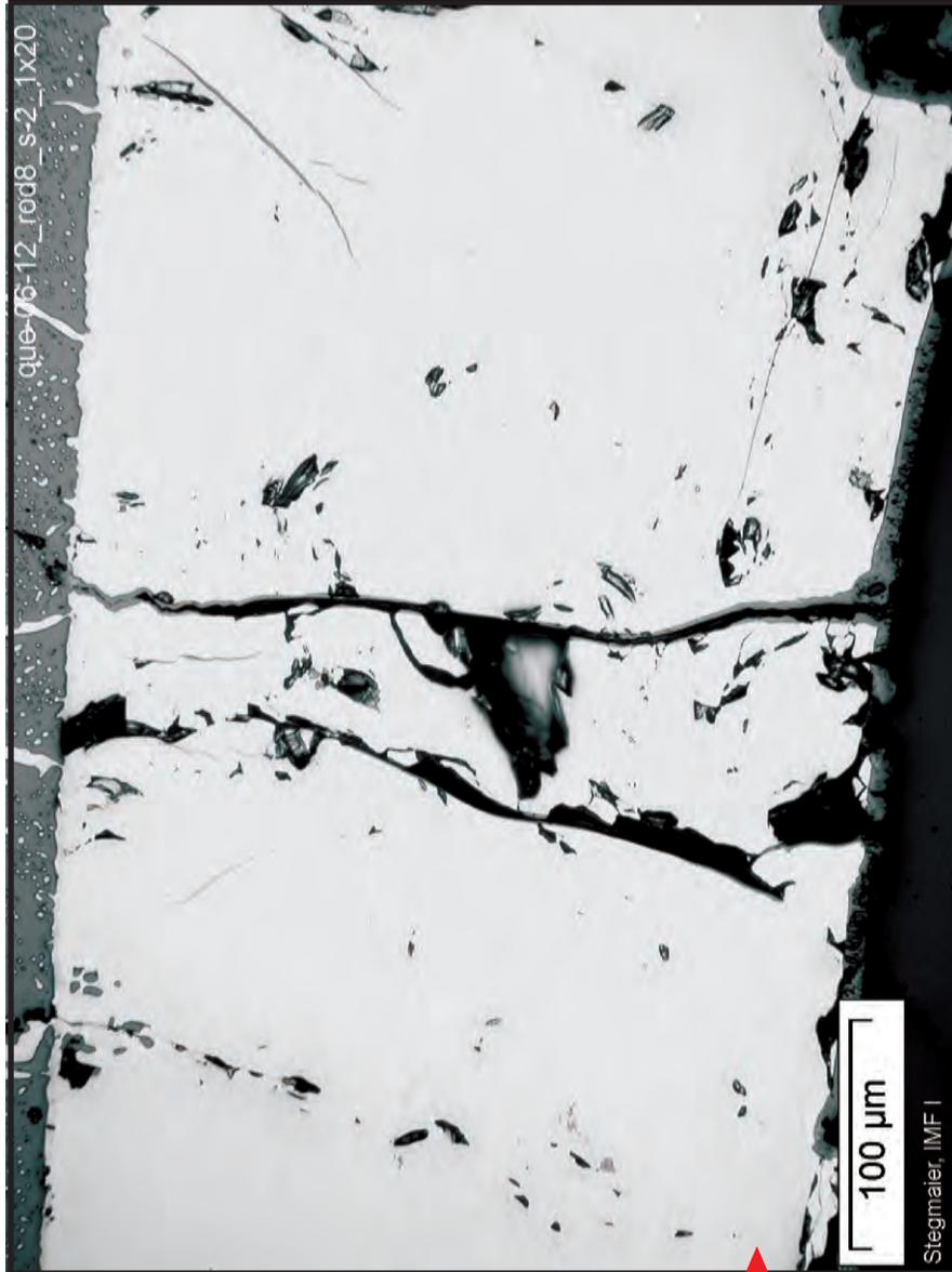
Fig. 70: Cross section at 1000 mm bundle elevation (QUE-06-12); rod No. 8, showing strong external and slight internal oxidation by steam, and non-molten cladding
