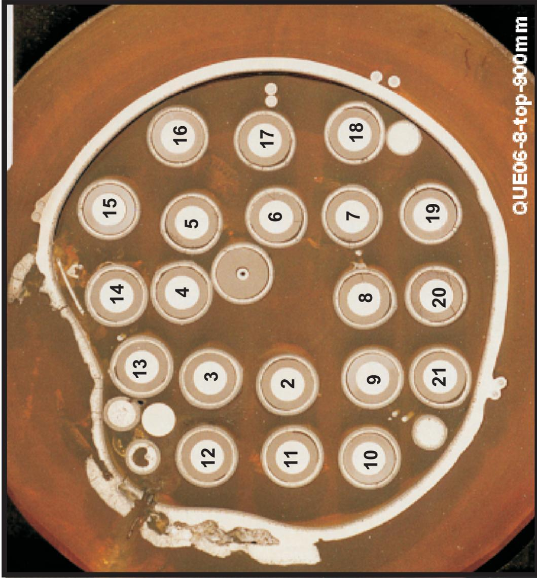
Fig. 59: Cross section at 900 mm bundle elevation (QUE-06-8); overview, state of rods No. 8 and 21
