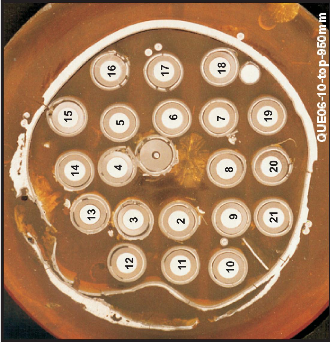
Fig. 63: Cross section at 950 mm bundle elevation (QUE-06-10); overview, rod No. 4 and central rod, both in direct contact
