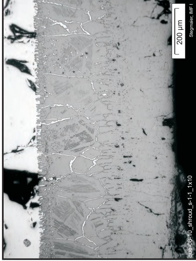
Fig.68: Cross section at 950 mm bundle elevation (QUE-06-10); internal scale of original shroud and oxidation of accumulated shroud melt
