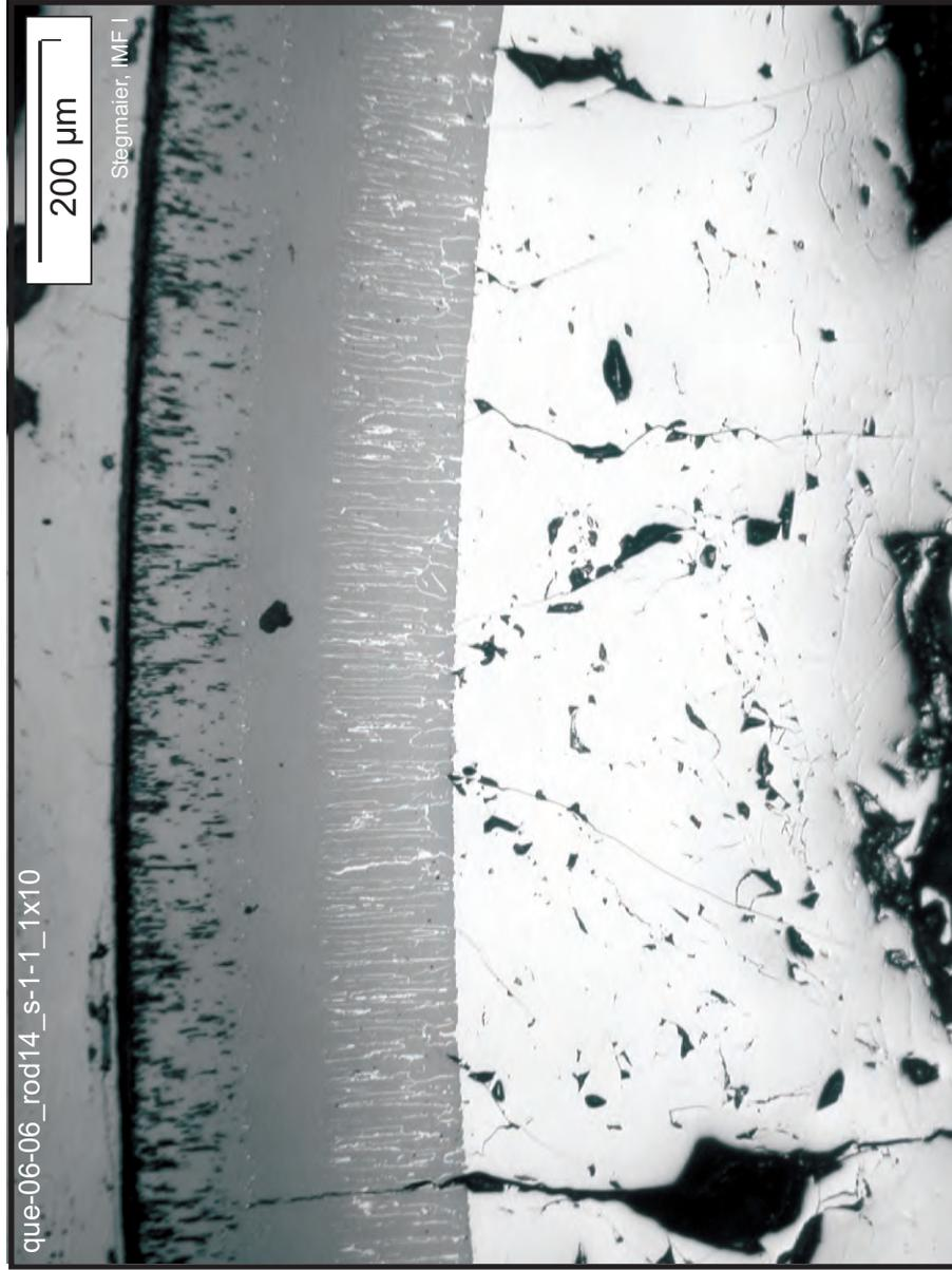
Fig. 55: Cross section at 850 mm bundle elevation (QUE-06-6); rod No. 14, showing a melt bridge from thermocouple to cladding, wetting of the duplex scale, and the partially molten cladding matrix
