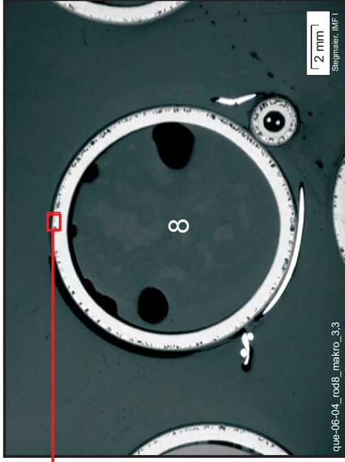
Rod No. 8, together with attached thermocouple
