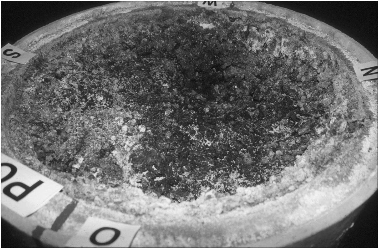
Figure 4-19 CometPC-H5: Top view of solidified melt with porous surface
