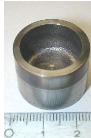
Fig. 5-24: The cup-shaped multi-layer W-V-ferritic steel sample.
