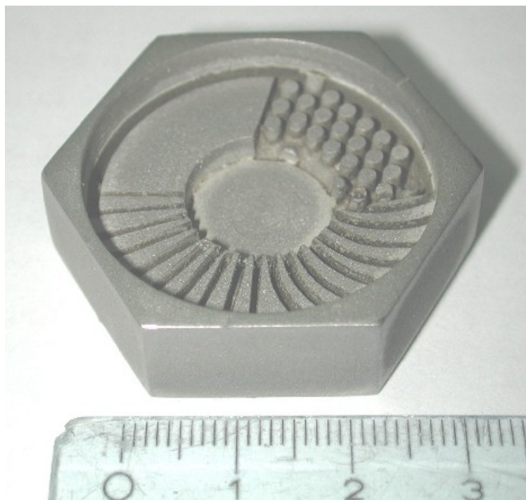
Fig. 5-5: Tungsten sample with different cooling shapes produced by EDM.
