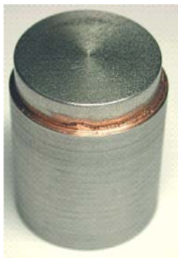
Fig. 5-36: Mo thimble joined through copper layer (option I-A).
