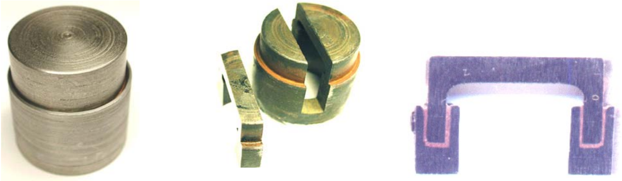
Fig. 5-37: W thimble joined through copper layer (option I-B).
