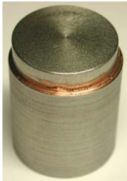
Fig. 5-31: Scheme of joining and general view of technological sample (option I).
