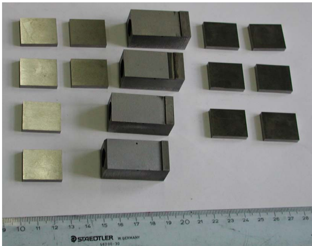
Fig. 5-30: Mock-up parts for development of the W/W joint (water-cooled heat sink from TZM and W tiles from sintered rolled tungsten).
