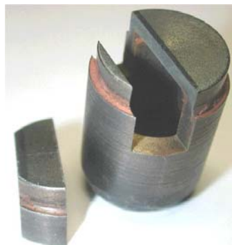
Fig. 5-36: Mo thimble joined through copper layer (option I-A).
