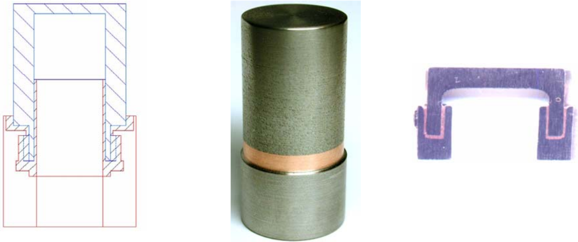
Fig. 5-20: Joining of refractory alloy (top part) to steel (bottom part) by Cu brazing and mechanical interlock.
