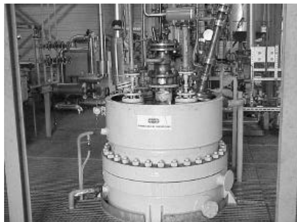
Fig. 15: Top of the 5+ MW(th) pilot scale pressurised entrained flow gasifier at Babcock Borsig Power (BBP), Freiberg, Saxony.
