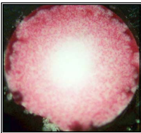
Figure 4-2: Loading profile resin A365, c(\text{NiCl}_2)=5\text{mmol/L} , d_p=580\ \mu\text{m} , t=30\ \text{min} , light microscope
