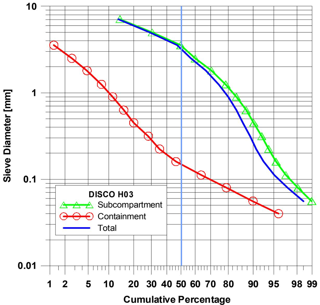
Fig. 70. Cumulative particle size distribution of debris in H03
