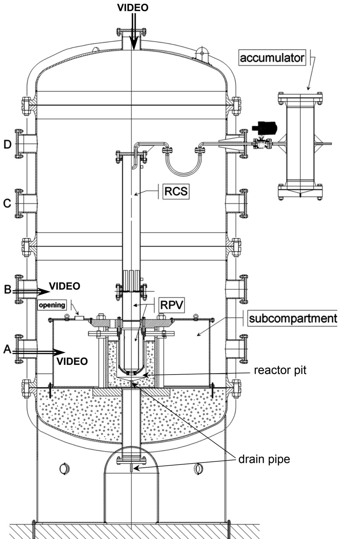
Fig. 2. The Containment pressure vessel with internal structures
