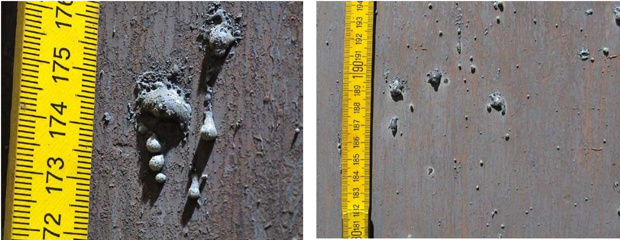
Fig. 56. Melt particles at containment wall
