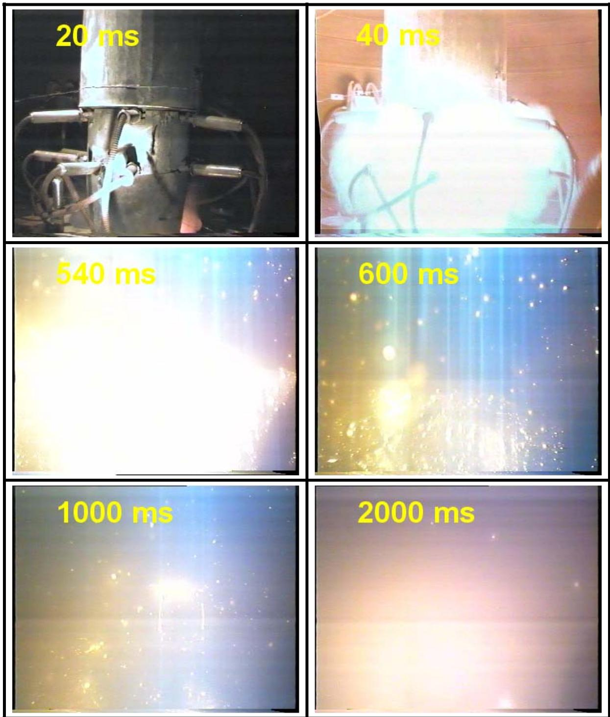
Fig. 48. Video pictures from containment near cavity exit from test H02
