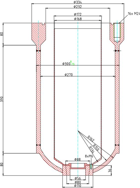
Fig. 12. Crucible with reduced diameter of BT2
