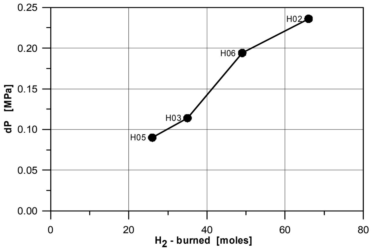
Fig. 46. Burned hydrogen versus pressure rise in the containment
