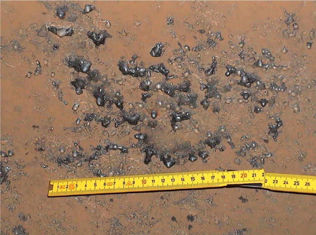
**Fig. 60. Close up of melt debris at containment top head, test H04**
