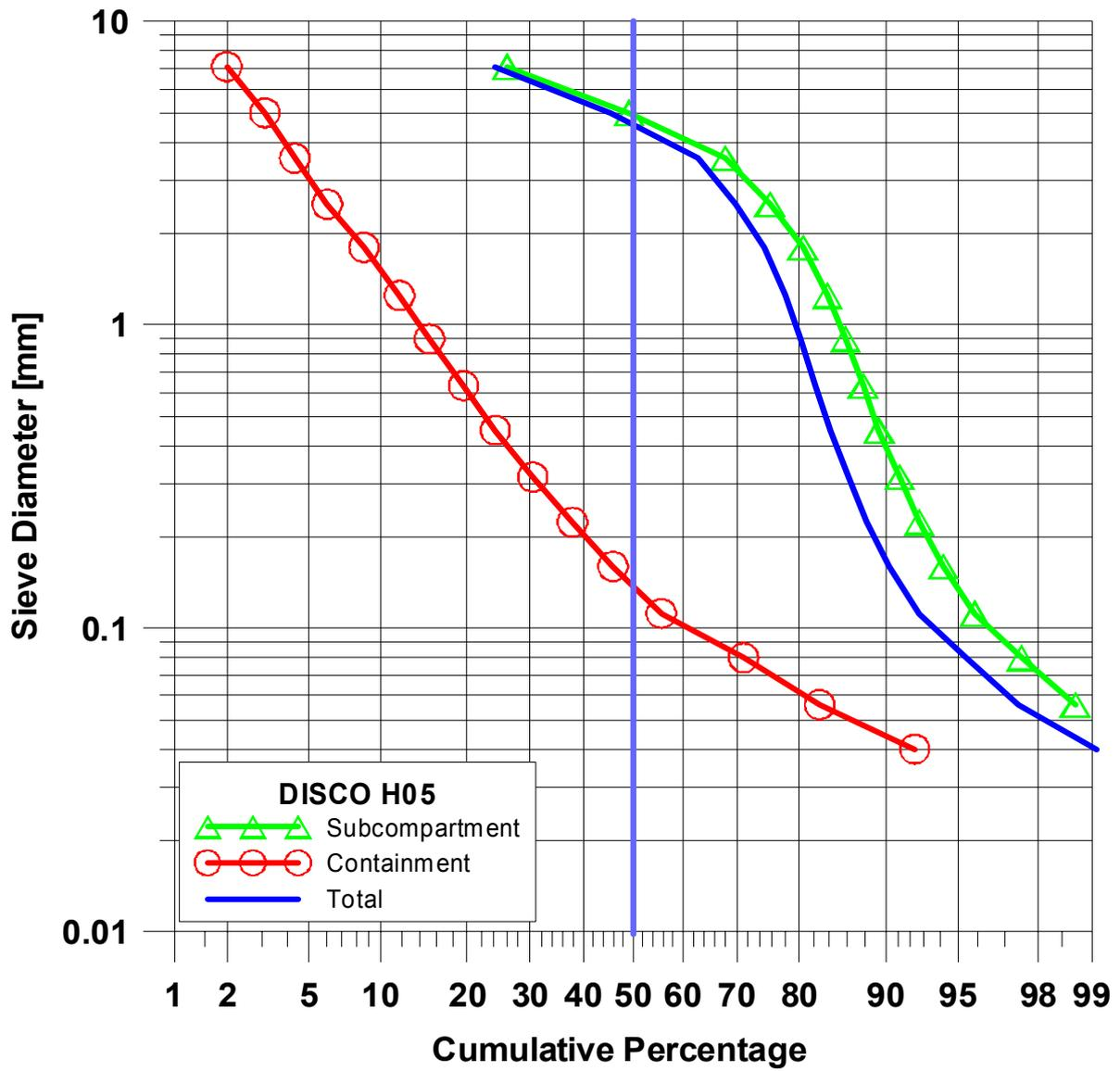
Fig. 72. Cumulative particle size distribution of debris in H05
