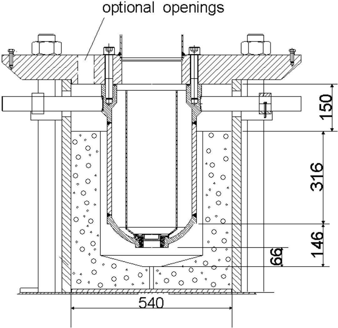
Fig. 8. The RPV-model (crucible) and cavity
