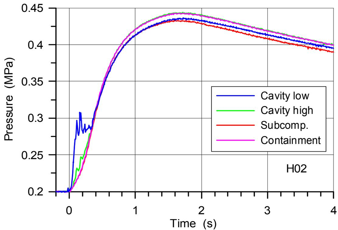
Fig. 32. Pressure in the cavity, subcompartment and containment in H02
