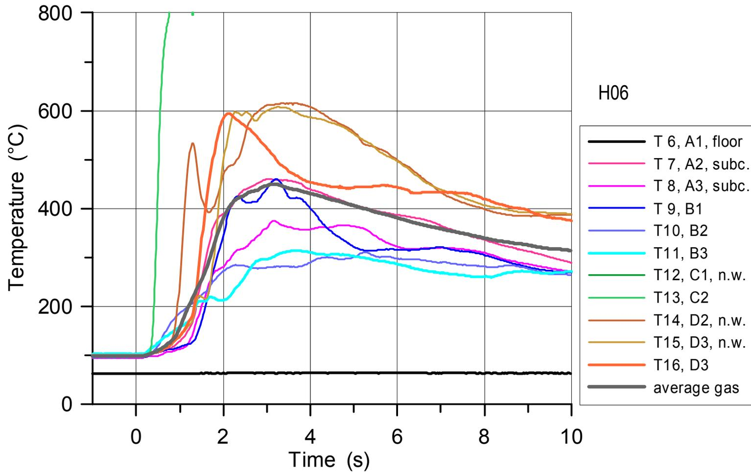
Fig. 45. Gas temperatures in the subcompartment and containment in H06
