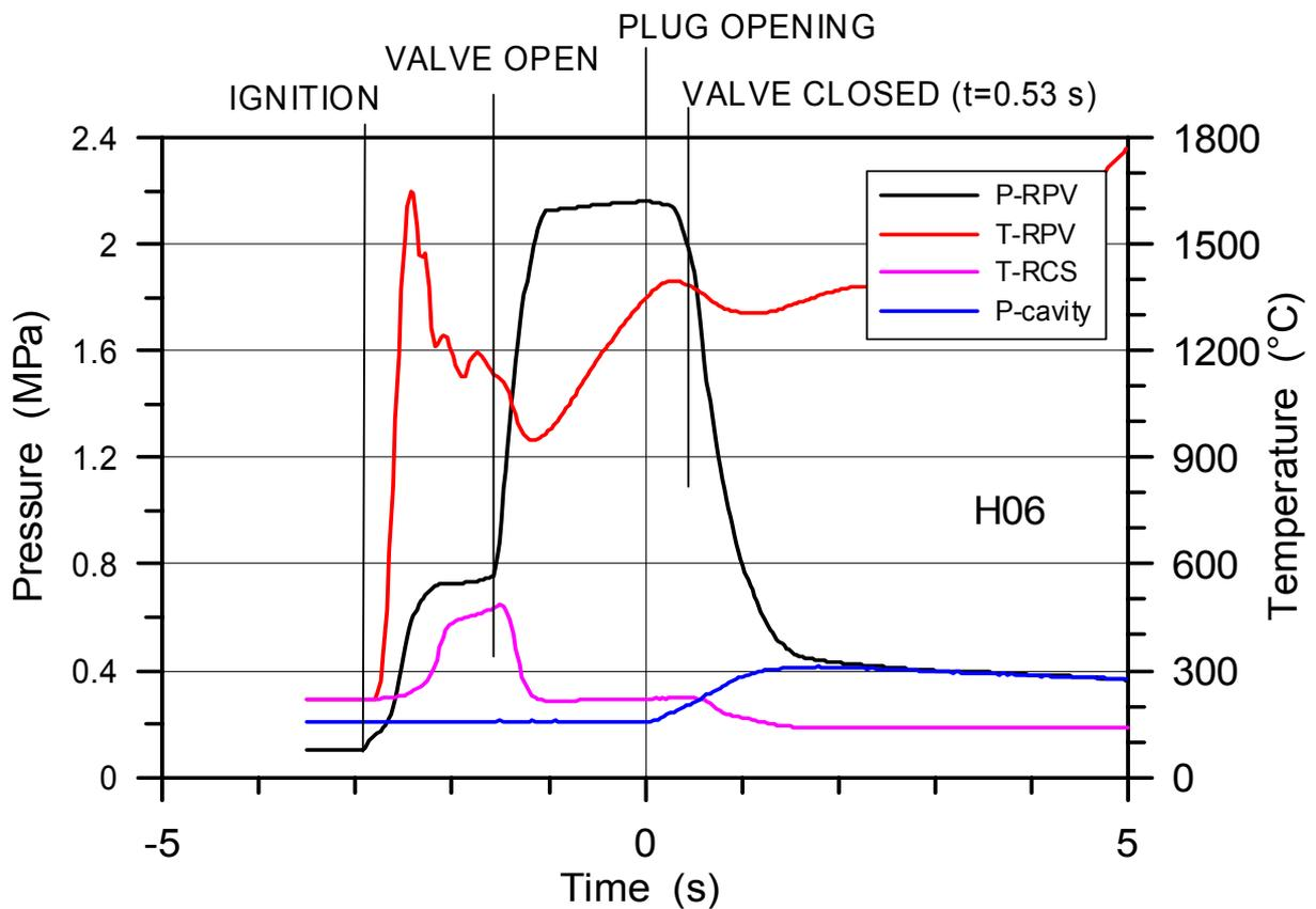
Fig. 23. Pressure, temperature and timing in H06
