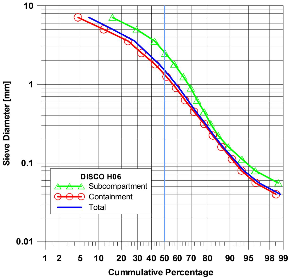
Fig. 73. Cumulative particle size distribution of debris in H06
