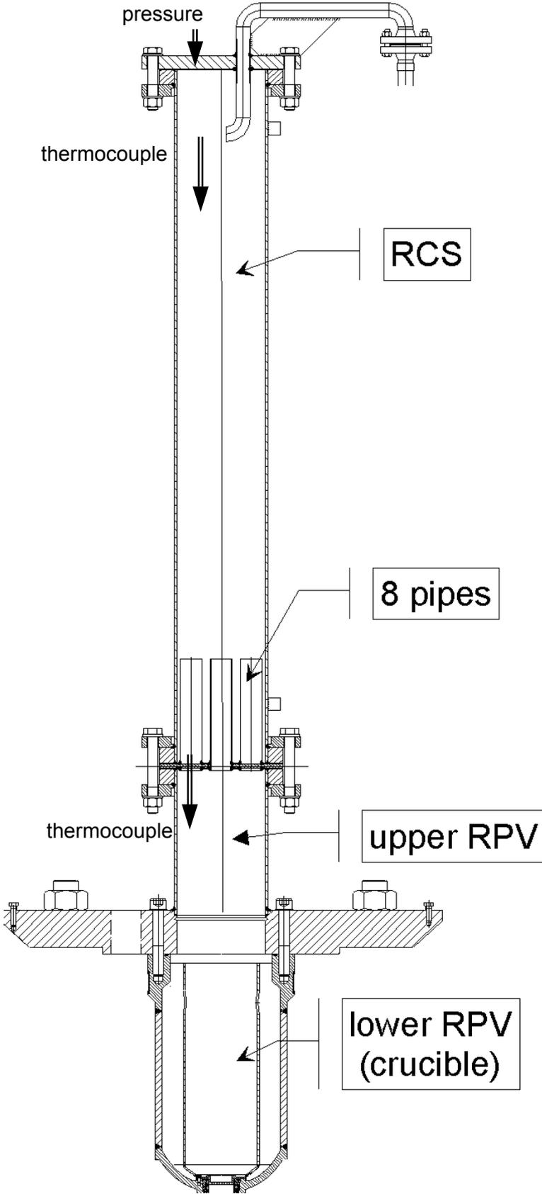
Fig. 5. The model of the RCS vessel and RPV
