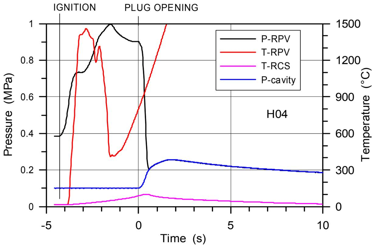
Fig. 21. Pressure, temperature and timing in H04 (no steam)
