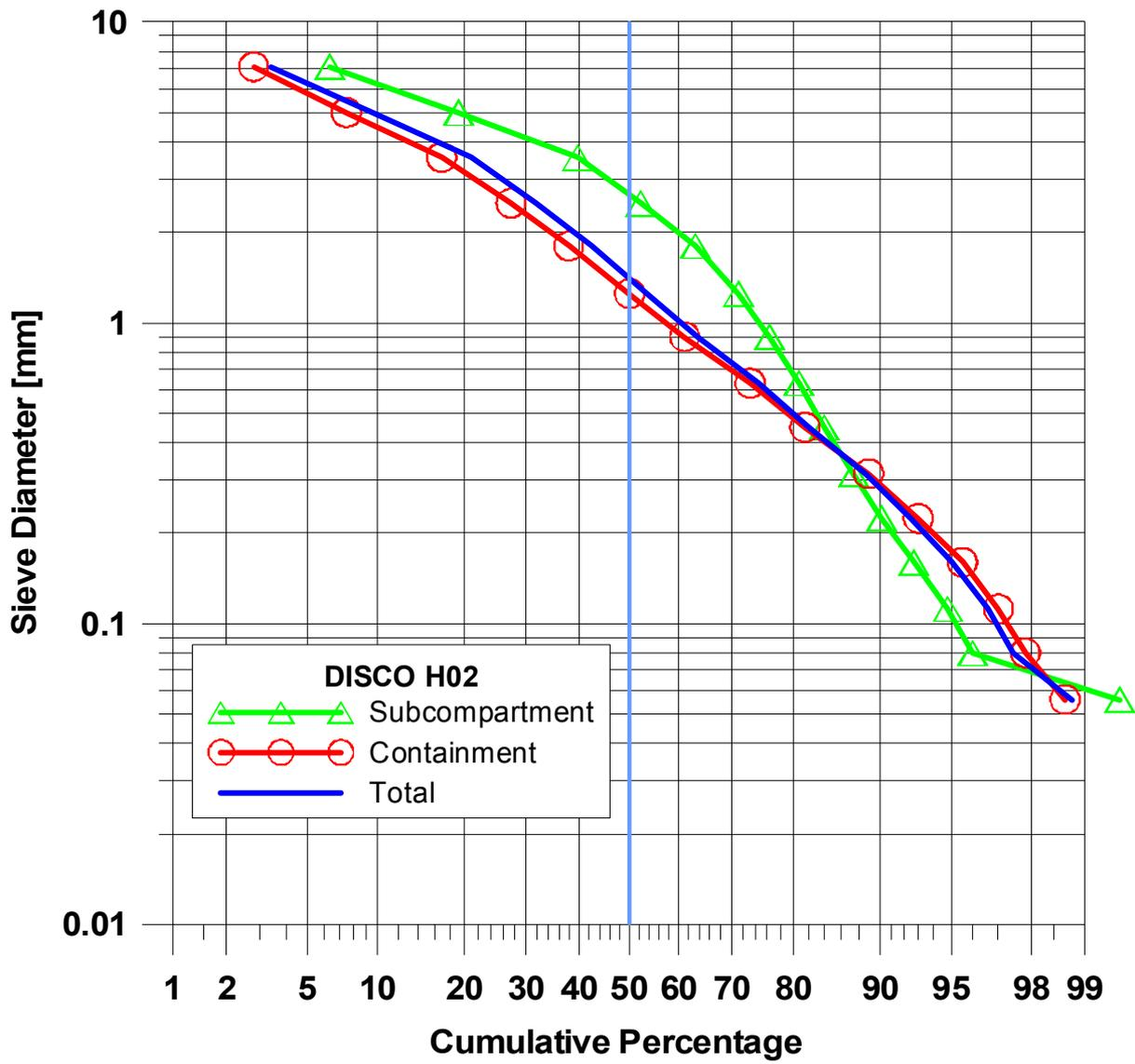
Fig. 69. Cumulative particle size distribution of debris in H02
