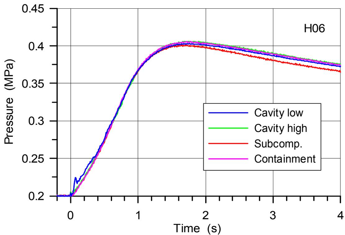
Fig. 36. Pressure in the cavity, subcompartment and containment in H06
