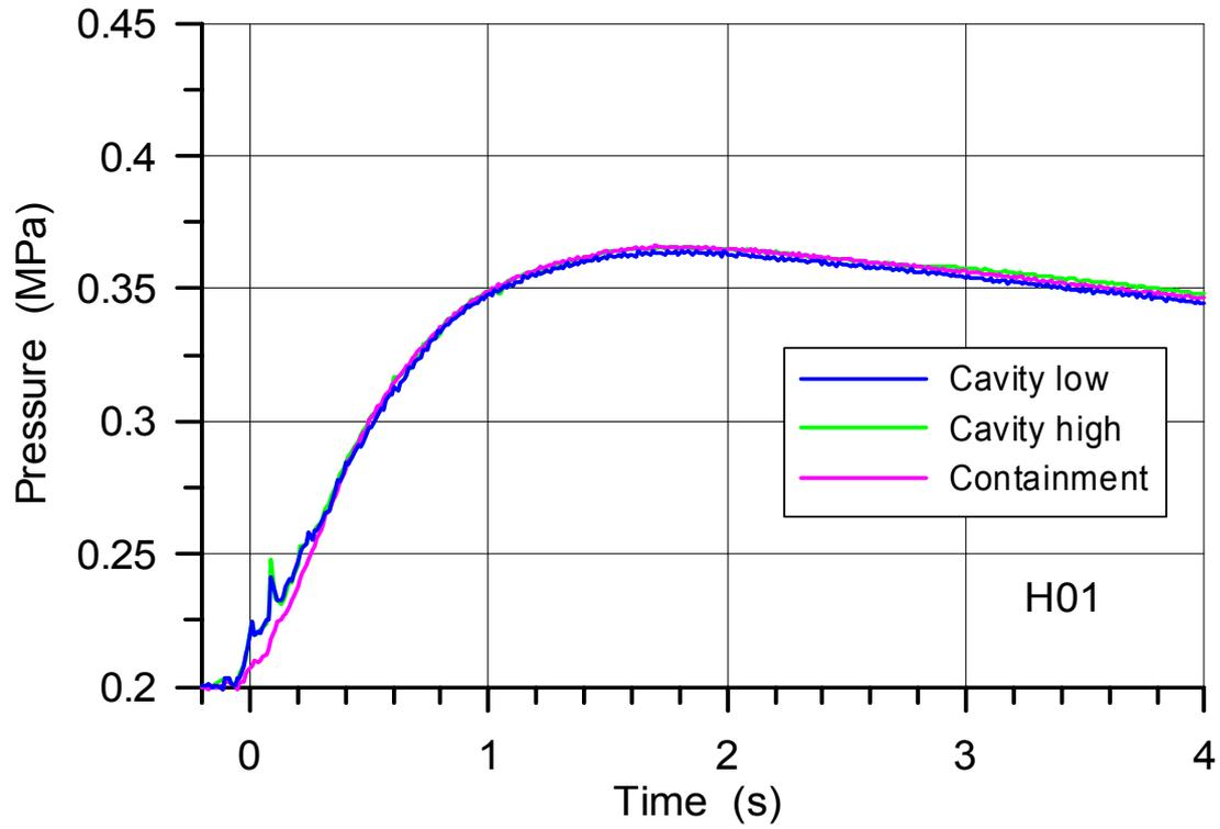
Fig. 31. Pressure in the cavity and containment in H01
