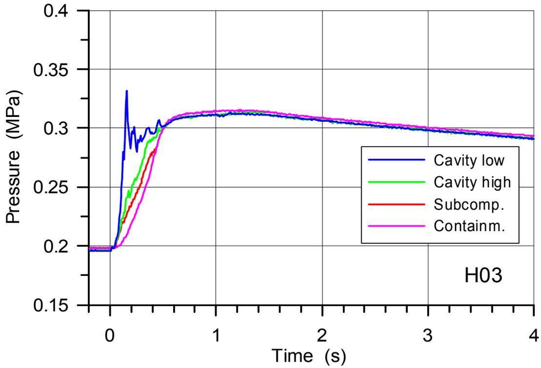
Fig. 33. Pressure in the cavity, subcompartment and containment in H03
