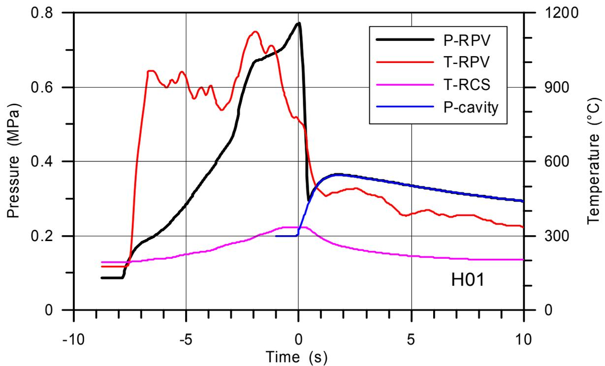
Fig. 18. Pressure and temperature in the RPV/RCS-vessel and the cavity in test H01
