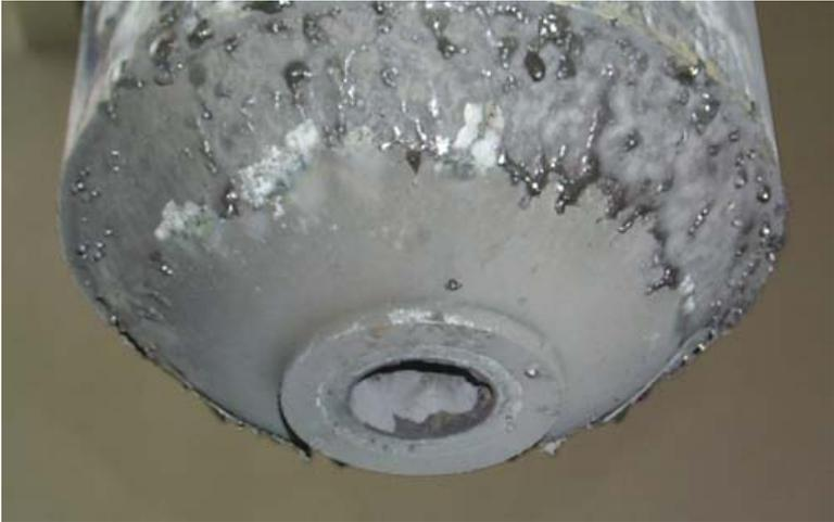
Fig. 54. Post test view of RPV lower head and hole
