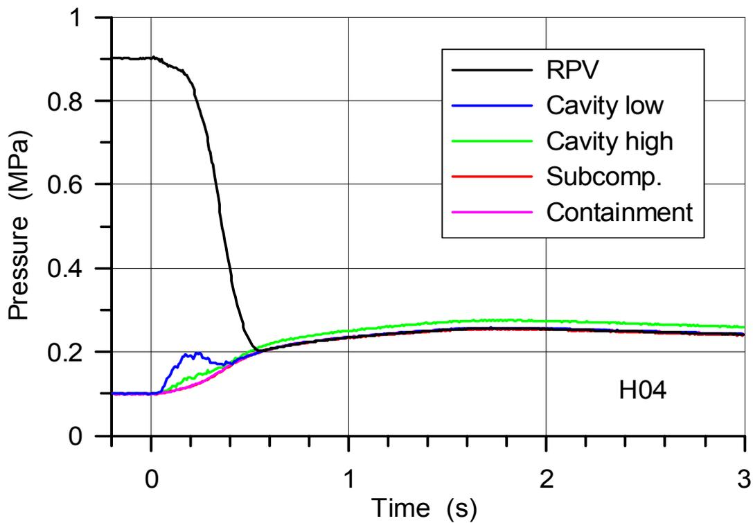
Fig. 27. Pressure in the RPV, cavity and containment in H04 (-0.2 to 3 s)
