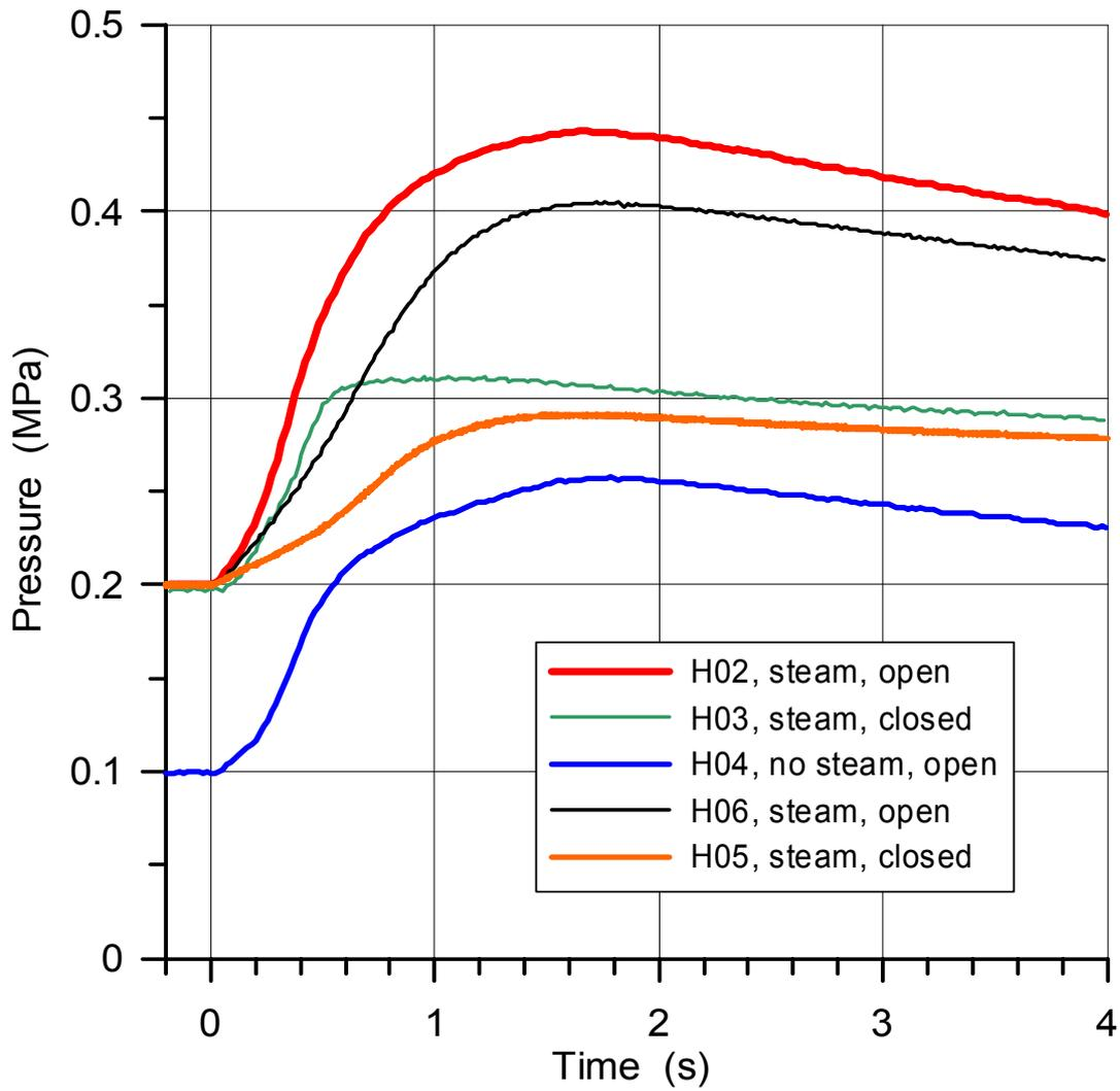
**Fig. 37. Comparison of pressure rise in the containment**
