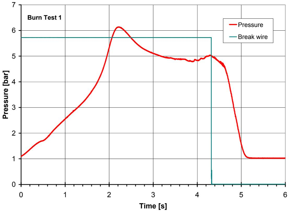
Fig. 13. Pressure in the RPV-RCS vessel during burn test BT1
