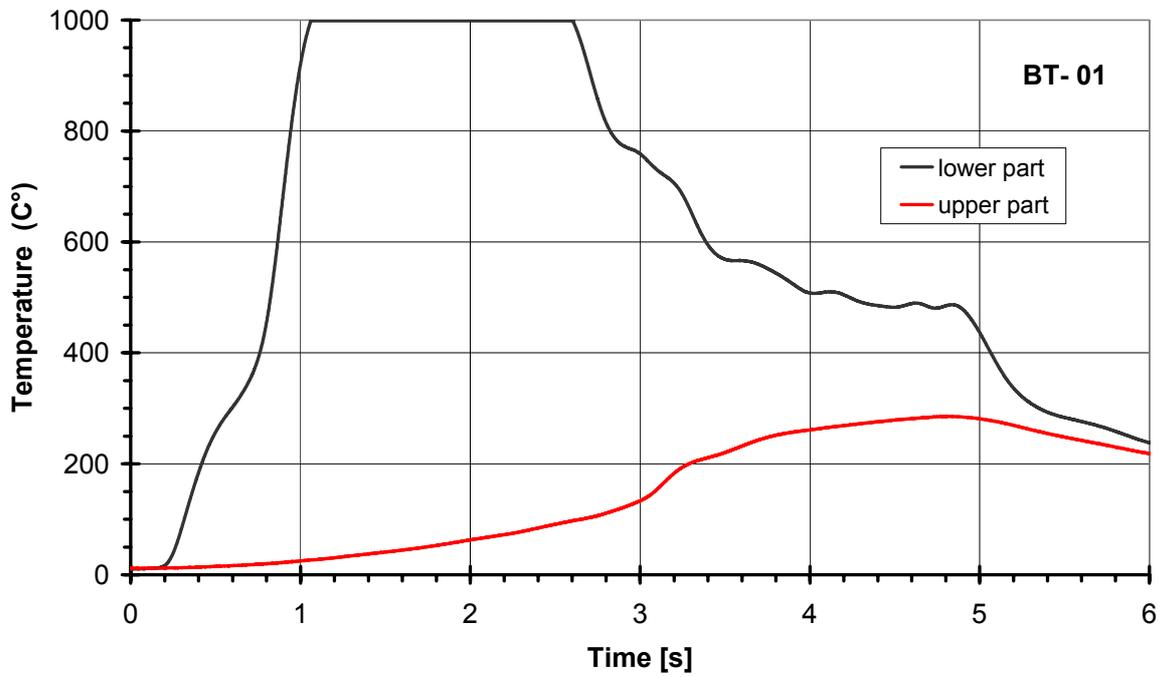
Fig. 14. Temperatures in the RPV-RCS vessel during burn test BT1
