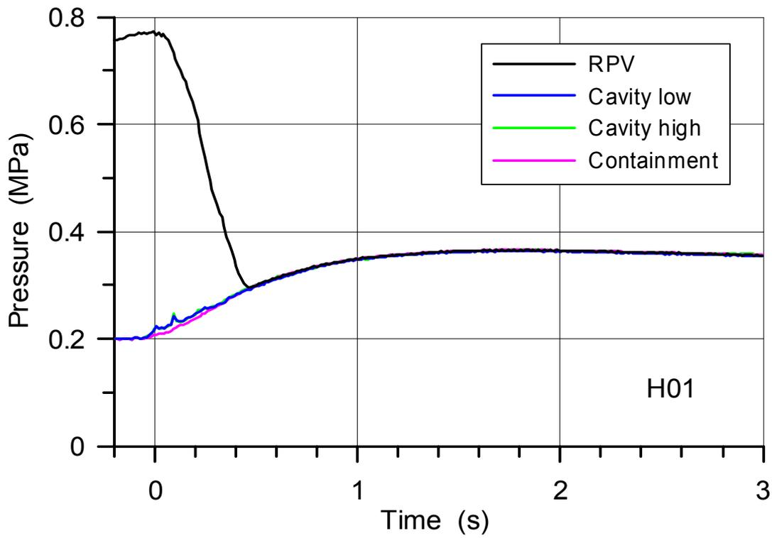
Fig. 24. Pressure in the RPV, cavity and containment in H01 (-0.2 to 3 s)
