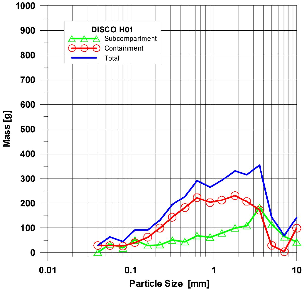
Fig. 62. Particle size distribution of debris in H01
