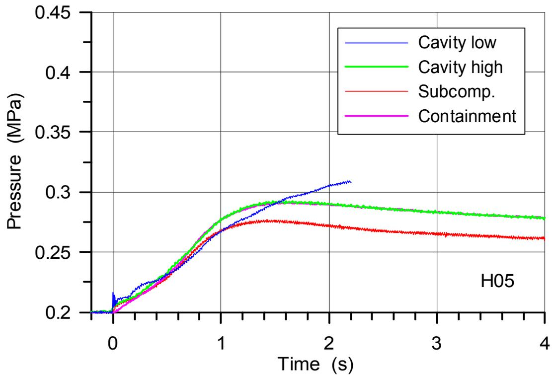
Fig. 35. Pressure in the cavity, subcompartment and containment in H05
