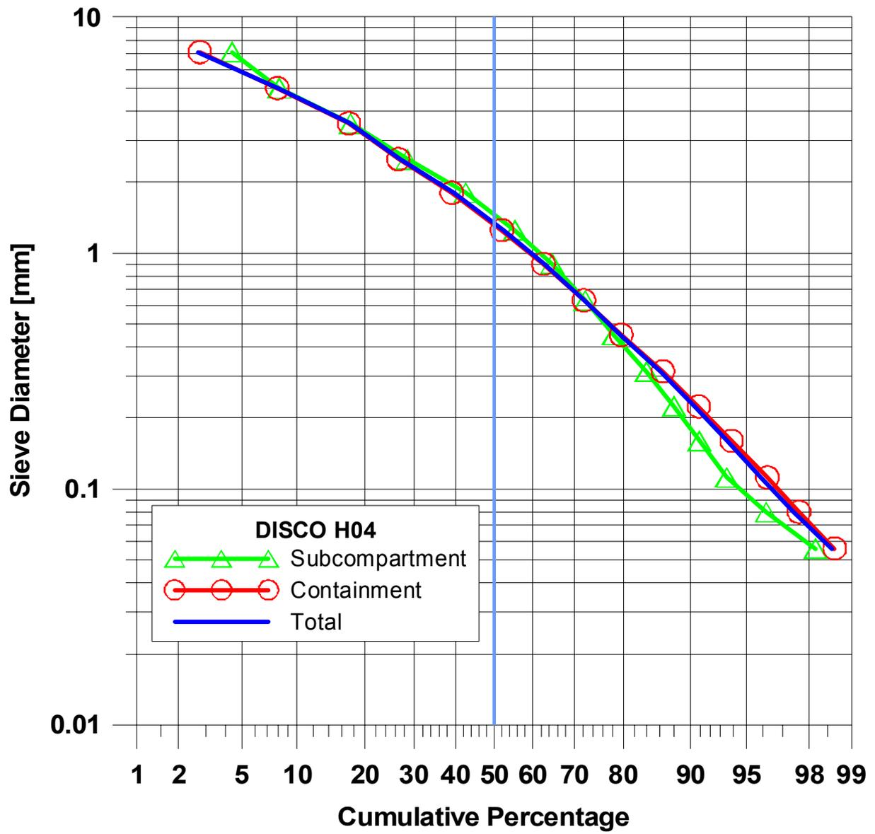
Fig. 71. Cumulative particle size distribution of debris in H04
