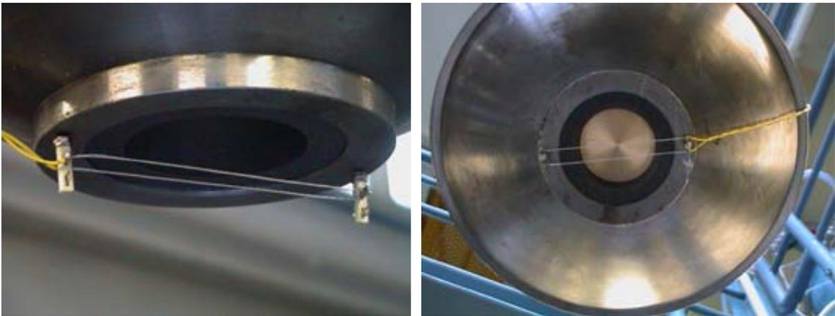
Fig. 9. Breakwires at the RPV exit hole
