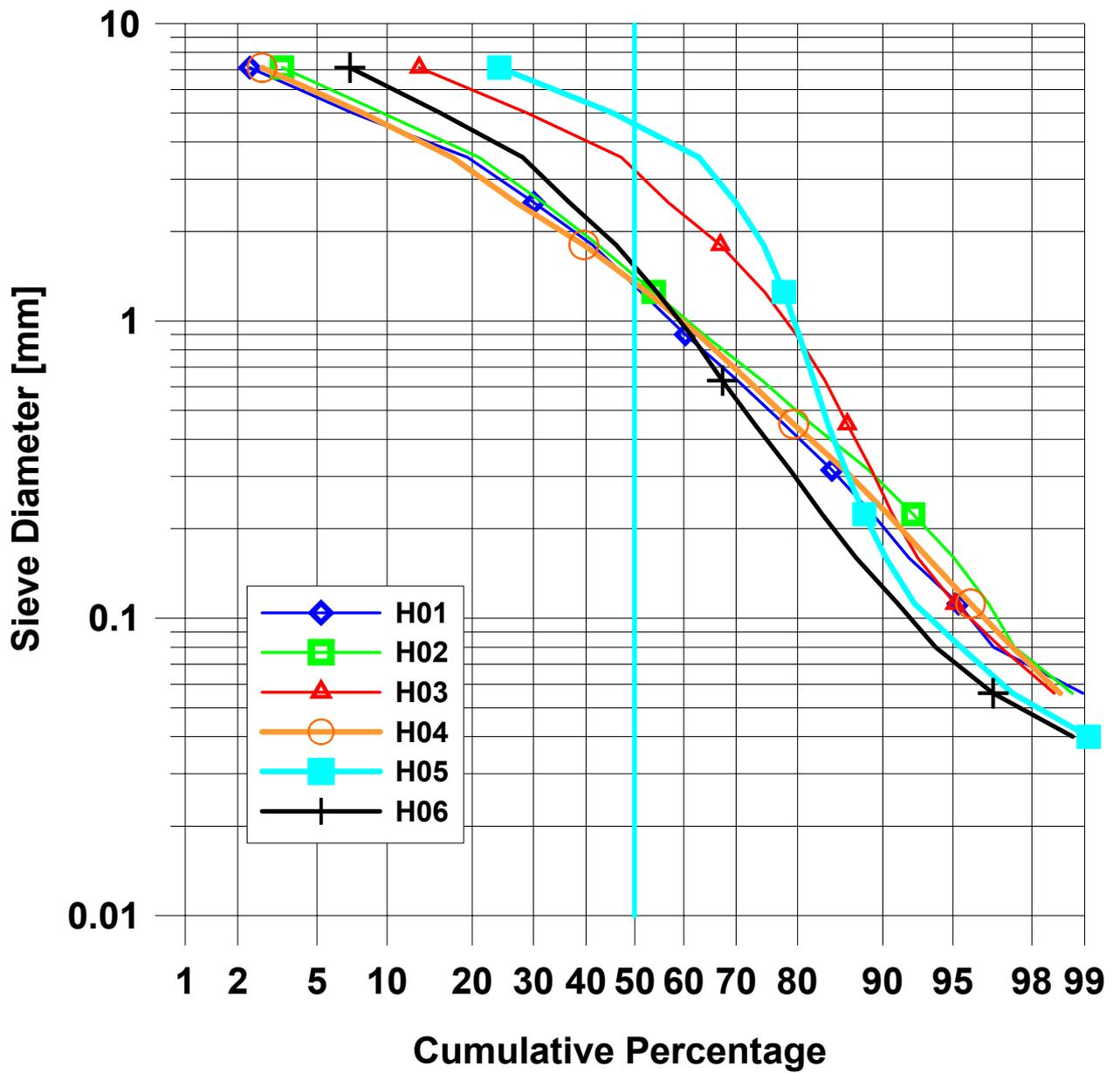
Fig. 74. Comparison of cumulative particle size distribution of debris
