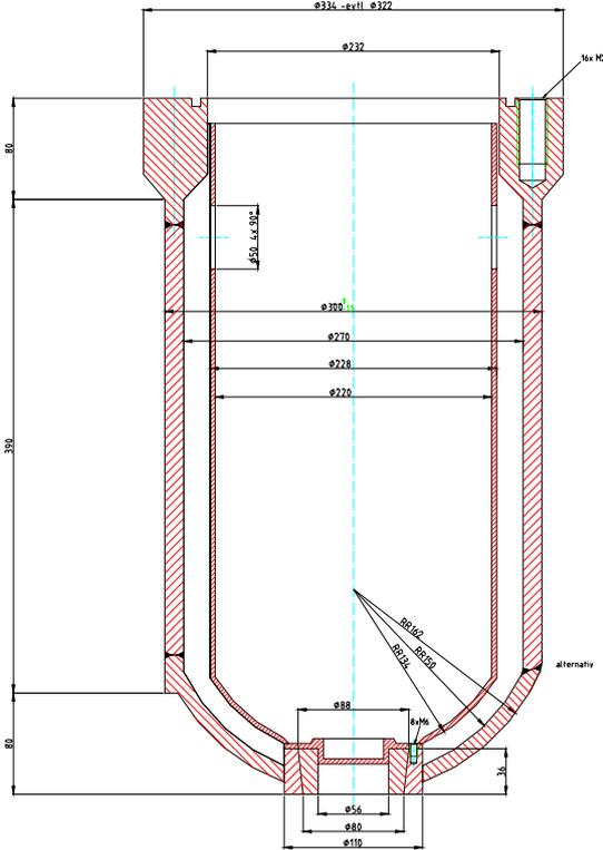
Fig. 11. Crucible of burn test BT1
