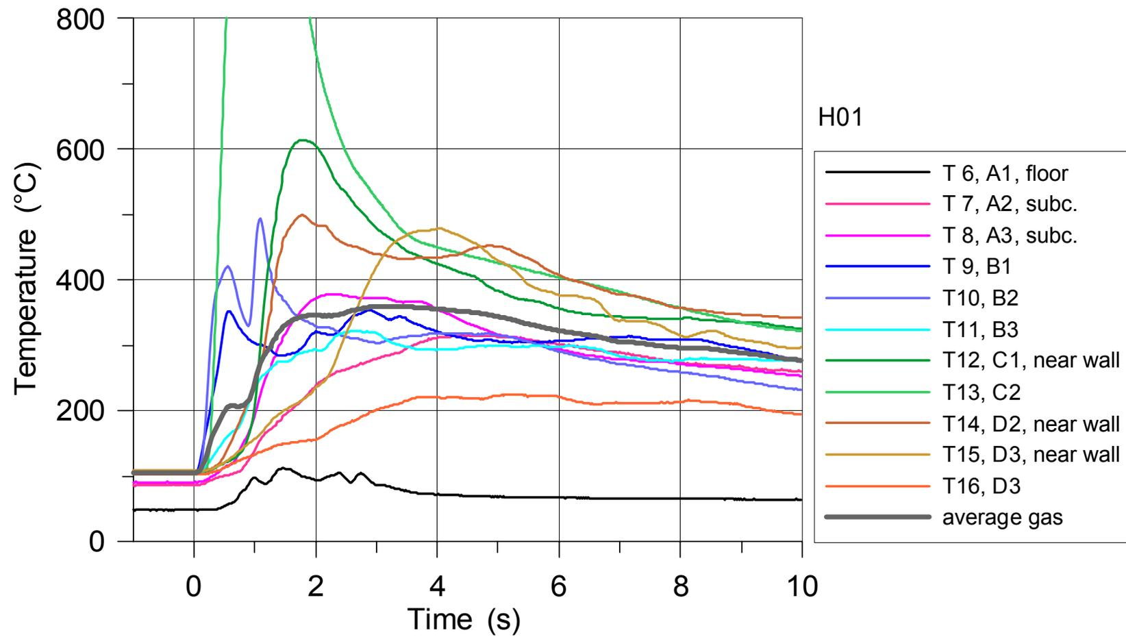
Fig. 40. Gas temperatures in the subcompartment and containment in H01
