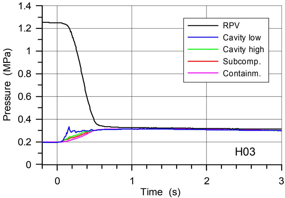
Fig. 26. Pressure in the RPV, cavity and containment in H03 (-0.2 to 3 s)
