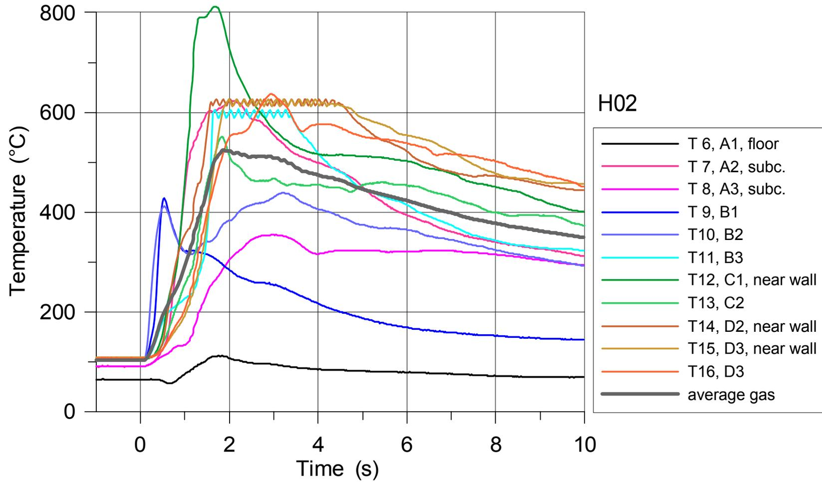
Fig. 41. Gas temperatures in the subcompartment and containment in H02
