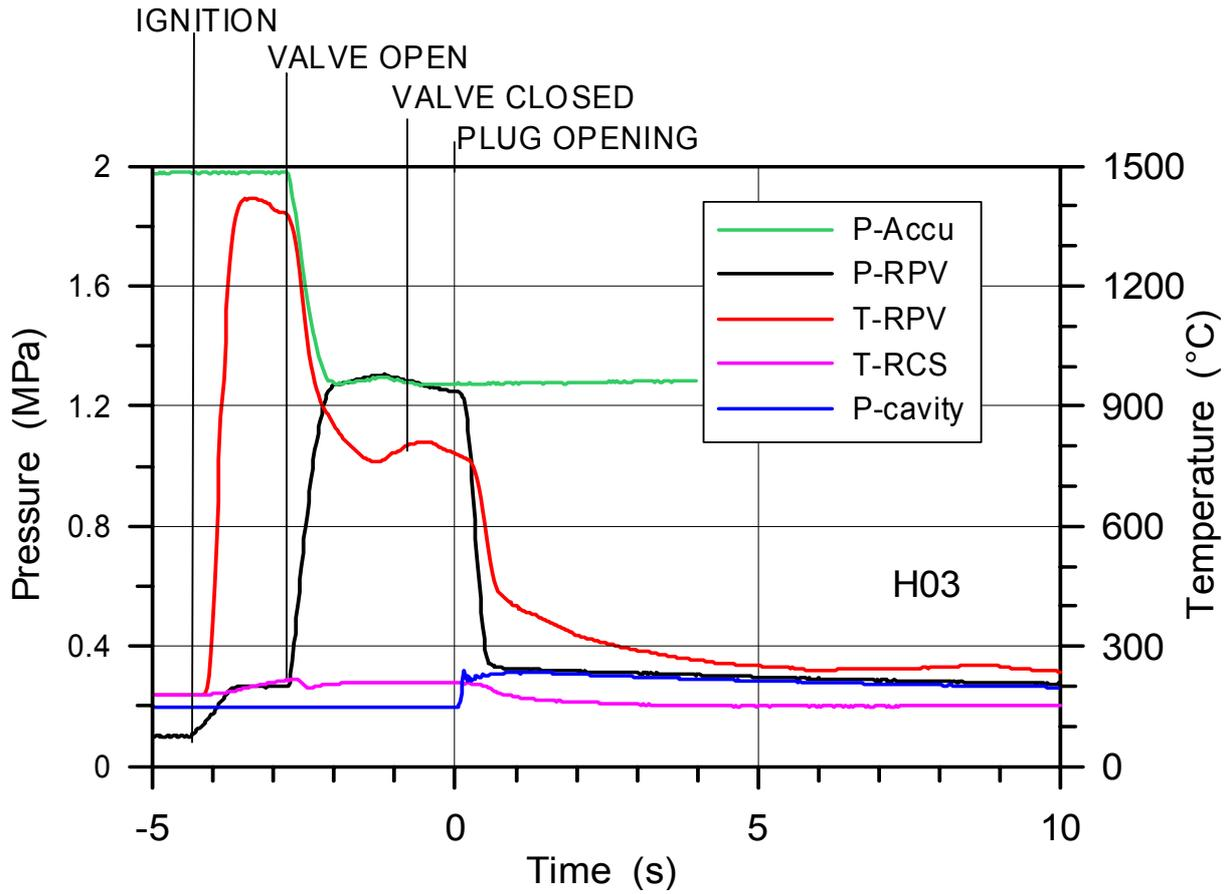
Fig. 20. Pressure, temperature and timing in H03
