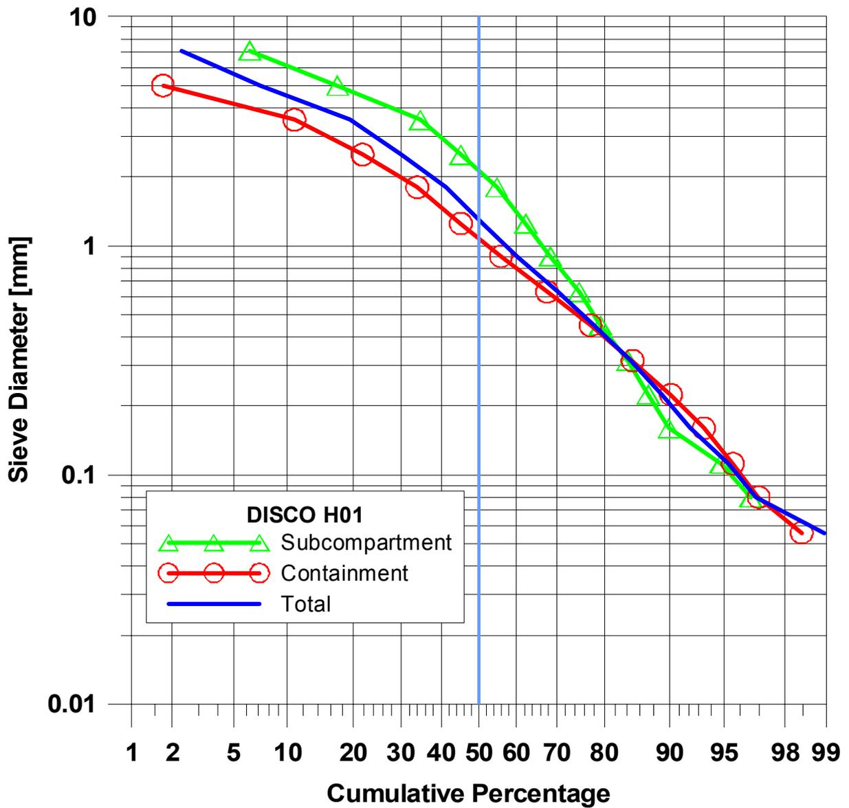
Fig. 68. Cumulative particle size distribution of debris in H01
