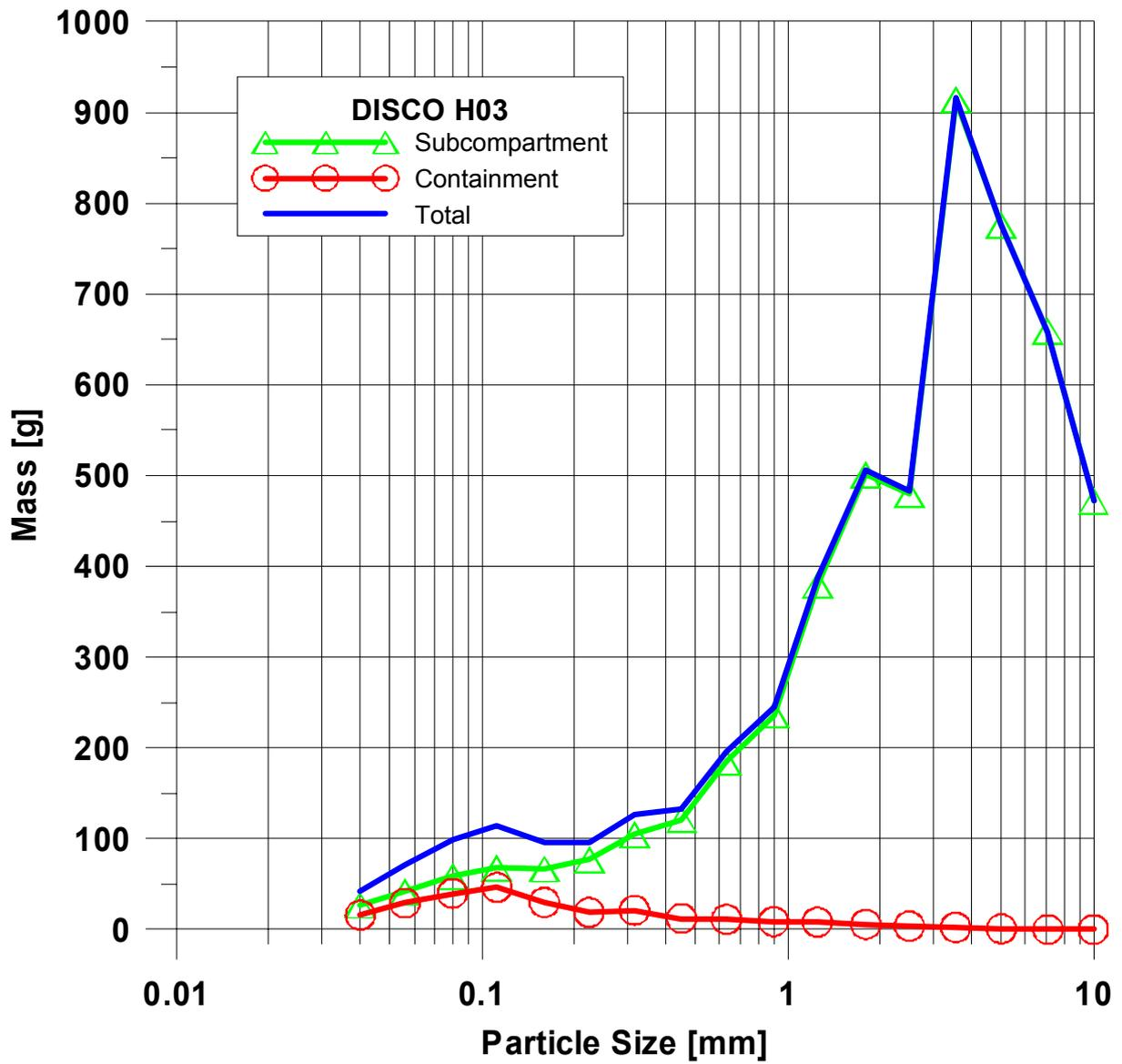
Fig. 64. Particle size distribution of debris in H03
