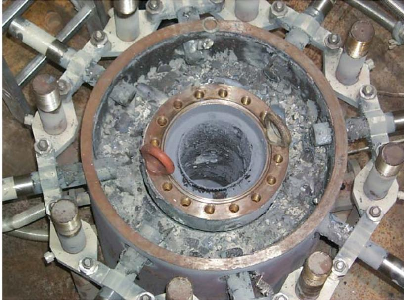
**Fig. 52. Post test view of concrete cavity and RPV/crucible**
