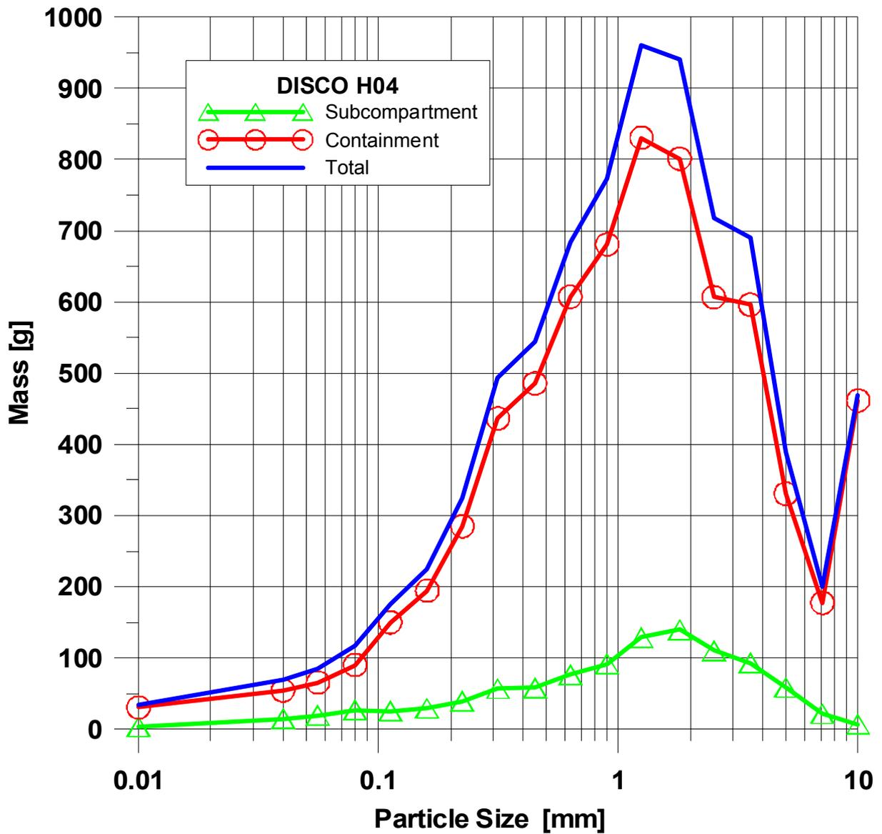
Fig. 65. Particle size distribution of debris in H04
