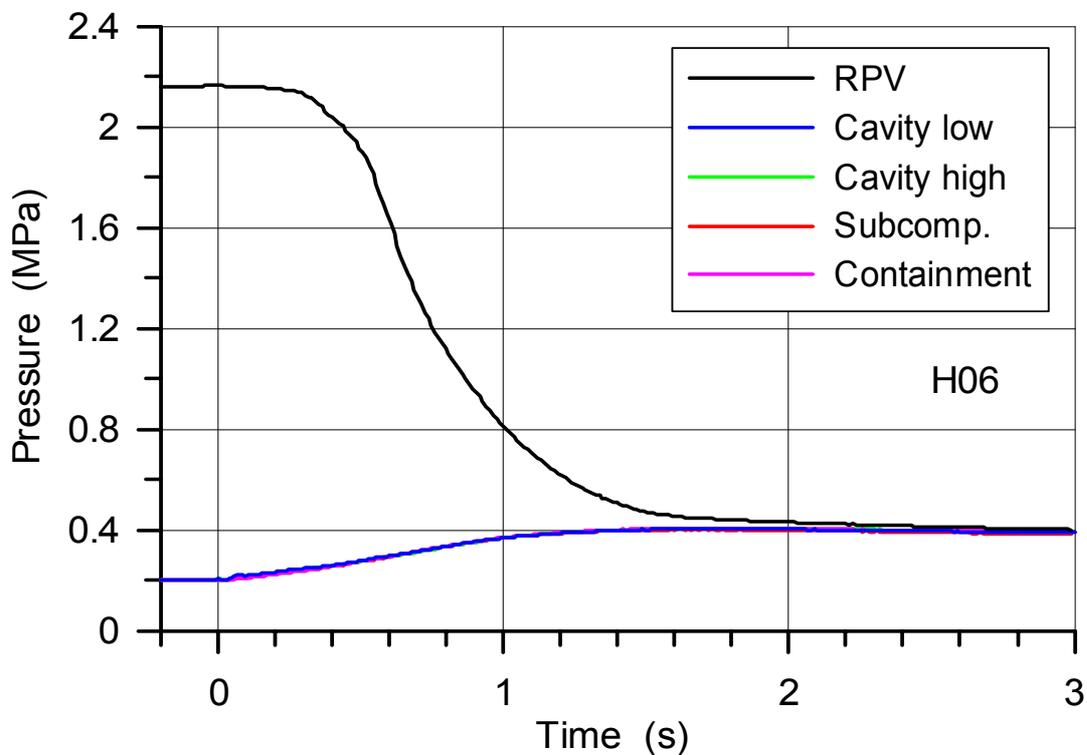
Fig. 29. Pressure in the RPV, cavity and containment in H06 (-0.2 to 3 s)
