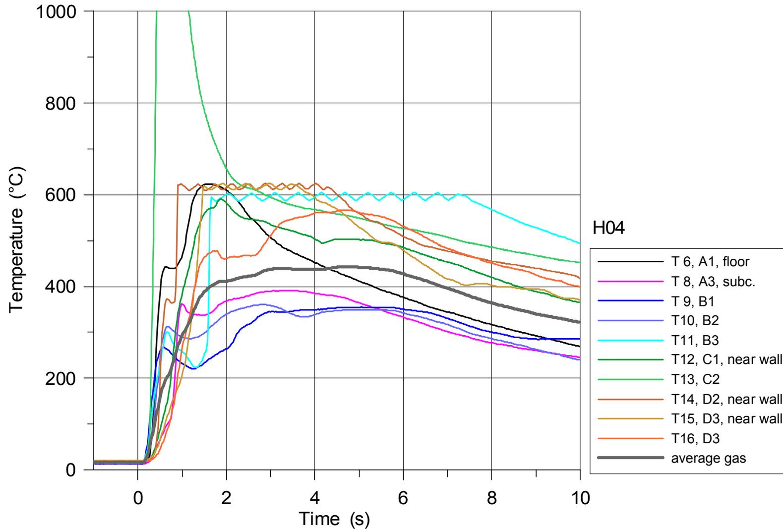
Fig. 43. Gas temperatures in the subcompartment and containment in H04
