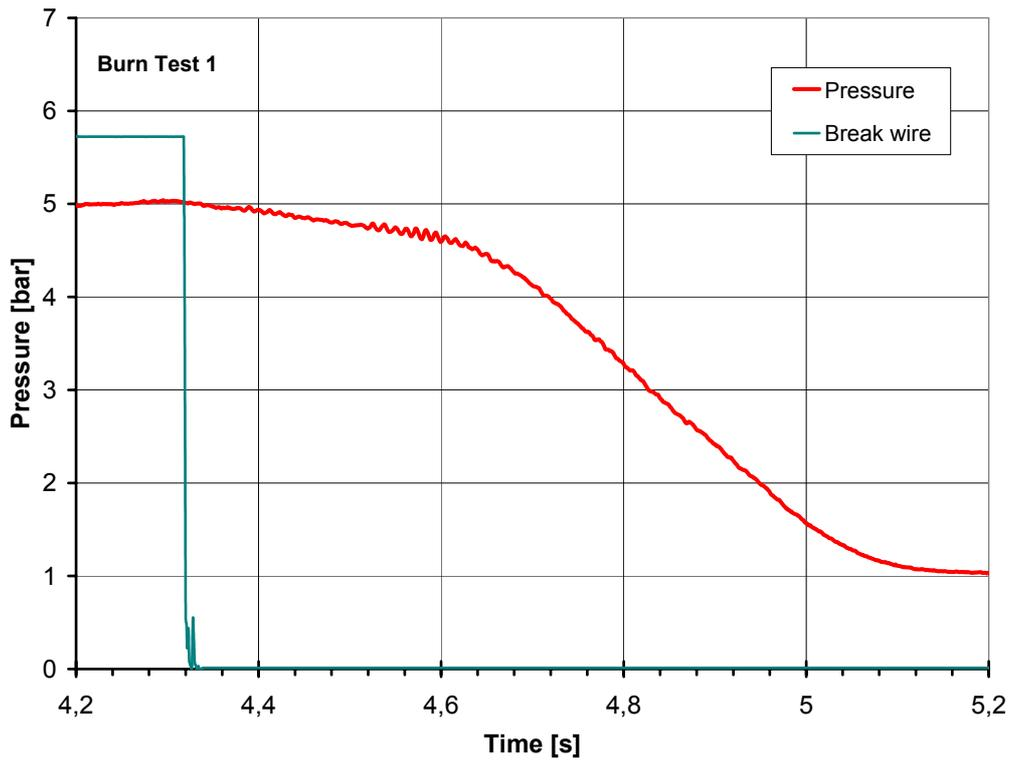
Fig. 15. Blow-down pressure in the RPV-RCS vessel during burn test BT1
