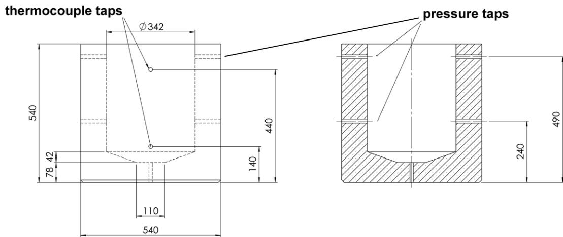
Fig. 7. The reactor pit made of concrete
