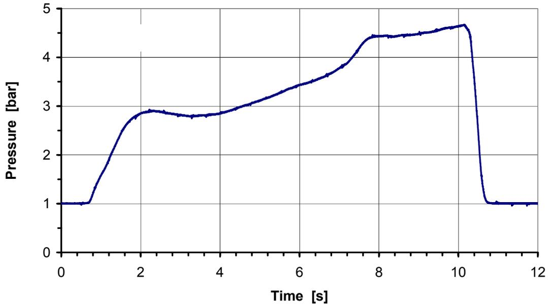
Fig. 16. Pressure in the RPV-RCS vessel during burn test BT2
