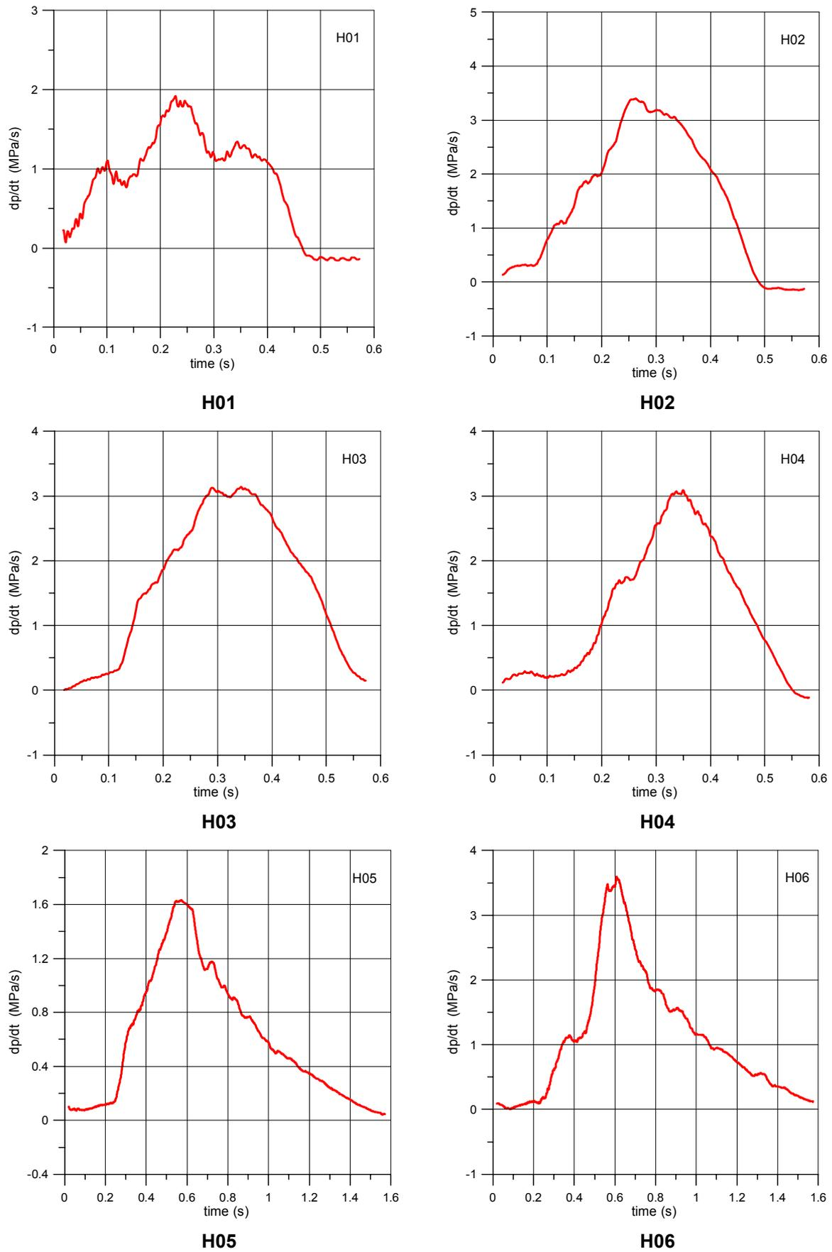
Fig. 30. Pressure gradient in RPV vessel
