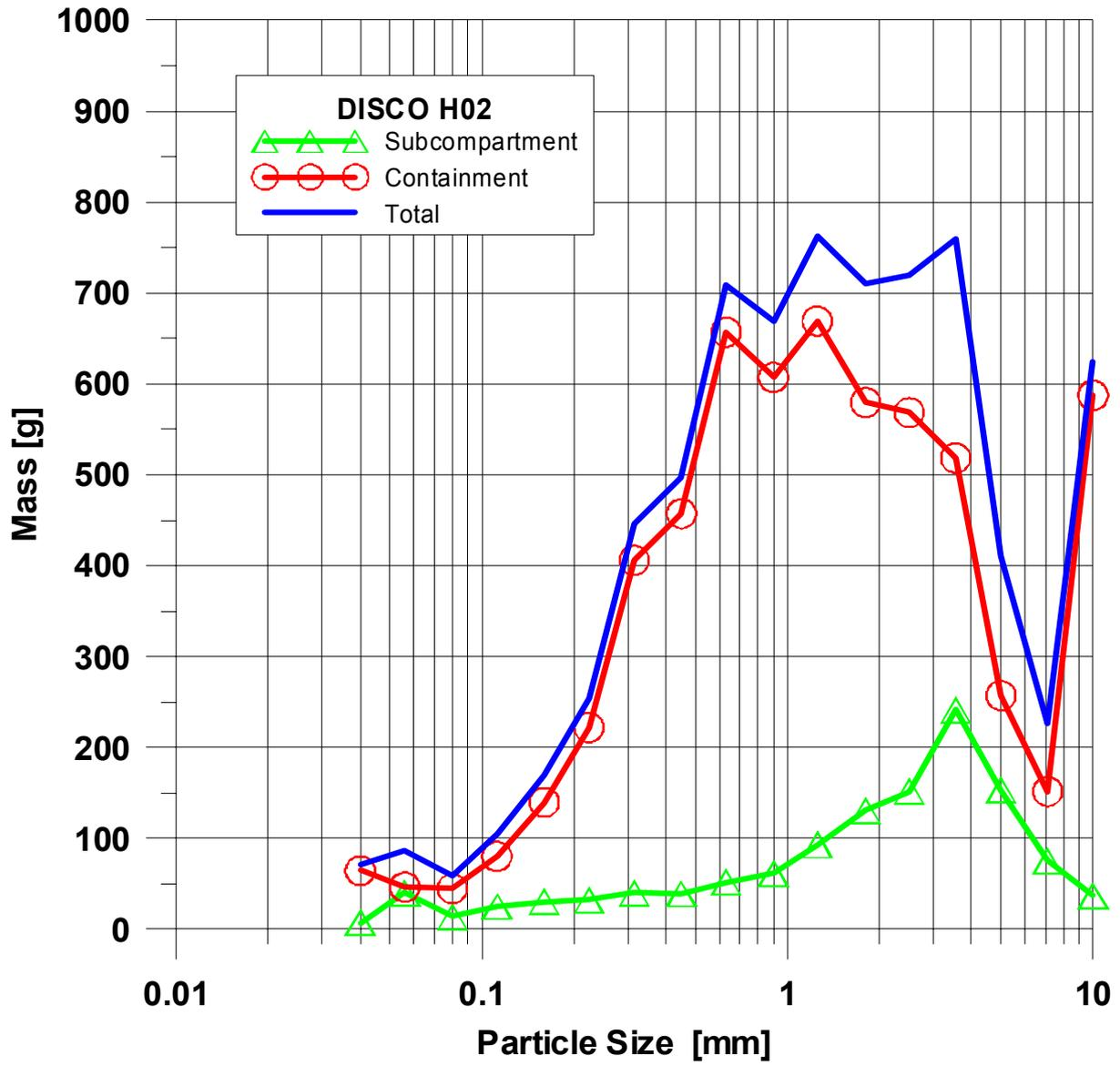
Fig. 63. Particle size distribution of debris in H02
