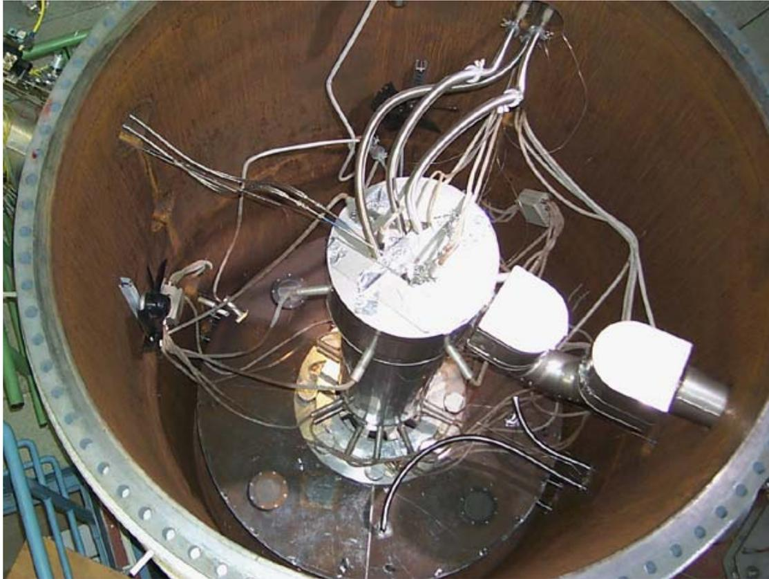
**Fig. 3. View into Containment pressure vessel, with RCS-RPV pressure vessel**
