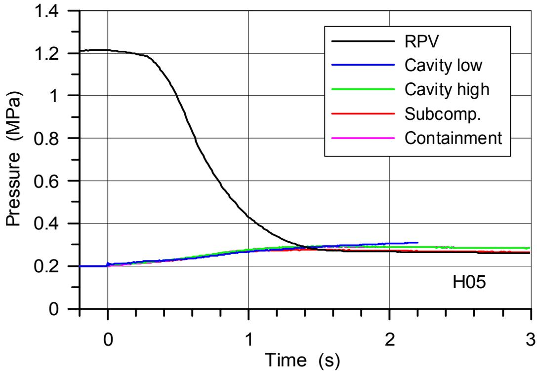
Fig. 28. Pressure in the RPV, cavity and containment in H05 (-0.2 to 3 s)
