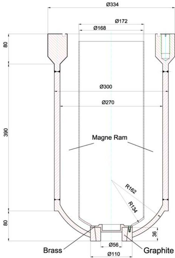
Fig. 6. The RPV model, crucible for the thermite melt
