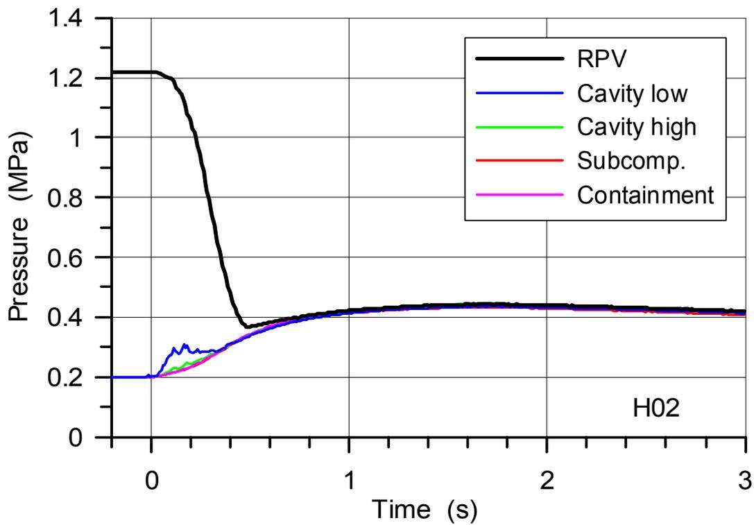
Fig. 25. Pressure in the RPV, cavity and containment in H02 (-0.2 to 3 s)
