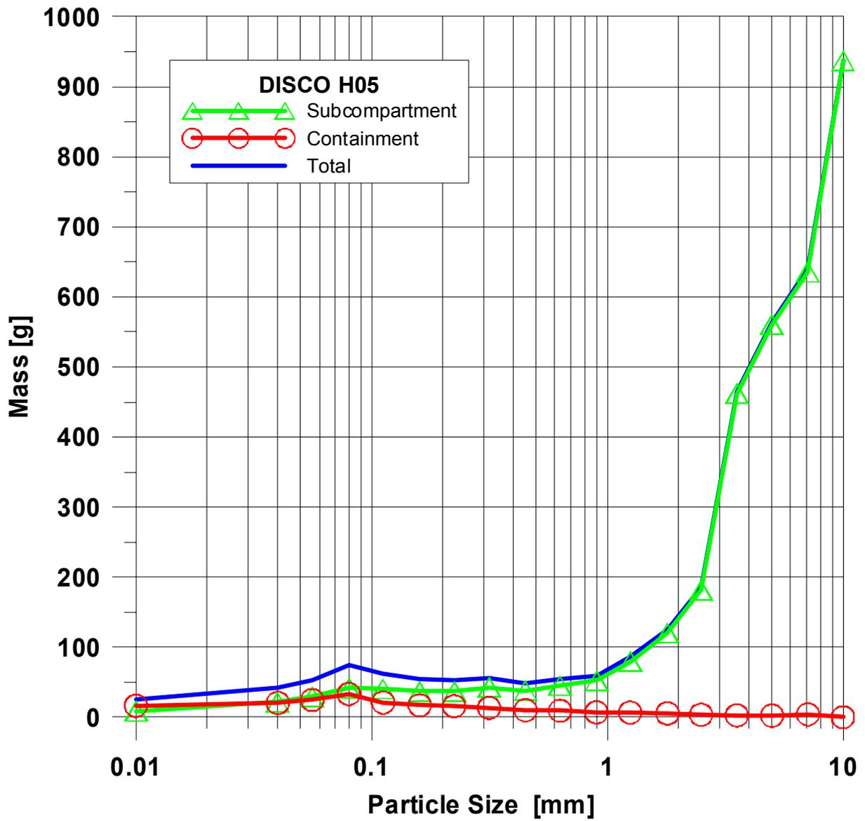
Fig. 66. Particle size distribution of debris in H05
