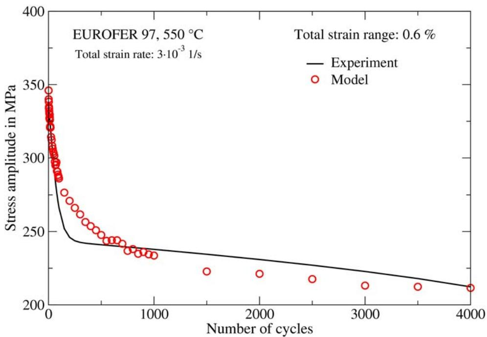
Fig. 4-26 Comparison between material (markers) and model (line) responses for the variation of stress amplitude versus the number of cycles of a strain controlled LCF test
