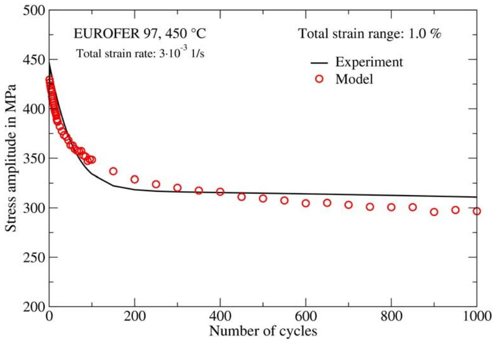
Fig. 4-20 Comparison between material (markers) and model (line) responses for the variation of stress amplitude versus the number of cycles of a strain controlled LCF test
