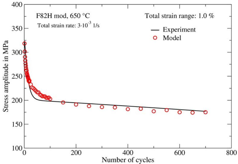
Fig. 4-15 Comparison between material (markers) and model (line) responses for the variation of stress amplitude versus the number of cycles of a strain controlled LCF test
