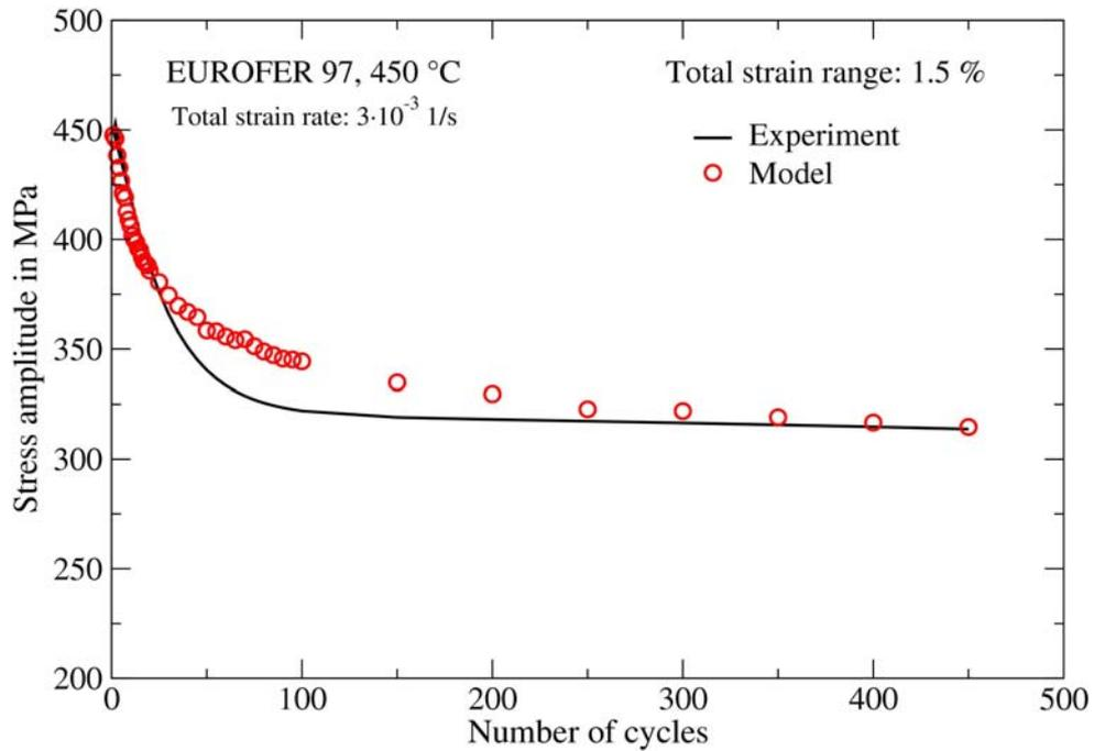
Fig. 4-19 Comparison between material (markers) and model (line) responses for the variation of stress amplitude versus the number of cycles of a strain controlled LCF test
