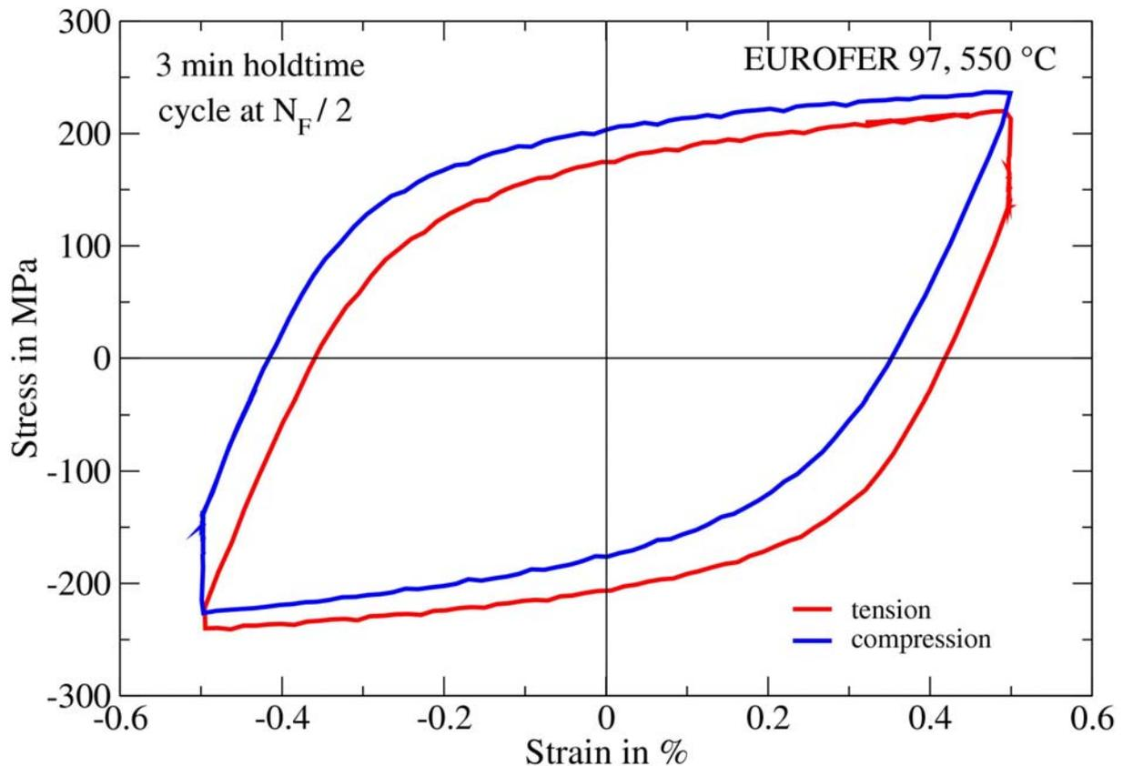
Fig. 2-5 Stress strain hysteresis loops at the half of the lifetime  $N_f / 2$  for the tests with hold time under tension and with hold time under compression, respectively
