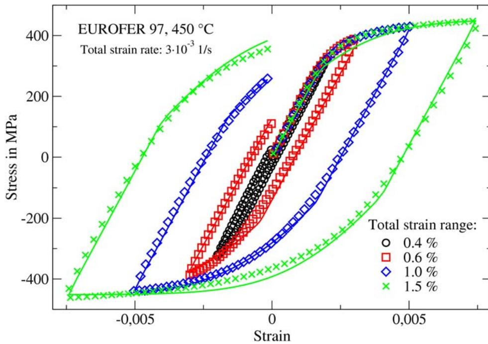
Fig. 4-18 Comparison between material (markers) and model (line) responses for the first stress strain hysteresis of strain controlled LCF tests performed with different total strain ranges
