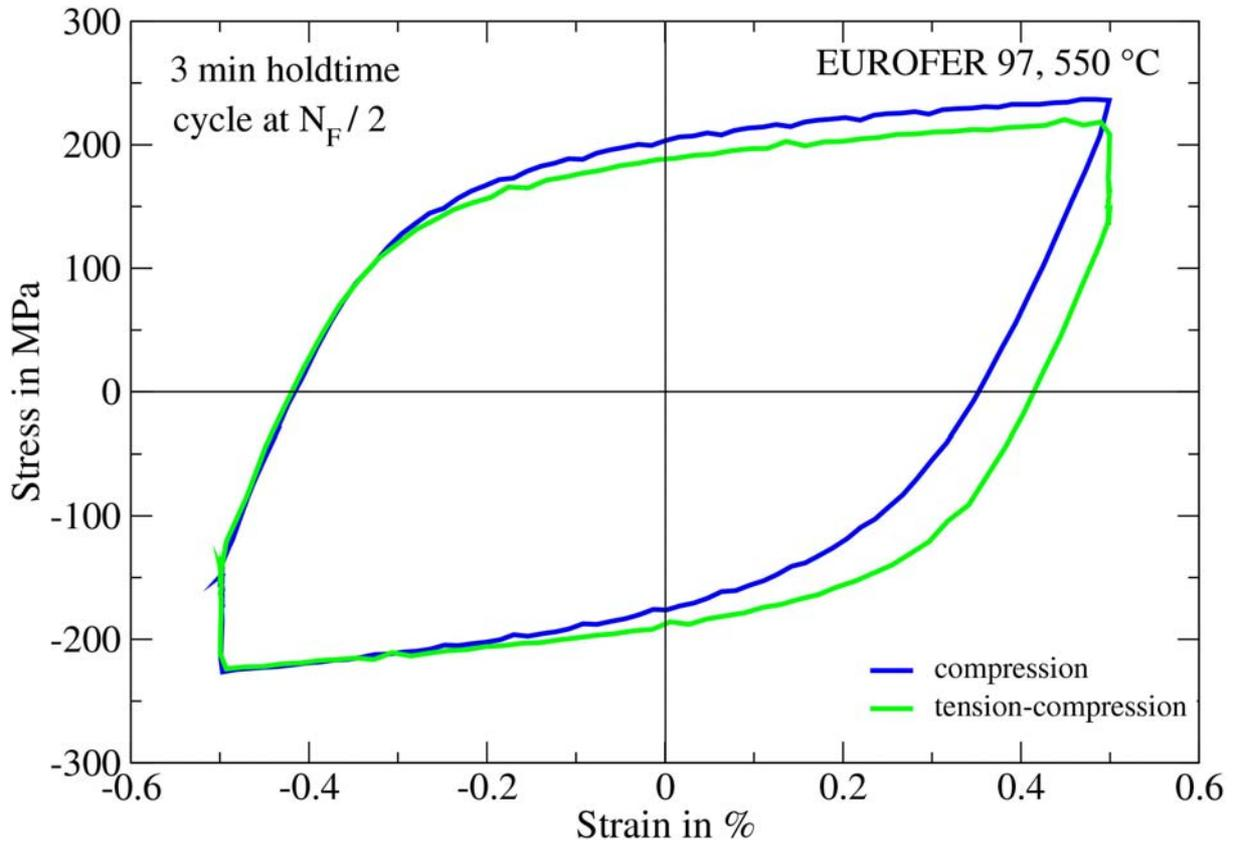
Fig. 2-6 Stress strain hysteresis loops at the half of the lifetime  $N_f / 2$  for the tests with hold time under compression and with hold time under tension and compression, respectively
