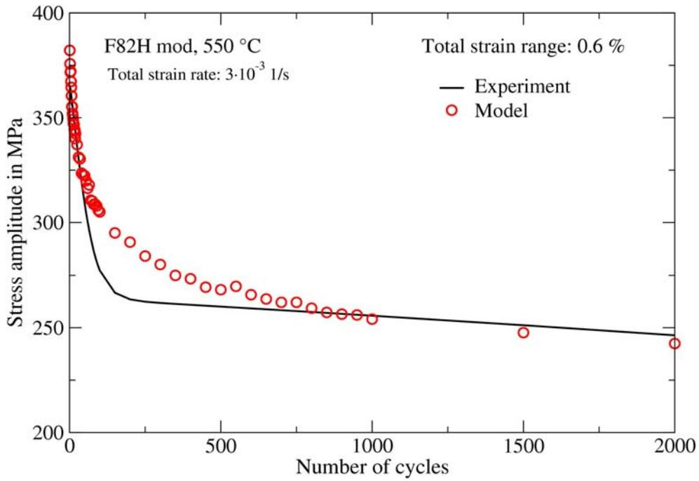
Fig. 4-11 Comparison between material (markers) and model (line) responses for the variation of stress amplitude versus the number of cycles of a strain controlled LCF test
