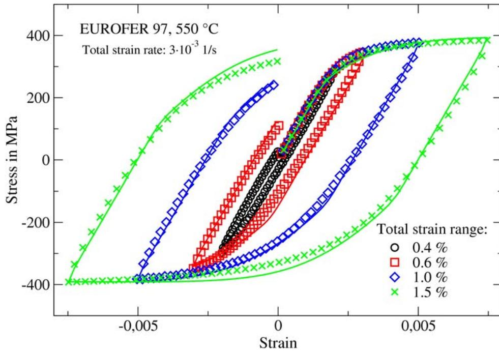
Fig. 4-23 Comparison between material (markers) and model (line) responses for the first stress strain hysteresis of strain controlled LCF tests performed with different total strain ranges
