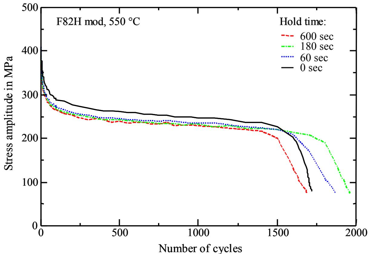
Fig. 2-2 Stress amplitude versus number of cycles for strain controlled LCF tests with different hold times under tension
