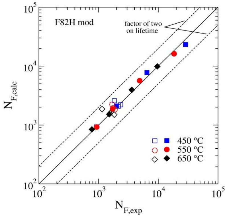
Fig. 4-3 Comparison between numbers of cycles to failure calculated by the coupled deformation damage model with those determined experimentally for F82H mod in LCF tests without (solid symbols) and with hold time (open symbols)
