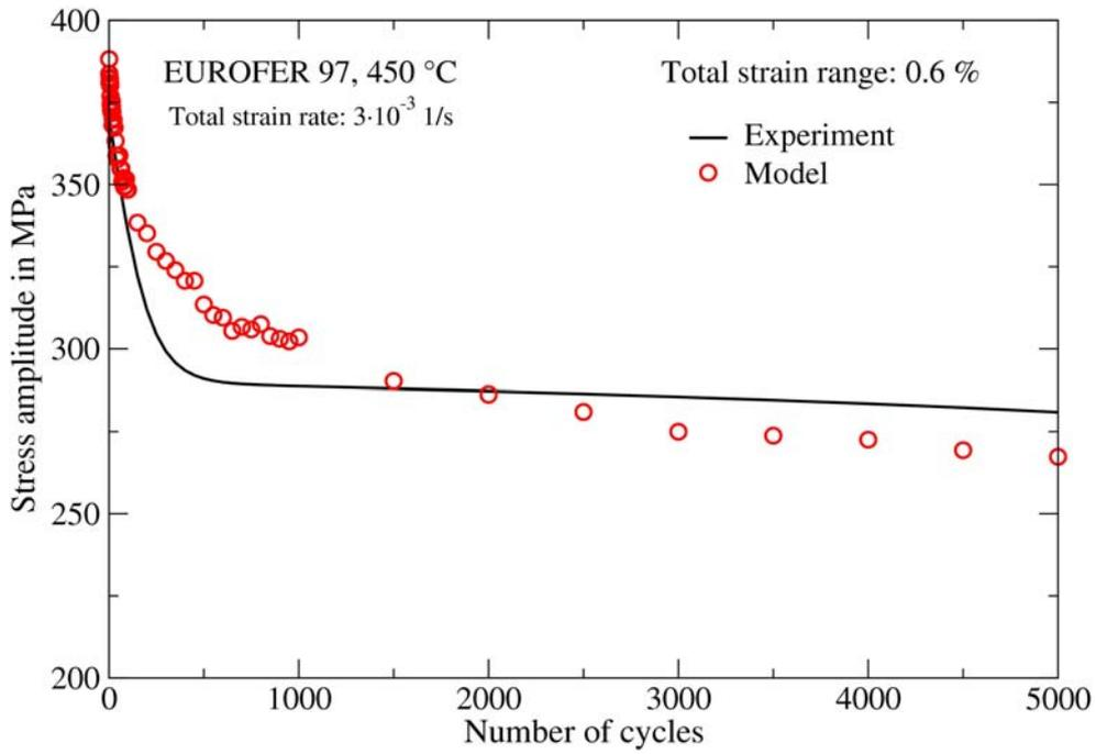
Fig. 4-21 Comparison between material (markers) and model (line) responses for the variation of stress amplitude versus the number of cycles of a strain controlled LCF test
