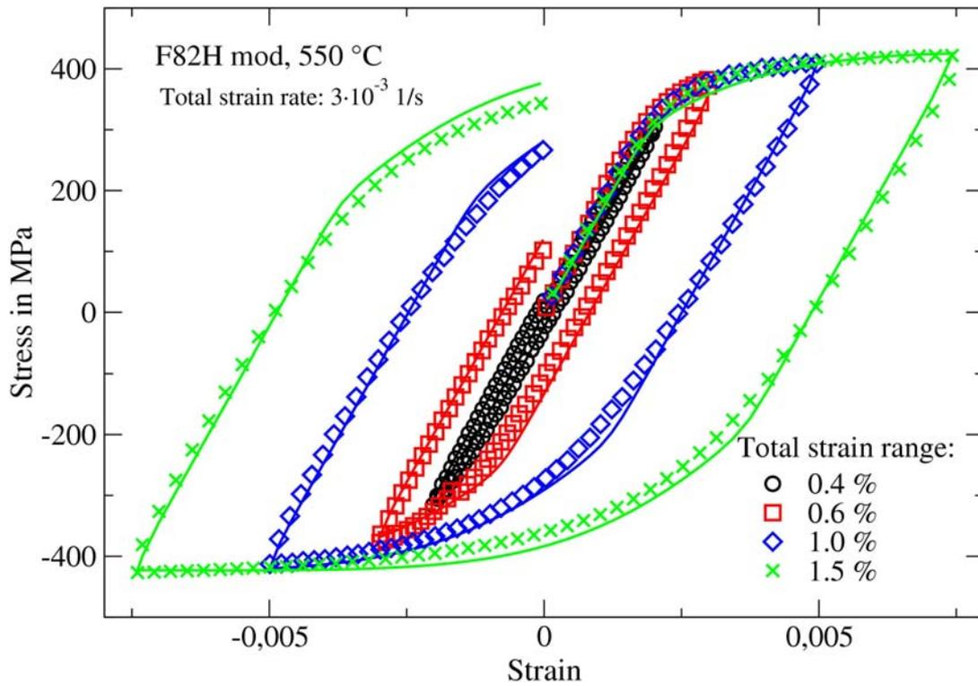
Fig. 4-1 Comparison between material (markers) and model (line) responses for the first stress strain hysteresis of strain controlled LCF tests performed with different total strain ranges
