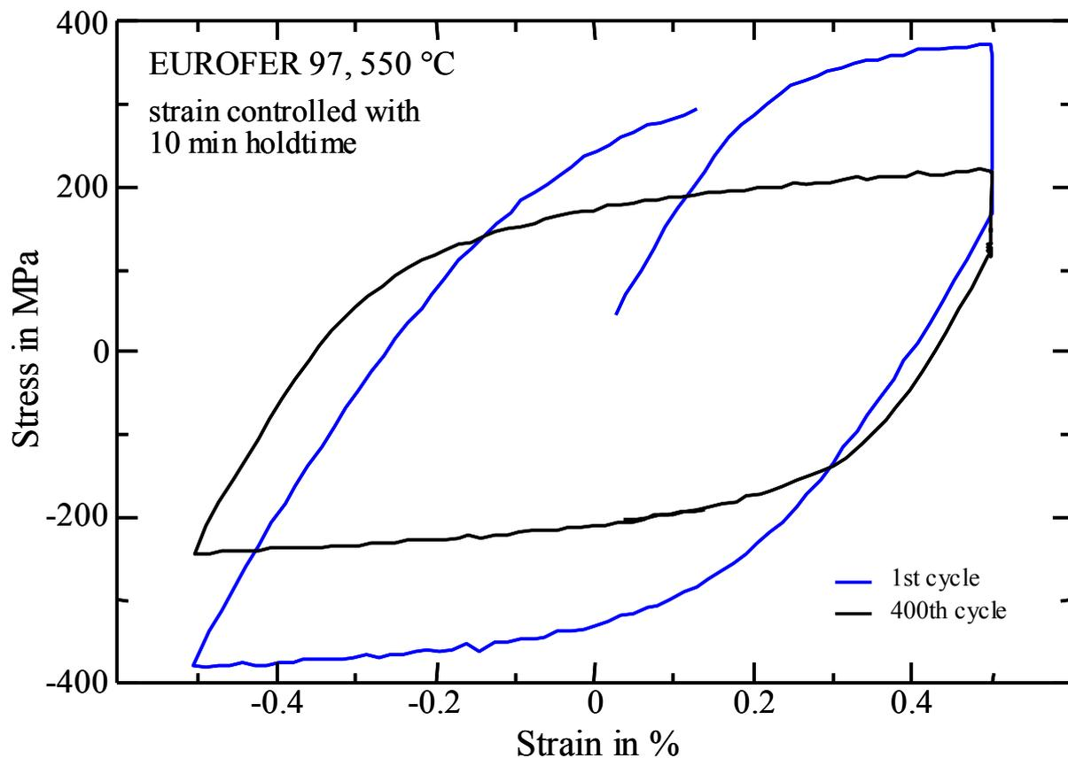
Fig. 2-3 Stress strain hysteresis loops for the 1<sup>st</sup> and 400<sup>th</sup> cycle of a strain controlled LCF tests with hold time under tension. The influence of cyclic softening on the peak stress as well on the stress relaxation and viscosity, respectively, can be noticed.
