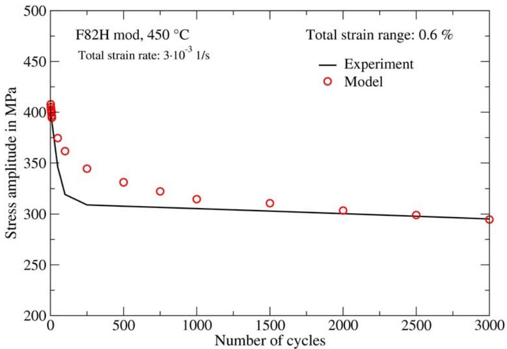
Fig. 4-8 Comparison between material (markers) and model (line) responses for the variation of stress amplitude versus the number of cycles of a strain controlled LCF test
