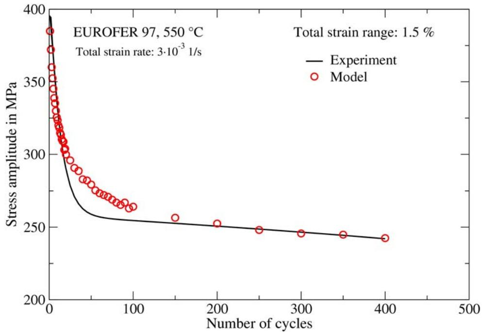
Fig. 4-24 Comparison between material (markers) and model (line) responses for the variation of stress amplitude versus the number of cycles of a strain controlled LCF test
