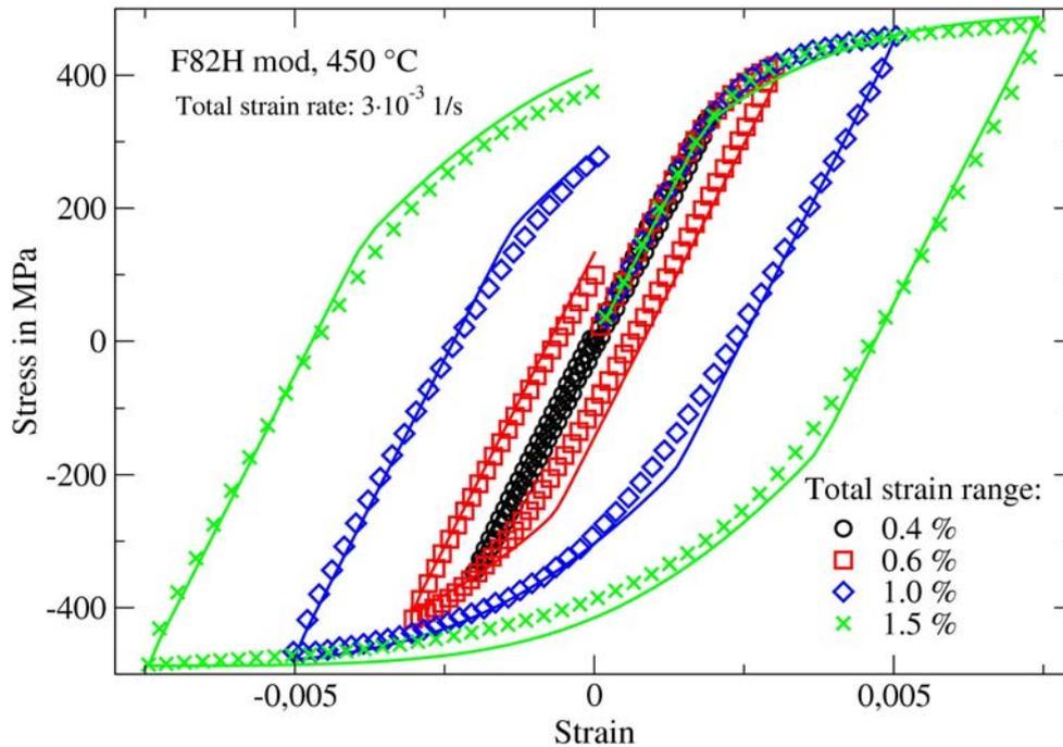
Fig. 4-5 Comparison between material (markers) and model (line) responses for the first stress strain hysteresis of strain controlled LCF tests performed with different total strain ranges
