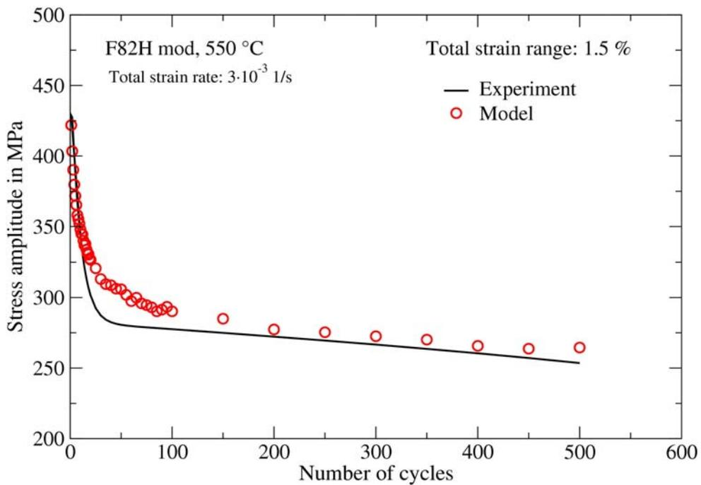
Fig. 4-10 Comparison between material (markers) and model (line) responses for the variation of stress amplitude versus the number of cycles of a strain controlled LCF test
