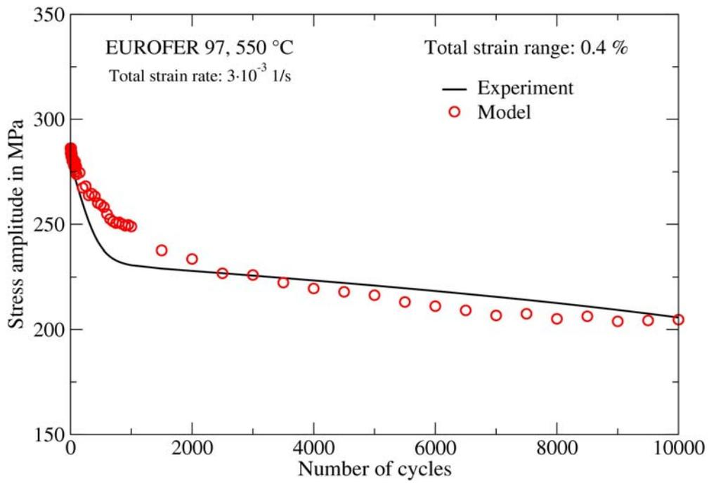
Fig. 4-27 Comparison between material (markers) and model (line) responses for the variation of stress amplitude versus the number of cycles of a strain controlled LCF test
