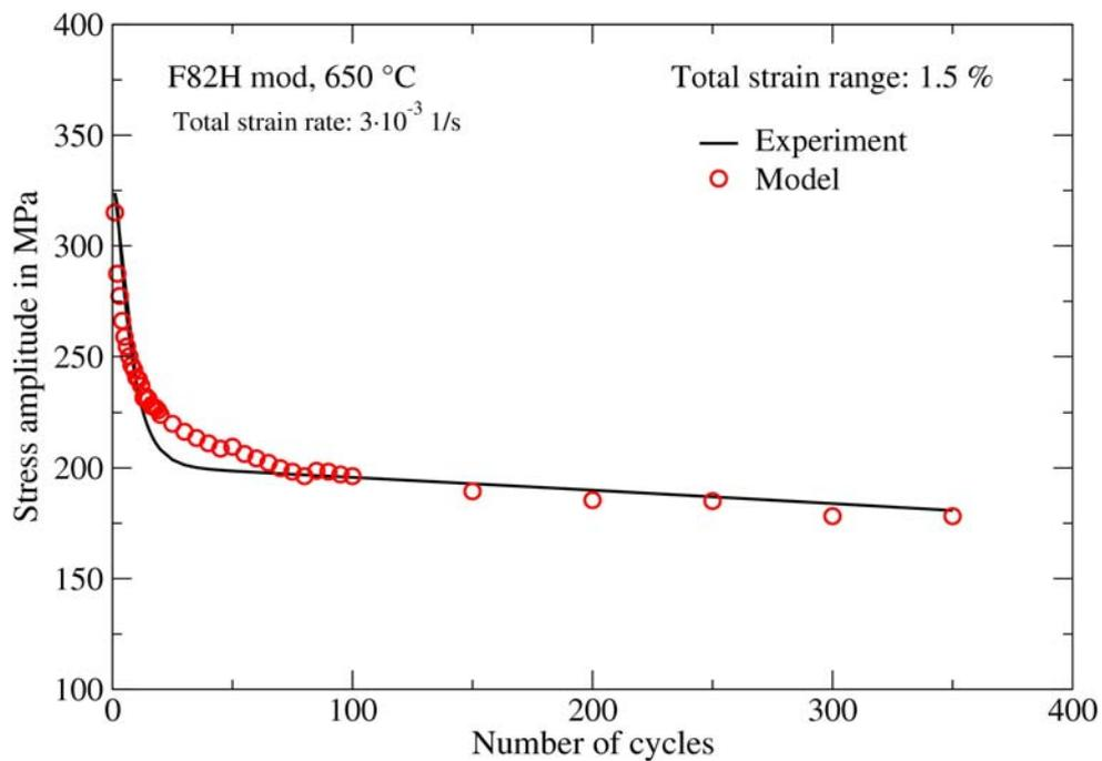
Fig. 4-14 Comparison between material (markers) and model (line) responses for the variation of stress amplitude versus the number of cycles of a strain controlled LCF test
