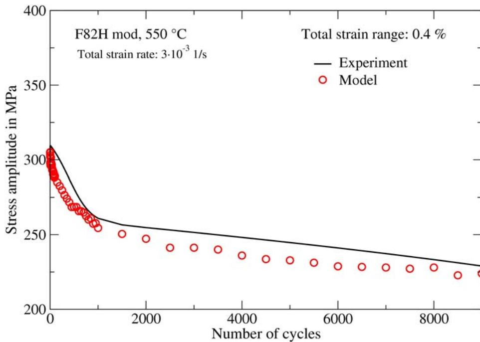
Fig. 4-12 Comparison between material (markers) and model (line) responses for the variation of stress amplitude versus the number of cycles of a strain controlled LCF test
