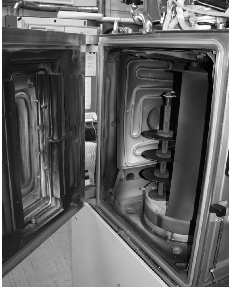
Fig. 1 Magnetron sputtering facility with saw blades to be coated being fixed on a substrate holder.
