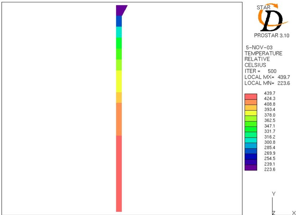
Fig. 11: Temperature distribution in the creep-fatigue test assembly calculated with STAR-CD, Case 8 (design variant with helium guide tube, without nuclear power)
