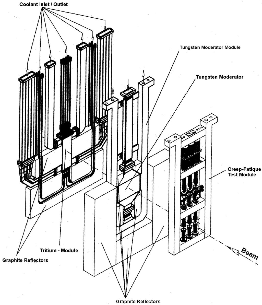
Fig. 1: Exploded view of the submodules of the Medium Flux Test Module
