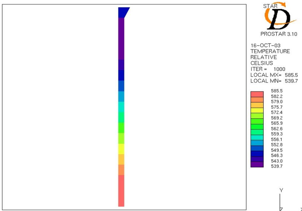
Fig. 9: Temperature distribution in the creep-fatigue test assembly calculated with STAR-CD, Case 6 (design variant with ceramic adapter and electrical power generation in the specimen thread, with nuclear heating)
