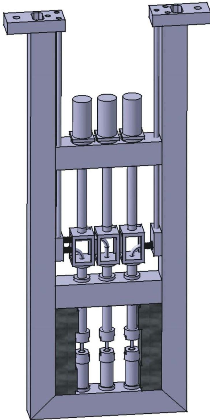
Fig. 2: Submodule with creep-fatigue specimens
