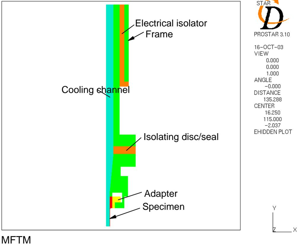
Fig. 4: Model of the thermal-hydraulic simulations using the CFD-Code STAR-CD
