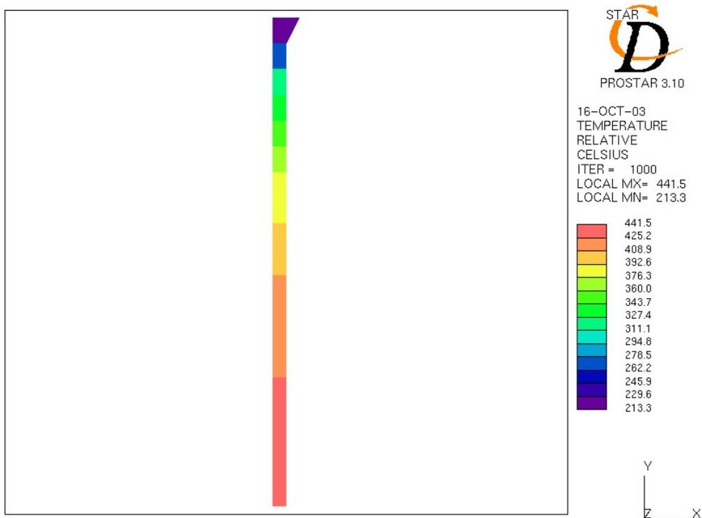
Fig. 7: Temperature distribution in the creep-fatigue test assembly calculated with STAR-CD, Case 2 (reference concept without nuclear power)
