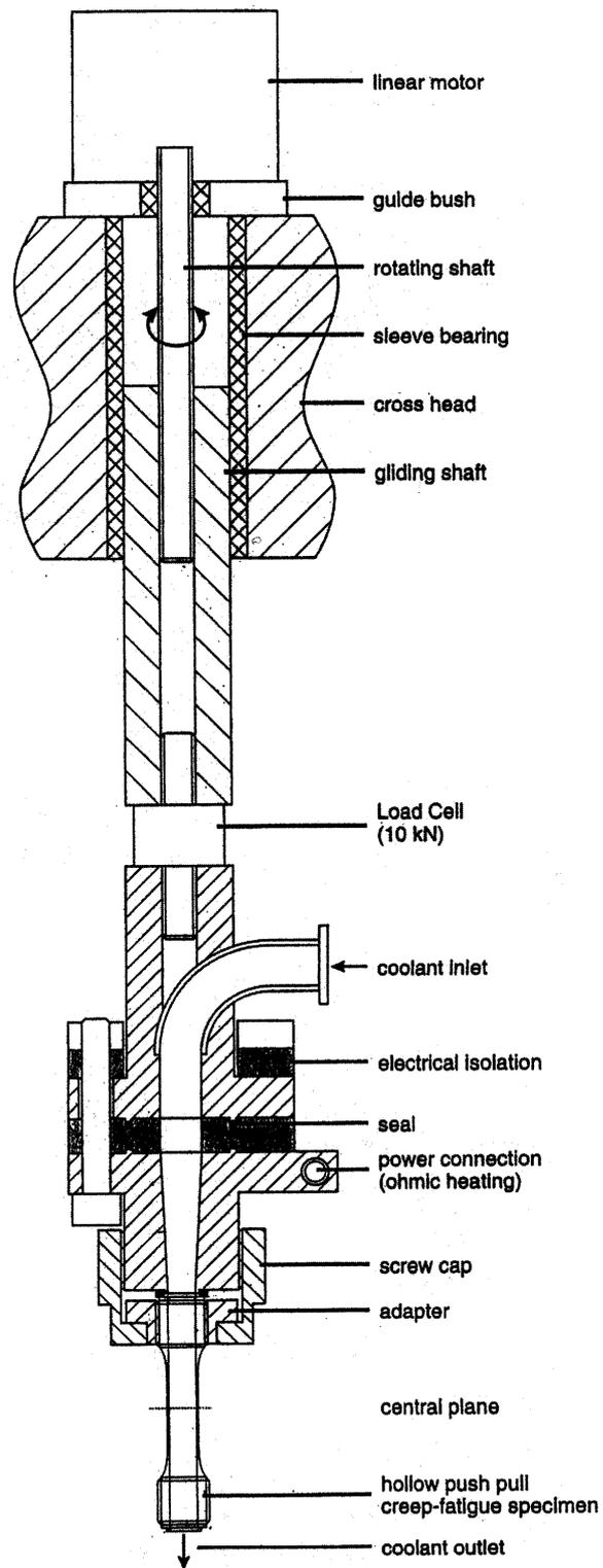
Fig. 3: IFMIF In-situ creep-fatigue experiments - Preliminary design of rod drive
