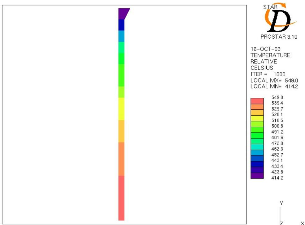
Fig. 6: Temperature distribution in the creep-fatigue test assembly calculated with STAR-CD, Case 1 (reference concept, with nuclear power)
