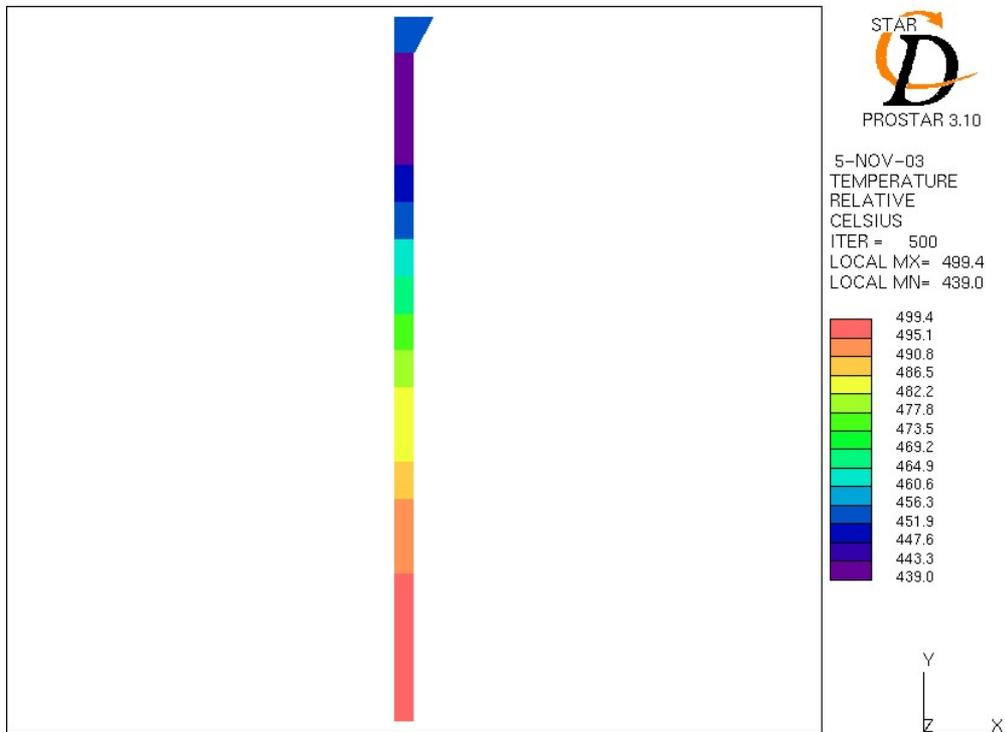
Fig. 10: Temperature distribution in the creep-fatigue test assembly calculated with STAR-CD, Case 7 (design variant with helium guide tube, with nuclear power)
