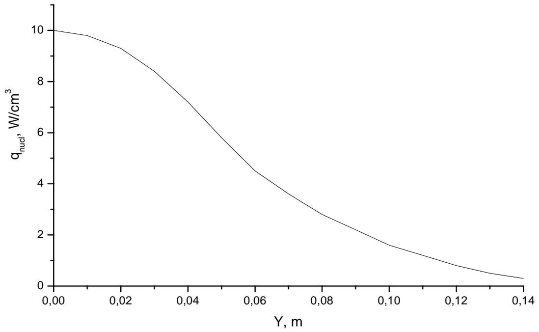
Fig. 5: Nuclear power density in steel along the axis of the central creep-fatigue specimen (extrapolated from data of the HFTM)
