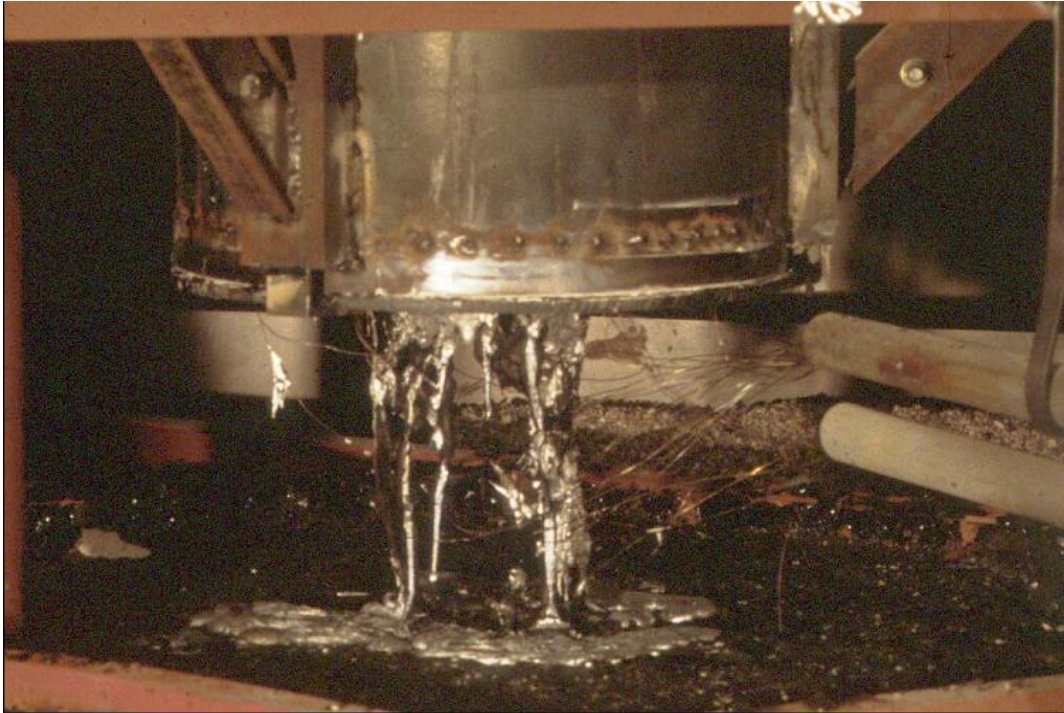
Figure 74: Photo of the test container after the test in KAPOOL 17
