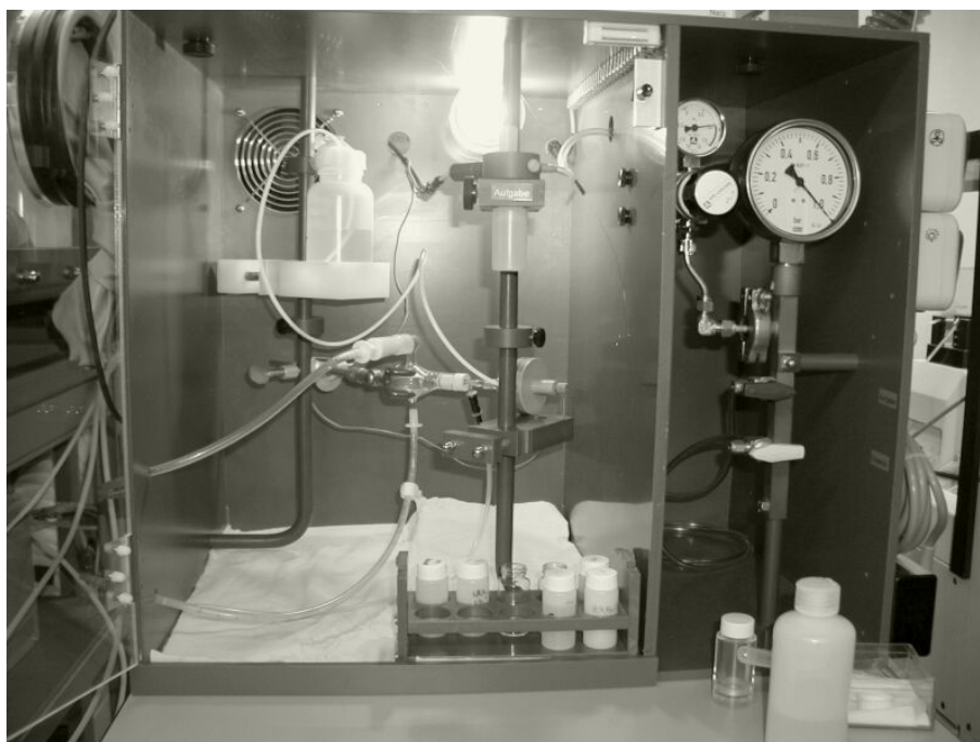
Fig. 1: Photo of the experimental set-up for the coupling of CE to ICP-MS
