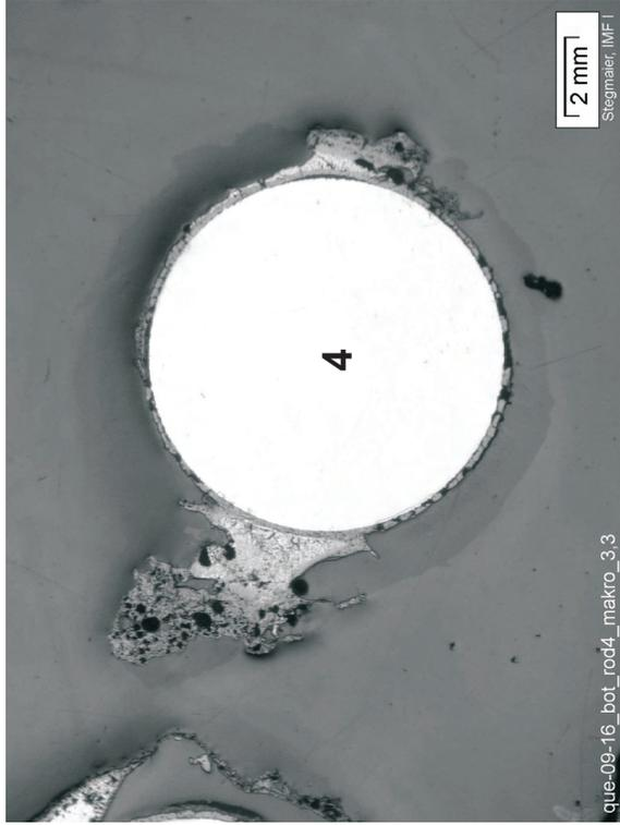
Rod #4, showing advanced oxidation of residual melt
