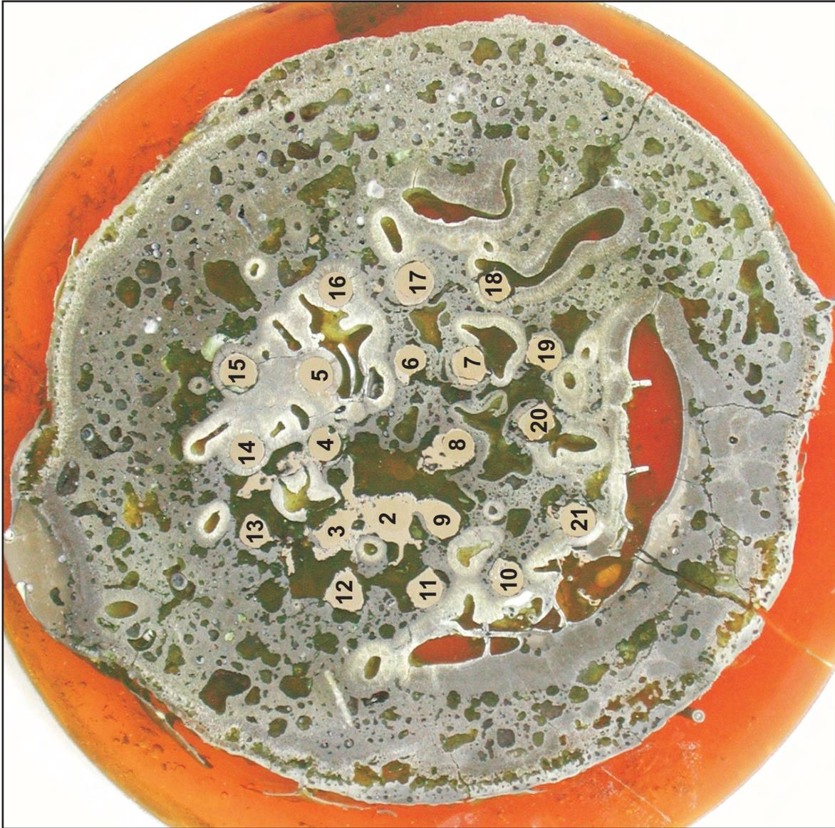
Fig. 56: QUENCH-09; Cross section at 590 mm bundle elevation (QUE-09-4); overview from top
