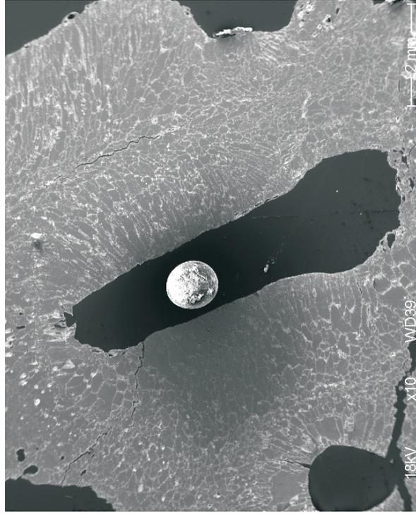
Fig. 97: QUENCH-09; Cross section at 590 mm elevation (QUE-09-4); non-porous melt pool, penetrated by steam flow channels, after complete conversion to ceramic state by pool oxidation mechanism; no control rod components detected in SEM/EDX analysis
