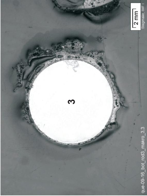
Rod #3, showing advanced oxidation and melting of the partly present cladding
