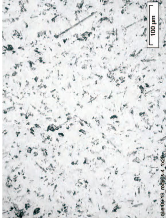
Fig. 49: QUENCH-09; Cross section at 460 mm bundle elevation (QUE-09-18); small melt lumps
