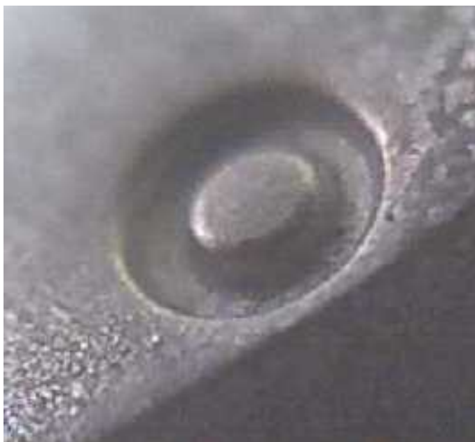
Fig. 4.1-10: Tungsten gaps (a-filled by copper, b- after etching).
