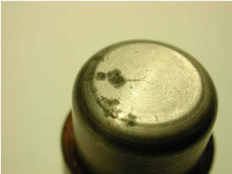
Fig. 4.5-5: Cracking of the WL-10 thimble after thermocycling.
