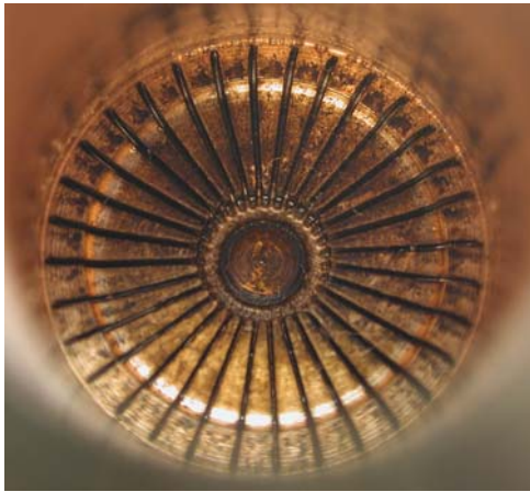
Fig. 3.1-1: EDM of HEMS mock-ups from CuCrZr for GPF experiments.
