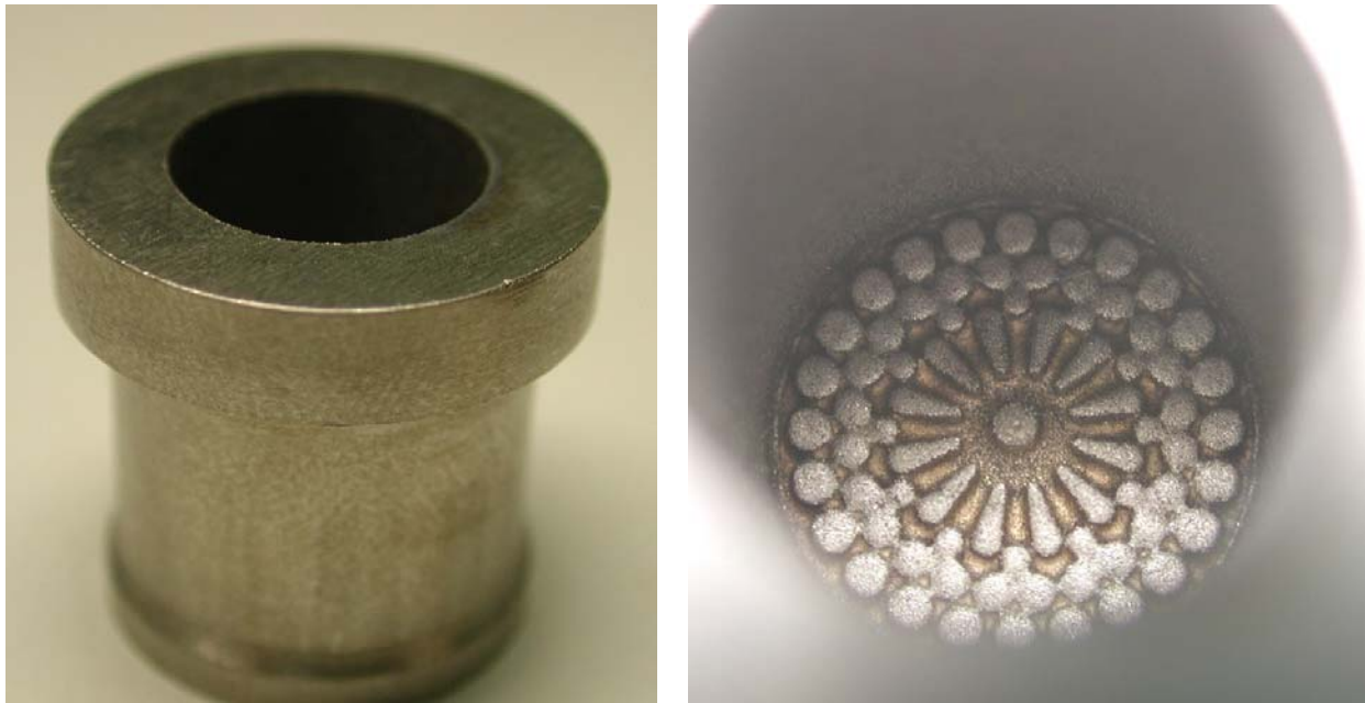
Fig. 4.1-4: Tungsten thimble with pin array structure, fabricated by EDM.
