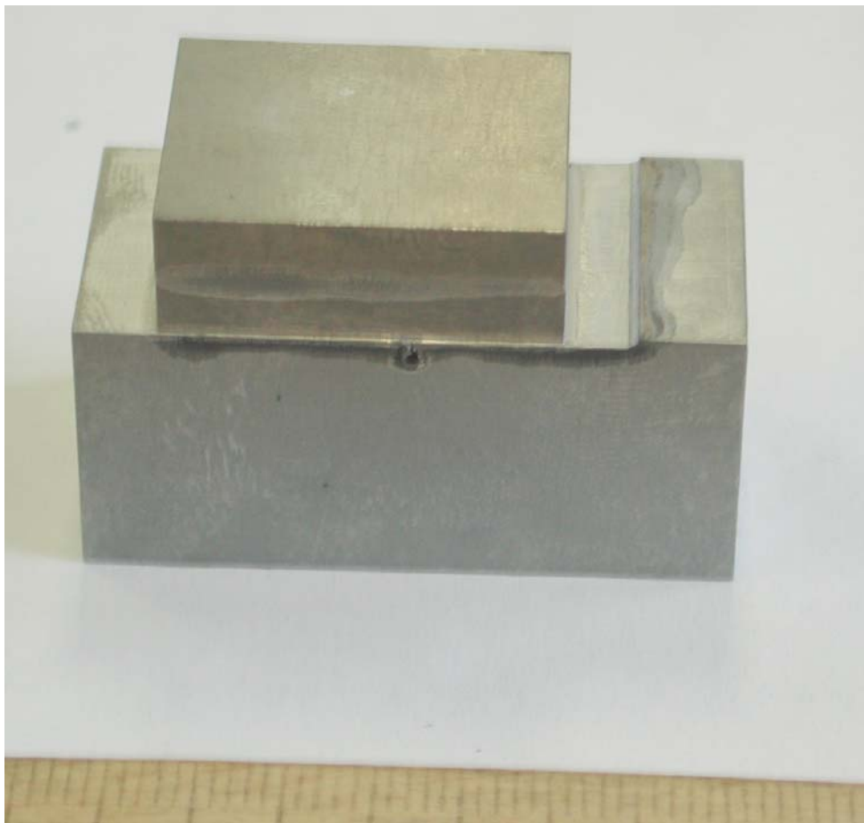
Fig. 4.4-6: Mock-up brazed with 71KHCP filler metal.
