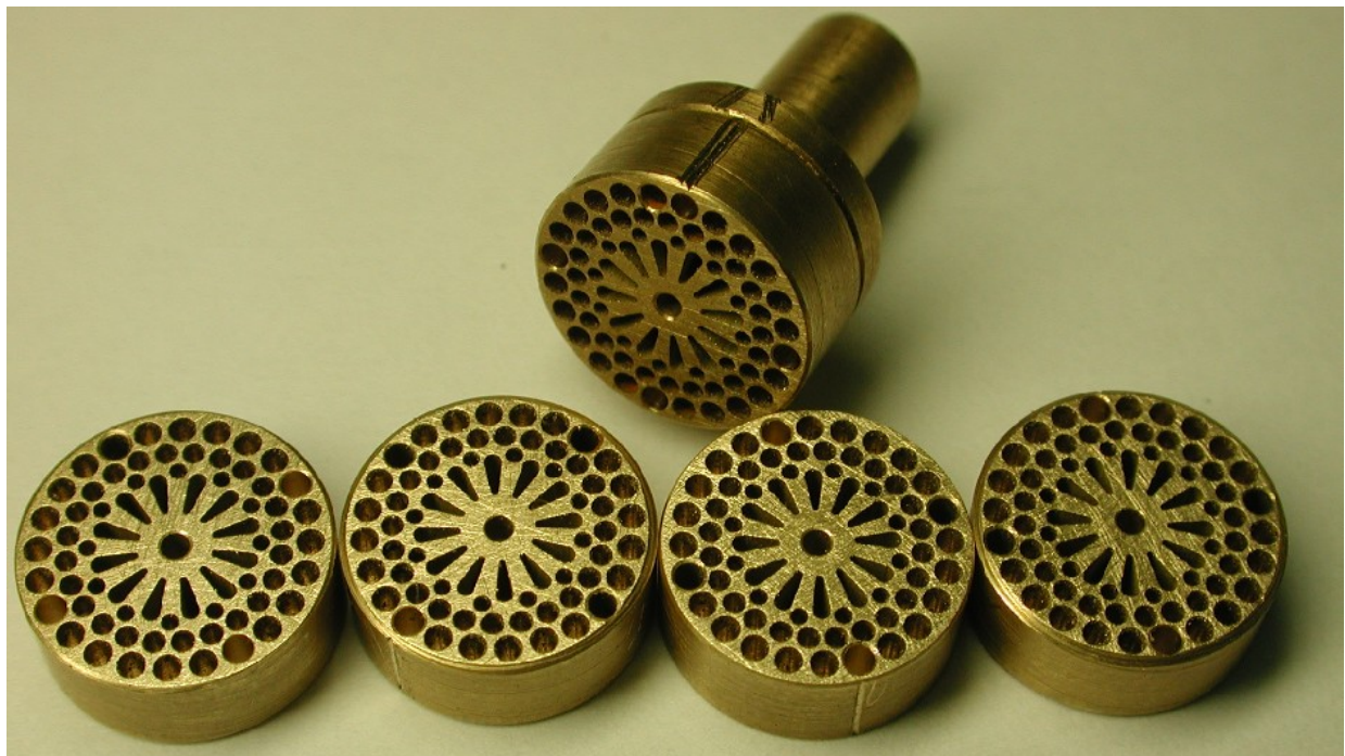
Fig. 4.1-2: Electrodes for the EDM of the FZK pin array design.
