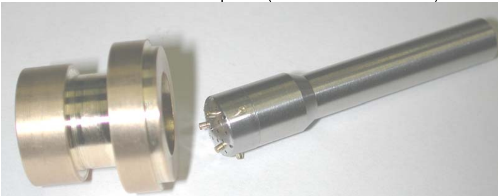
Fig. 3.1-2: HEMJ cartridges and spacers for the second GPF test campaign.
