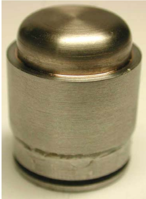
Fig. 4.5-6: Mock-up with a W-Cu thimble.
