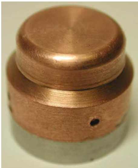
Fig. 4.5-7: Mock-up with CVD tungsten (Cu-steel structure before W-coating deposition).
