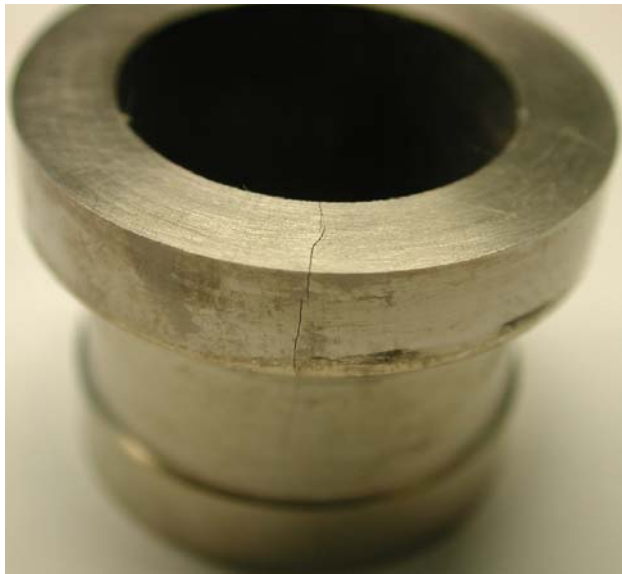
Fig. 4.1-9: Cracks in the tungsten thimble.
