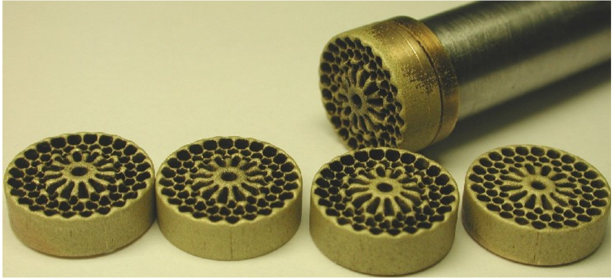
Fig. 4.1-5: The view of the electrodes after EDM.
