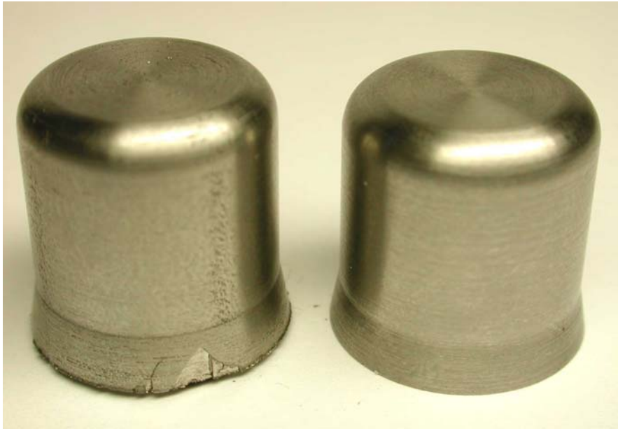
Fig. 3.3-1: SC (left) and lanthanated (right) tungsten after machining.
